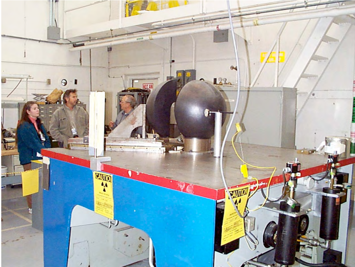
Figure 14.4. “Flattop” criticality assembly apparatus at TA-18.
