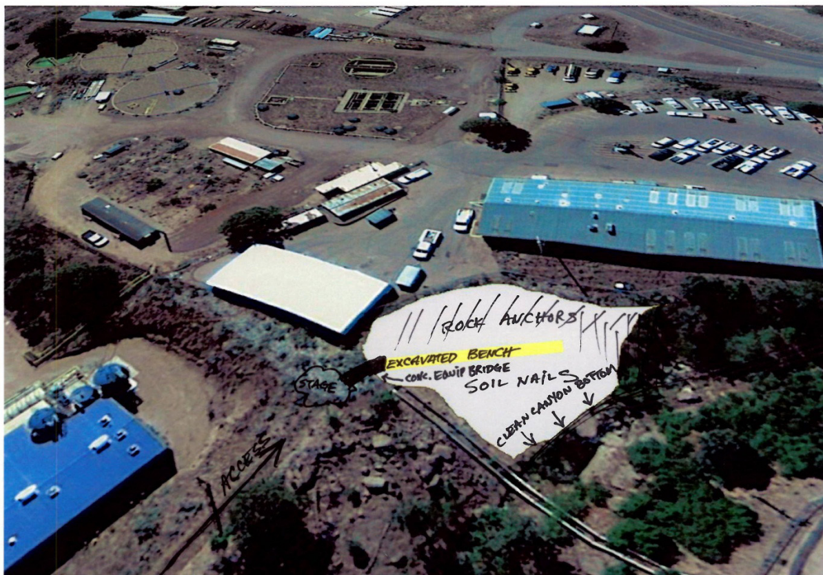
Figure 11 No exposure shotcrete option at Site 03-056(c)
