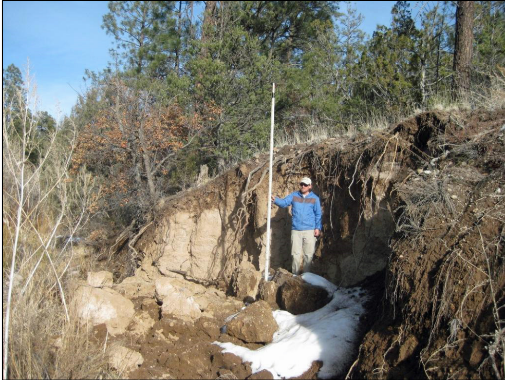
Photo A1-3 February 2015 photograph of lateral bank migration and northward stream channel migration in the area of maximum sediment erosion and maximum sediment deposition at cross-section UPW-6, looking downstream
