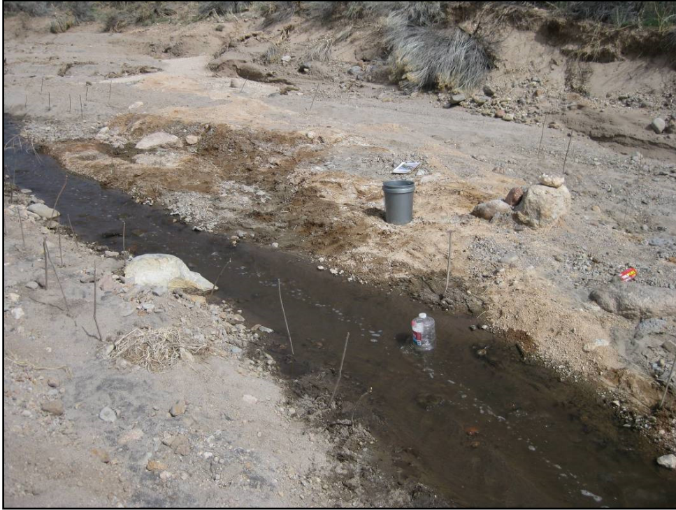
Figure B-2.2-5 Tertiary Puye Formation bedrock exposed in Bank 2 at the surface causing refusal. Tertiary Puye Formation bedrock also present in Bank 1, April 17, 2014
