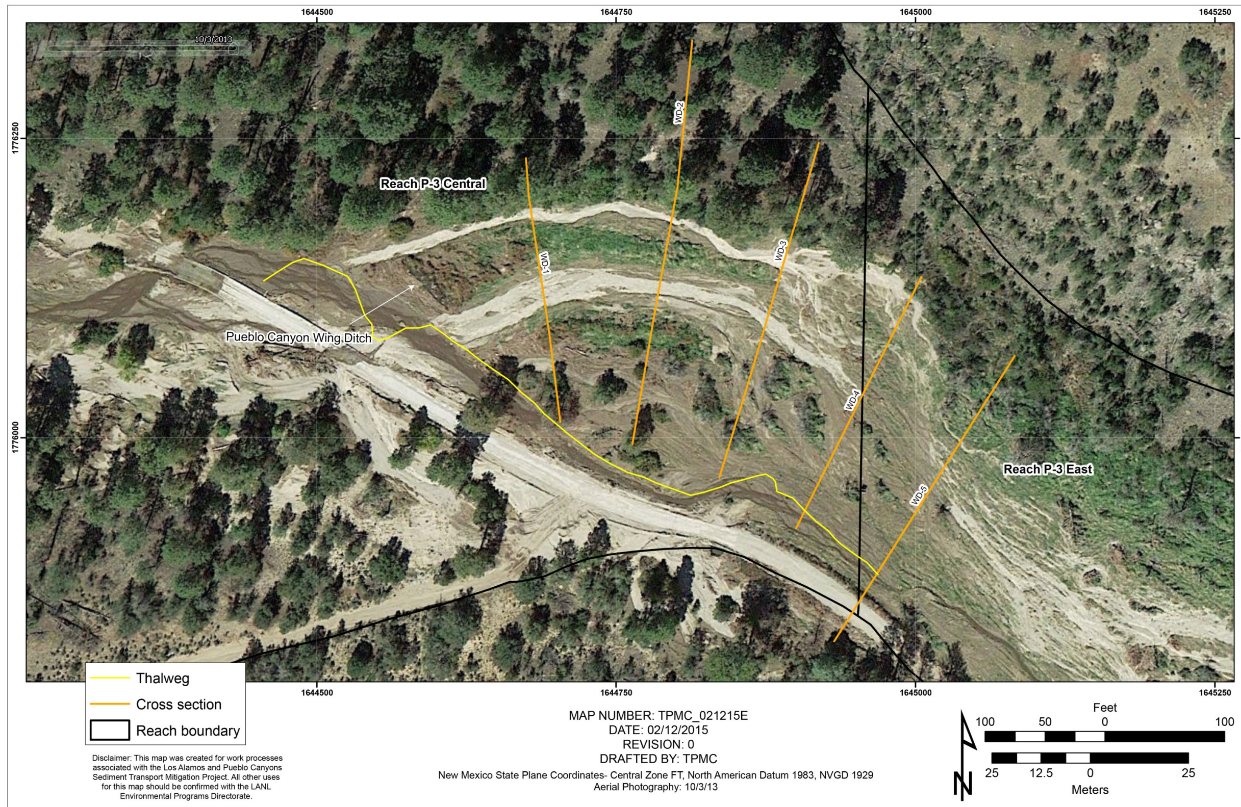
Figure A-3.3-1 Orthophoto showing the locations of surveyed cross-sections and thalweg profiles near the Pueblo Canyon wing ditch
