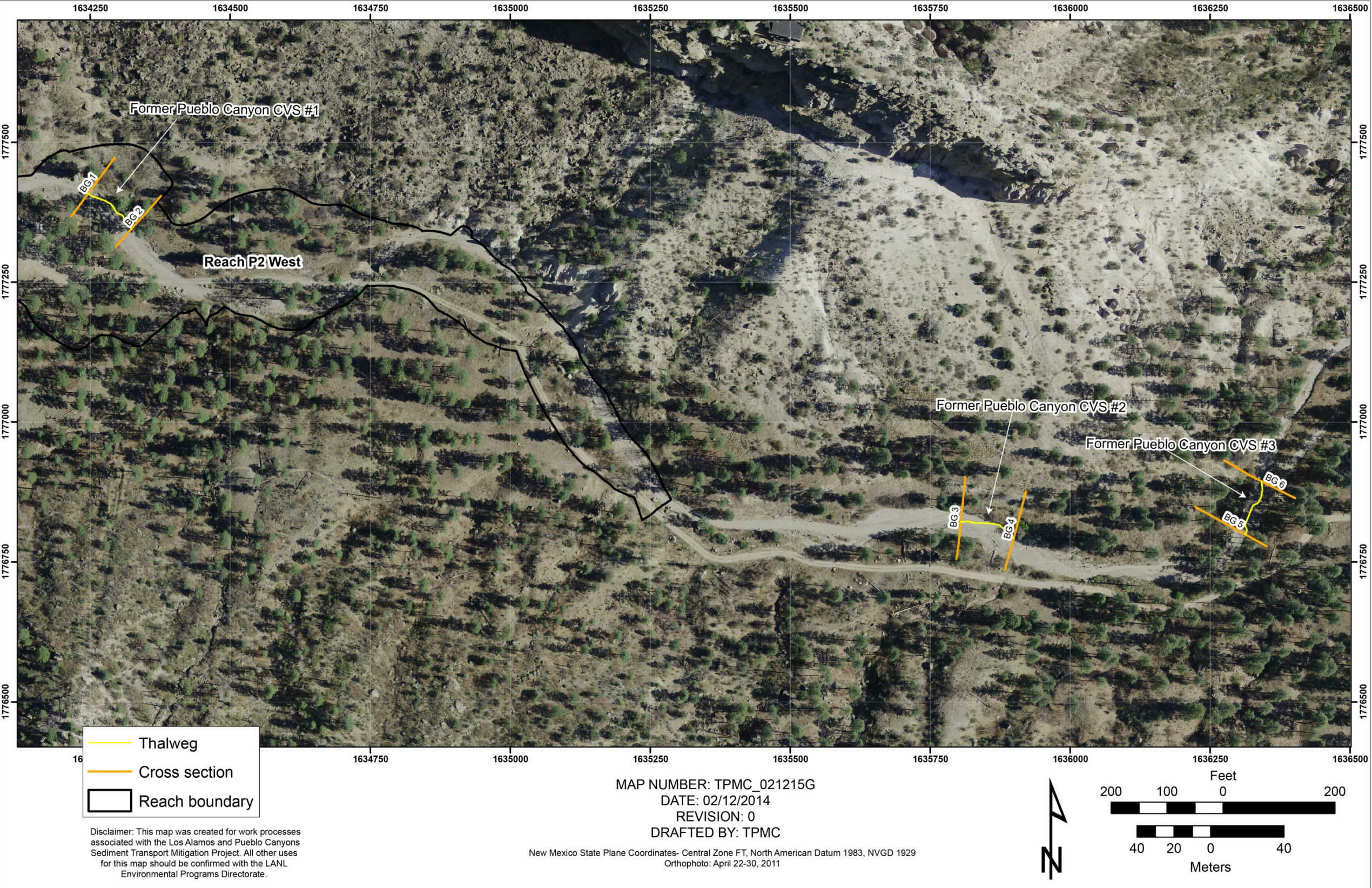
Figure A-3.1-1 Orthophoto showing the locations of surveyed cross-sections and thalweg profiles at the Pueblo Canyon Background sections above the WWTF
