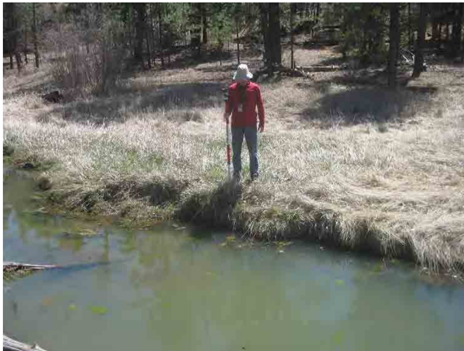
Photo A1-21 Erosion (~1.0 ft) of bank materials detected in area of well-defined channel directly upstream of DP Canyon GCS: (a) looking north at left bank and (b) looking south at right bank
