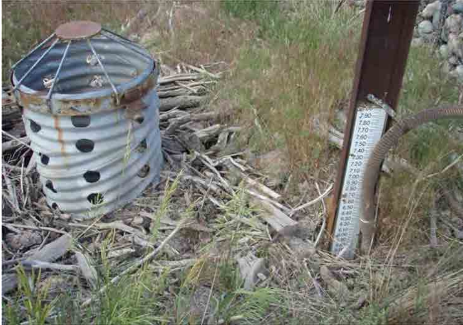
Photo C-4.1-2 June 2016 — Standpipe is unobstructed for top four holes. Staff gage reads 5.7 ft.
