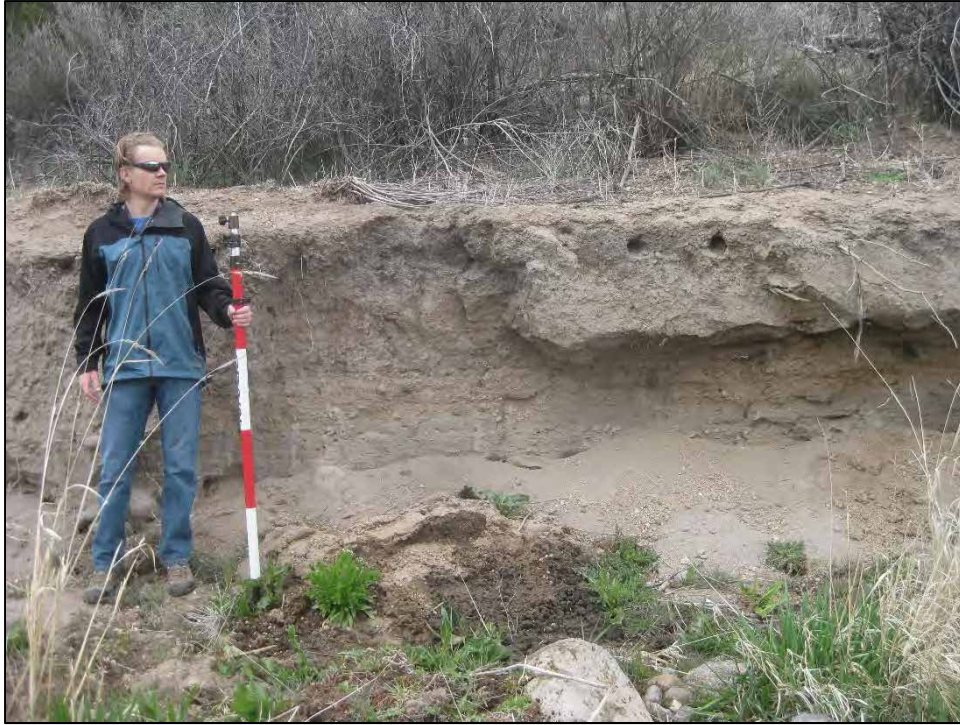
Photo A1-12 Detected change (+2.1 ft) from collapse of channel bank sediments in Pueblo Canyon lower willow planting area, looking north
