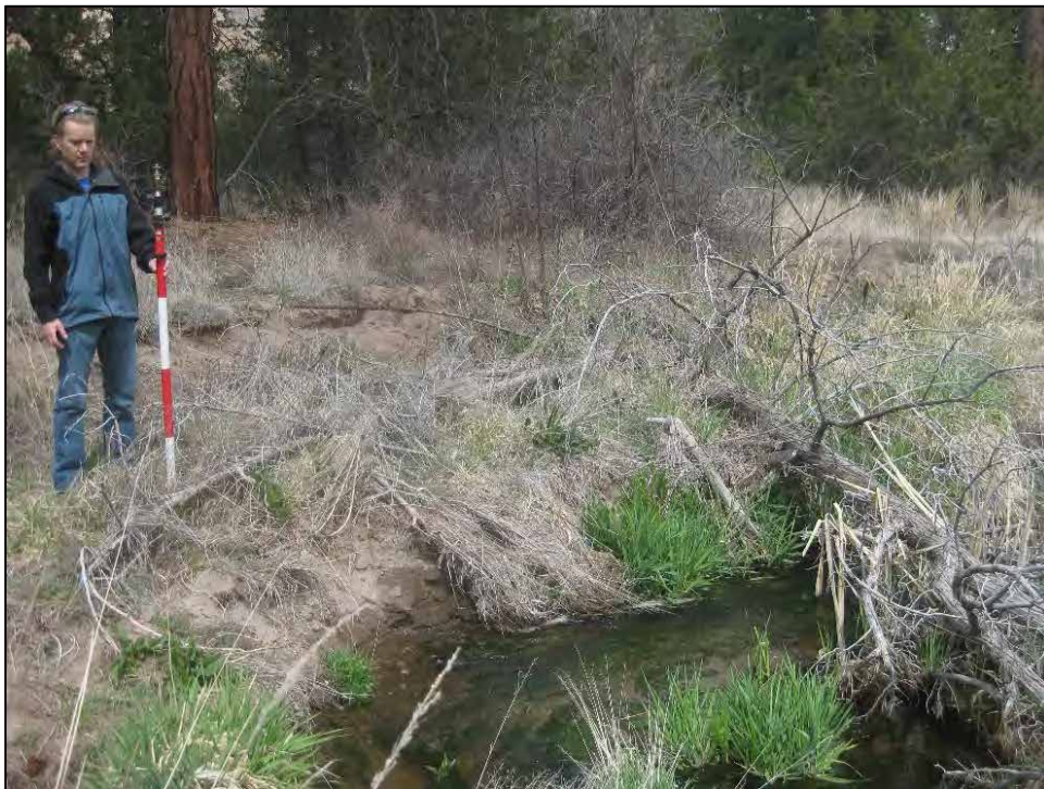
Photo A1-9 Detected erosion (~1.9 ft) on active channel banks at upstream area of wing ditch, looking northeast
