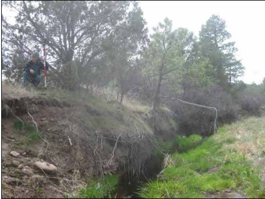
Photo A1-6 Detected geomorphic change near stream gage E059.5 in the Pueblo Canyon upper willow planting area, looking west. Geomorphic change at this location is characterized by the slumping/creeping of unconsolidated sediment and boulders that comprise the channel bank. No channel process change is observed.
