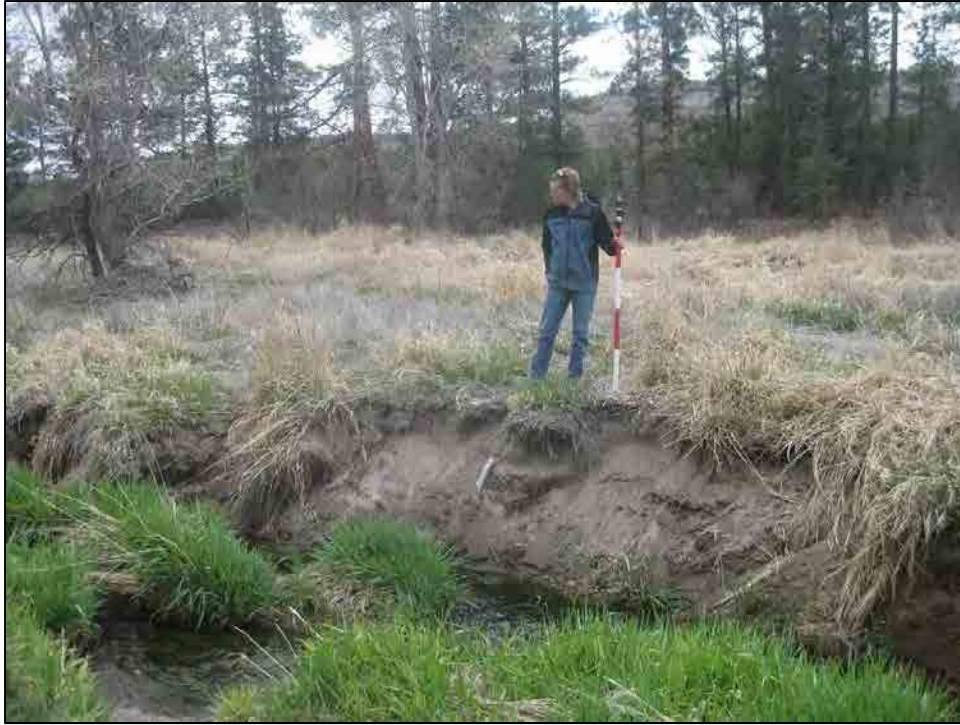
Photo A1-8 Detected erosion (~2.39 ft) on active channel banks at upstream area of wing ditch, looking south
