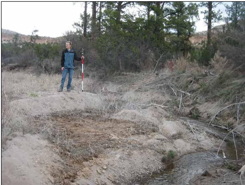
Photo A1-13 Lateral channel migration and incision (-1.26 ft) detected near the western edge of reach P-4 Central in Pueblo Canyon grade-control structure (GCS) area, looking northwest
