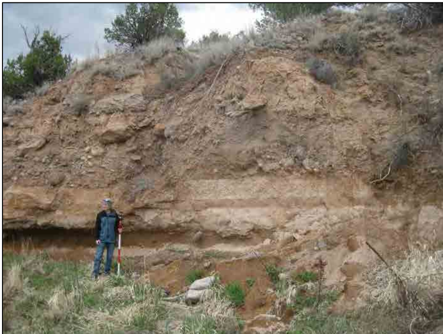
Photo A1-5 Maximum negative elevation change (-11.3 ft) Pueblo Canyon upper willow planting area, looking east. Loss of overhanging slope sediments and rocks resulted in large magnitude of elevation change detected on this bank. Actual volume change of observed sediments at the base of the bank is minor.
