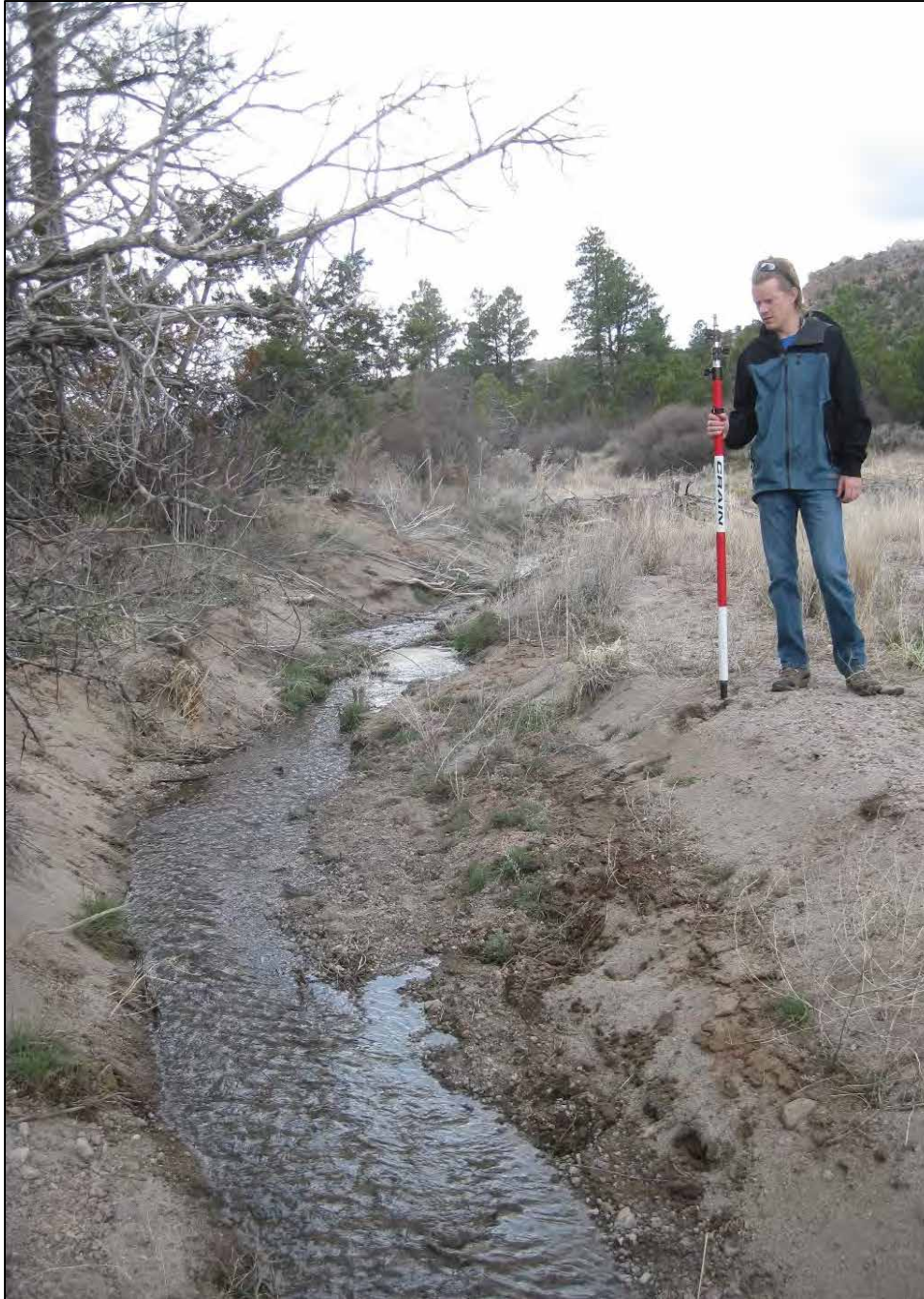
Photo A1-14 Channel incision (~1.26 ft) detected near the western edge of reach P-4 Central in Pueblo Canyon GCS area, looking east
