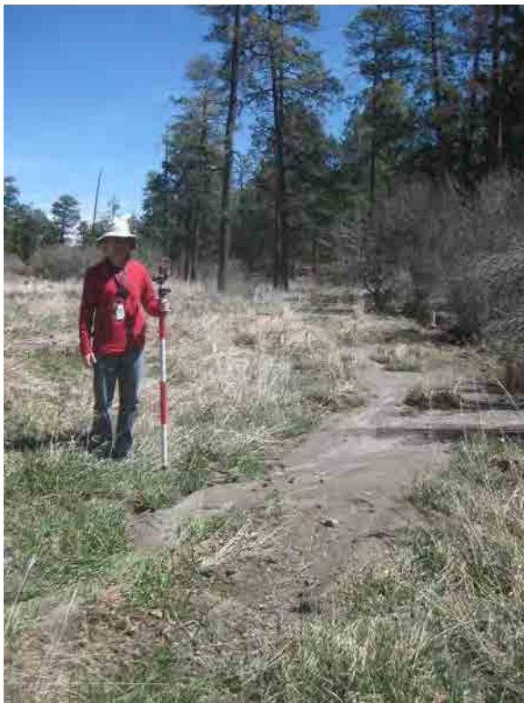
Photo A1-20 Deposition (+1.21 ft) of channel fill materials detected in area of braided channels above DP Canyon GCS, looking east
