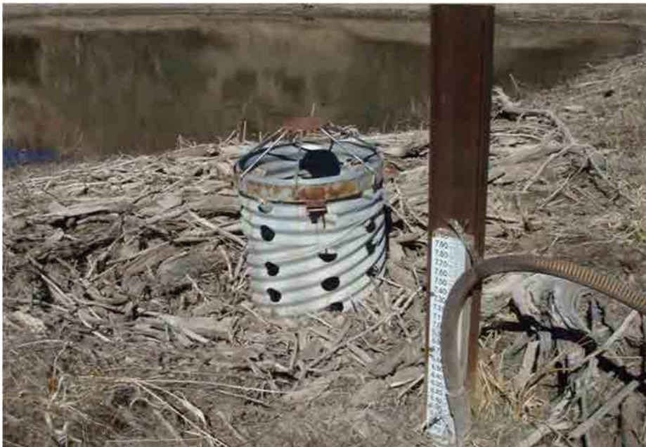
Photo C-4.1-1 March 2016 — Standpipe is unobstructed for top four holes, five holes buried. Staff gage reads 5.7 ft.
