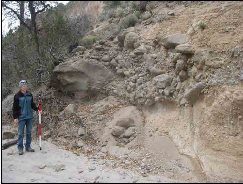
Photo A1-2 Additional area of detected change (-5.5 ft) in Pueblo Canyon background area, looking northwest. Channel banks are eroding via rock/soil fall into the main channel.
