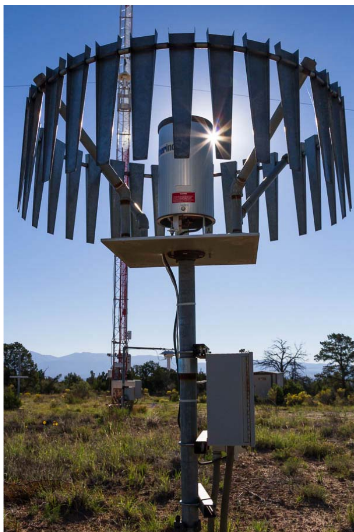
TA-53 Precipitation gage (foreground) and meteorological tower (background)
