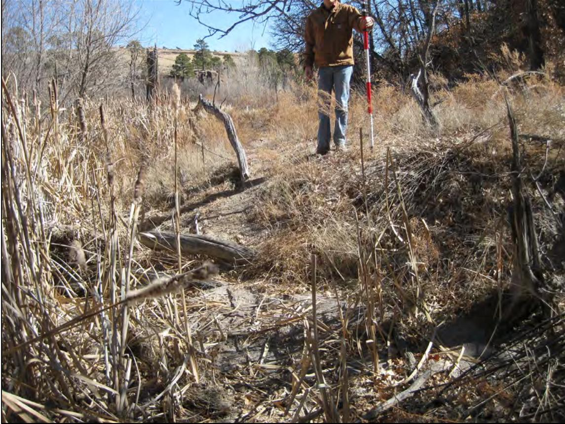
**Photo B1-2** Example of bank survey interpretation of break in slope. No evidence of erosion based on field check. February 2017 photo looking northeast.
