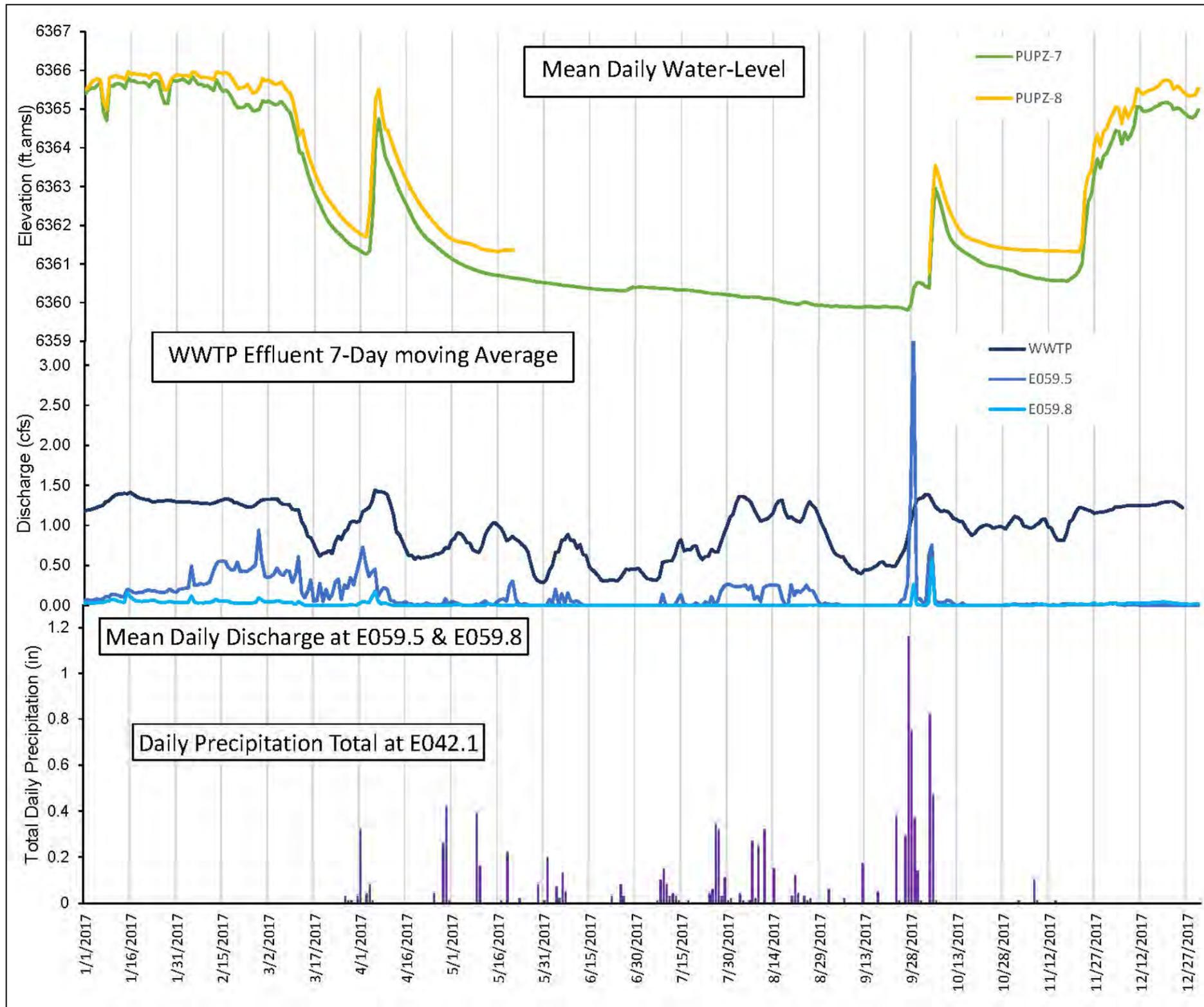
Figure B-2.0-3 Mean daily water level (ft amsl) in piezometers PUPZ-7 and PUPZ-8; 7-d moving average of Los Alamos WWTP effluent discharge; mean daily discharge at gaging stations E059.5 and E059.8; and total daily precipitation at E042.1
