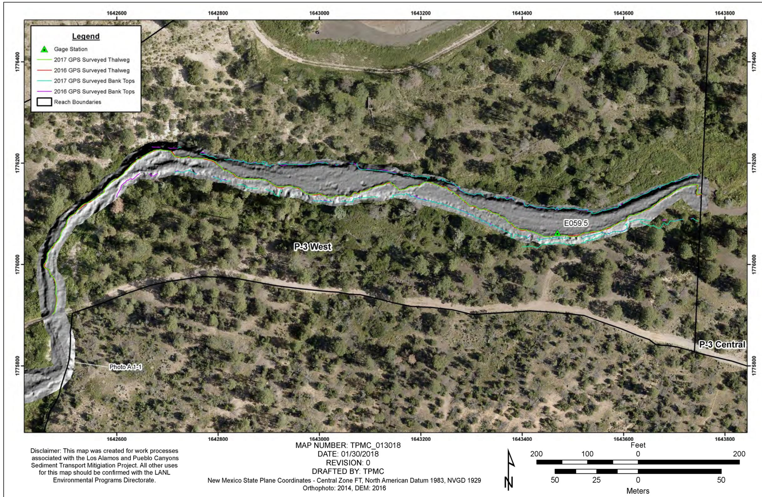
Figure A-4.2-1 2014 orthophoto with 2016 hillshade DEM and 2016 versus 2017 surveyed channel banks and thalweg at the Pueblo Canyon upper willow planting area
