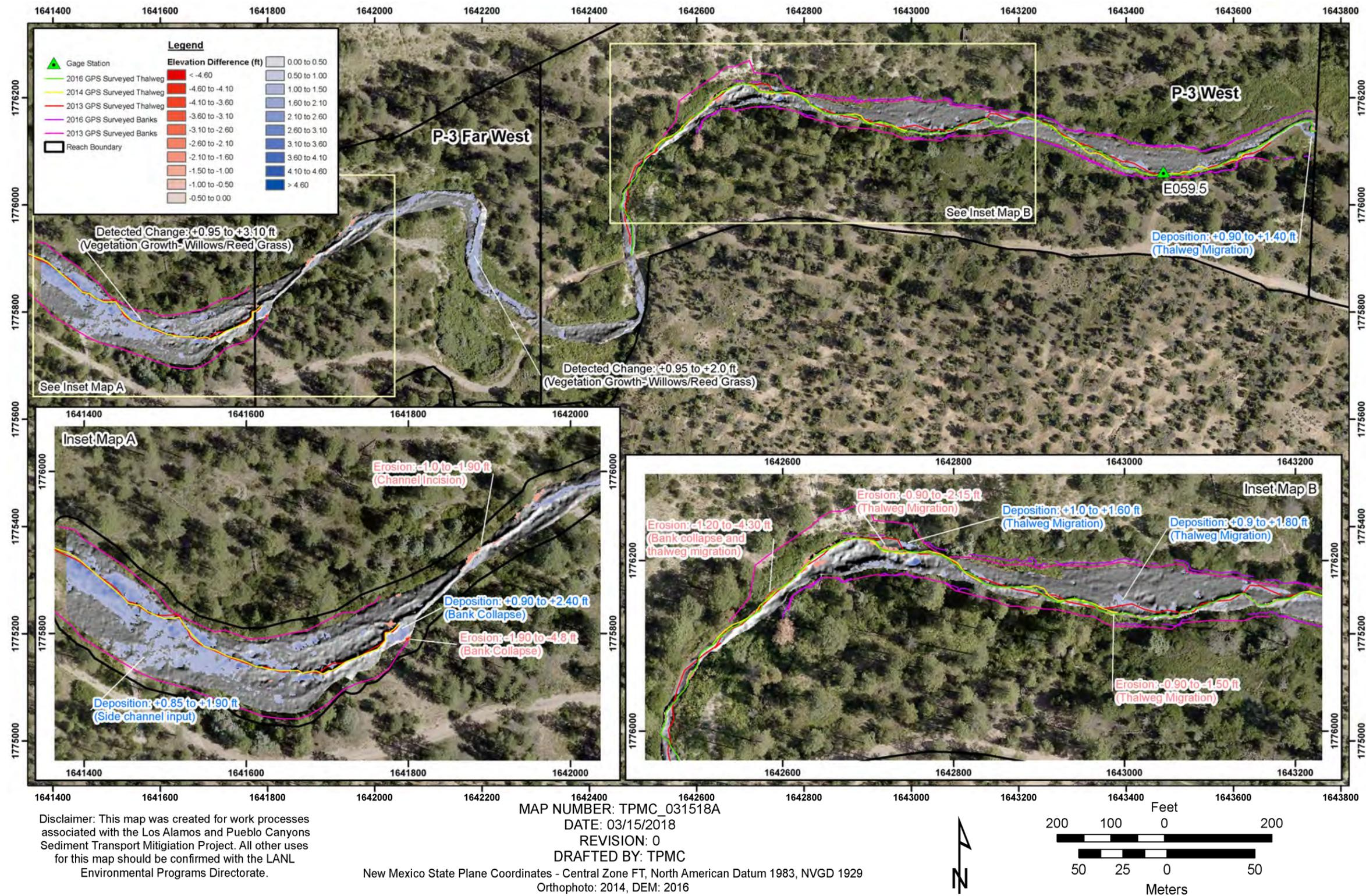
Figure A3-3.1-2 2014 orthophoto with 2016 hillshade DEM and 2014 to 2016 GCD results at the Upper Pueblo Canyon Willow Planting Monitoring Area. FIS calibration was based on observable changes between DEMs.
