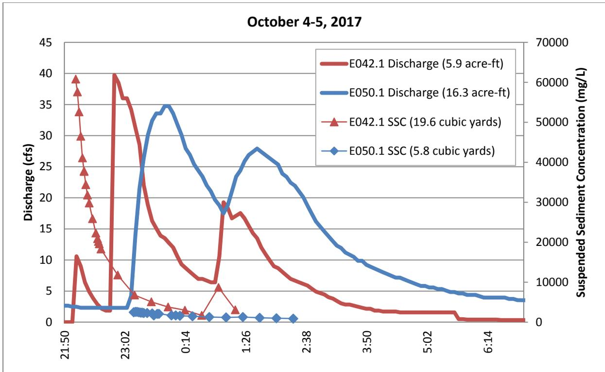
Figure 3.4-3 (continued) Discharge and SSC at E042.1 and E050.1 in upper Los Alamos Canyon on days when sampling of the same runoff event occurred
