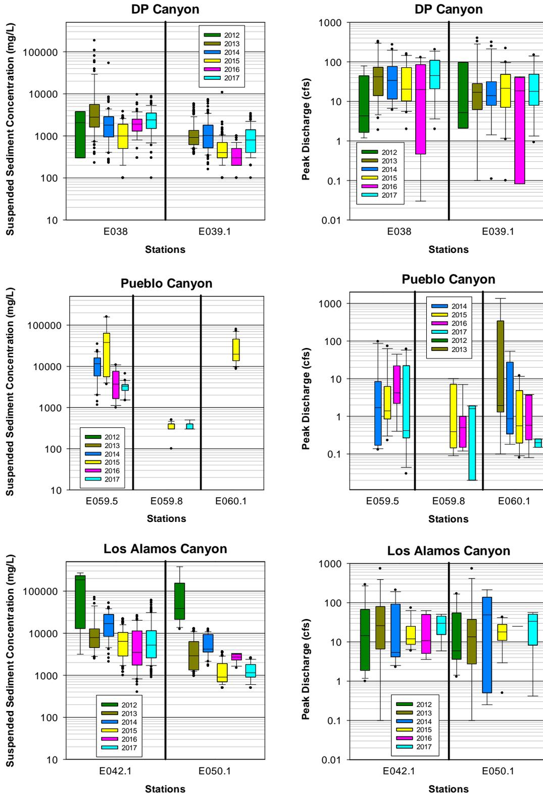
**Figure 3.4-1** Box-and-whisker plots of SSC (left) and peak discharge (right) upstream and downstream of the watershed mitigations in DP (top), Pueblo (middle), and Los Alamos (bottom) Canyons over the past 6 yr of monitoring
