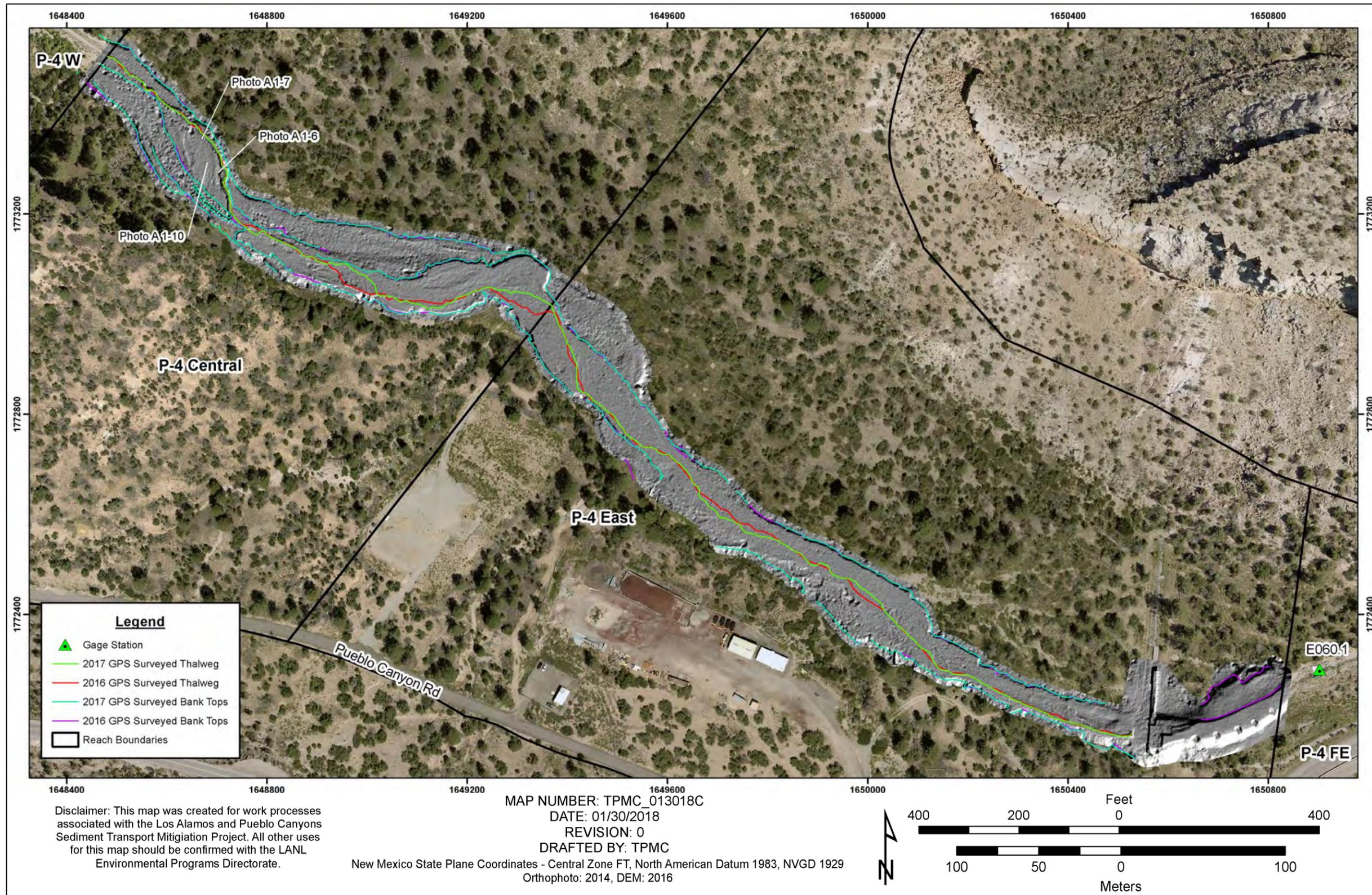
Figure A-4.5-1 2014 orthophoto with 2016 hillshade DEM and 2016 versus 2017 surveyed channel banks and thalweg at the Pueblo Canyon GCS area
