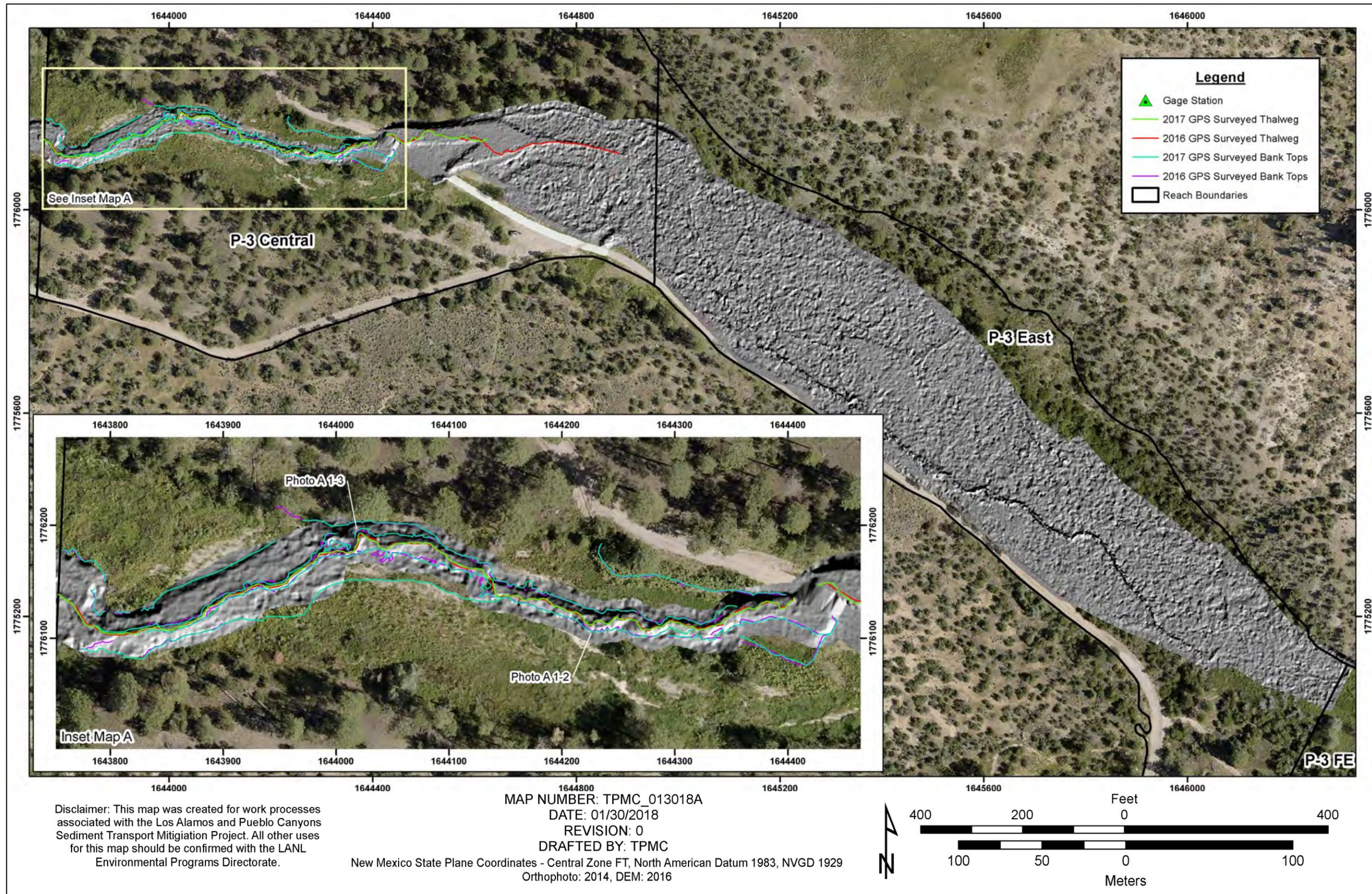
Figure A-4.3-1 2014 orthophoto with 2016 hillshade DEM and 2016 versus 2017 surveyed channel banks and thalweg at the Pueblo Canyon wing ditch area
