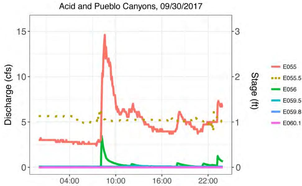
Figure 3.2-3 (continued) Hydrographs during each sample-triggering runoff event for each canyon from up- to downstream reaches
