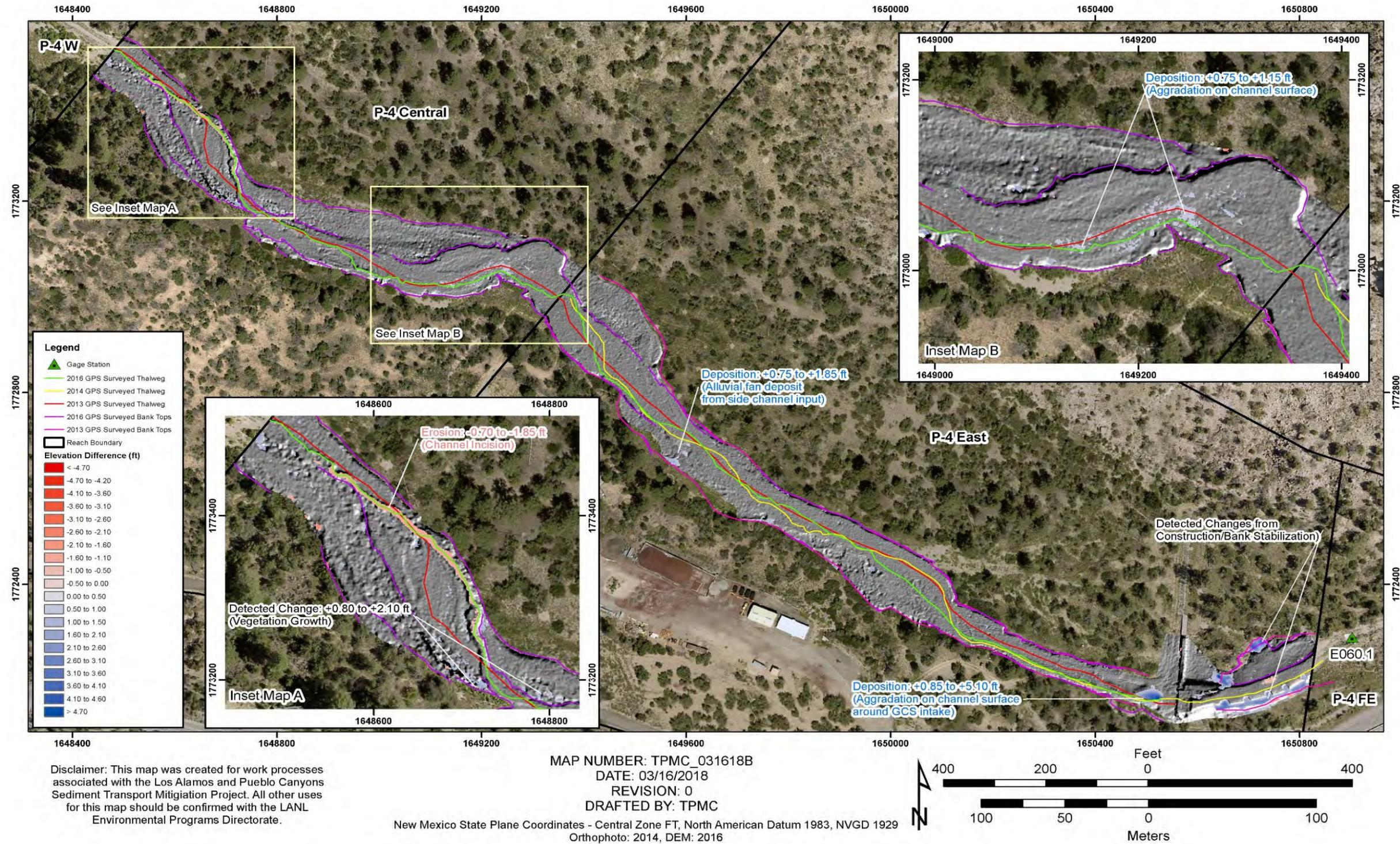
Figure A3-3.1-5 2014 orthophoto with 2016 hillshade DEM and 2014 to 2016 GCD results at the Pueblo Canyon GCS Monitoring Area. FIS calibration was based on observed differences between DEMs and field observations.
