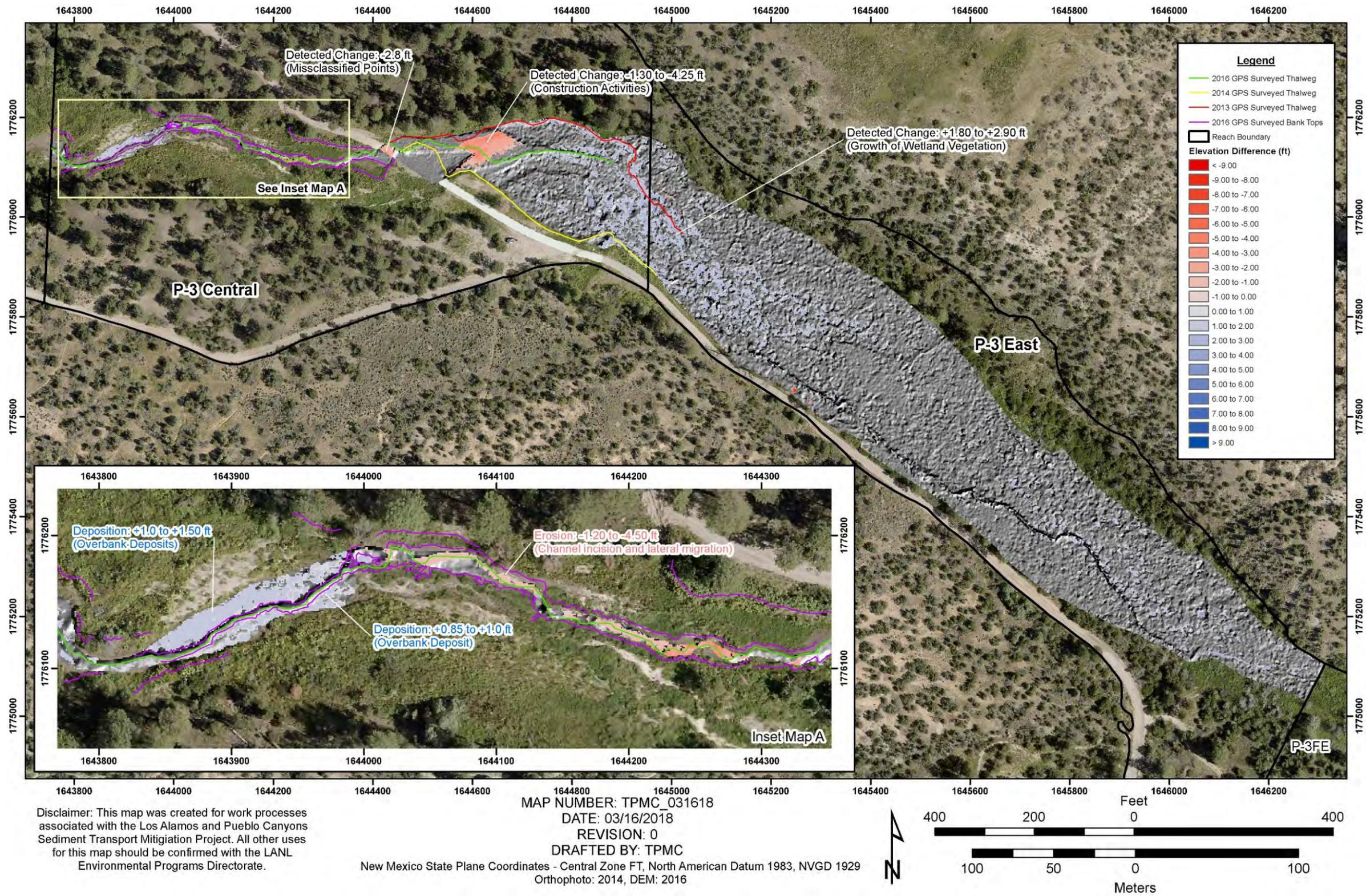
Figure A3-3.1-3 2014 orthophoto with 2016 hillshade DEM and 2014 to 2016 GCD results at the Pueblo Canyon Wing Ditch Monitoring Area. FIS calibration was based on calculated difference between GPS and DEM elevation values.
