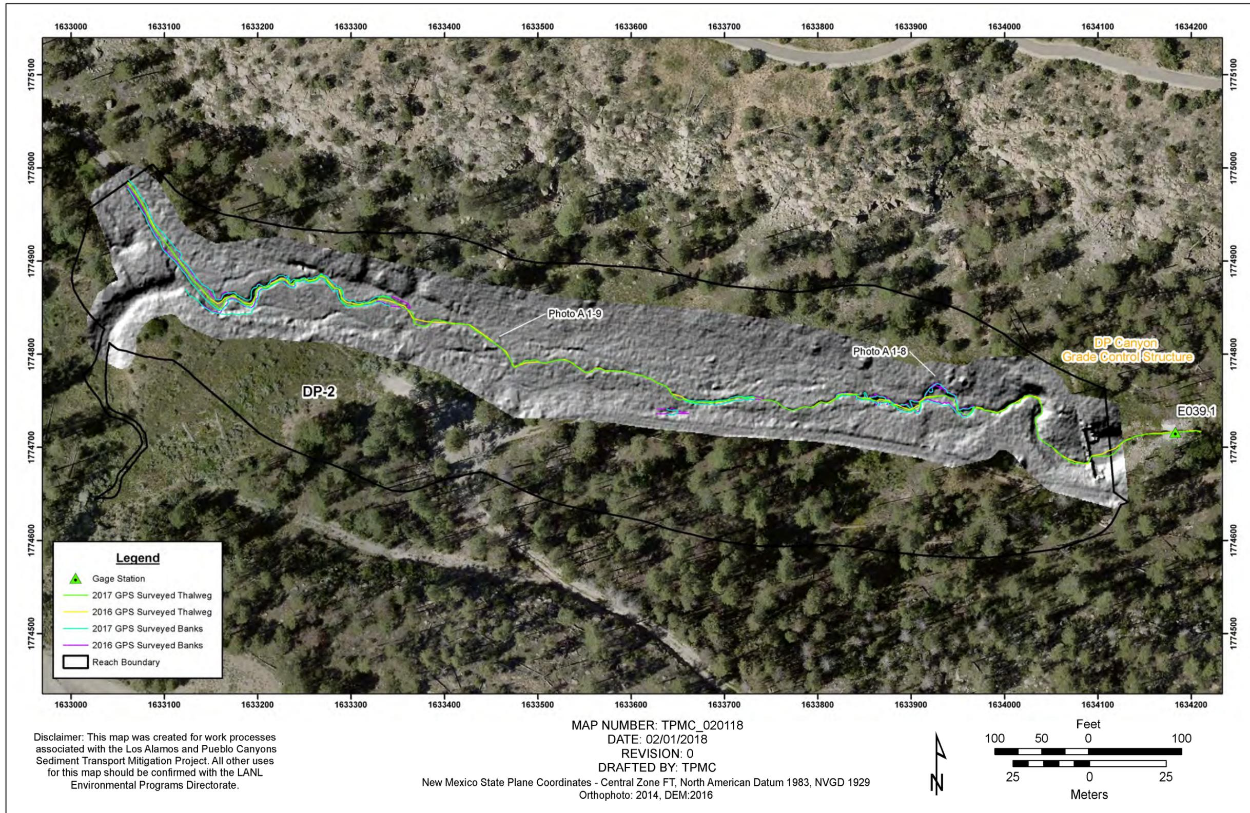
Figure A-4.8-1 2014 orthophoto with 2016 hillshade DEM and 2016 versus 2017 surveyed channel banks and thalweg at the DP Canyon GCS area
