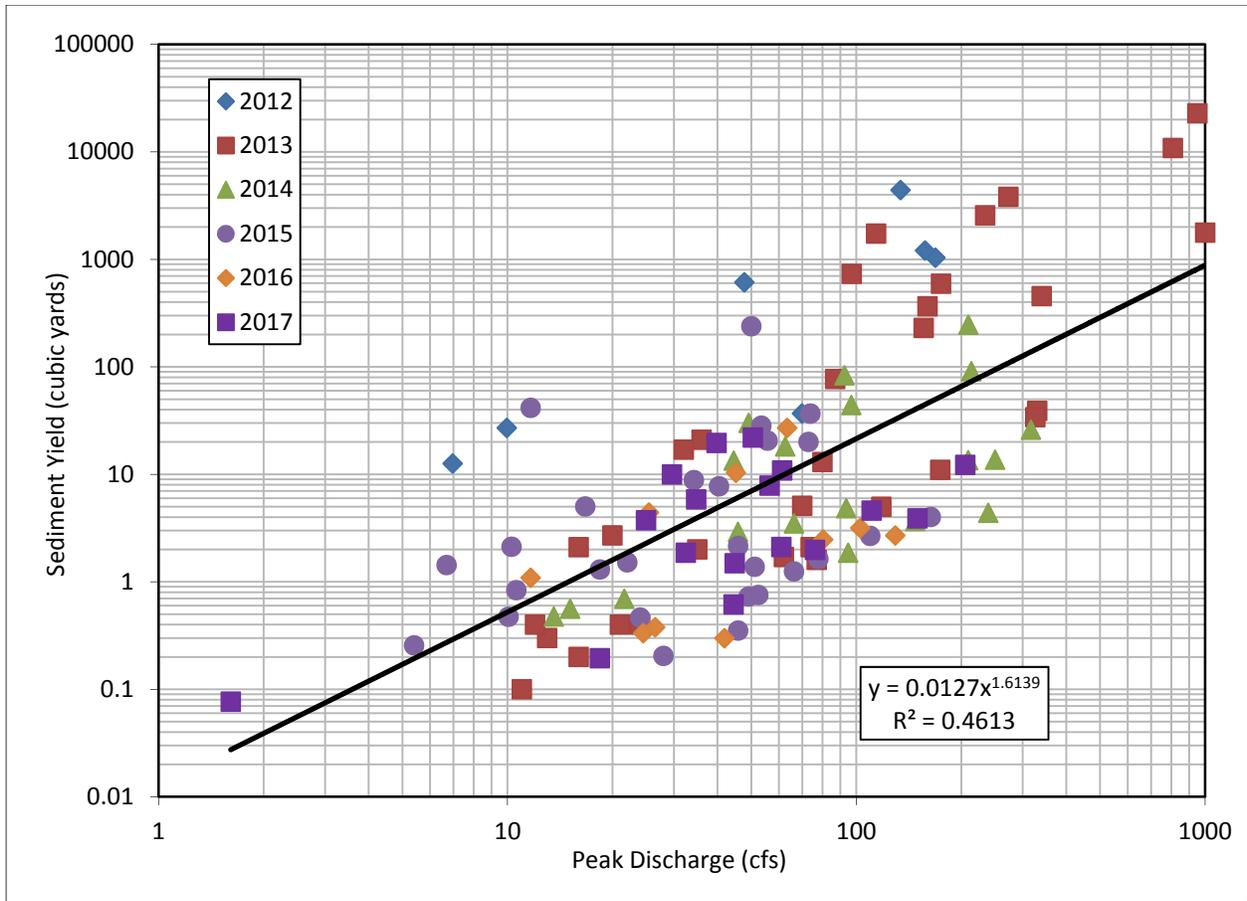
Figure 3.2-6 Relationship between SSC-based sediment yield and peak discharge over the past 6 yr of monitoring
