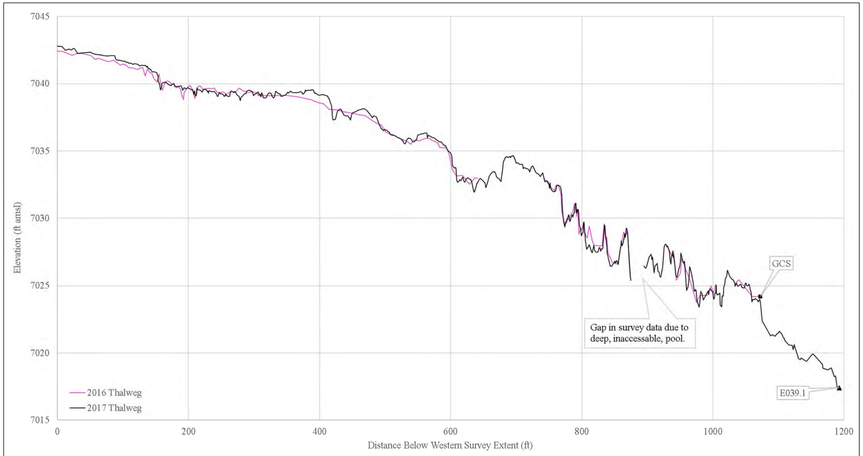
Figure A-4.8-2 Thalweg profile in DP Canyon GCS area (~25 times vertical exaggeration)
