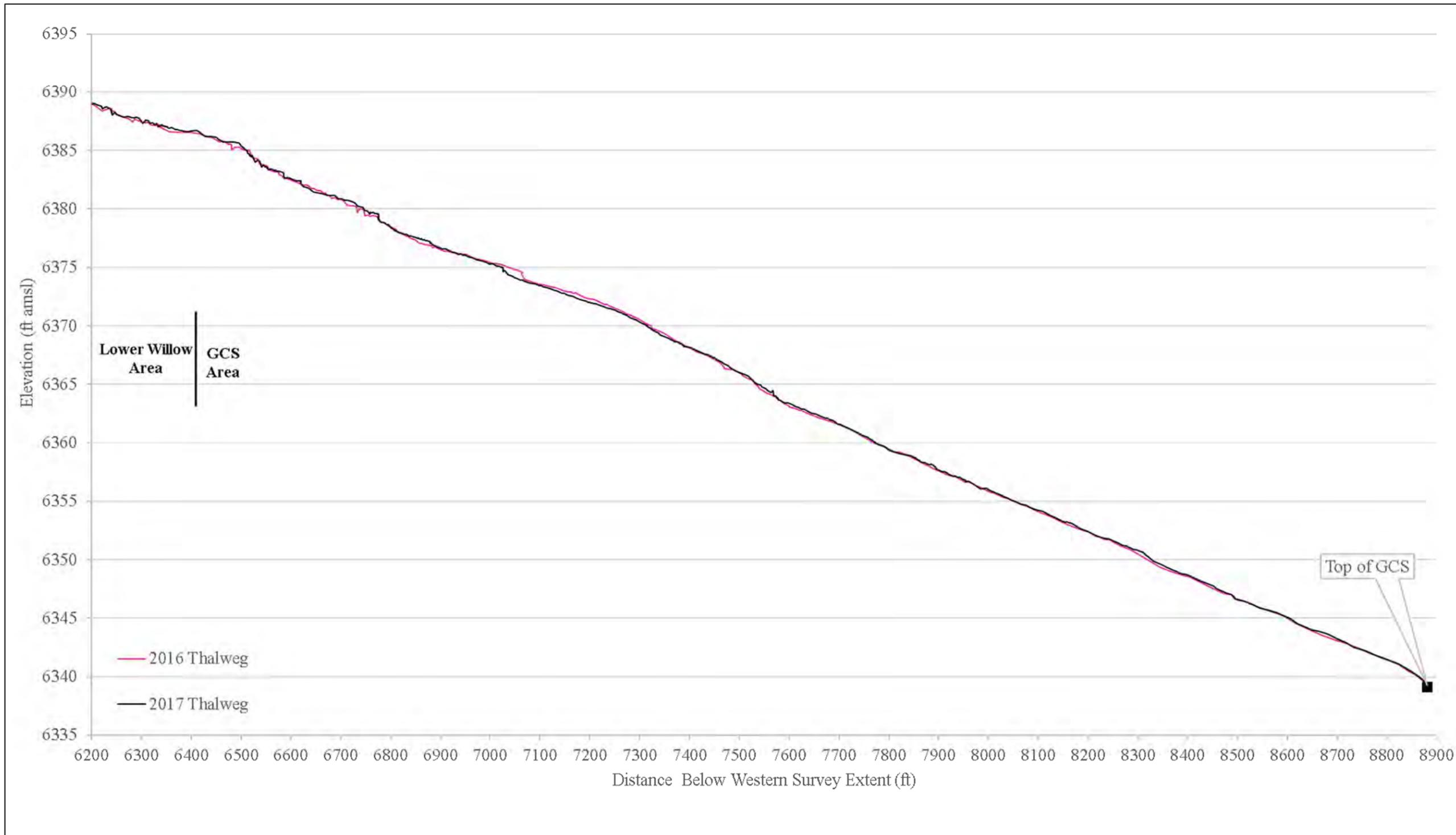
Figure A-4.5-2 Thalweg profile of the Pueblo Canyon GCS area (~25 times vertical exaggeration)
