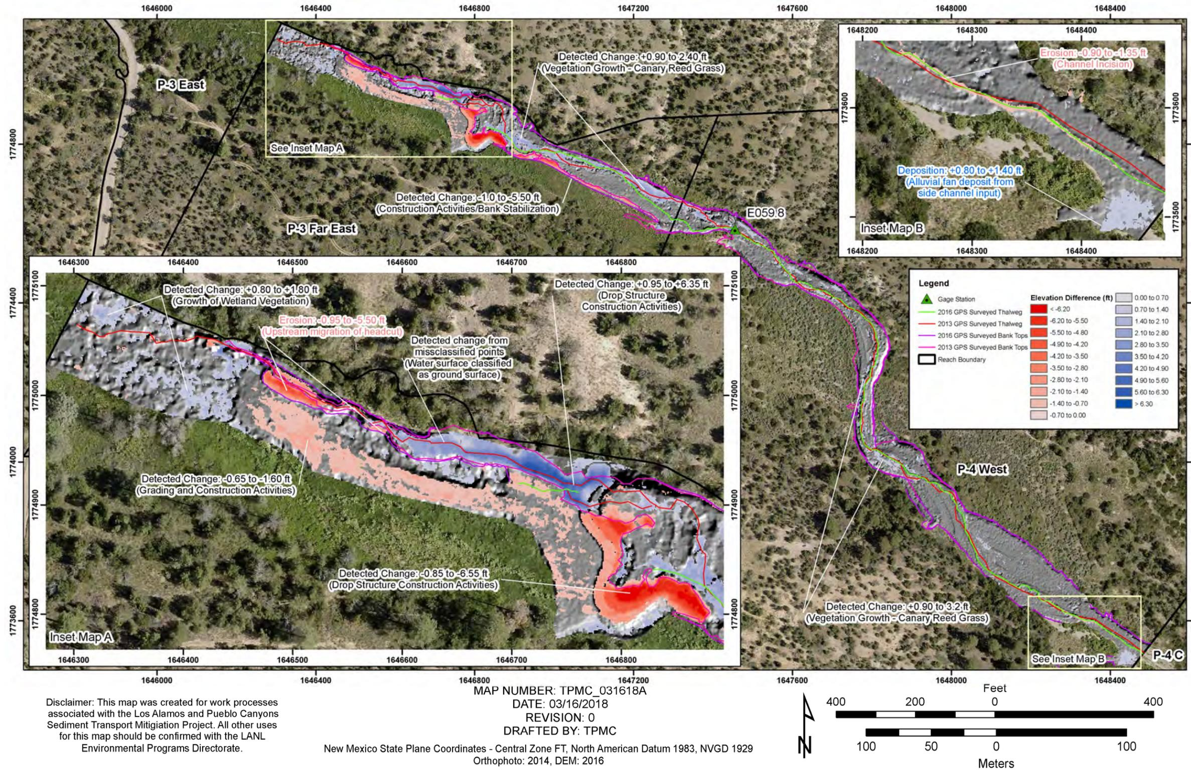
Figure A3-3.1-4 2014 orthophoto with 2016 hillshade DEM and 2014 to 2016 GCD results at the Lower Pueblo Canyon Willow Planting Monitoring Area. FIS calibration was based on observed differences between DEMs and field observations.
