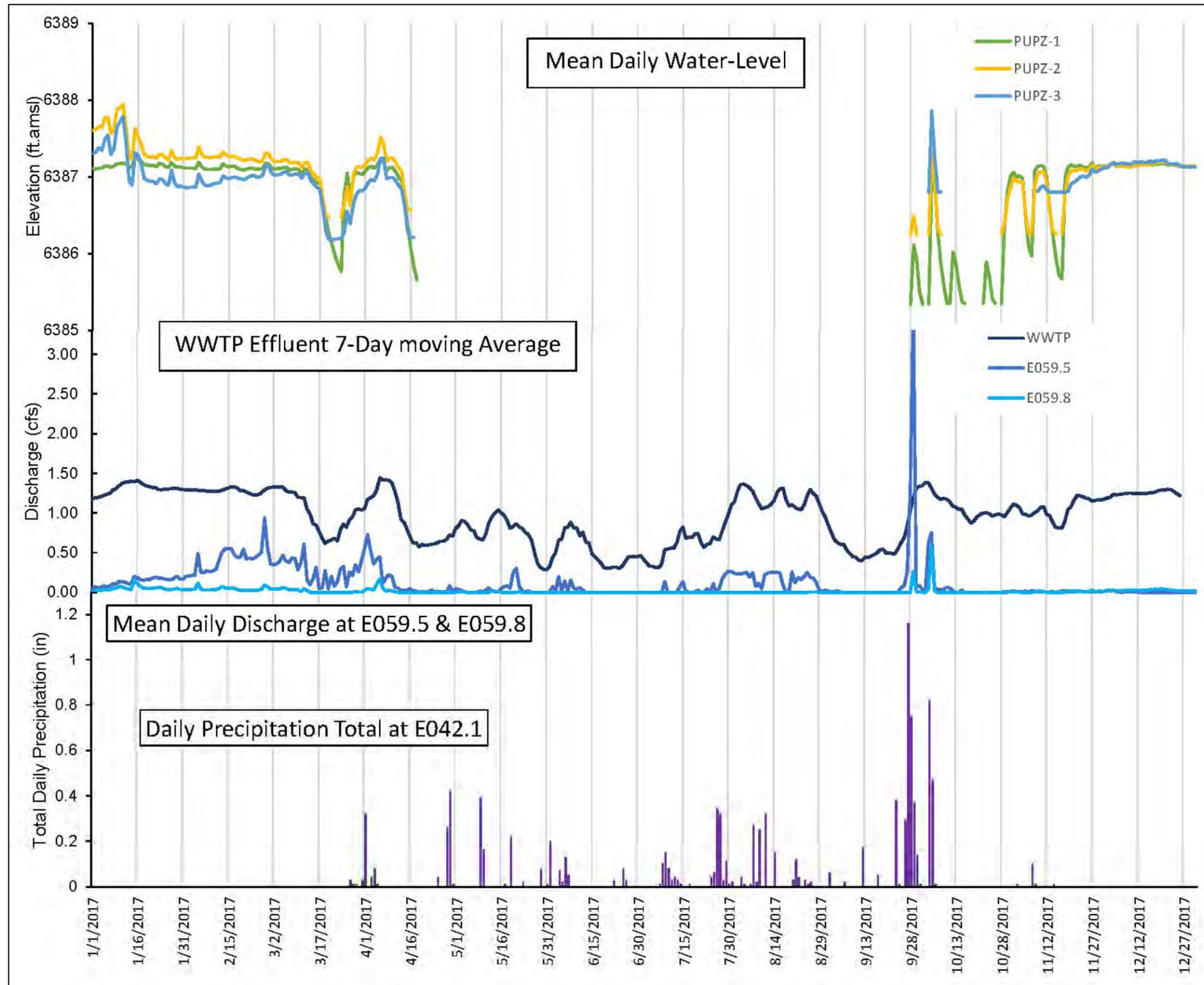
Figure B-2.0-1 Mean daily water level (ft above mean sea level [amsl]) in piezometers PUPZ-1, PUPZ-2, and PUPZ-3; 7-d moving average of Los Alamos wastewater treatment plant (WWTP) effluent discharge; mean daily discharge at gaging stations E059.5 and E059.8; and total daily precipitation at E042.1
