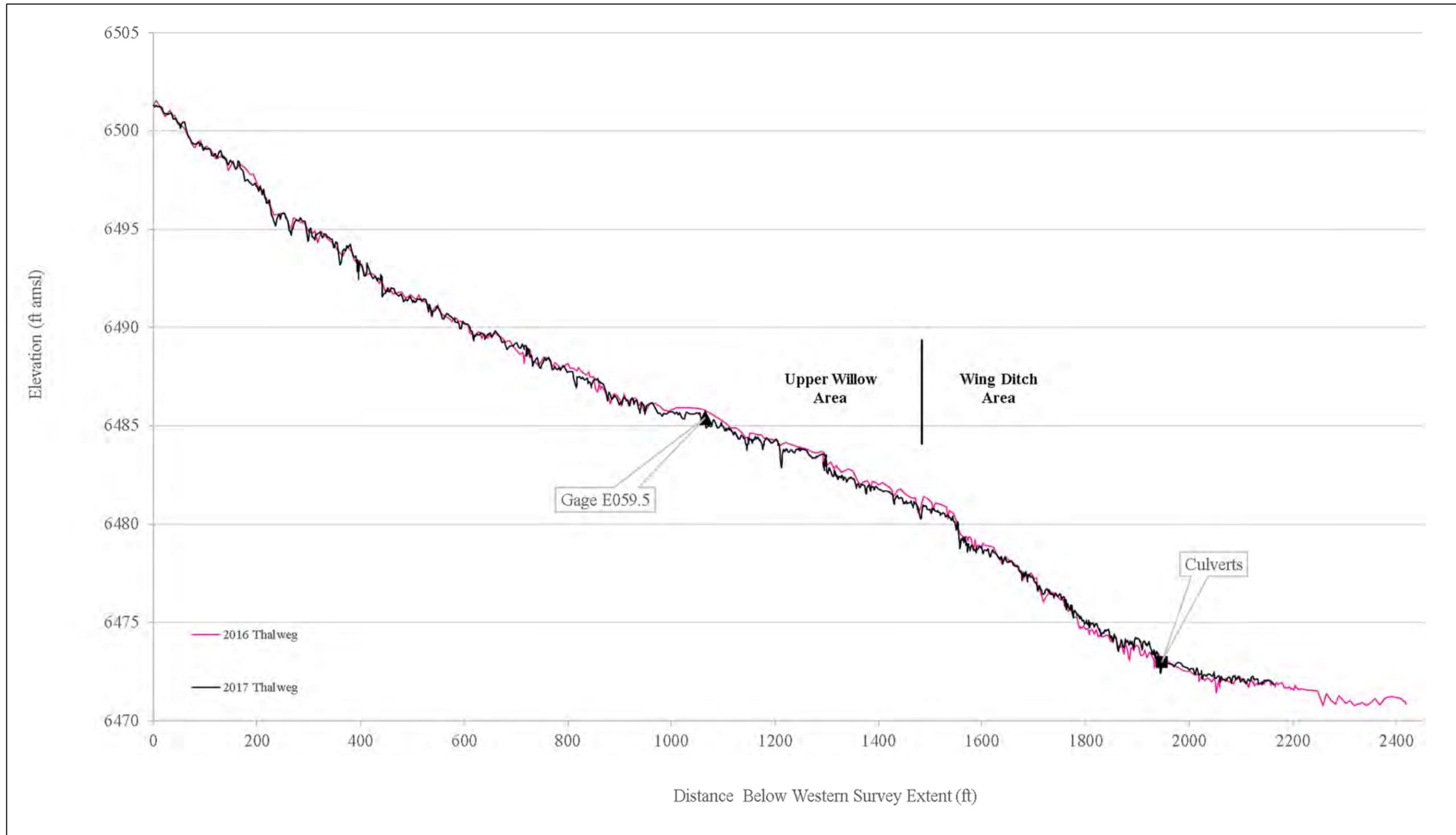
Figure A-4.2-2 Thalweg profile of the Pueblo Canyon upper willow planting and wing ditch areas (~38 times vertical exaggeration)
