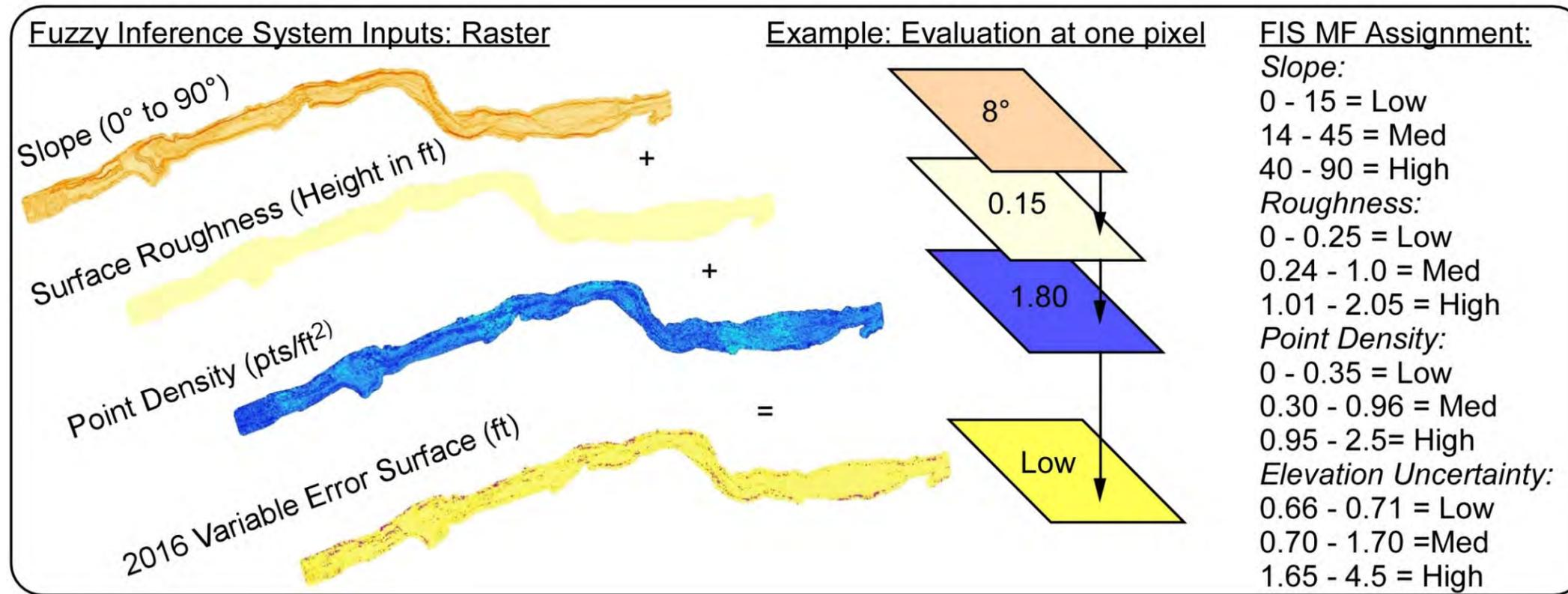
Figure A3-2.3-1 FIS error modeling concept of defining an error value for each pixel based on the quality of the surface as influenced by three characteristics: slope, point density, and surface roughness
