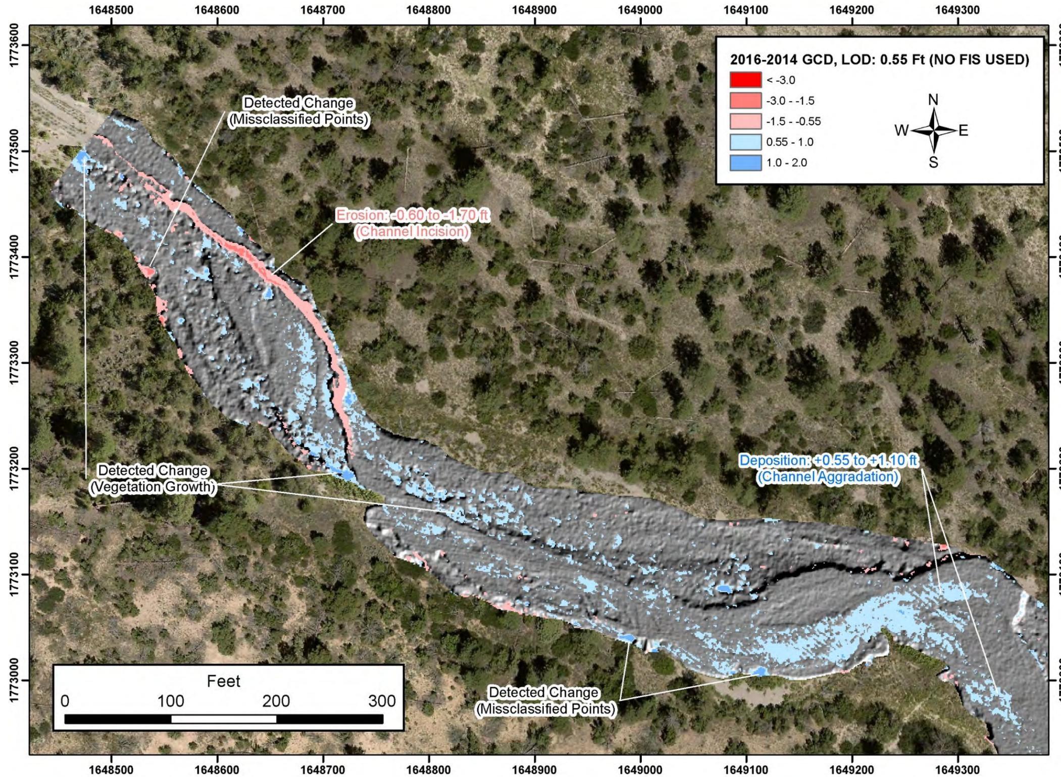
Figure A3-2.4-1 GCD analysis with a Min. LoD of 0.55 ft. 2014 orthophoto with 2016 hillshade DEM and 2014 to 2016 GCD results at the Pueblo Canyon grade-control structure area. Many non-geomorphic detections from vegetation growth, issues with modeling steep banks, and poor point classification are evident using the Min. LoD method for thresholding changes.
