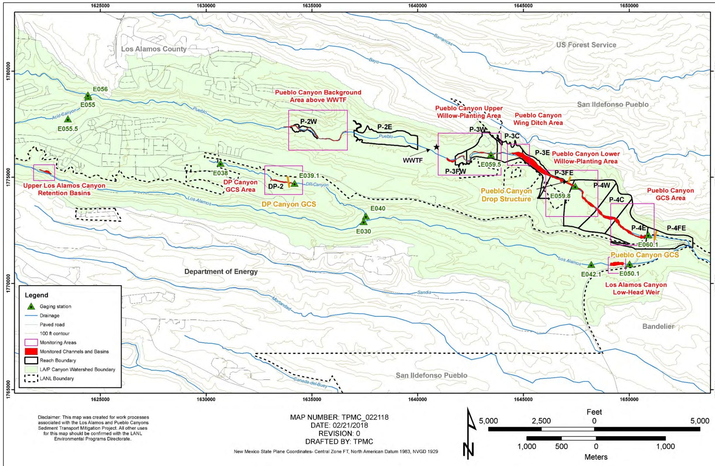
Figure A3-1.0-1 Los Alamos, Pueblo, and DP Canyon channel systems showing sediment transport monitoring areas, monitoring area extents, and stream gages
