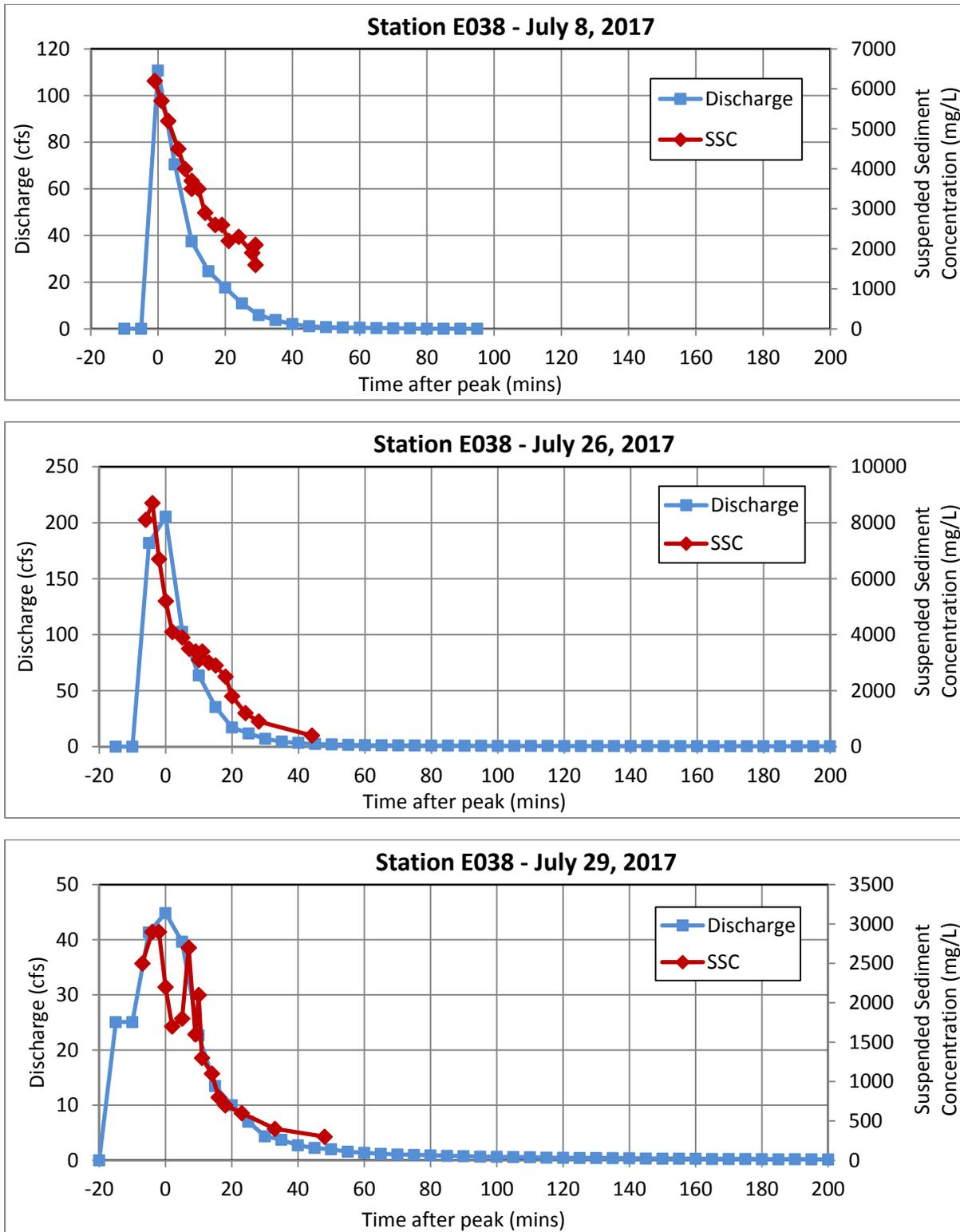
Figure 3.2-4 Discharge and SSC for events sampled at E038, E039.1, E042.1, E050.1, E059.5, and E059.8
