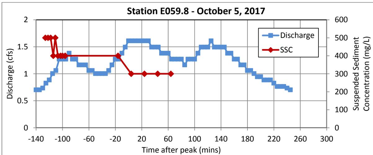
Figure 3.2-4 (continued) Discharge and SSC for events sampled at E038, E039.1, E042.1, E050.1, E059.5, and E059.8
