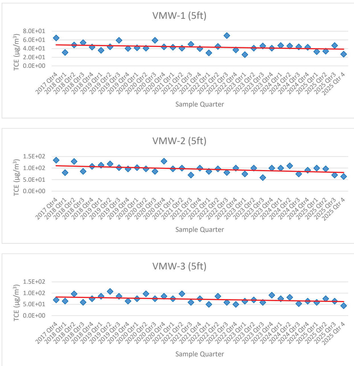
Figure 2. Data plots for TA-63 TWF soil vapor monitoring wells inside the permitted unit.
