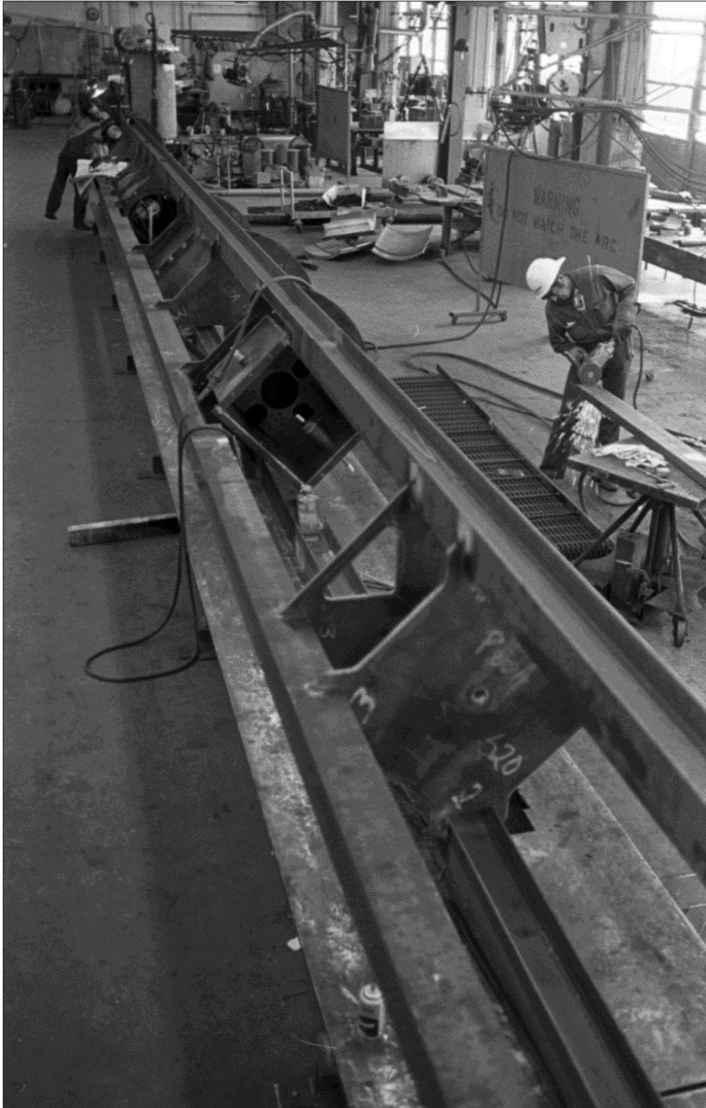
Figure 3-13. Steelworkers fabricate a diagnostic rack in the TA-03 Zia Company shop in 1975 (LANL image, accession no. PUB 75233-061).
