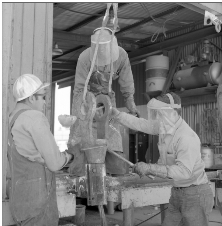
Figure 3-17. Laboratory employees prepare to pour hot liquid zinc into the sleeve of a socket in 1968 (LANL image, accession no. 21-00002079-PUB 68193).
