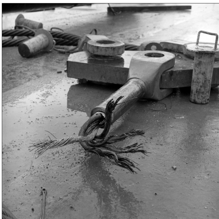
Figure 3-18. A wire-rope and socket assembly following strength testing in 1968. The holding power of the sockets was generally greater than the strength of the wire-ropes (LANL image, accession no. 21-00002059-PUB 68193).
