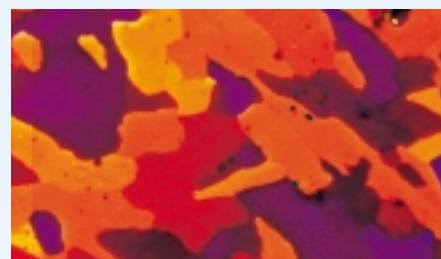
Polycrystalline \delta -phase plutonium alloy
