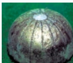
Half sphere of as-cast \delta -plutonium alloy
