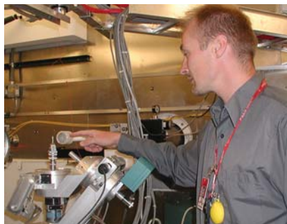
Figure 4. Protein Crystallography Paul Langan of the Bioscience Division points out the single-crystal \alpha -glycine sample used in the protein crystallography station.
