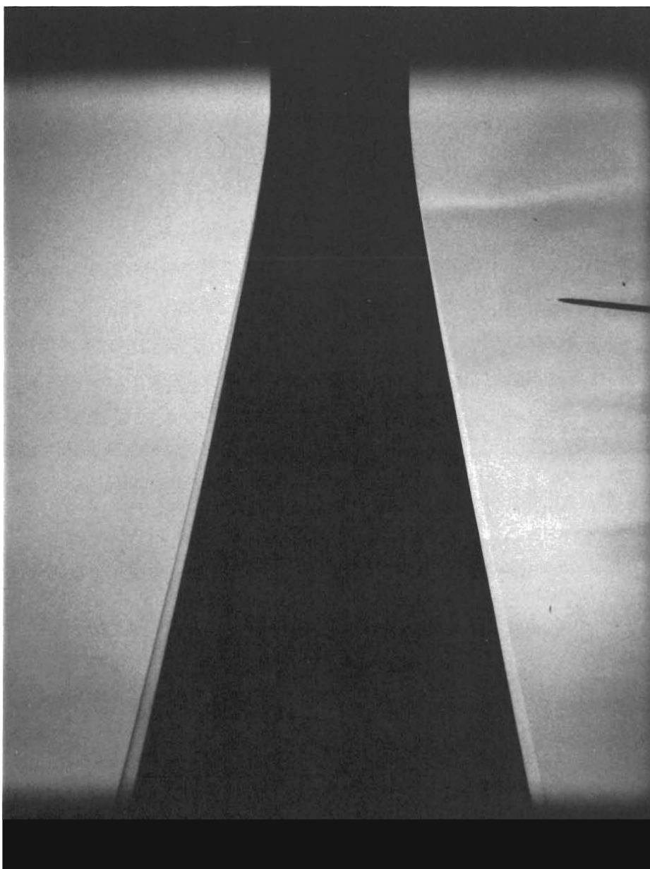
Fig. 12. Silhouette flash photograph of a cylinder test. The explosive charge, 300 mm long and 25 mm in diameter, was encased in a copper tube with 2.5-mm wall thickness. Explosive in the tube has been detonated at the bottom and is accelerating the copper outward. A very short section of undisturbed tube can be seen at the top. Measurements of the shape of the copper wall can be used to compute the expansion isentrope of the explosive products. Shock waves in the surrounding gas can be seen around the tube.
