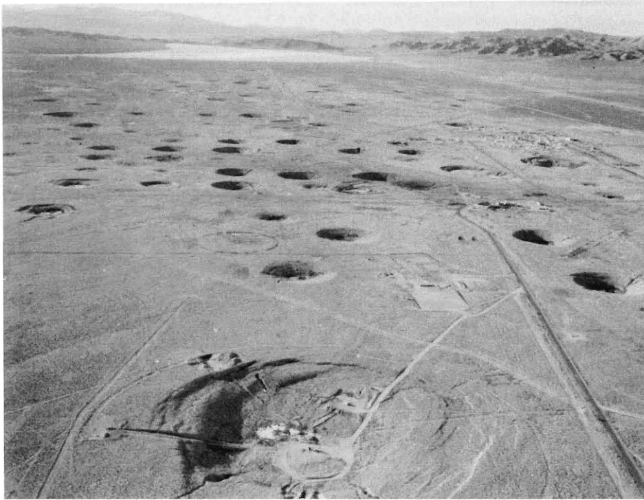
Aerial view of subsidence craters from underground nuclear tests in Yucca Flat at the NTS. The so-called Yucca Lake is in the background, and the Control Point complex is to the right of the dry lake.
