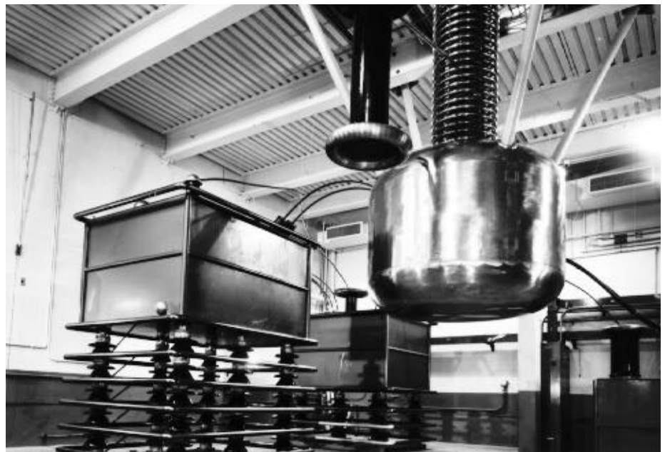
The Illinois Cockcroft-Walton Accelerator. This accelerator was used by John Manley and his group to investigate the efficacy of different metals as a “tamper”—a liner surrounding the nuclear explosive that acts as a neutron reflector and makes the explosive chain reaction more efficient. Gold, uranium, platinum, tungsten, and other metals were investigated as possible tampers.
