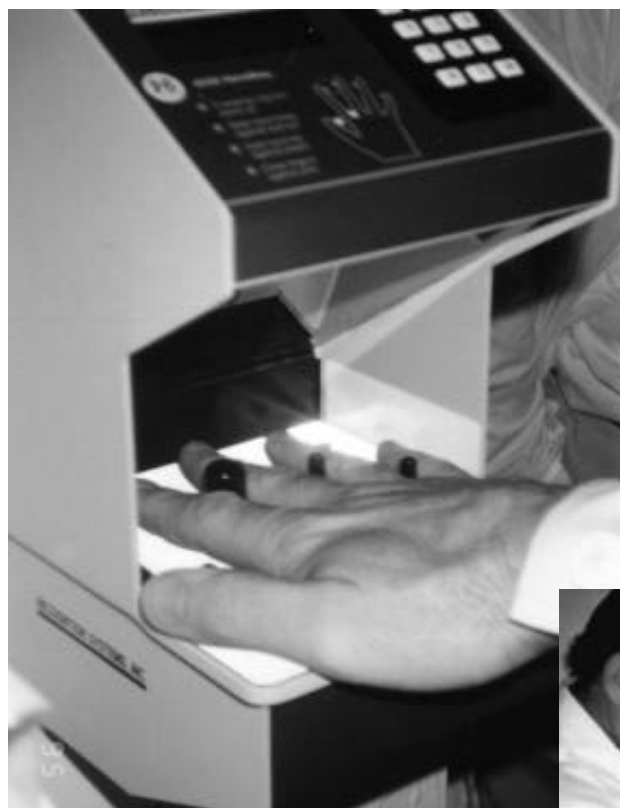
Figure 3. Access Controls The palm reader on the left determines a worker's identity on the basis of the size and shape of their hand. The size and shape are calculated from the capacitance between the hand and a grid of plates inside the palm reader. The palm, badge, and personal identification number readers (below) are used to identify workers throughout a nuclear facility. On the basis of a worker's identity, access to nuclear materials may be allowed or denied.
