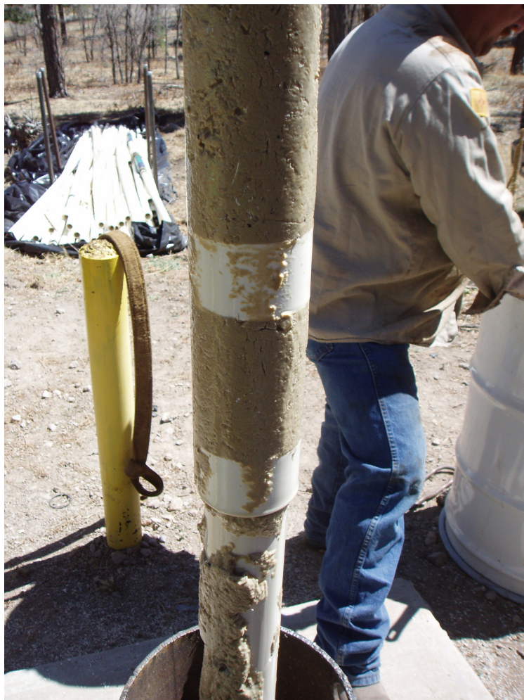
Figure 4.1-1 Photograph of Westbay sample port 2A at 1428 ft bgs encased in bentonite.
