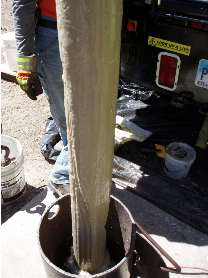
Figure 4.1-2 Photograph from approximately 1440 ft bgs showing screen 2, annular space between Westbay casing and stainless steel well casing completely occluded with bentonite.
