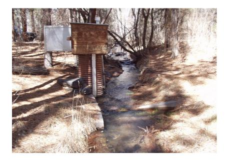
**Equipment.** The station is equipped with a Sutron 8210 data logger (5-min interval) with a shaft encoder float system (5-min interval) housed in a 3-× 4-ft metal shelter over a 24-in. CMP stilling well on the right bank. An outside staff gage is available for reference. Wading measurements are made 30 to 40 ft upstream from the gage. A high-flow measurement can be made from the bridge upstream 200 ft above the gage.
