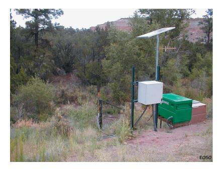
**Equipment.** The station is equipped with a Sutron 8210 data logger (5-min interval) and a Sutron Accubar bubble sensor and shaft encoder float system. No provision has been made for discharge measurements above the wading stage.
