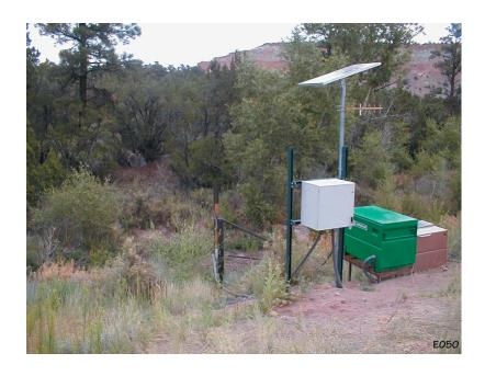
**Equipment.** The station is equipped with a Sutron 8210 data logger (5-min interval) and a Sutron Accubar bubble sensor and shaft encoder float system. No provision has been made for discharge measurements above the wading stage.
