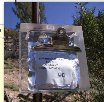
A TLD dosimeter attached to the fence on the border between TA-54 and San Ildefonso Pueblo.
