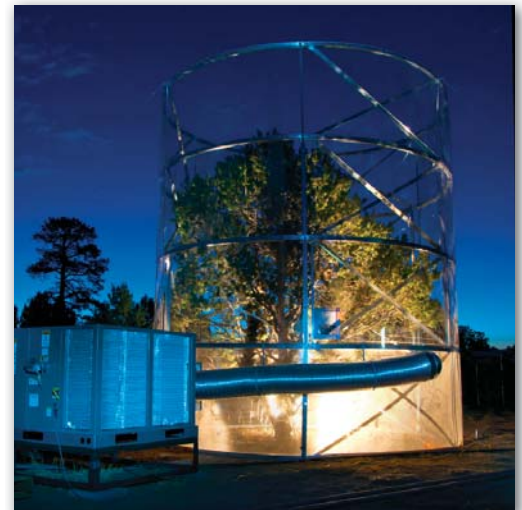
Enclosed in an acrylic chamber, a piñon tree and a juniper tree at the Los Alamos SUMO field site are introduced to increased temperature and decreased water to simulate the effects of climate change and determine how trees die.
