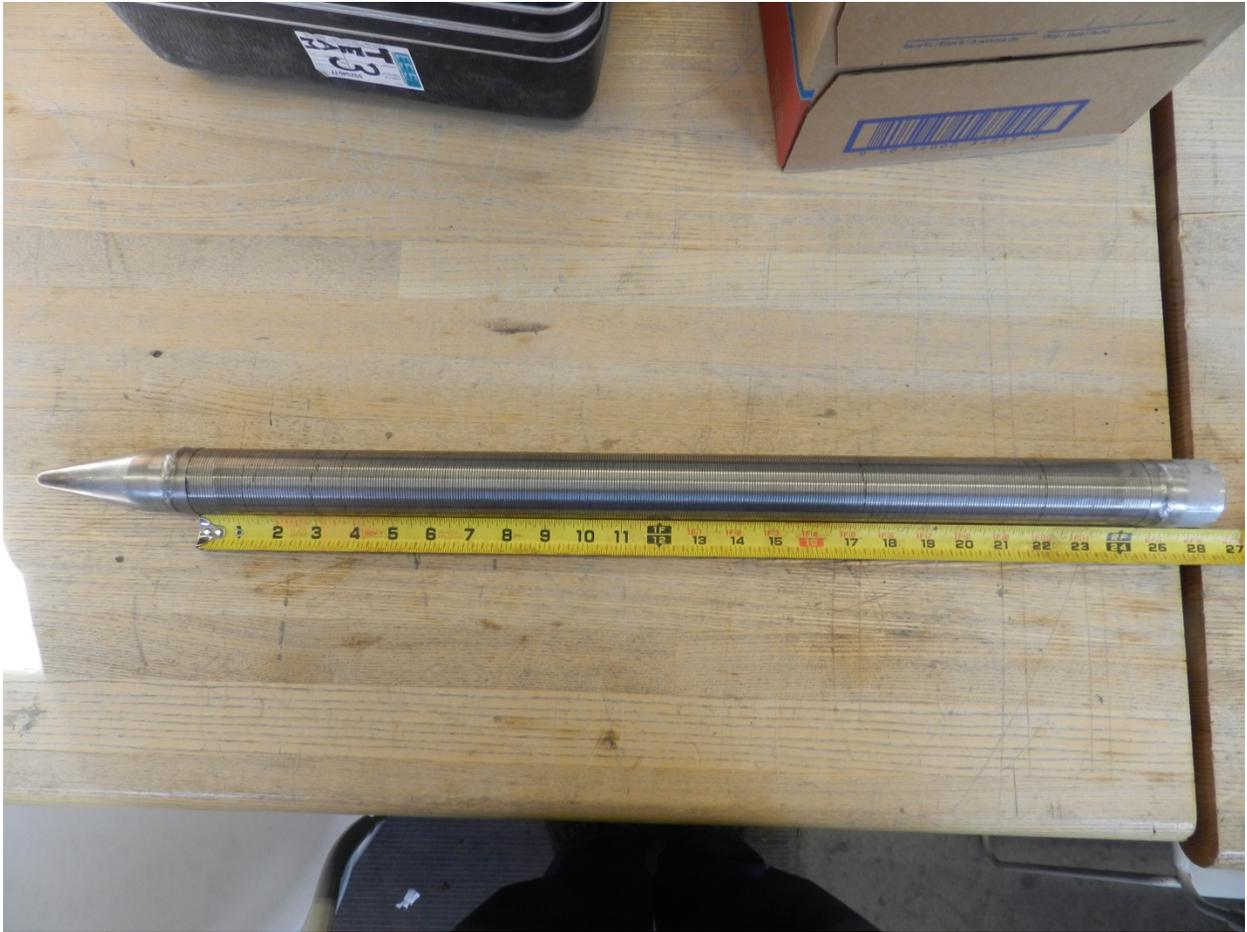
**Figure 1.5-1** A drive point with 2-ft screen used in the study
