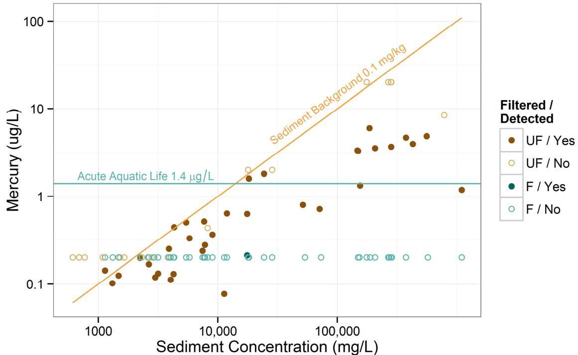
Figure 4.3-6 SSC vs. mercury for each gage station
