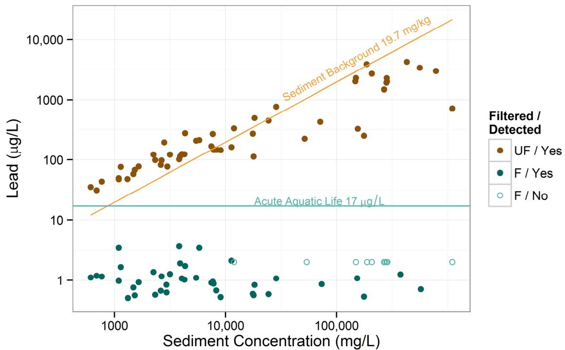
Figure 4.3-21 SSC vs. lead for each gage station
