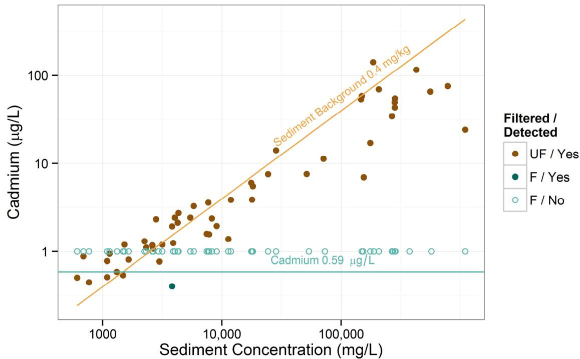
**Figure 4.3-18 SSC vs. cadmium for each gage station**
