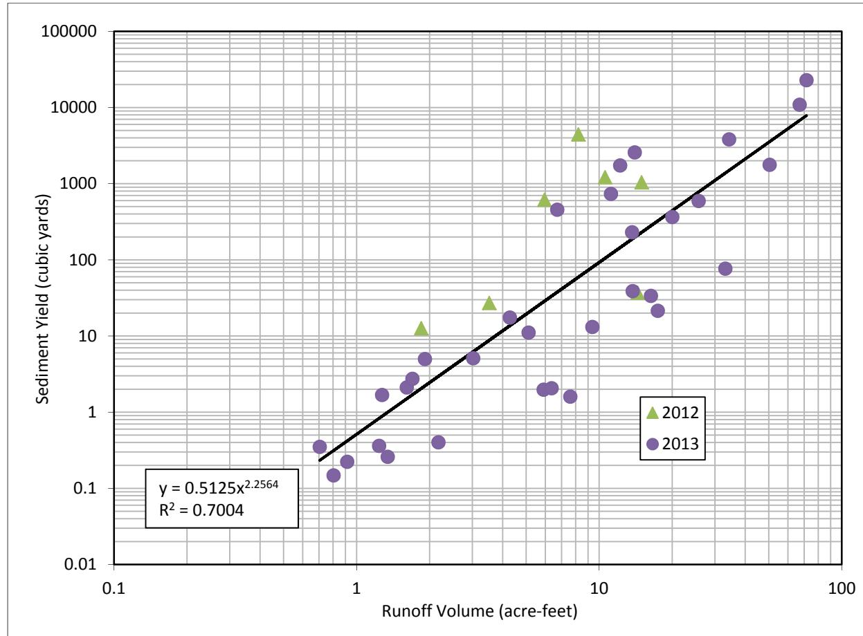
**Figure 3.2-5 Relationship between SSC-based sediment yield and runoff volume over the past 2 yr of monitoring**
