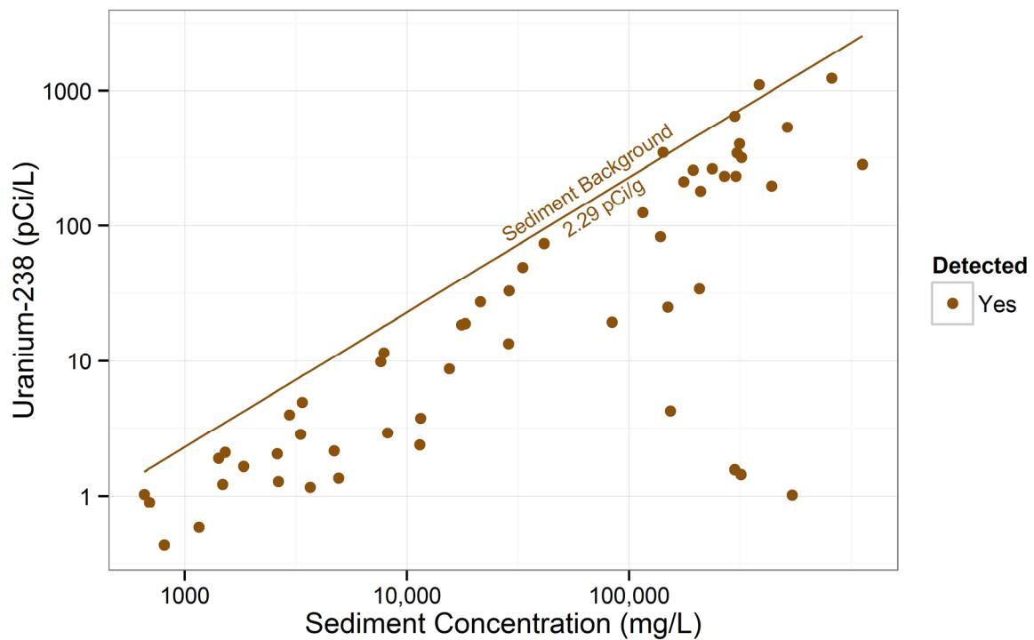
Figure 4.3-13 SSC vs. uranium-238 for each gage station
