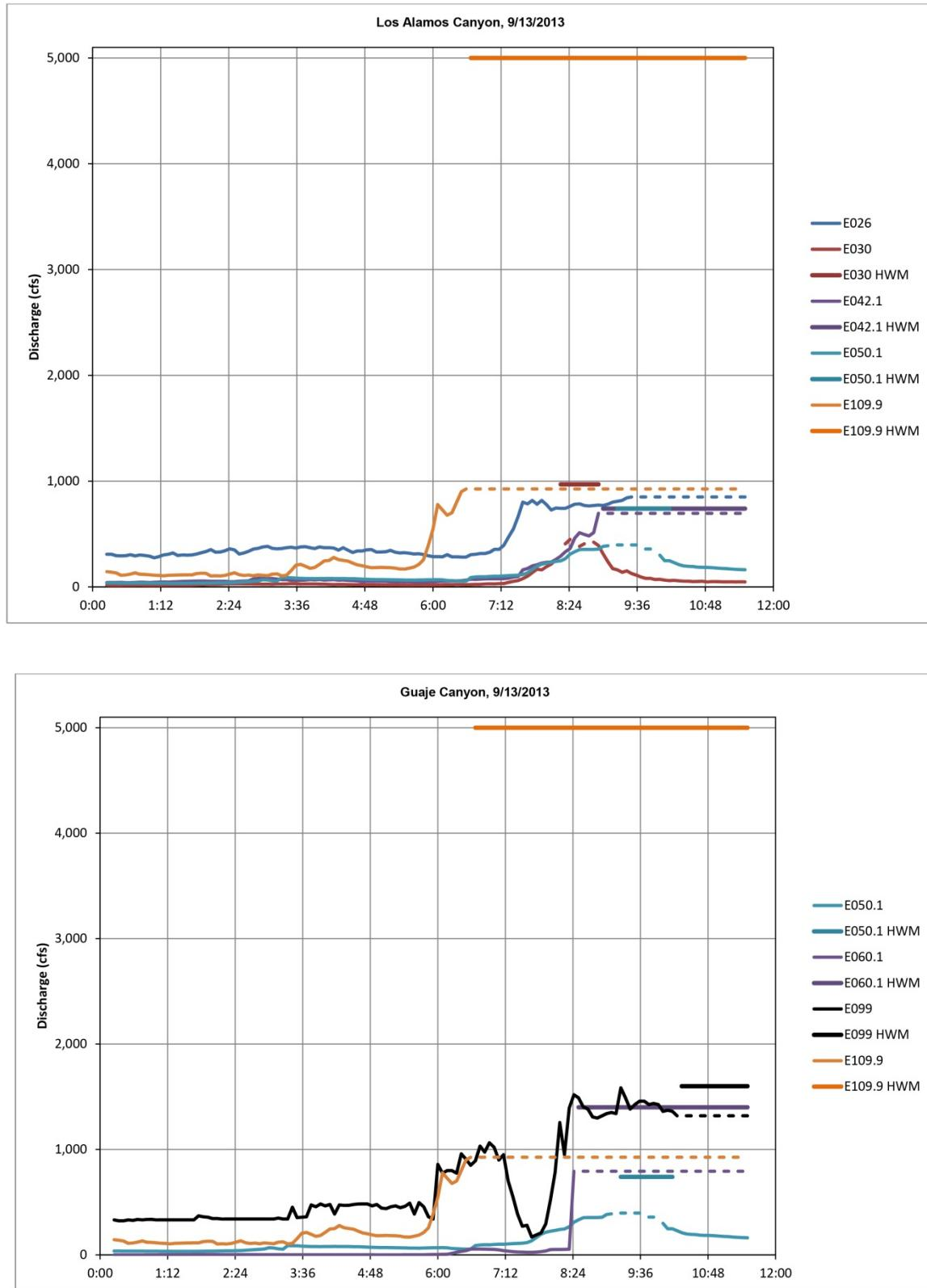
**Figure 3.2-3 (continued)** Hydrographs during each sample-triggering runoff event for each canyon from up- to downstream reaches
