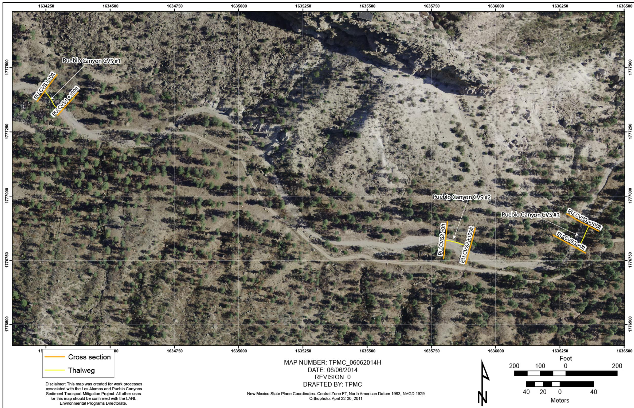
Figure A-3.1-1 Orthophoto showing the locations of surveyed cross-sections and thalweg profiles at the Pueblo Canyon CVSs
