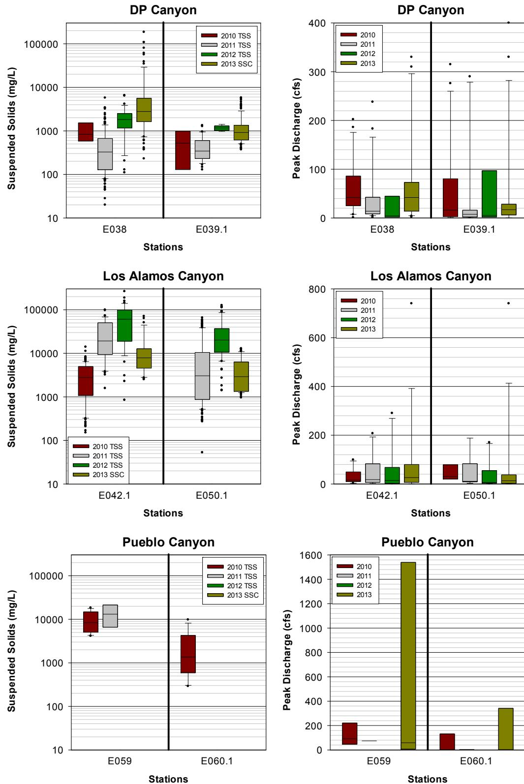
**Figure 3.4-2** Box and whisker plots of TSS and SSC (left) and peak discharge (right) upstream and downstream of the watershed mitigations in DP (top), Los Alamos (middle), and Pueblo (bottom) Canyons over the past 4 yr of monitoring
