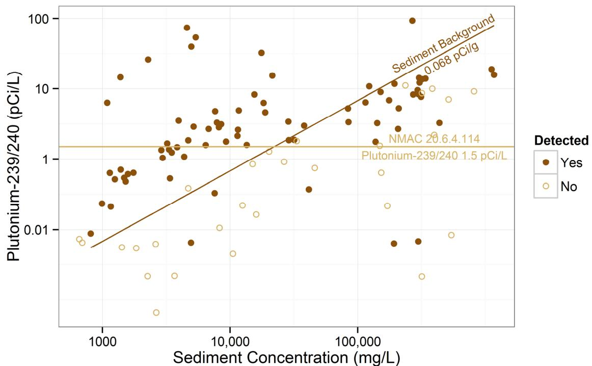
**Figure 4.3-28 SSC vs. plutonium-239/240 for each gage station**
