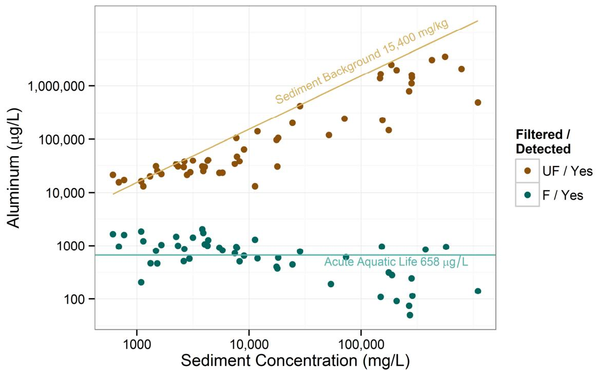
**Figure 4.3-1** SSC vs. aluminum for each gage station
