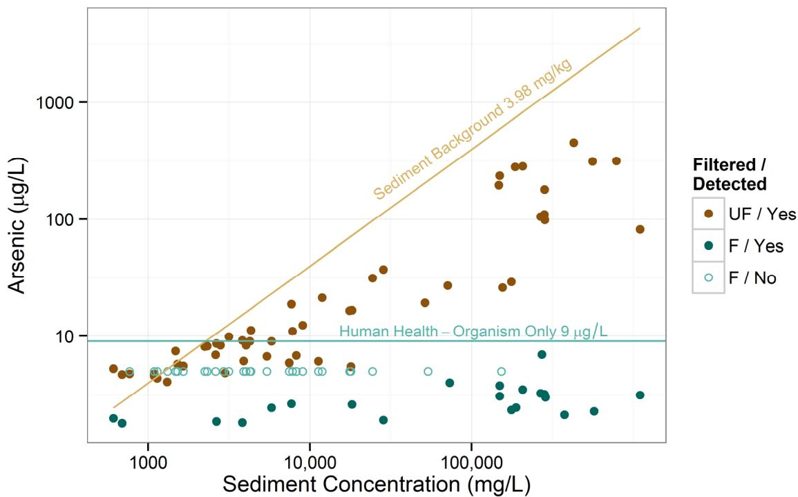
**Figure 4.3-3 SSC vs. arsenic for each gage station**
