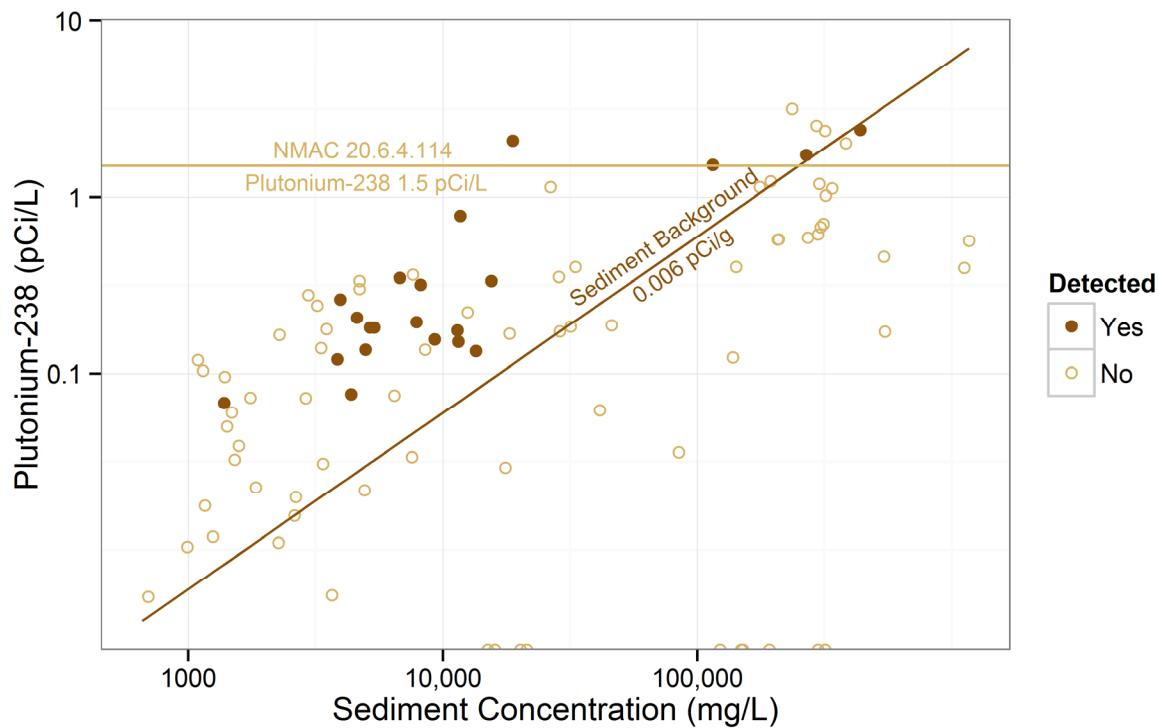
Figure 4.3-29 SSC vs. plutonium-238 for each gage station
