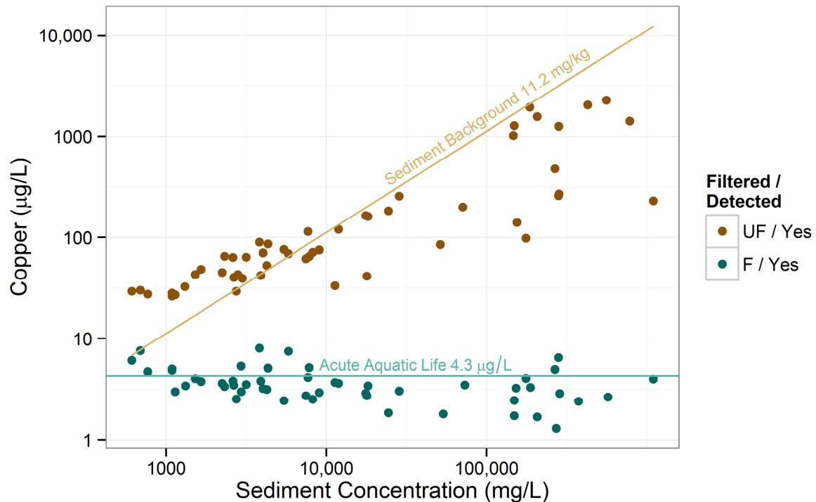
**Figure 4.3-20 SSC vs. copper for each gage station**
