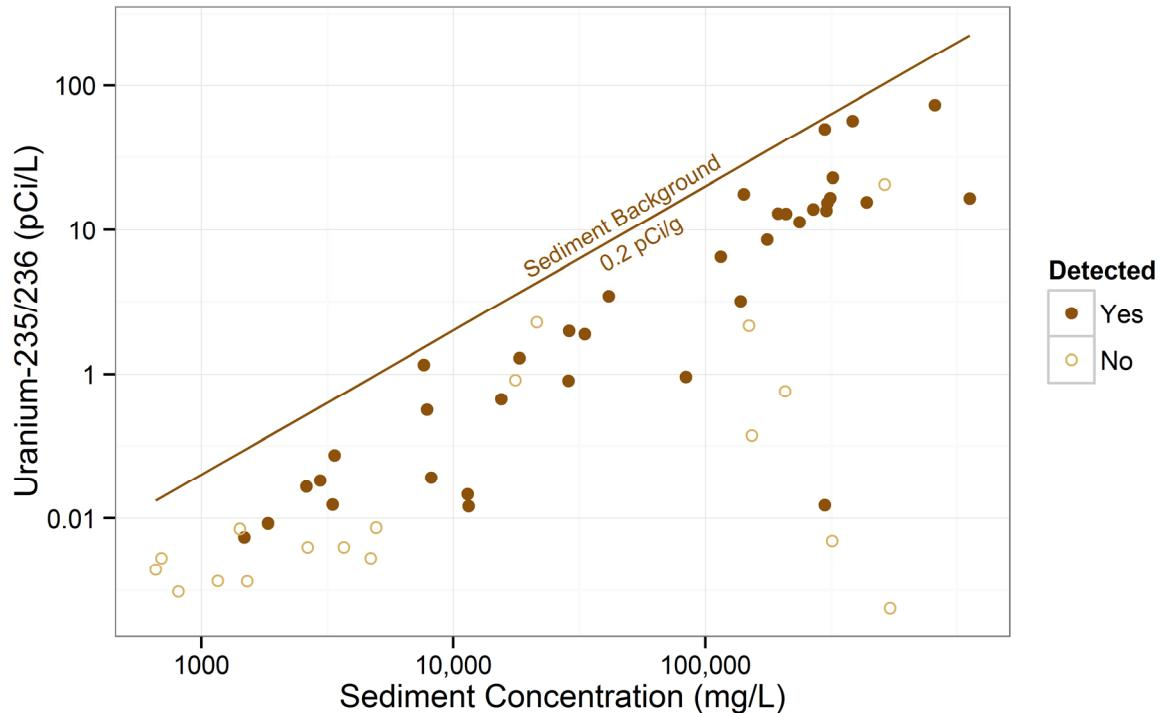
**Figure 4.3-12** SSC vs. uranium-235 for each gage station
