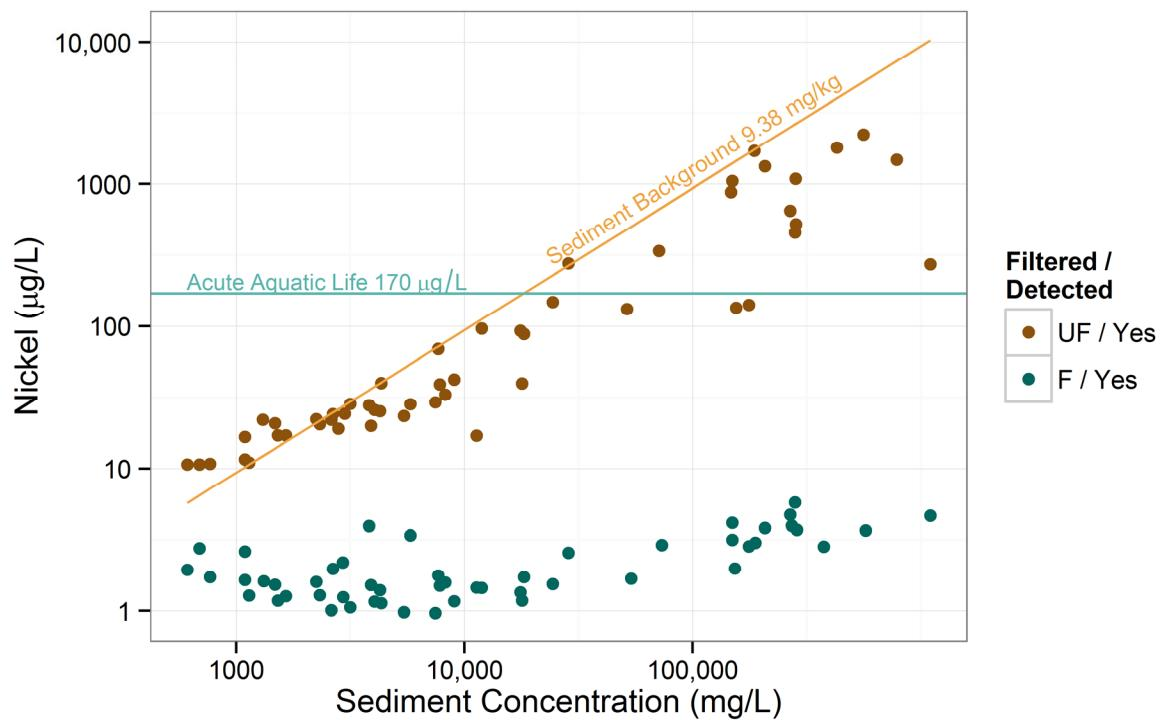
**Figure 4.3-7 SSC vs. nickel for each gage station**
