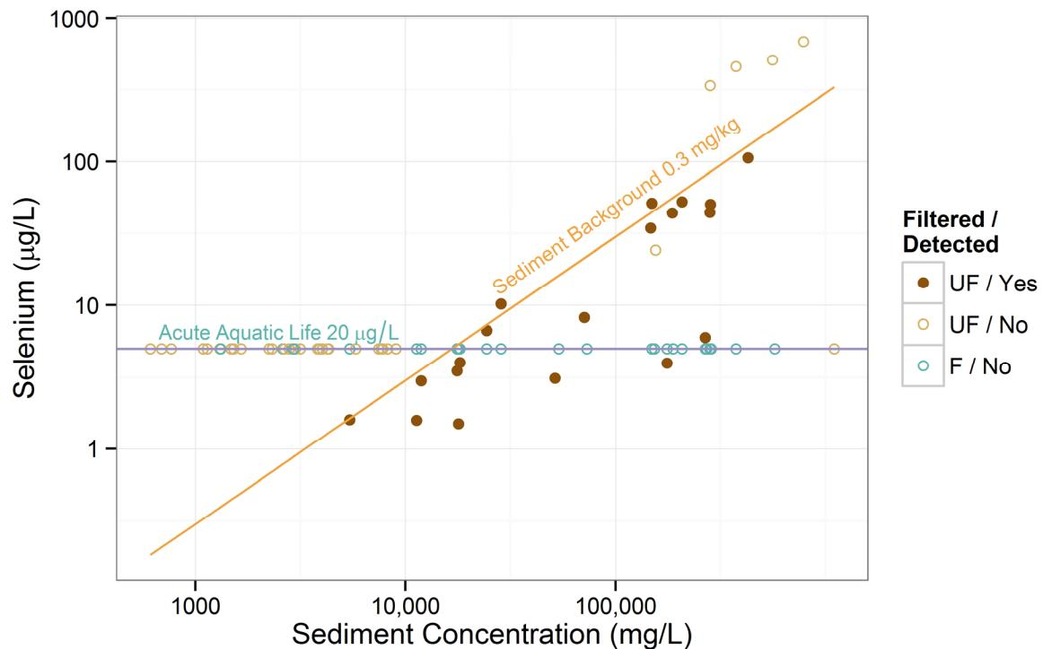
**Figure 4.3-8 SSC vs. selenium for each gage station**
