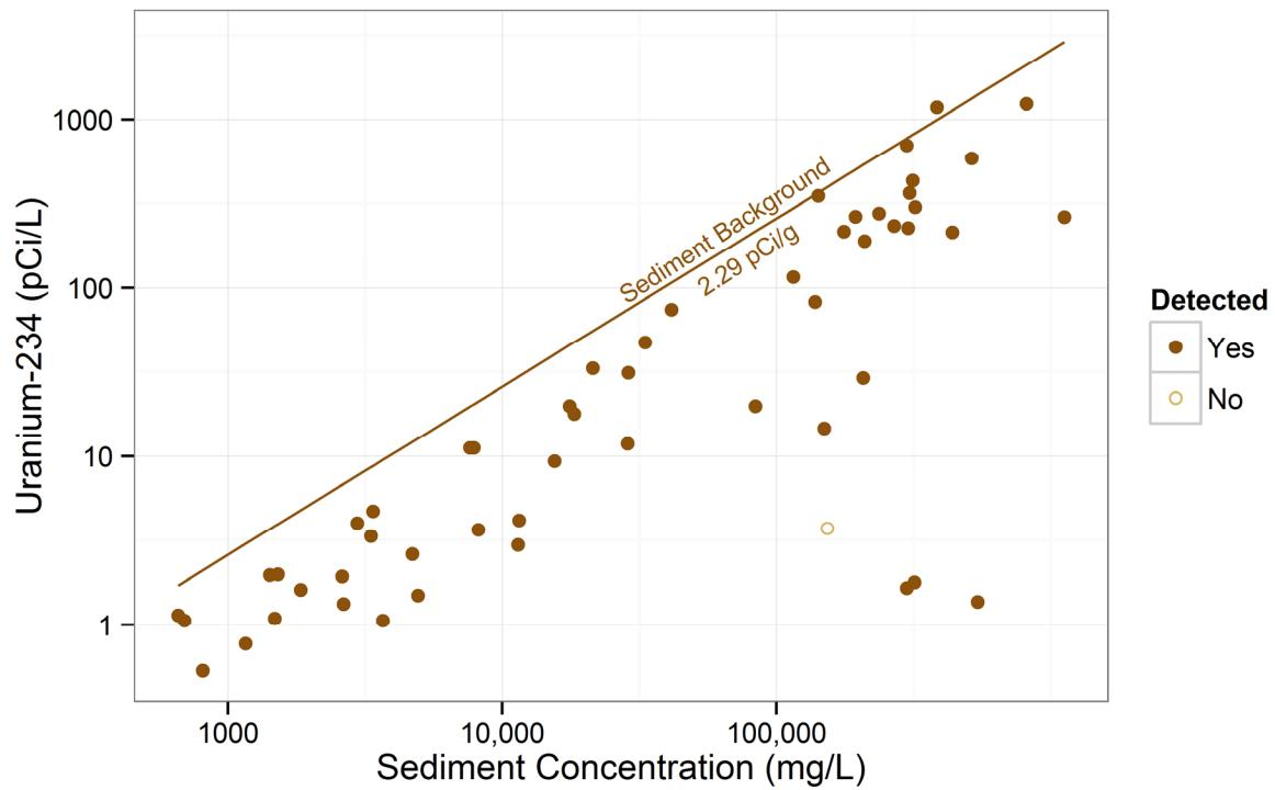
**Figure 4.3-11** SSC vs. uranium-234 for each gage station
