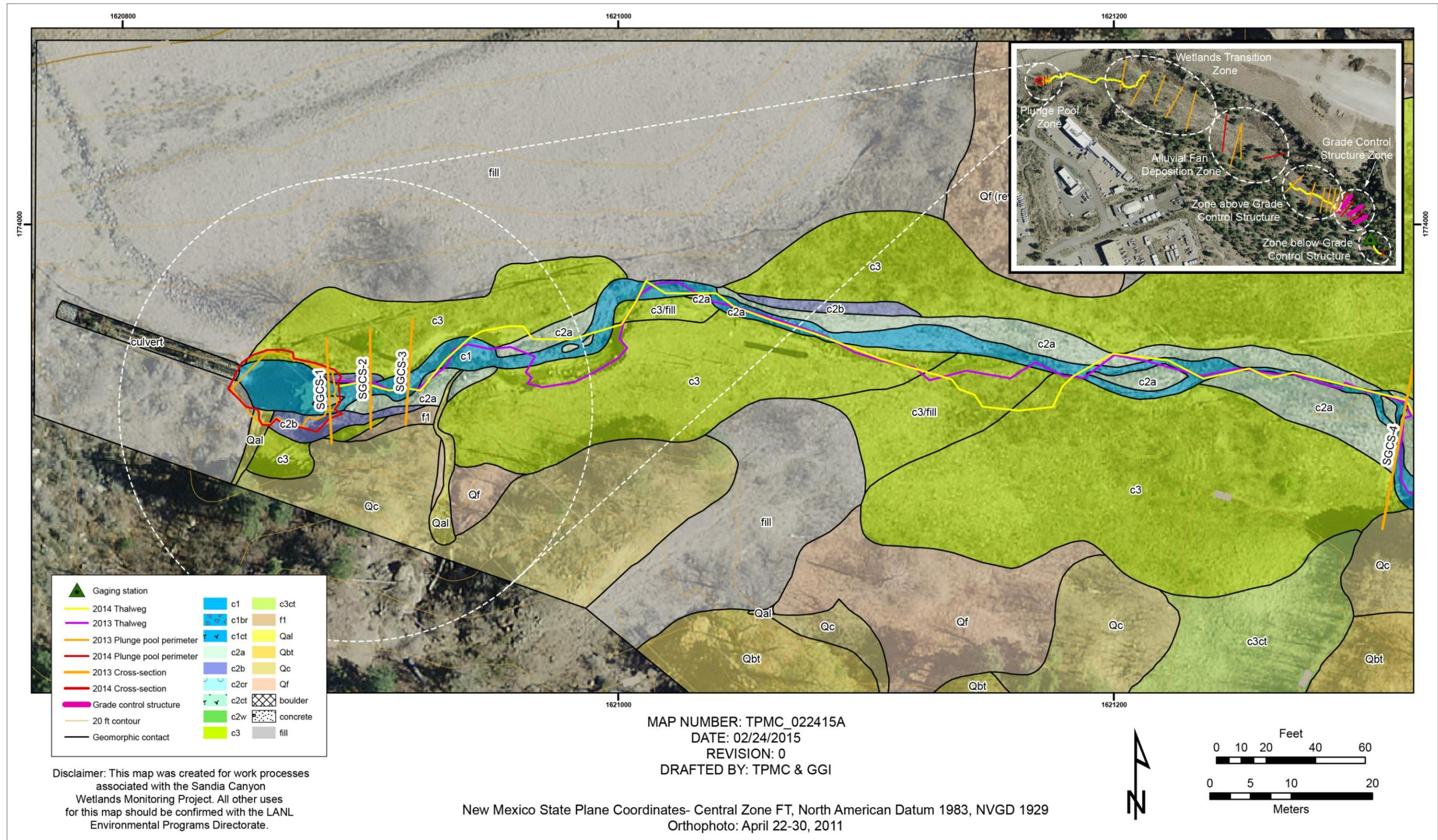
**Figure B-4.1-1** Geomorphic map overlain on an orthophoto showing the locations of cross-section transects and thalweg surveys at the Plunge Pool Zone in Sandia Canyon Reach S-2. The plunge pool perimeter as surveyed for MY2013 and MY2014 is shown in orange (MY2013) and red (MY2014).
