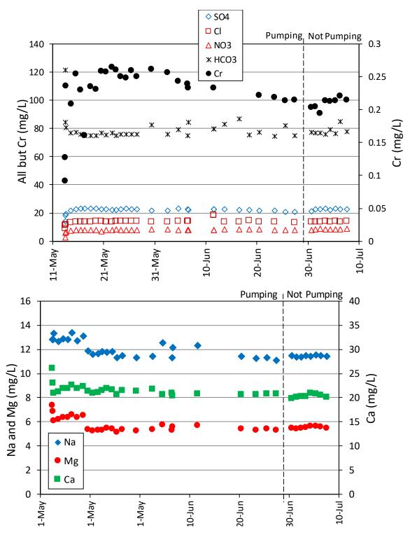
Figure 4.0-4Concentrations of key constituents in R-62 during the long-term pumping test of<br/>R-62 (at 1–1.5 gpm), including the period immediately after pumping ended
