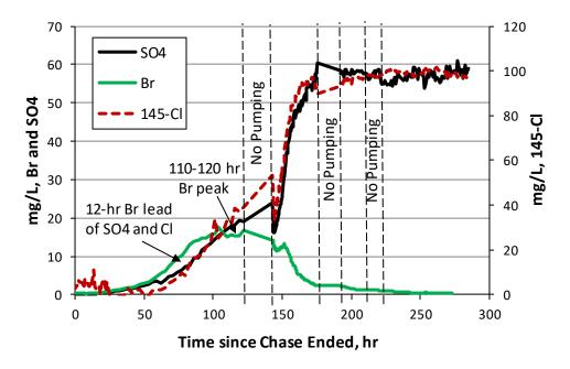
Figure 3.2-2 Tracer and aquifer water breakthroughs during the R-28 push-pull tracer test, showing Br breakthrough relative to conservative anions that were in aquifer water but not in treated water (SO₄<sup>=</sup>) or vice-versa (CI<sup>-</sup>, which had a concentration of about 145 mg/L in treated water and 45 mg/L in aquifer water)
