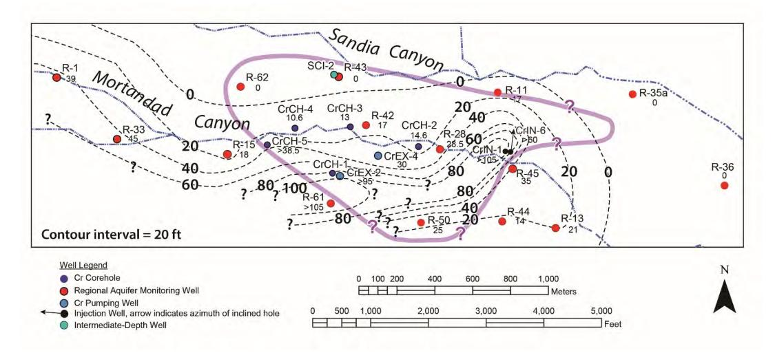
Figure 3.4-1 Isopach map showing thickness of the Puye pumiceous subunit [Tpf(p)] in the vicinity of the chromium plume (purple) in Mortandad Canyon. Only wells where the thickness of Tpf(p) was determined are shown.
