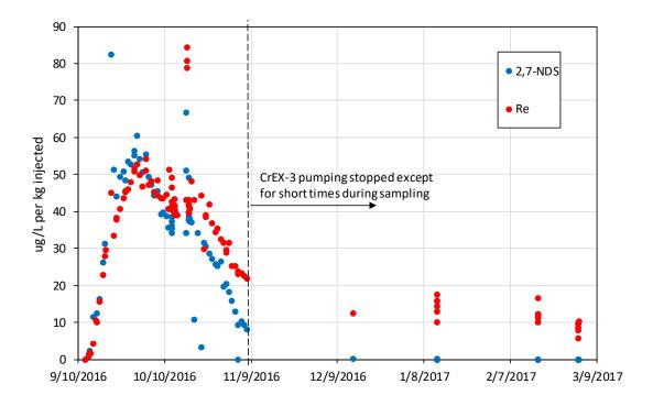
Figure 6.3-2 Normalized concentrations of tracers injected into CrPZ-2a in CrEX-3, including additional samples collected after pumping ended.
