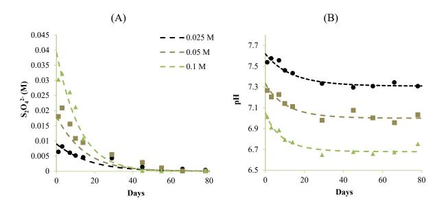
Figure 4.1-5 Simulation of experiments conducted in the HCO<sub>3</sub><sup>-</sup>-buffered solution. Panel (A) shows the dithionite concentration, and Panel (B) shows pH. The figure compares calibrated model curves (dashed lines) and experimental data (points) for the different concentrations of dithionite used in these experiments.
