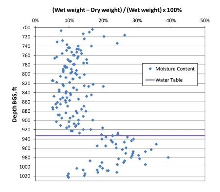
Figure A-3.0-11 Moisture content vs depth in CrCH-3
