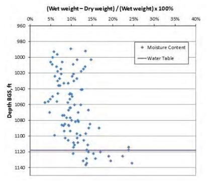
Figure A-3.0-1 Moisture content vs depth in CrCH-1
