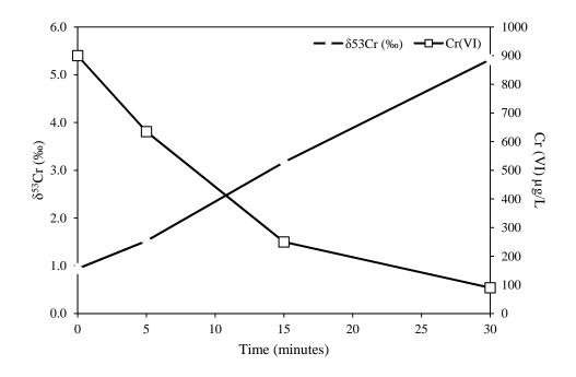
Figure 4.0-6b Experimental  $\delta^{53}$ Cr and [Cr] data for a second ZVI experiment plotted as a time series
