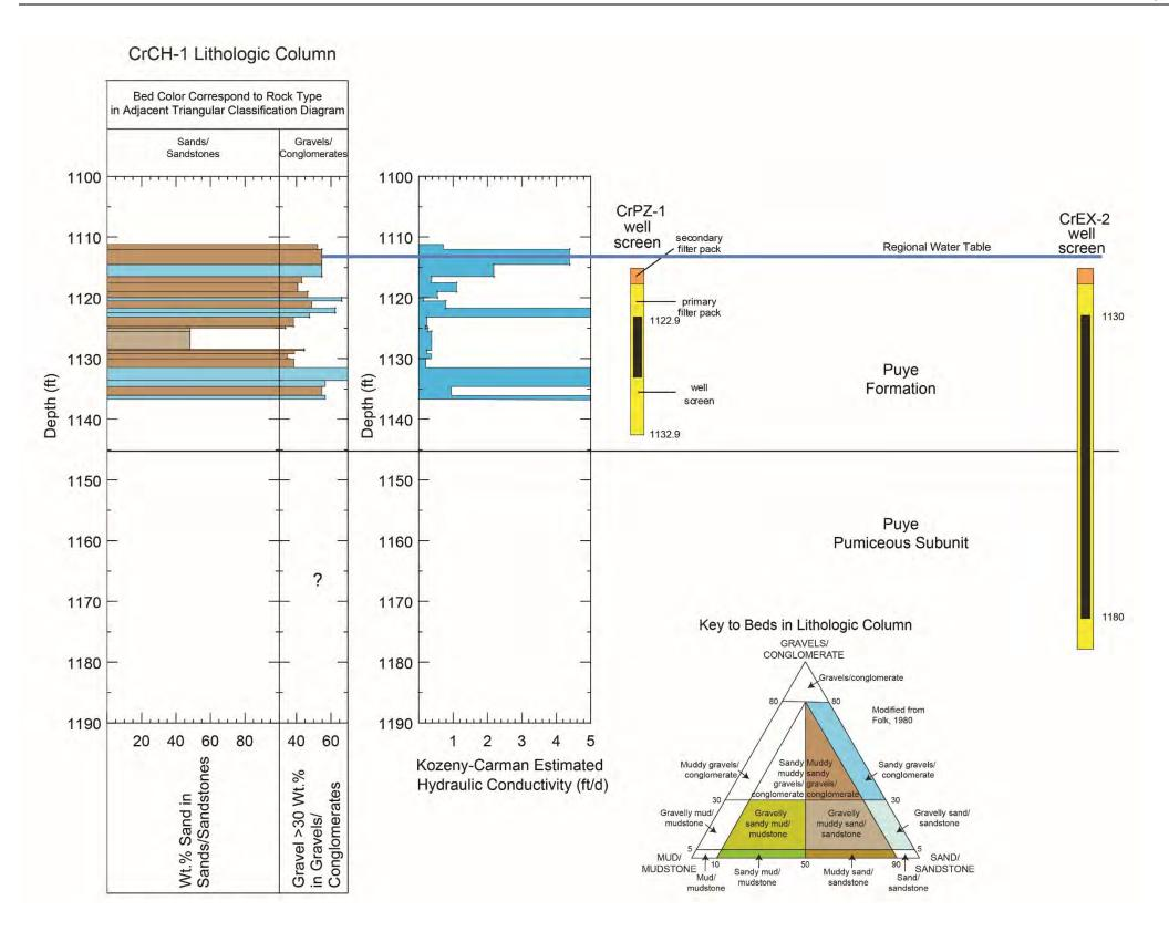
CrCH-1 lithologic column showing rock types for individual beds making up strata in the upper part of the regional aquifer. The CrPZ-1 (completed in the CrCH-1 borehole) and R-28 well screens are shown for Figure 3.3-2 reference. The contact between the Puye Formation and the Puye pumiceous subunit is based on well CrEX-2, which is located on the same drill pad. CrEX-2 did not fully penetrate the Puye pumiceous subunit at a total depth of 1240 ft.
