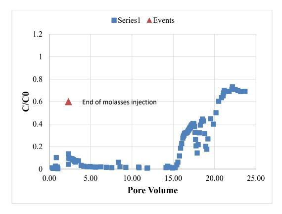
Figure 3.2-4 Chromium breakthrough in column 2 biostimulated by the injection of 2.3 pore volumes of a solution containing 3.4 g/L molasses
