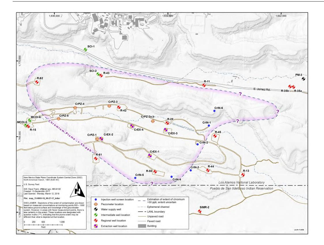
Figure 2.1-1 Map showing the footprint of the chromium plume in the regional aquifer beneath Los Alamos National Laboratory. Groundwater monitoring wells interrogating the regional aquifer (red), the deep intermediate aquifer (green), nearby water-supply wells (blue/black), and groundwater contours are shown.
