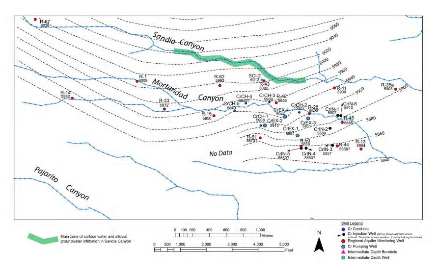
Figure B-9 Structure contour map for stratal contact in middle of Puye Formation identified using borehole gamma logs
