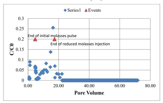
Figure 3.2-5 Chromium breakthrough in column 2 biostimulated by the injection of 4.8 pore volumes of a solution containing 3.4 g/L (10 mM) molasses followed by 12.6 pore volumes of a solution containing 0.34 g/L molasses
