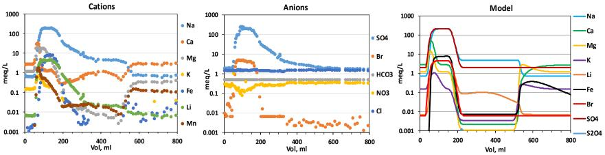
Figure 4.3-5 Breakthrough curves of cations and anions in the Miocene pumiceous column experiment and corresponding predictions of the 1-D transport model
