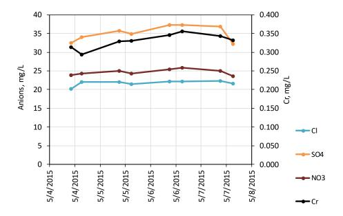
Figure A-3.0-15 Concentrations of anions and Cr as a function of time during pumping of CrCH-3 with a Bennett pump capable of about 0.5 gal. per minute
