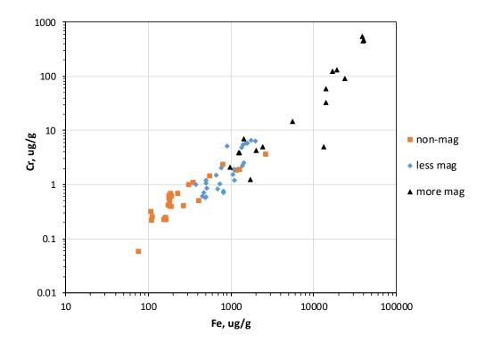
Figure 3.3-7 Cumulative log Cr vs log Fe of leachates from samples in fourth set of leaching experiments (0.1 M HNO<sub>3</sub> leaching), color coded by degree of magnetism of samples (see legend). All samples were believed to be uncontaminated.
