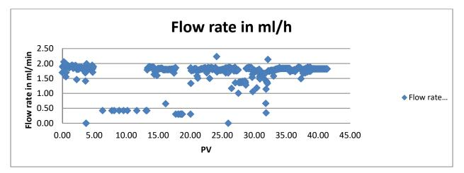
Figure 3.2-7 Flow rate for column 2 biostimulated with two successive injection of R-42 water amended with molasses
