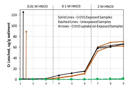
Figure 3.2-2 Cumulative chromium leached from bentonite exposed to Cr(VI) solutions as a function of leaching step in two experiments with duplicate samples in each experiment (solid lines). Green dashed lines correspond to unexposed samples. The arrows indicate the Cr(VI) uptake measured on the corresponding solid-line samples before leaching.
