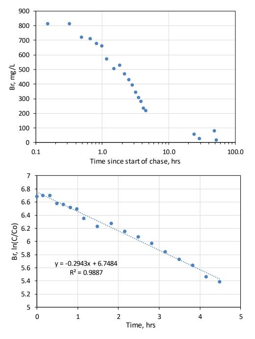
Figure 6.2-1 Decline in bromide tracer concentration observed in CrPZ-2a after the chase started in CrPZ-2b. Top: raw concentrations vs log time; bottom: In(C/Co), where Co is the initial concentration, vs time. Note that the initial concentration was essentially the same as the concentration injected into CrPZ-2b.
