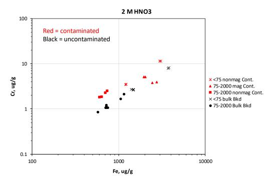
Figure 3.3-2 Cumulative log Cr vs log Fe of leachates from samples in first set of leaching experiments after 2 M HNO<sub>3</sub> leaching steps
