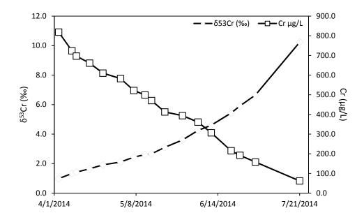
Figure 4.0-6c Microbial bioreduction experimental  $\delta^{53}$ Cr and [Cr] concentration data plotted as a time series
