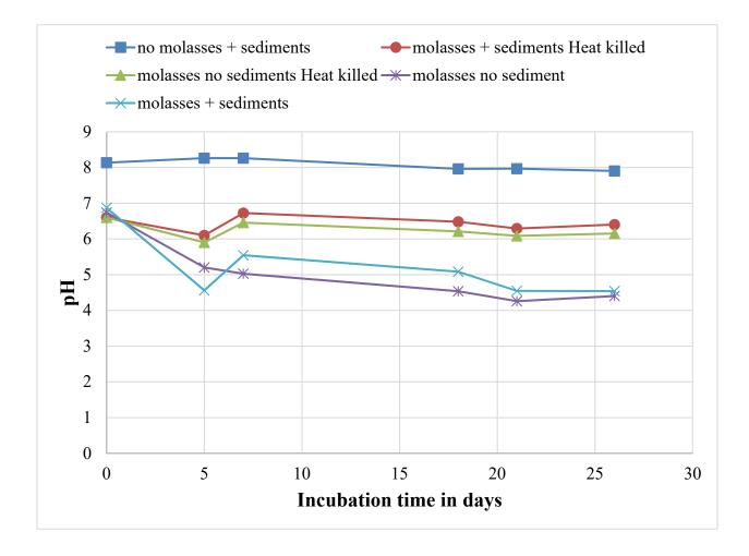
Figure 3.1-13 Changes in pH during the microcosm experiment biostimulated with molasses. The molasses concentration was fixed in all reactors to 1.8 g/L.
