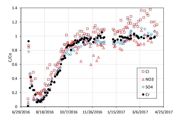
Figure 5.0-1 Concentrations of major anions and Cr(VI) in R-42 during the drift phase of the high-pH push-drift test at R-42. Concentrations are expressed as fractions of pretest concentrations.
