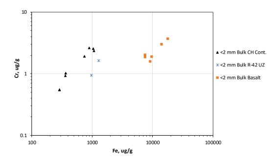
Figure 3.3-4 Cumulative log Cr vs log Fe of leachates from samples in second set of leaching experiments (0.1 M HNO<sub>3</sub> leaching). All samples were considered potentially contaminated.
