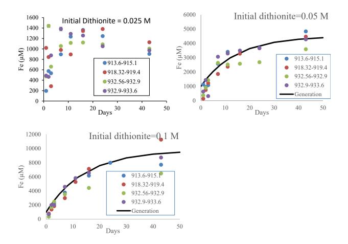
Figure 4.3-2 Iron generation in batch experiments with four different sediments (identified by depth [ft] from CrCH-2) with 10 mL of solution for every 5 g sediment. Curves were generated using the kinetic model discussed in text.
