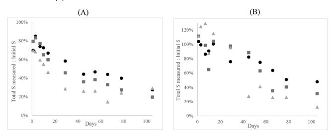
Figure 4.1-4 Percent recovery of S relative to the starting amount in HCO<sub>3</sub><sup>-</sup>-buffered (A) and EDTA/OH<sup>-</sup>-buffered (B) solutions
