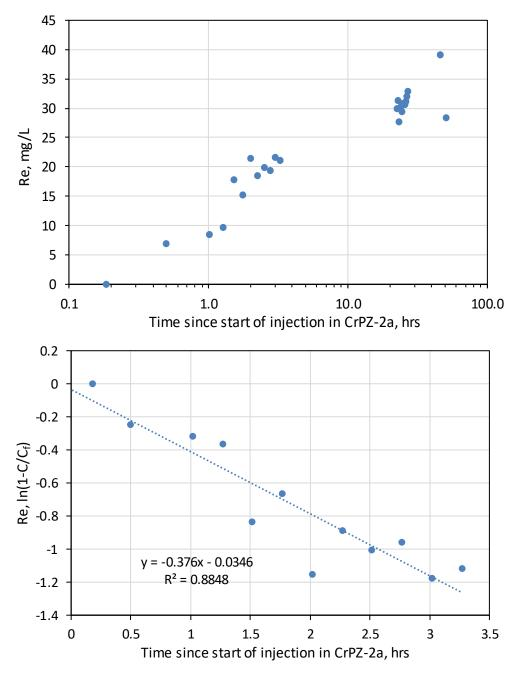
Figure 6.2-2 Rise in rhenium tracer concentration observed in CrPZ-2b after the tracer injection started in CrPZ-2a (top). Bottom figure is a plot of In(1-C/Cf), where Cf is the final concentration, vs time. Note that the final concentration was essentially the same as the injection concentration in CrPZ-2a (a little over 30 mg/L Re).
