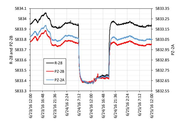
Figure 6.1-3 Pressure responses in CrPZ-2a, CrPZ-2b, and R-28 during 12-h pump test of CrEX-3 (at ~40 gpm)
