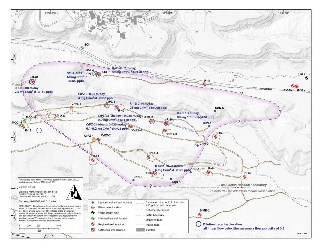
Figure 2.0-1 Locations of dilution tracer tests with estimated linear groundwater flow velocities and Cr(VI) fluxes at each of the locations
