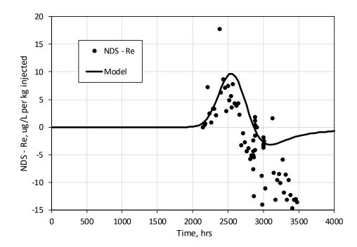
Figure 6.3-4 Model match to *differences* in normalized breakthrough curves of tracers injected into CrPZ-2a in CrEX-3. The model results are the same as for Figure 6.3-3. Note that the late-time differences are poorly matched presumably because of the degradation of 2,7 NDS.
