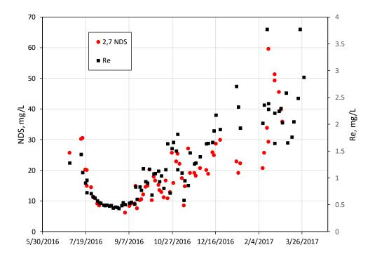
Figure 6.2-3 Concentration histories of tracers injected into CrPZ-2a measured in passive samples collected from CrPZ-2a after the injection and chase
