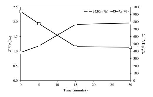
Figure 4.0-6a Experimental  $\delta^{53}$ Cr and [Cr] data for the initial ZVI experiment plotted as a time series
