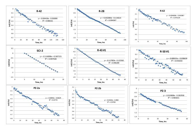
Figure 2.0-2 Tracer concentration histories (In C/Co vs time) in each dilution tracer test (plots intended to show quality of the test data)
