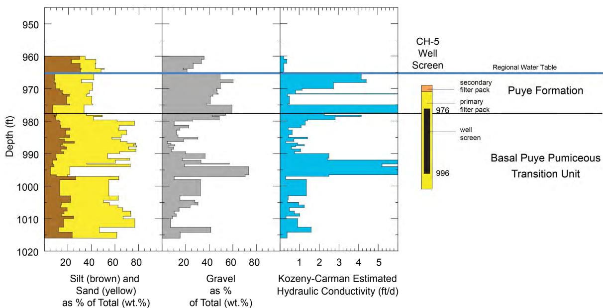
Figure 3.3-13 CrCH-5 grain-size variations for beds making up strata in the upper part of the regional aquifer. CrPZ-5 well screen, which was completed in the CrCH-5 bore hole, is shown for reference.
