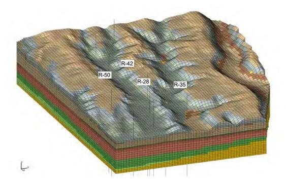
Figure 1.1-2 Block diagram showing the computational grid of the chromium 3-D vadose-zone / regional-aquifer model. View is towards the northwest and the canyons, from left to right, are Mortandad, Sandia, and Los Alamos. Vertical lines show well locations. Y-axis indicates north.
