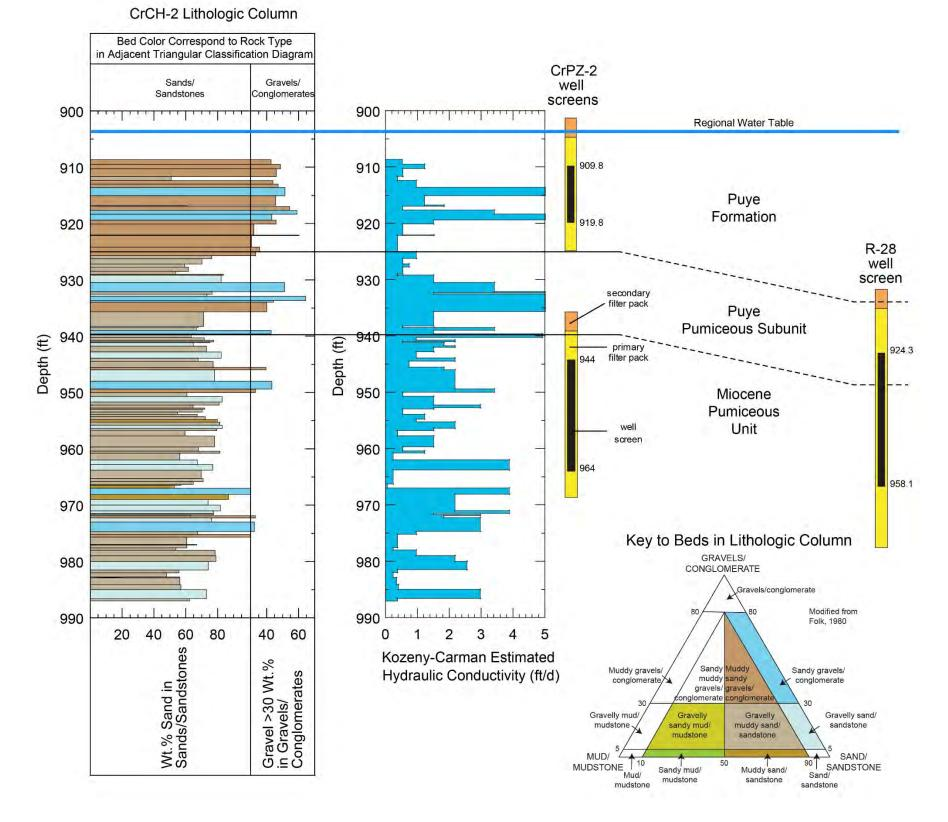
Figure 3.3-5 CrCH-2 lithologic column showing rock types for individual beds making up strata in the upper part of the regional aquifer. CrPZ-2 (completed in the CrCH-2 borehole) and R-28 well screens are shown for reference.
