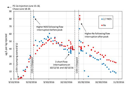
Figure 6.3-1 Normalized breakthrough curves of tracers injected into CrPZ-2a in CrEX-3 during pumping of CrEX-3
