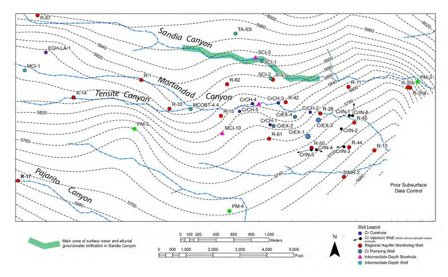
Figure B-10 Structure contour map for base of Puye Formation. Contours based on the sitewide geologic model. Wells installed after 2015 shown for reference.
