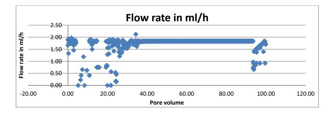
Figure 3.2-6 Flow rate for column 4 biostimulated with an injection of R-42 water amended with molasses
