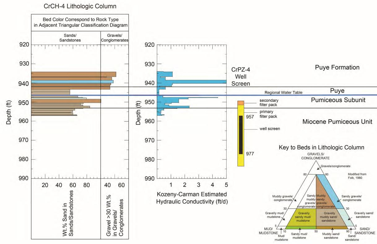
Figure 3.3-12 CrCH-4 lithologic column showing rock types for individual beds making up strata in the upper part of the regional aquifer. CrPZ-4 well screen, which was completed in the CrCH-4 bore hole, is shown for reference.
