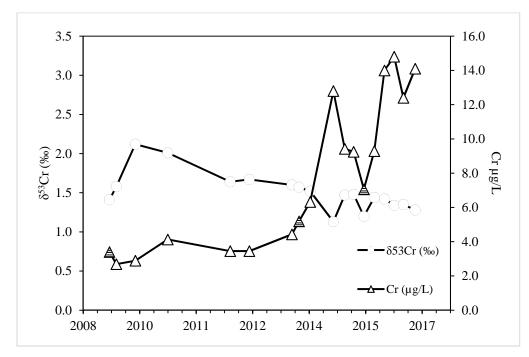
Figure 4.0-2b R-43(2) quarterly  $\delta^{53}$ Cr sampling analysis with corresponding [Cr] from 2008 to 2016. Total chromium data were included in the study data set only if a  $\delta^{53}$ Cr sample was acquired during the same time period. Hashed triangles represent non-detect samples for [Cr].
