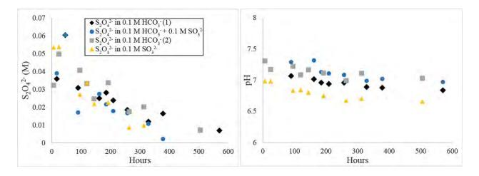
Figure 4.1-8 Anaerobic decomposition of dithionite in background solutions of  $HCO_3^-$ ,  $SO_3^{2^-}$ , and  $HCO_3^- + SO_3^{2^-}$
