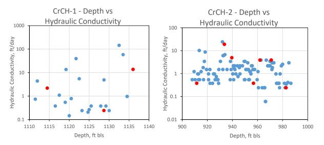
Figure 2.3-8 Hydraulic conductivity (as deduced from particle-size distribution data using the Kozeny-Carman equation) vs depth for lithologically distinct intervals in CrCH-1 and CrCH-2. Red data points correspond to material used in Cr(VI) batch uptake experiments.
