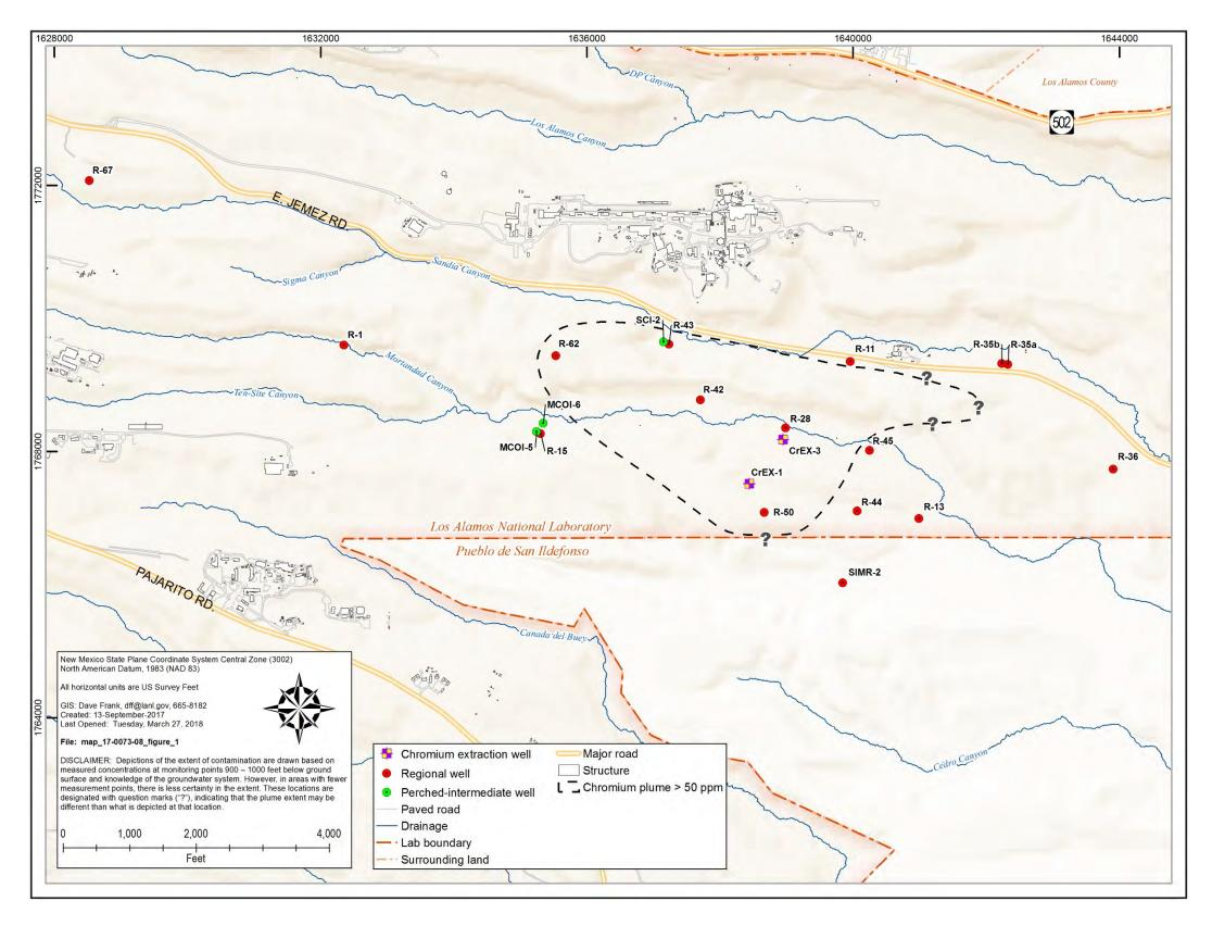
Location Map showing outfalls, the Sandia Canyon wetland, the primary Cr(VI) infiltration zone, location of monitoring wells, and the area of Cr(VI) concentration Figure 1.0-1 exceeding 50 µg/L in the regional aquifer. Well WST-600902 is off the map to the west, outside the area of influence of the chromium plume.
