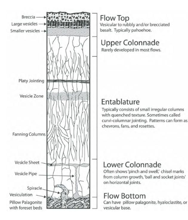
Figure 2.4-1Diagram showing typical internal features in a basalt lava flow (after Reidel et al.<br/>2013). The figure is idealized and not all features are present for every flow.
