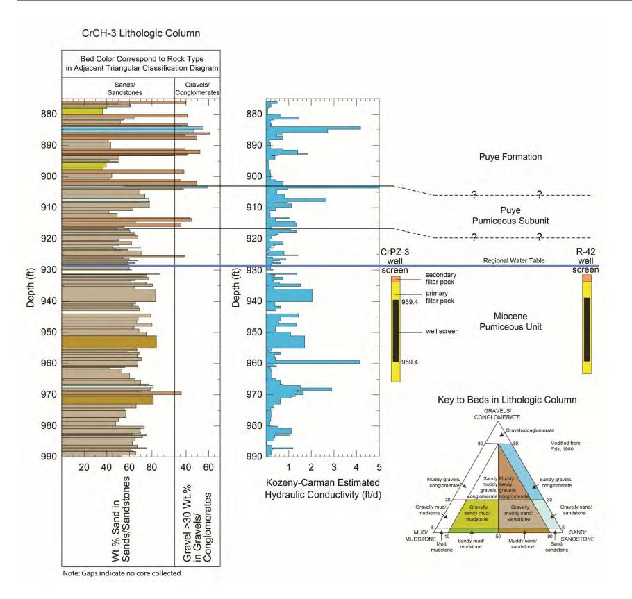
Figure 3.3-10 CrCH-3 lithologic column showing rock types for individual beds making up strata in the upper part of the regional aquifer. CrPZ-3 (completed in the CrCH-3 borehole) and R-42 well screens are shown for reference.
