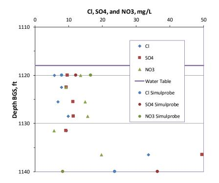
Figure A-3.0-4 Anion concentrations in pore water below the water table vs depth in CrCH-1. Simulprobe samples are included and shown as circles.
