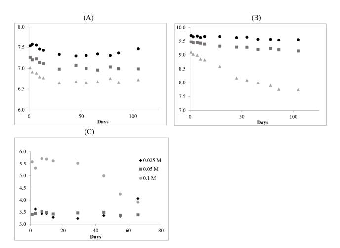
Figure 4.1-3 pH through time in HCO<sub>3</sub><sup>-</sup>-buffered (A), EDTA/OH<sup>-</sup>-buffered (B), and unbuffered (C) solutions
