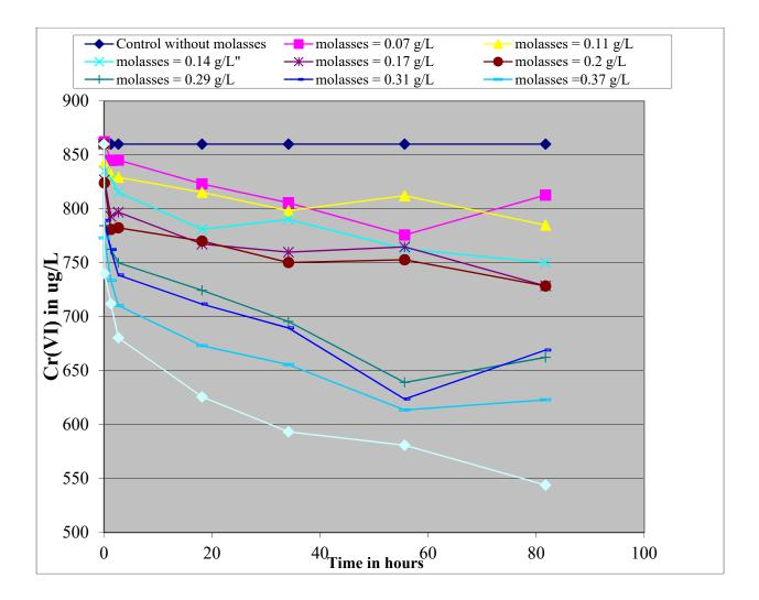
Figure 3.1-12 Chromate reduction by molasses under sterile conditions. Molasses was sterile filtered using 0.2 µm syringe filters. The pH of the groundwater was pH = 8.8 and did not change.
