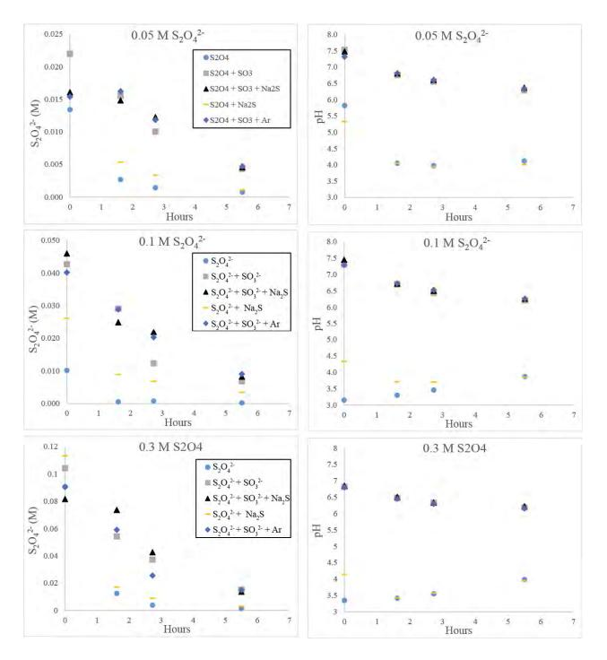
Figure 4.1-7 Decomposition of  $S_2O_4^{2-}$  in various buffer solutions left open to the atmosphere and accompanying pH measurements
