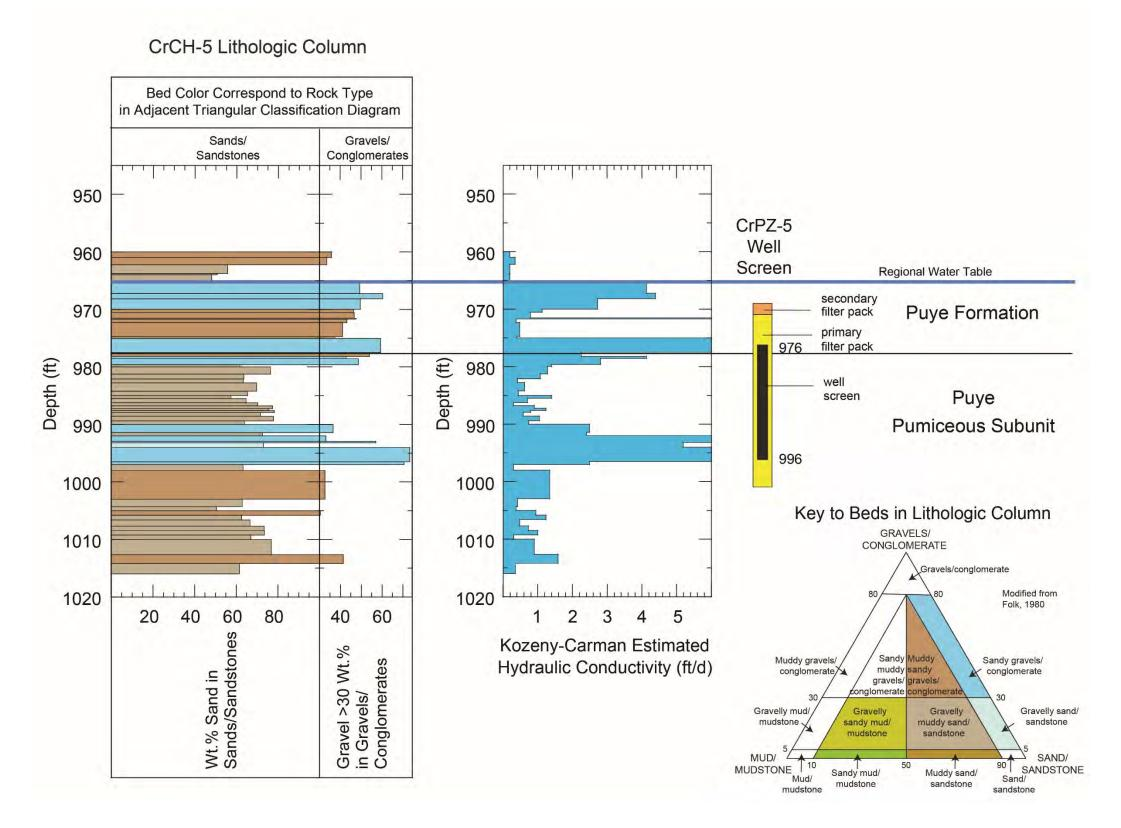
Figure 3.3-14 CrCH-5 lithologic column showing rock types for individual beds making up strata in the upper part of the regional aquifer. CrPZ-5 well screen, which was completed in the CrCH-5 bore hole, is shown for reference.
