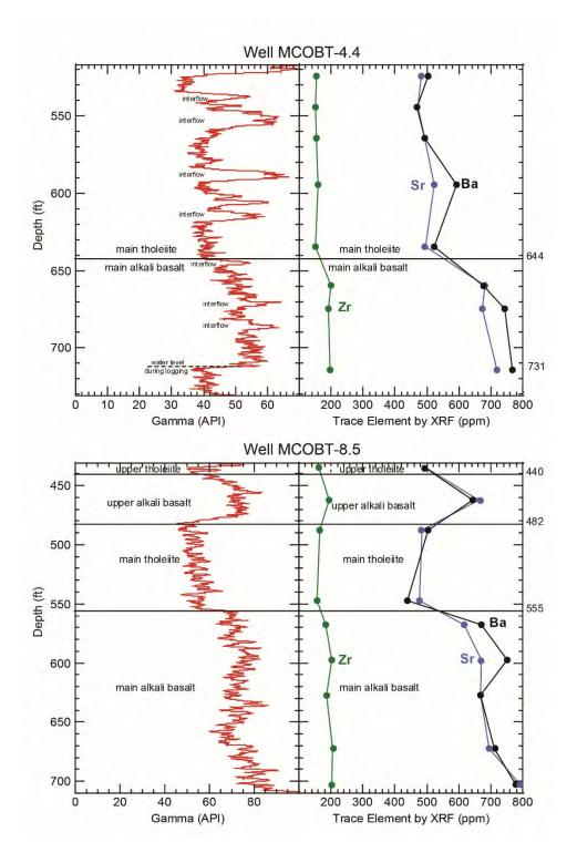
Figure 2.3-2 Borehole gamma and trace element (zirconium, strontium, and barium) plots for the Cerros del Rio basalt in wells MCOBT-4.4 and MCOBT-8.5. Differentiation of tholeiites and alkali basalts based on gamma activity is supported by XRF chemical data collected for cuttings samples (WoldeGabriel and Broxton, unpublished data).
