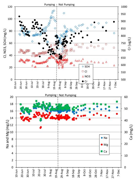
Figure 4.0-1 Concentrations of key constituents in R-42 during the long-term pumping test of R-42 in 2013, including the period after pumping ended (top: major anions and Cr(VI), bottom: major cations). Note the difference in the Cr concentration scale in the upper plot. The rise in concentration of SO₄<sup>=</sup> and Cl<sup>-</sup> before pumping ended, followed by the drop after pumping ended, are believed to be an analytical artifact (see Figure 4.0-2).
