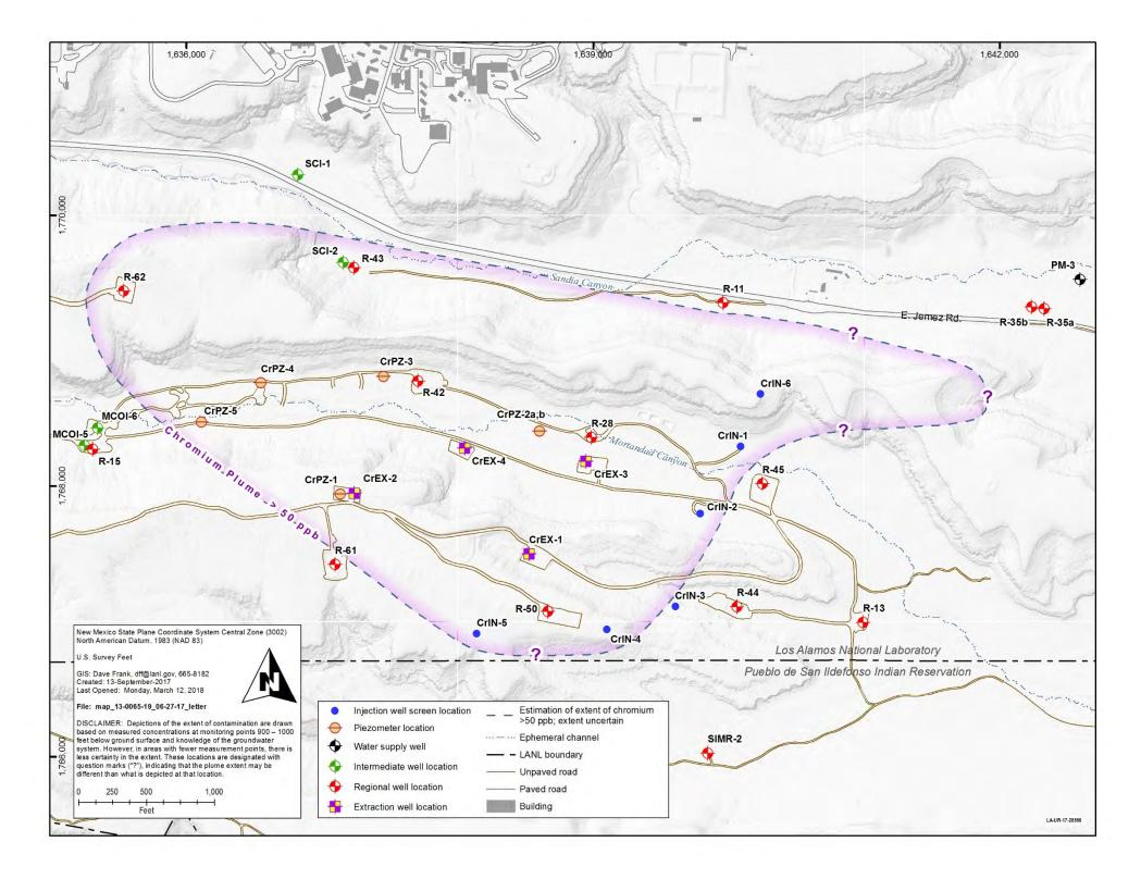
Map showing the approximate extent of the hexavalent chromium plume as defined by the 50-µg/L New Mexico groundwater standard. Locations of monitoring wells, piezometers, extraction wells and injection Figure 1.0-1 wells are also shown.
