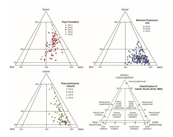
Figure 3.4-5 Folk (1980) clastic rock classification applied to the Pliocene and Miocene rocks at the top of the regional aquifer beneath Mortandad Canyon based on particle-size data for cores collected from CrCH-1, CrCH-2, CrCH-3, CrCH-4, and CrCH-5
