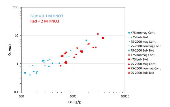
Figure 3.3-1 Cumulative log Cr vs log Fe of leachates from both contaminated and uncontaminated samples in first set of leaching experiments after 0.1 M HNO<sub>3</sub> leaching steps (blue) and 2 M HNO<sub>3</sub> leaching steps (red).
