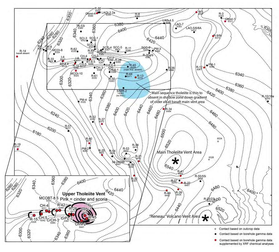
Structure contour map for top of tholeiites of the main tholeiites/alkali basalt sequence of the Cerros del Rio basalt. The inset map shows the top of the tholeiites in upper tholeiites/alkali basalt sequence (thick Figure B-6 black contours) superimposed on the top of the main tholeiite structure contours (dashed lines). The upper tholeiite/alkali basalt flows are present only in wells shown in inset.
