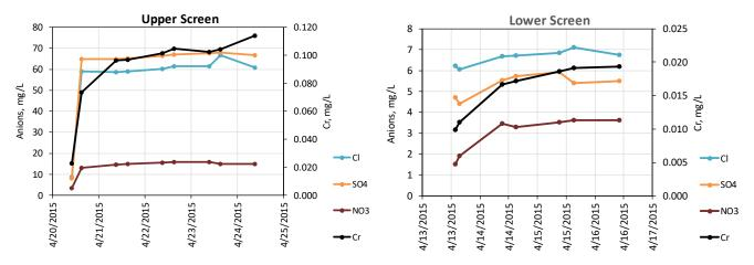
Figure A-3.0-10 Concentrations of anions and Cr as a function of time during pumping of both piezometers (upper and lower screens) of CrCH-2 with a Bennett pump capable of about 0.5 gal. per minute
