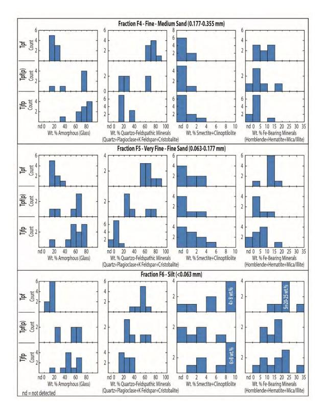
Figure 3.4-6 Histograms showing selected mineralogy for the F4, F5, and F6 particle-size fractions of Pliocene and Miocene rocks in the upper regional aquifer beneath Mortandad Canyon. Rock units include the Puye Formation (Tpf), Puye pumiceous subunit [Tpf(p)], and Miocene pumiceous unit (Tjfp). nd indicates Not detected by XRD
