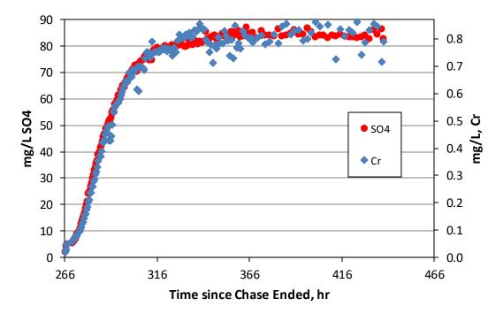
Figure 3.3-1 Breakthroughs of SO₄<sup>=</sup> and Cr(VI) in R-42 during the pull phase of the push-pull test in R-42
