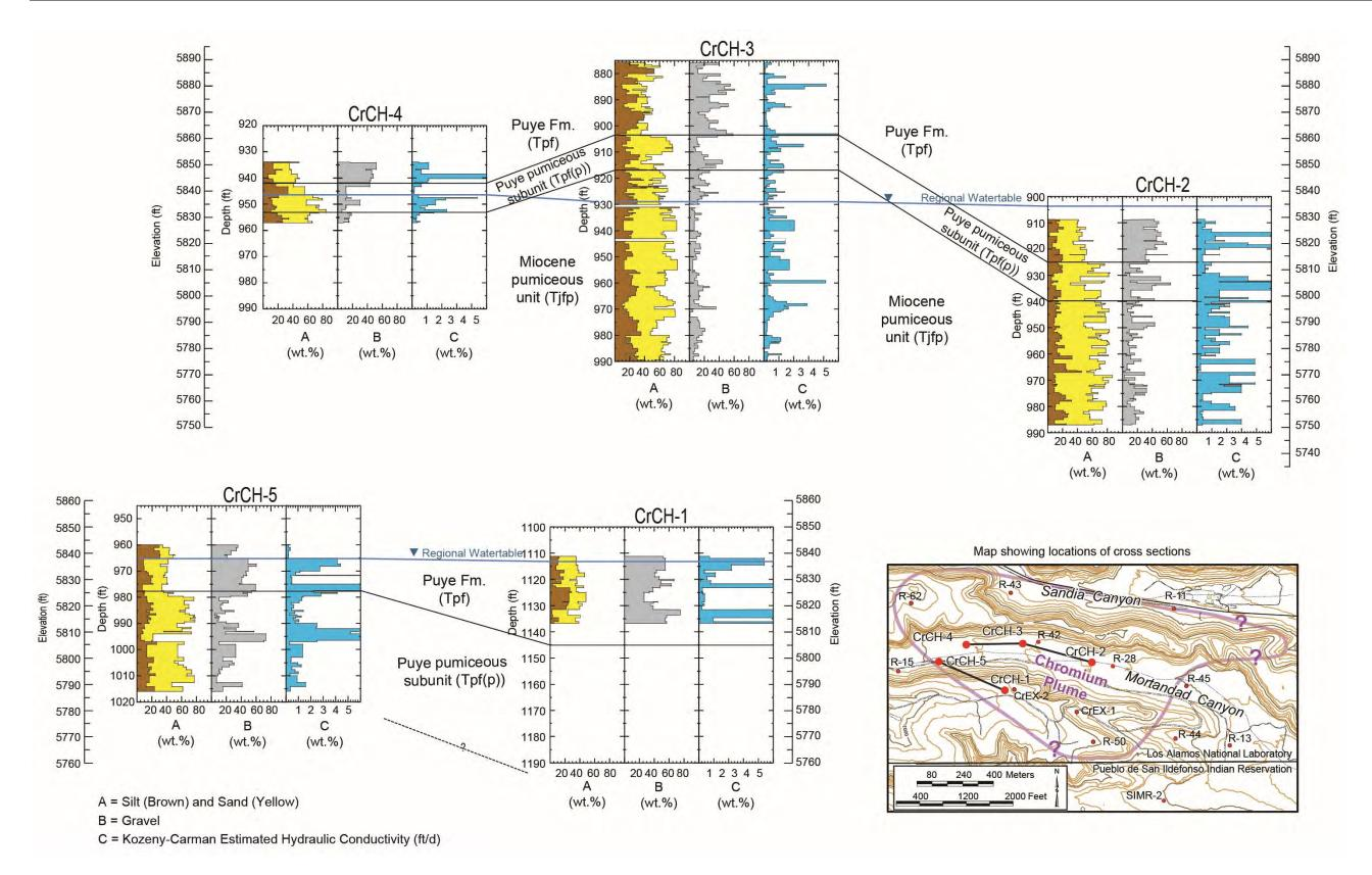
Figure 3.4-7 Schematic cross-sections portraying the aquifer hydraulic structure based on particle-size data and estimates of hydraulic conductivity for CrCH-1, CrCH-2, CrCH-3, CrCH-4, and CrCH-5
