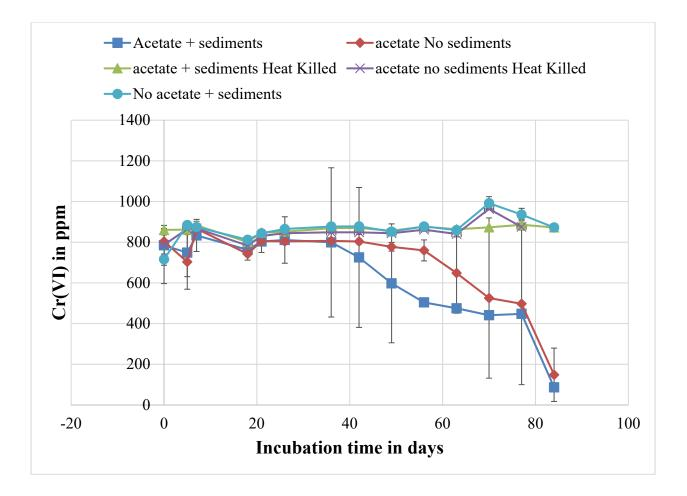
Figure 3.1-8 Chromate reduction in liquid cultures amended with 0.82 g/L acetate and incubated anaerobically in the presence and absence of sediments. Reactors received 100 mL of R-42 water and 1.0 g of sediments. Heat killed control reactors were autoclaved to sterilize the reactors.
