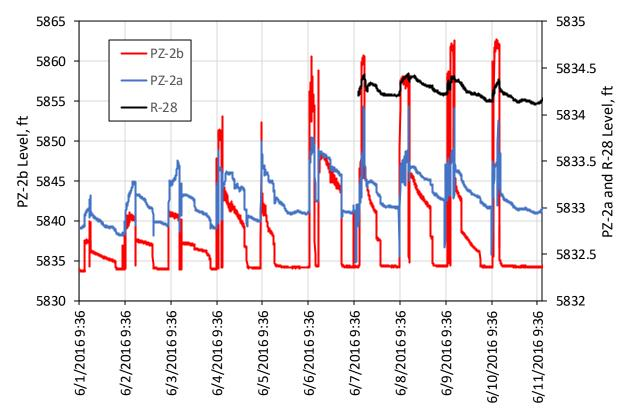
Figure 6.1-1 Pressure responses in CrPZ-2a, CrPZ-2b and R-28 during the tracer and chase injections into CrPZ-2b
