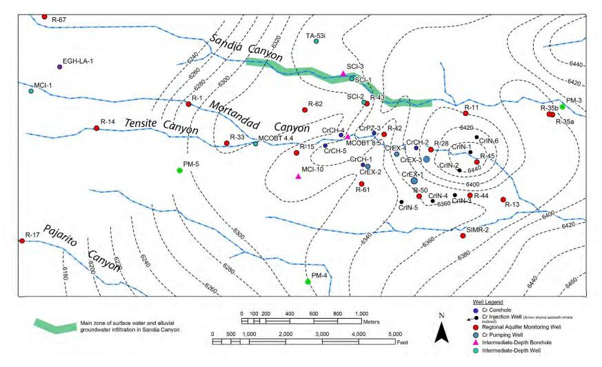
Figure B-5 Structure contour map for Cerros del Rio basalt (Tb4 undivided). Shows eroded top of all Tb4 basalt types (tholeiites and alkali basalts) regardless of source areas. Contours based on the sitewide geologic model. Wells installed after 2015 shown for reference.
