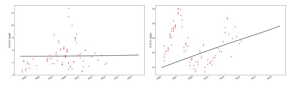
Figure 2.2-2 (continued) The model-predicted (black line) vs the observed (red dots) chromium concentrations at the site monitoring wells. The predicted concentrations are based on the best values estimated for the model parameters. These concentrations also represented the "central" tendencies of the multiple realizations presented in Figure 2.2-7 below.
