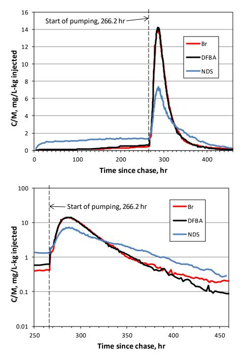
Figure 3.1-1 Normalized tracer concentrations as a function of time in the R-42 push-pull tracer test. Top shows entire test duration after chase, and bottom shows only the pumping period with a log scale for concentrations. Bromide concentrations were not background-subtracted.
