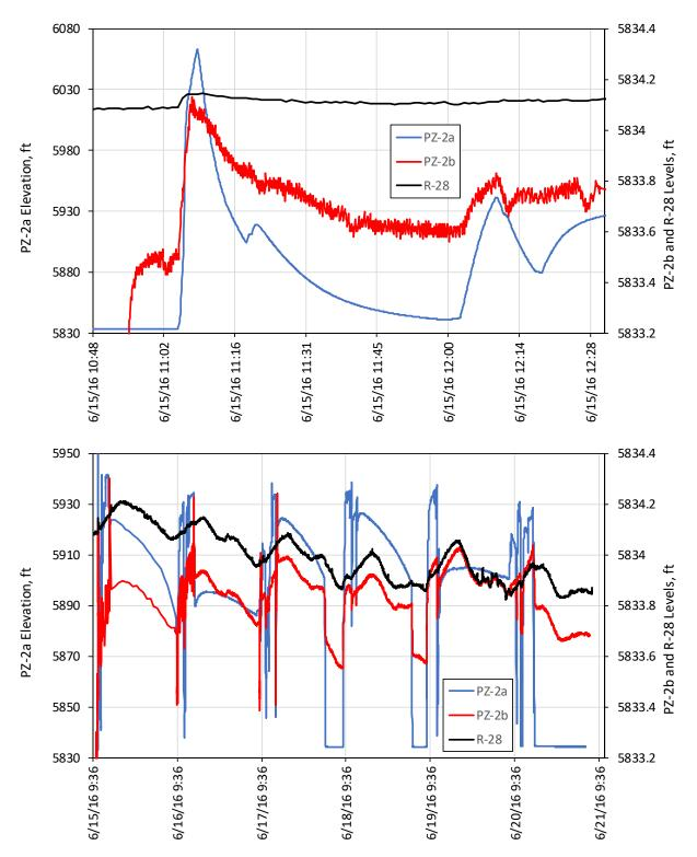
Figure 6.1-2 Pressure responses in CrPZ-2a, CrPZ-2b and R-28 during the tracer and chase injections into CrPZ-2a. Top shows responses to initial pressure spike in CrPZ-2a when injection rate was discovered to be too high, and bottom shows the entire history of the injection.
