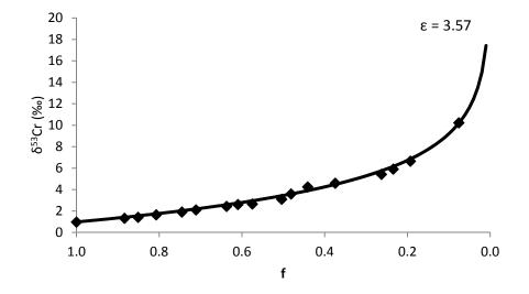
Figure 4.0-7b Microbial reduction experimental  $\delta^{53}$ Cr and associated f with  $\epsilon$  = 3.57
