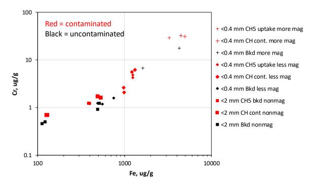
Figure 3.3-6 Cumulative log Cr vs log Fe of leachates from samples in third set of leaching experiments (0.1 M HNO<sub>3</sub> leaching), color coded by contaminated or uncontaminated
