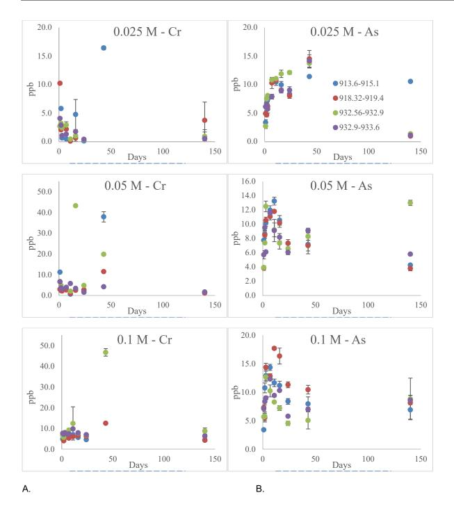
Figure 4.3-3 Release of Cr (A) and As (B) from batch sediments. The molarity indicates the starting concentration of the dithionite solution.
