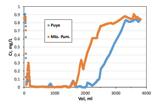
Figure 4.3-7 Cr(VI) breakthroughs in the two dithionite column experiments.
