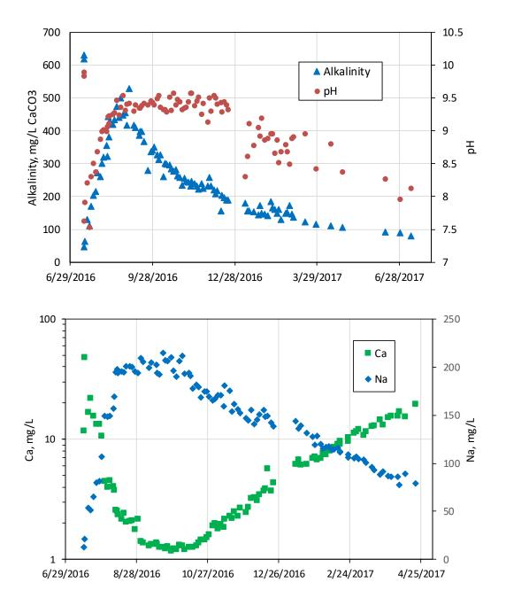
Figure 5.0-2 pH, alkalinity, and sodium and calcium concentrations in R-42 during the drift phase of the high-pH push-drift test at R-42. Note the log scale for calcium.
