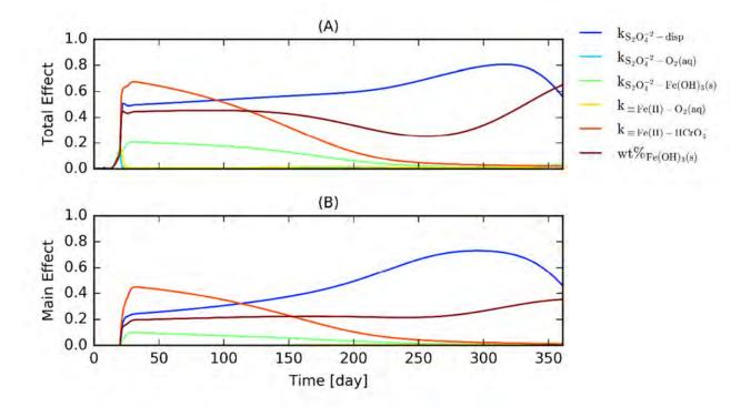
Figure 2.3-9 Global sensitivity analysis (eFAST) of geochemical treatment model. See Table 2.3-2 for a description of the parameters.
