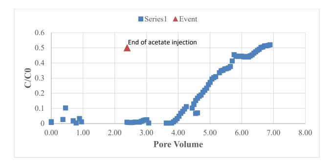
Figure 3.2-2 Chromium attenuation in column 3 biostimulated by the injection of 2.4 pore volumes of a solution containing 0.82 g/L (10 mM) ae
