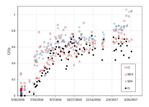
Figure 6.2-4 Concentrations of major anions and Cr(VI) in CrPZ-2a measured in passive samples collected from CrPZ-2a after the injection and chase, which were both potable water. Concentrations are expressed as fractions of pretest concentrations.
