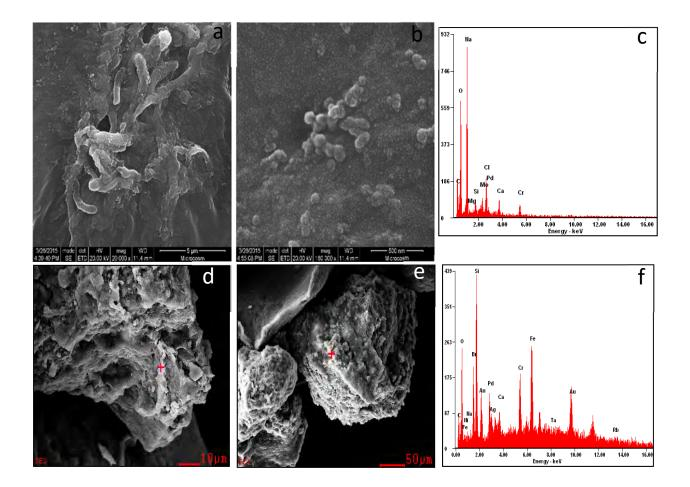
Figure 3.2-10 SEM images of microorganisms and biofilm coatings on sediment grains and EDS spectra. (a) Microbial cells coated with massive Cr(III) precipitates; (b) spherical aggregates of biogenic Cr(III) precipitates; (C) EDS spectrum of the surface of biofilm containing chromium precipitates; (d, e) sediment grains with biofilm coatings; (f) EDS spectrum from the surface of sediment grains coated with biofilm.
