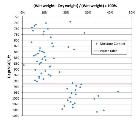
Figure A-3.0-16 Moisture content vs depth in CrCH-4
