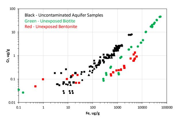
Figure 3.2-3 Cumulative log Cr vs log Fe of leachates from uncontaminated aquifer samples (black), unexposed biotite (green), and unexposed bentonite (red). Data for all nine steps of sequential acid leaching (0.01 M, 0.1 M, and 2 M HNO<sub>3</sub>) are shown (cumulative amounts after each step). Aquifer samples have higher Cr/Fe ratios than either biotite or bentonite.
