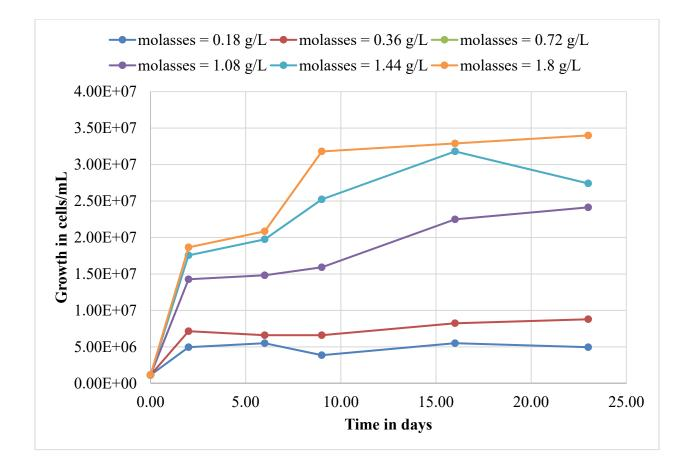
Figure 3.1-3 Microbial growth in reactors biostimulated with molasses and incubated anaerobically. Initial conditions are: Water used from R-42 with 888 μg/L Cr(VI). Initial pH = 8.8 and final pH = 4.85.
