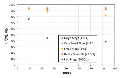
Figure 2.3-3 Results of batch uptake experiments conducted on different fractions separated from bulk sonic core from CrCH-4, 967 ft below land surface (BLS). All experiments were conducted using R-42 water with a starting concentration of ~950 μg/L Cr(VI), and the y-axis is the concentration of Cr(VI) remaining in solution. The iron fragments were separated from the core material. Numbers in parentheses in the legend are the solution-to-solid mass ratio for each fraction.
