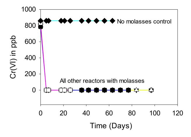
Figure 3.1-11 Bioreduction of chromate in reactors amended with molasses in the absence and presence sediments. A control with degassed R-42 water was setup as a control without addition of molasses.
