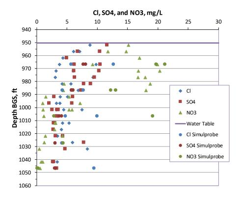
Figure A-3.0-19 Anion concentrations in pore water below the water table vs depth in CrCH-4. Simulprobe samples are included and shown as circles.
