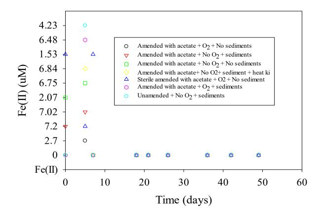
Figure 3.1-9 Concentration of ferrous iron in the different reactors stimulated with acetate
