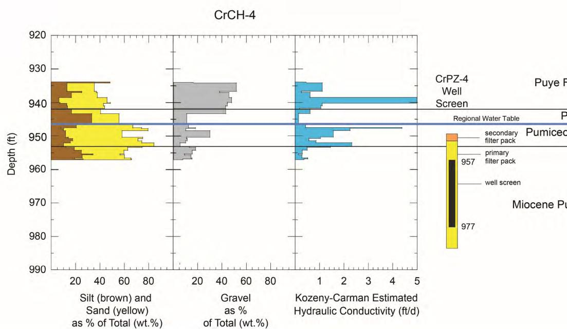
Figure 3.3-11 CrCH-4 grain-size variations for beds making up strata in the upper part of the regional aquifer. CrPZ-4 well screen, which was completed in the CrCH-4 bore hole, is shown for reference.
