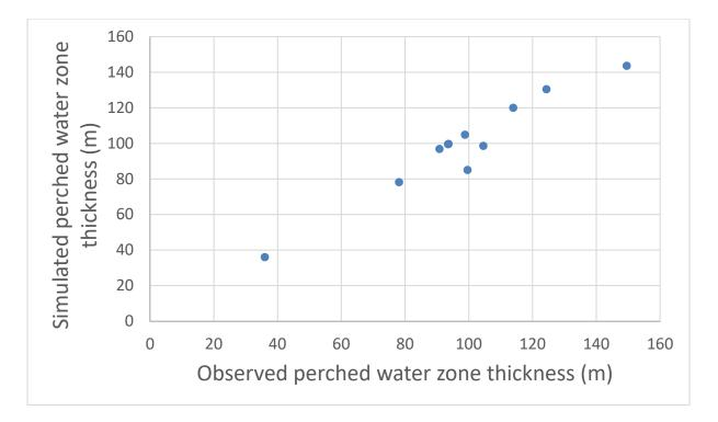
Figure 2.1-4 Simulated vs observed thicknesses of the perched-intermediate saturated zone at 11 calibration target locations. Perfect matches will be along 1:1 line.
