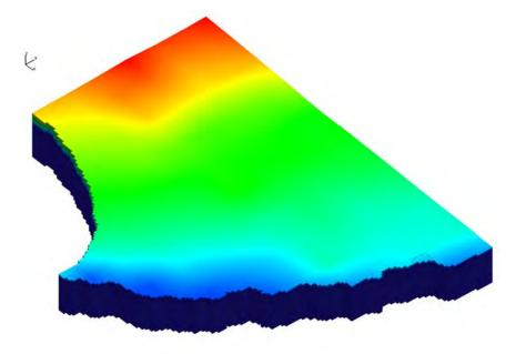
Figure 1.2-1 Block diagram showing the grid used for the regional-scale aquifer model. View is towards the northwest and the y-axis indicates north. The coloring represents the elevation of the regional-aquifer water table in 2012. The red regions to the west are high pressures in the area of mountain-front recharge beneath the Sierra de los Valles. The blue regions to the east represent the impact of discharge near the Rio Grande.
