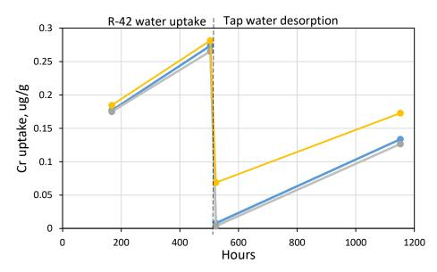
Figure 2.3-7 Cr(VI) uptake onto material from CrCH-5, 998–1005 ft BLS, which did not settle by gravity after 120 h, and subsequent desorption of Cr(VI) after exposure to Los Alamos tap water. Solution-to-solid mass ratios ranged from about 0.7:1 to 1.4:1.
