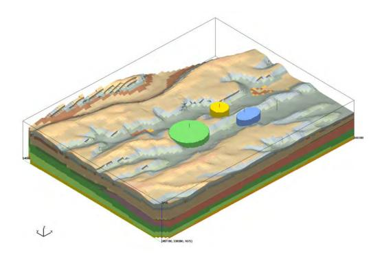
Figure 1.1-3 Block diagram showing the computational grid and locations of three hydraulic windows in the perched water zone above the regional aquifer. Each ellipse is intersected by the reduction zone inside the basalts and near well locations R-42, R-62, and R-43. View is towards the northeast with the y-axis indicating north.
