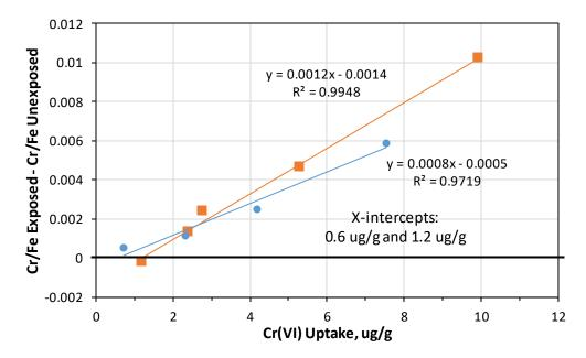
Figure 3.2-6 Cumulative Cr/Fe ratios of 0.1 M HNO<sub>3</sub> leachates from Cr(VI)-exposed biotite samples minus Cr/Fe ratio of leachates from unexposed biotite samples vs Cr(VI) uptake on exposed samples. Each data point is the average of two duplicate measurements. X-intercepts of linear regression lines are estimates of method detection limit for Cr(VI) uptake on biotite.
