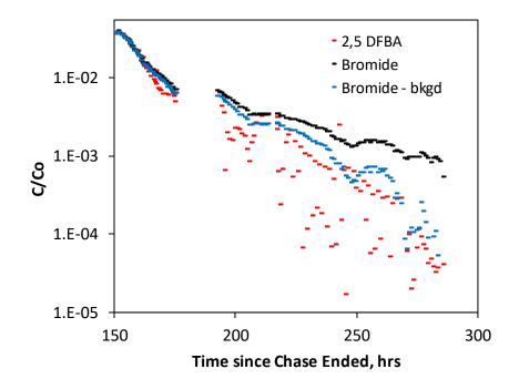
Figure 3.1-2 Normalized tracer concentrations as a function of time in the R-28 push-pull tracer test. Bromide concentrations are background-corrected in upper plot. Bottom plot shows late-time data with log concentration scale, highlighting differences between raw bromide and background-subtracted bromide concentrations. Note that concentrations are plotted as fractions of injection concentrations (as opposed to concentration divided by injection mass).
