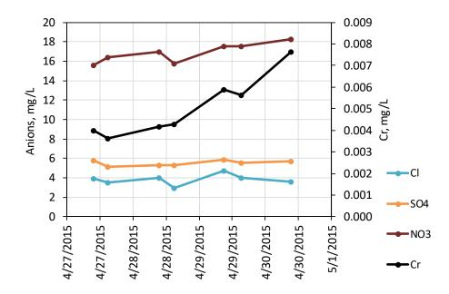
Figure A-3.0-20 Concentrations of anions and Cr as a function of time during pumping of CrCH-4 with a Bennett pump capable of about 1 gal. per minute
