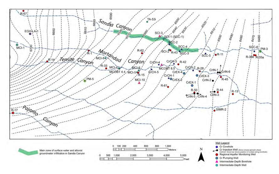
Figure B-3 Structure contour map for stratal contact in middle of Otowi Member identified using borehole gamma logs
