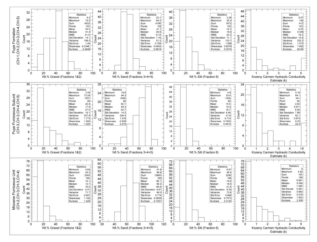
Figure 3.4-3 Histograms for grain size and estimated hydraulic conductivity of Pliocene and Miocene rocks in the upper regional aquifer beneath Mortandad Canyon
