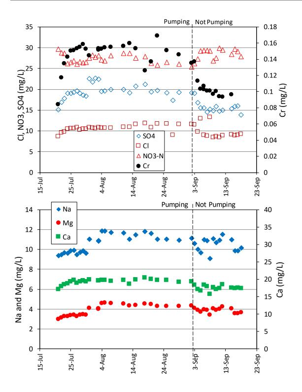
Figure 4.0-5 Concentrations of key constituents in R-43 S1 during the long-term pumping test of R-43 S1 (at 7–8 gpm), including the period immediately after pumping ended
