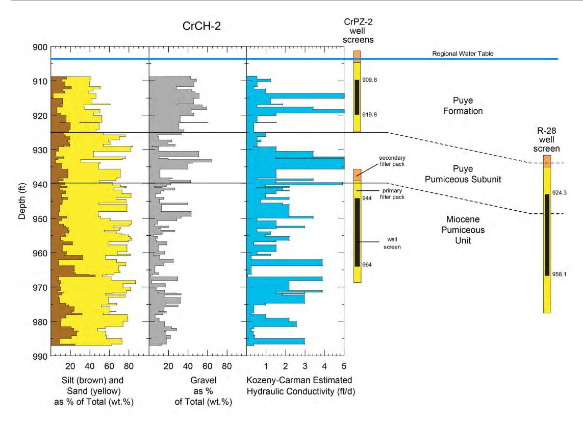
Figure 3.3-4 CrCH-2 grain-size variations for beds making up strata in the upper part of the regional aquifer. CrCPZ-2 (completed in the CrCH-2 borehole) and R-28 well screens are shown for reference.
