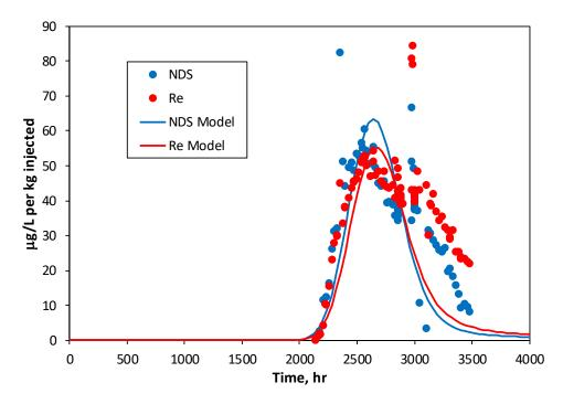
Figure 6.3-3 Model match to normalized breakthrough curves of tracers injected into CrPZ-2a in CrEX-3 through the end of pumping on 12/7/2016. Note that the model does not attempt to match the responses to flow interruptions.
