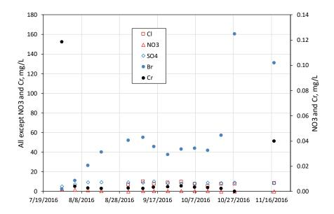
Figure 6.2-5 Concentration histories of major anions, bromide tracer, and Cr(VI) in CrPZ-2b, measured in passive samples collected from CrPZ-2b after the injection and chase. Note that the initial high Cr(VI) concentration is possibly a signature of water from CrPZ-2a that was pushed down into CrPZ-2b during the CrPZ-2a injection (the Cr value is higher than anything ever measured in CrPZ-2b, but somewhat lower than pretest Cr concentrations in CrPZ-2a).
