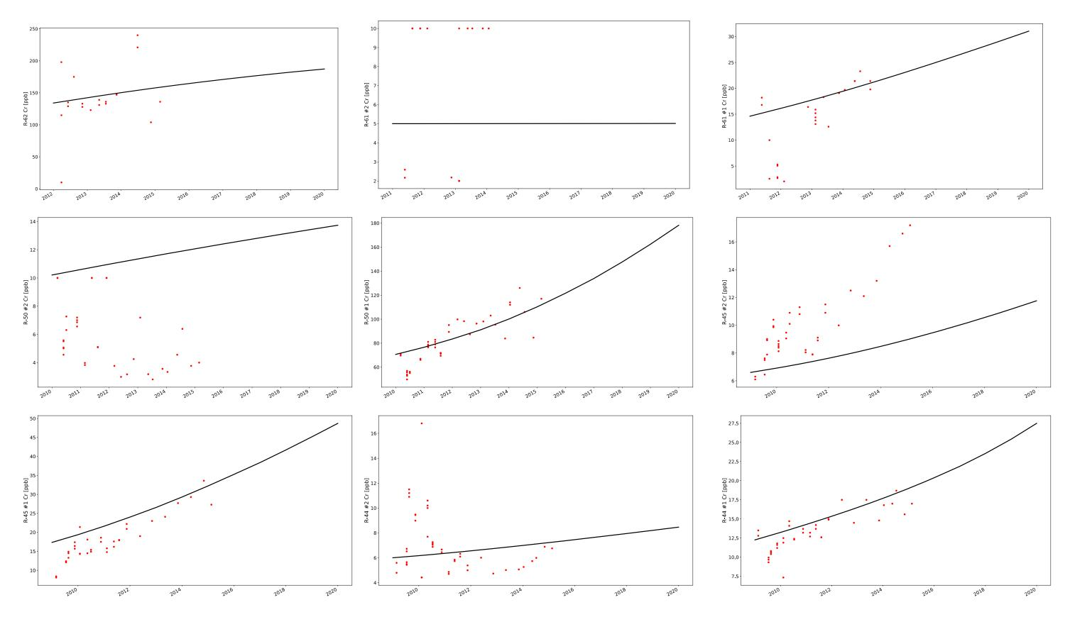
Figure 2.2-2 The model-predicted (black line) vs the observed (red dots) chromium concentrations at the site monitoring wells. The predicted concentrations are based on the best values estimated for the model parameters. These concentrations also represented the "central" tendencies of the multiple realizations presented in Figure 2.2-7 below.
