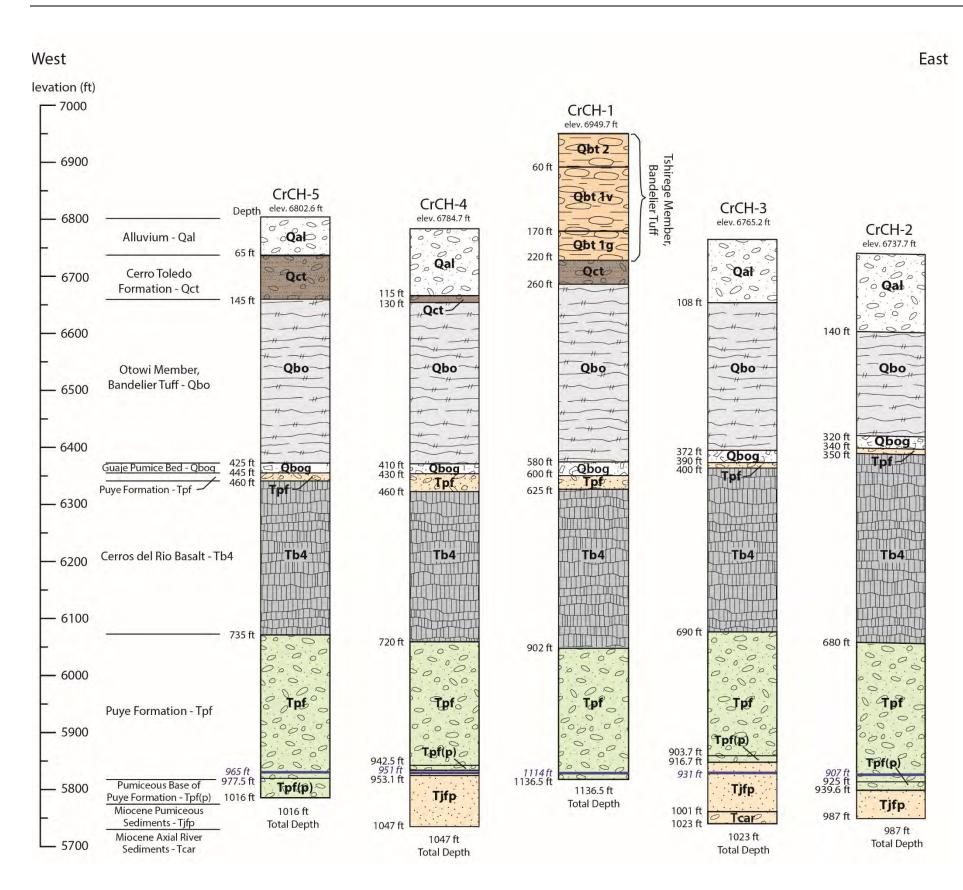
Figure 3.2-1 Stratigraphic columns showing geologic contacts and water levels (blue lines) for core holes in Mortandad Canyon
