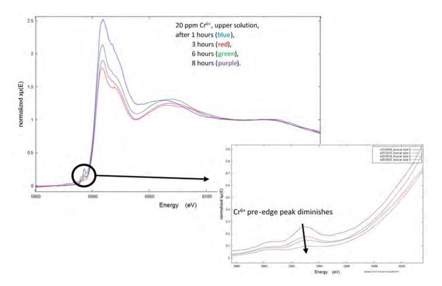
Figure 4.0-5 Time sequence of XANES spectra of a suspension of 0.25–0.7-μm fines in a solution that was initially 20 mg/L Cr(VI). The fines were isolated by gravity setting from a sonic core hole sample taken from core hole CrCH-1, and they represented 0.9 wt% of the sediment sample.
