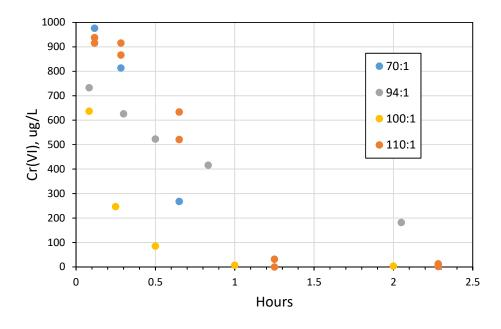
Figure 2.3-2 Results of batch uptake experiments conducted on zero-valent iron filings at various solution-to-solid mass ratios (see legend). All experiments were conducted using R-42 water with a starting concentration of 900–1000 μg/L Cr(VI), and the y-axis is the concentration of Cr(VI) remaining in solution. Chromium uptakes ranged from 50 to 100 μg Cr/g, but they did not represent the full capacity of the zero-valent iron for Cr(VI).
