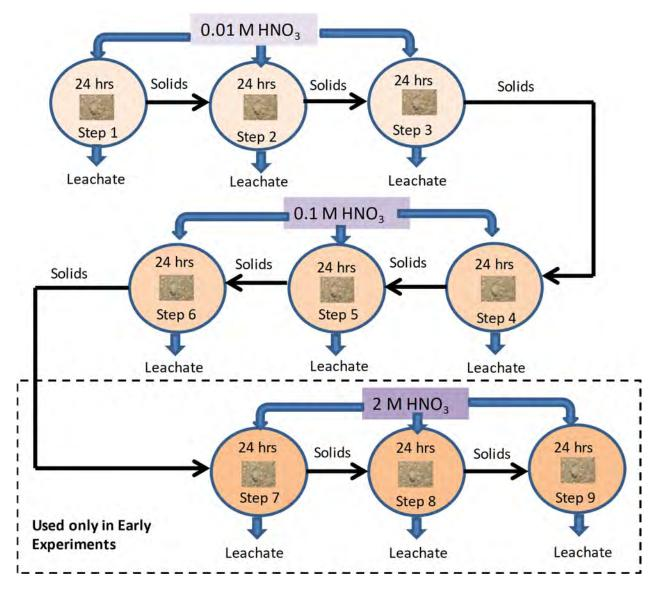
Figure 3.1-2 Workflow of sequential acid leaching procedure. Leachate to solid mass ratio was 10:1 in most tests. Note that the 2 M HNO<sub>3</sub> steps were used only in early experiments.
