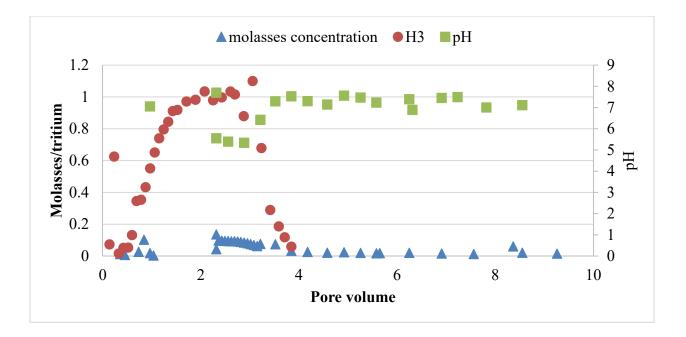
Figure 4.0-3Breakthrough curves showing pH, molasses, and tritium transport through column<br/>2 during the injection of molasses for 3.2 pore volumes
