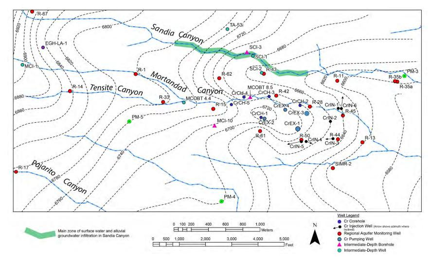
Figure B-1 Structure contour map for base of Tshirege Member subunit Qbt 1g. Contours based on the sitewide geologic model. Wells installed after 2015 shown for reference.
