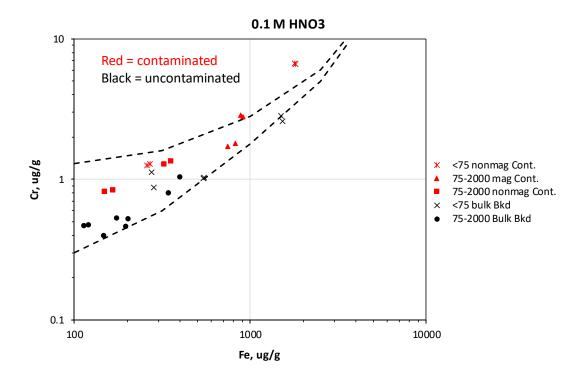
Figure 3.3-3 Cumulative log Cr vs log Fe of leachates from samples in first set of leaching experiments after 0.1 M HNO<sub>3</sub> leaching steps. Vertical difference between dashed lines corresponds to 1  $\mu$ g Cr(VI)/g, which is approximately the method detection limit for biotite.
