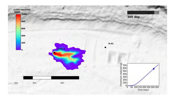
Figure 2.3-2 Map showing simulation of the injection of a strong chemical reducing agent (sodium dithionite) at CrPZ-3. The figure shows the concentration of Cr(VI) removed as a result of remediation 11 mo after the injection. Although a large amount of Cr(VI) has been removed by this time, relatively slow pore water velocities (0.1 m/d; ~0.33 ft/d) prevent the migration of the treated plume to R-42.
