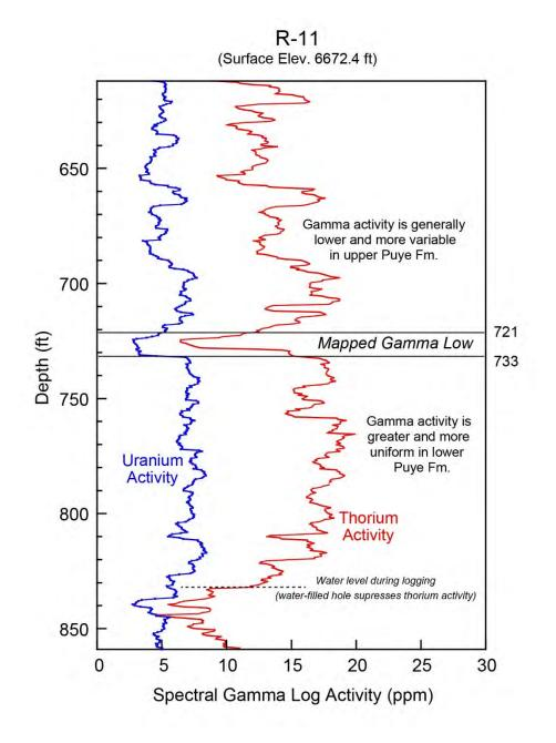
Figure 2.3-3 Borehole spectral gamma activity for uranium and thorium in the Puye Formation for well R-11. Log data collected by Schlumberger, Inc. in an open borehole.
