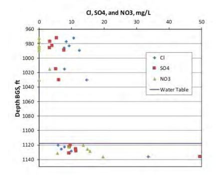
Figure A-3.0-2 Anion concentrations in pore water vs depth in CrCH-1
