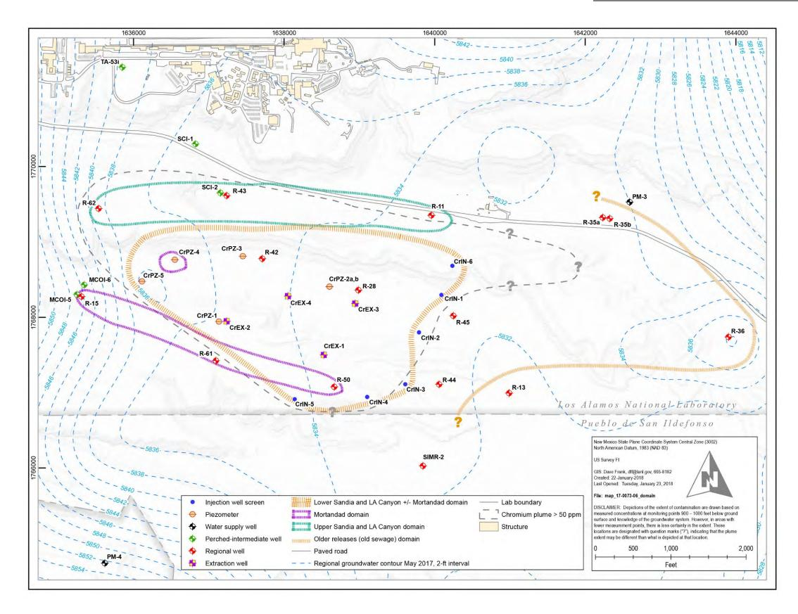
Figure 3.0-1 Contaminant domains as identified from fingerprint diagrams
