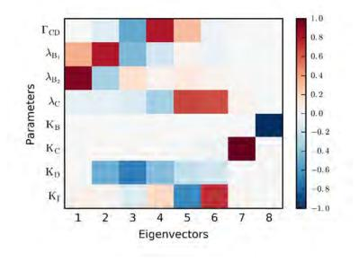
Figure 2.3-7 Local sensitivity analysis of biochemical treatment model. See Table 2.3-1 for a description of the parameters. The figure presents the eigenvectors of the estimated parameter covariance matrix, which defines the parameter uncertainty and sensitivity.
