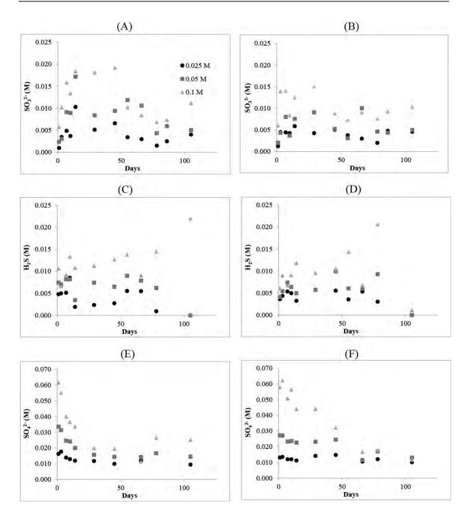
Figure 4.1-2 Concentrations of SO<sub>3</sub><sup>2-</sup> (A, B), H<sub>2</sub>S (C, D), and SO<sub>4</sub><sup>2-</sup> (E, F) through time in HCO<sub>3</sub><sup>--</sup> buffered (A, C, E) and EDTA/OH<sup>-</sup>-buffered (B, D, F) solutions
