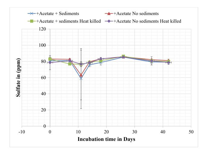
Figure 3.1-7 Sulfate reduction in R-42 water amended with 0.82 g/L acetate and incubated anaerobically in the presence and absence of sediments. Reactors received 100 mL of R-42 water and 1.0 g of sediments. R-42 water chemistry is presented in the materials and methods section.
