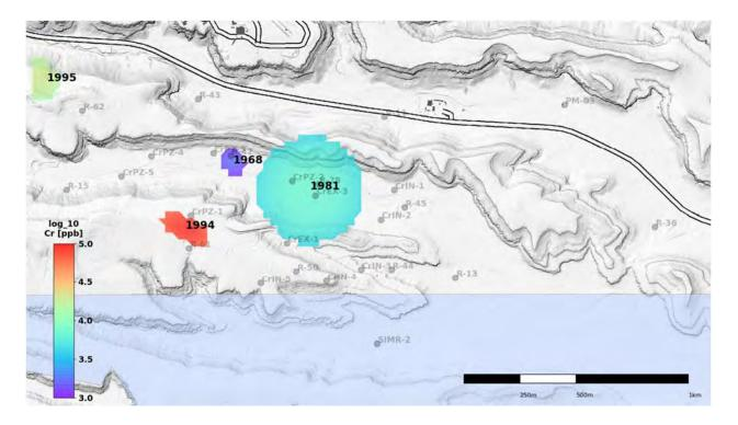
Figure 2.2-4 Maps of model-predicted contaminant sources; the number, size, shape, location, start time, and concentrations of the contaminant sources are estimated automatically during the model calibration. The figure shows the estimated four contaminant sources, the start times (in calendar years), their size, and concentrations (as log transformed values).
