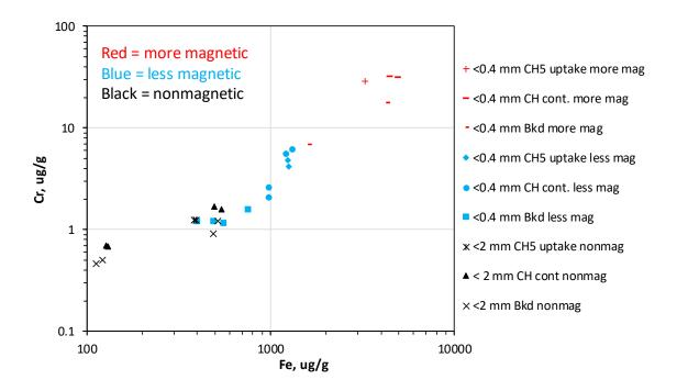
Figure 3.3-5 Cumulative log Cr vs log Fe of leachates from samples in third set of leaching experiments (0.1 M HNO<sub>3</sub> leaching), color coded by degree of magnetism of samples
