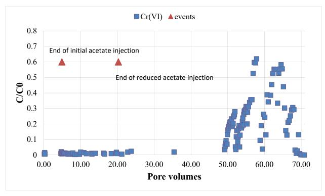
Figure 3.2-3 Chromium attenuation in column 1 biostimulated by the injection of 4.8 pore volumes of a solution containing 0.82 g/L (10 mM) acetate followed by 15.4 pore volumes of a solution containing 0.08 g/L (0.1mM) ace
