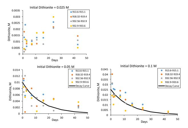
Figure 4.3-1 Dithionite decomposition in batch experiments with four different sediments (identified by depth [ft] from CrCH-2) with 10 mL of solution for every 5 g sediment. Curves were generated using the kinetic model discussed in text.
