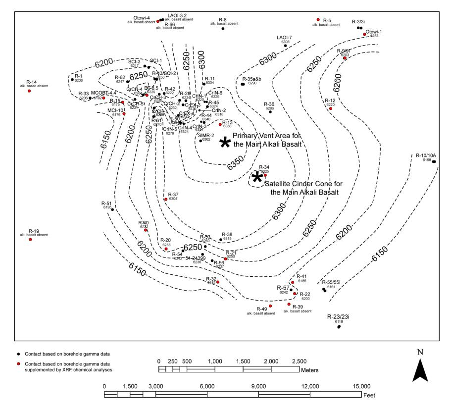
Figure B-7 Structure contour map for top of alkali basalt of the main tholeiite/alkali basalt sequence of the Cerros del Rio basalt
