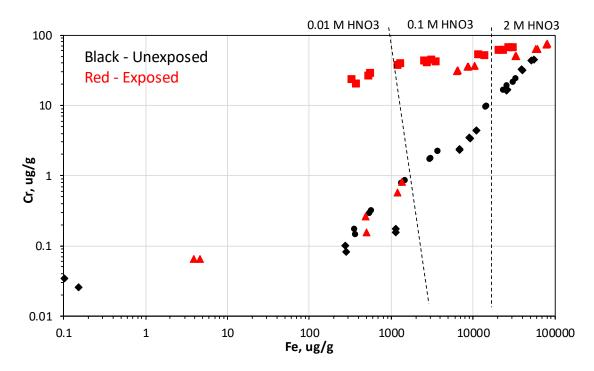
Figure 3.2-4 Cumulative log Cr vs log Fe of leachates from Cr(VI)-exposed and unexposed biotite samples. Leachates are from experiments of Figure 3.2-1.
