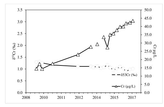
Figure 4.0-2d R-45(1) quarterly  $\delta^{53}$ Cr sampling analysis with corresponding [Cr] from 2008 to 2016. Total chromium data were included in the study data set only if a  $\delta^{53}$ Cr sample was acquired during the same time period.
