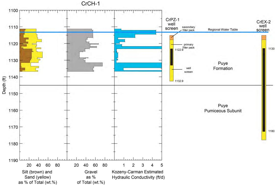
Figure 3.3-1 CrCH-1 grain-size variations for beds making up strata in the upper part of the regional aquifer. The CrPZ-1 (completed in the CrCH-1 borehole) and R-28 well screens are shown for reference. The contact between the Puye Formation and the Puye pumiceous subunit is based on well CrEX-2, which is located on the same drill pad. CrEX-2 did not fully penetrate the Puye pumiceous unit at a total depth of 1240 ft.
