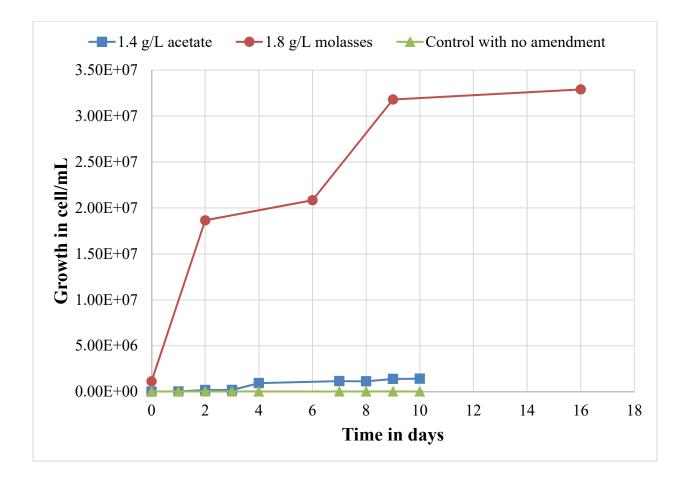
Figure 3.1-2 Microbial growth in R-42 water stimulated by either 1.4 g/L sodium acetate or 1.8 g/L molasses. Cell numbers were determined by reading the optical density at 600 nm which were converted to cell numbers using calibration curves establishes specifically for each carbon source. The water parameters of the R-42 water are as described in the materials section.
