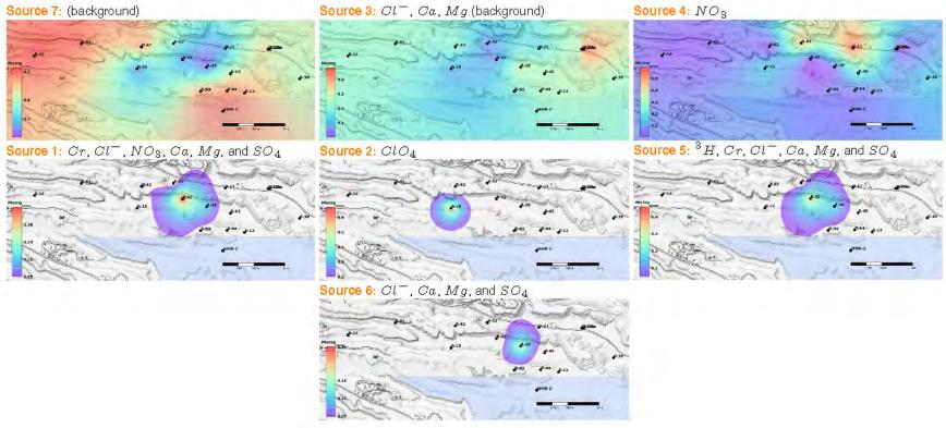
Figure 3.2-2 (continued) Spatial maps of transient mixing ratios of the seven groundwater types (sources) identified to be present at the site monitoring wells. The maps show the mixing ratio of each source (groundwater type). The mixing ratios are estimated at the wells and interpolated in space between the wells using an interpolation technique. The maps represent 12 temporal snapshots from 2005 to 2016.
