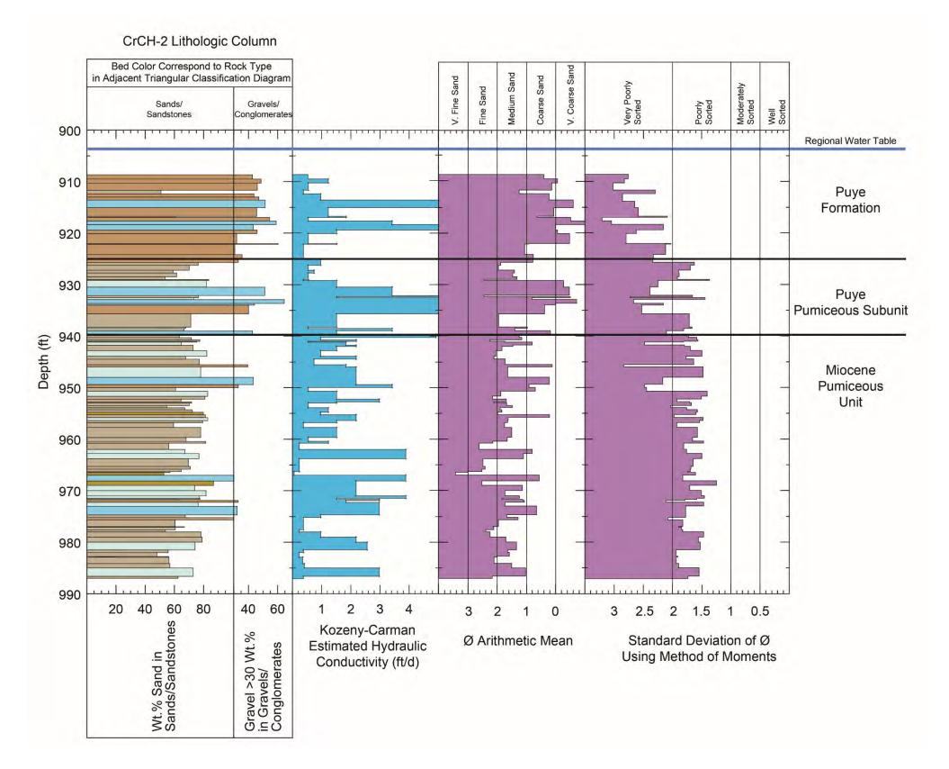
Comparison of the CrCH-2 lithologic column and estimated hydraulic conductivity to the mean grain size (shown as Ø arithmetic mean) and sorting characteristics (shown as standard deviation of Ø using the Figure 3.3-6 method of moments). The Ø arithmetic mean and standard deviation of Ø were calculated from the CrCH-2 sieve data following the methodology of Folk (1980).
