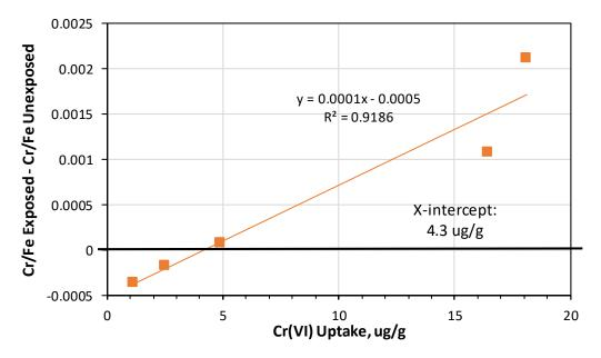
Figure 3.2-7 Cumulative Cr/Fe ratios of 0.1 M HNO<sub>3</sub> leachates from Cr(VI)-exposed bentonite samples minus Cr/Fe ratio of leachates from unexposed bentonite samples vs Cr(VI) uptake on exposed samples. Each data point is the average of two duplicate measurements. X-intercept of linear regression line is estimate of method detection limit for Cr(VI) uptake on bentonite.
