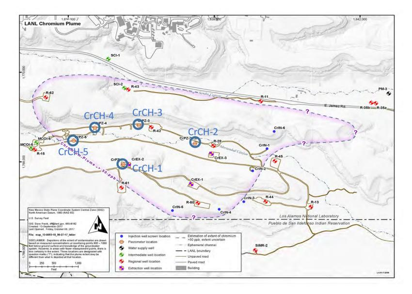
Figure A-1.0-1 Locations of the sonic core holes within the Cr(VI) plume, as demarcated by the inferred 50-µg/L contour
