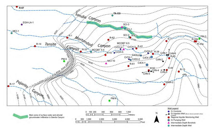
Figure B-8 Structure contour map for base of Cerros del Rio basalt. Contours based on the sitewide geologic model. Wells installed after 2015 shown for reference.
