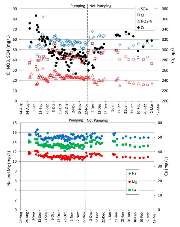
Figure 4.0-3 Concentrations of key constituents in R-28 during the long-term pumping test of R-28 (at 27–28 gpm), including the period after pumping ended (top: major anions and Cr(VI), bottom: major cations). Note the difference in the Cr concentration scale in the upper plot. Only Cr shows any significant changes (within the error of the measurements) over the time of the test. Charge balance errors were much smaller for the R-28 test than for the R-42 test.
