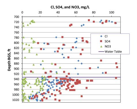
Figure A-3.0-12 Anion concentrations in pore water vs depth in CrCH-3
