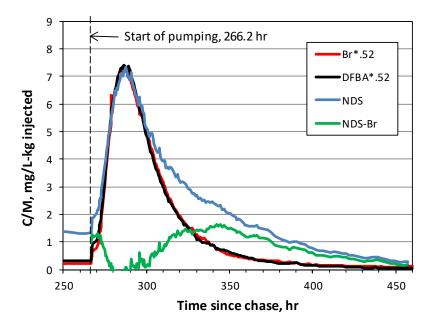
Figure 3.2-1 Response of 1,5-NDS dilution tracer at R-42 during the push-pull test after subtracting out the contribution of the residual tracer that was still in the wellbore at the start of the test (approximately 52% of the tracer, which was assumed to be represented by the Br and 2,6-DFBA responses multiplied by 0.52). The green curve is the resulting response of the dilution tracer that was assumed to have left the wellbore during the dilution tracer test.
