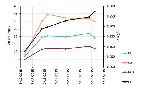
Figure A-3.0-25 Concentrations of anions and Cr as a function of time during pumping of CrCH-5 with a Bennett pump capable of about 0.5 gal. per minute
