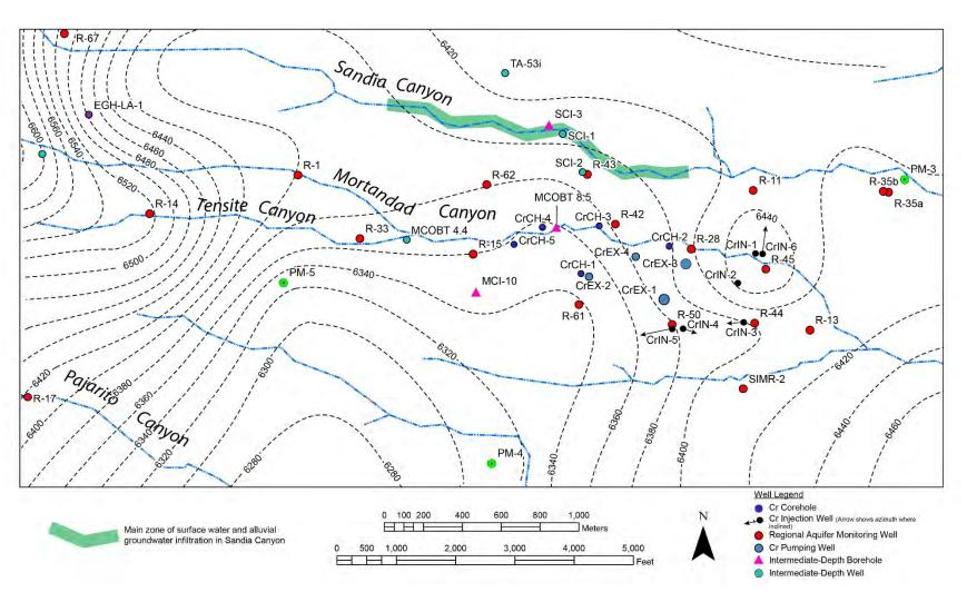
Figure B-4 Structure contour map for base of Guaje Pumice Bed. Contours based on the sitewide geologic model. Wells installed after 2015 shown for reference.
