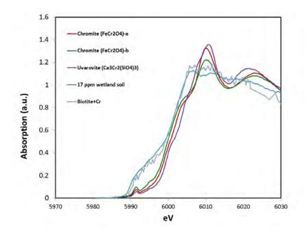
Figure 4.0-2 XANES spectra of chromite-a, chromite-b, uvarovite, Sandia Canyon wetland sample with chromium concentration of 17  $\mu$ g/g, and Cr(VI)-spiked biotite with chromium concentration of 18  $\mu$ g/g
