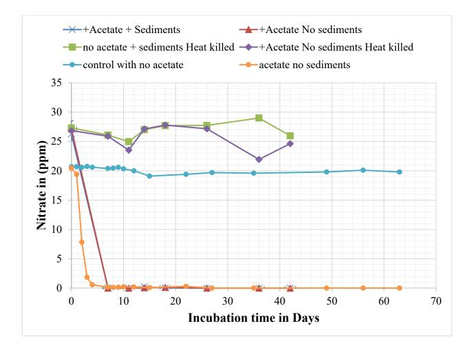
Figure 3.1-6 Nitrate reduction in R-42 water amended with 0.82 g/L acetate and incubated anaerobically in the presence and absence of sediments. Reactors received 100 mL of R-42 water and 1.0 g of sediments. R-42 water chemistry is presented in the materials and methods section.
