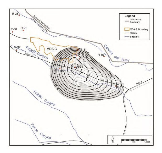
Figure 2.5-2 Structure contour map for top of dacite lavas near the east end of MDA G in Pajarito Canyon. Map taken from the WC15c sitewide geologic model.
