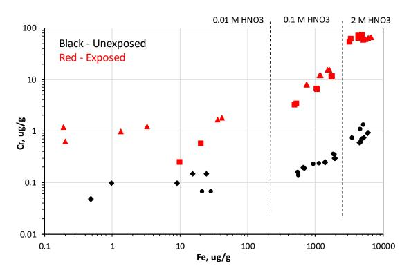
Figure 3.2-5 Cumulative log Cr vs log Fe of leachates from Cr(VI)-exposed and unexposed bentonite samples. Leachates are from experiments of Figure 3.2-2.
