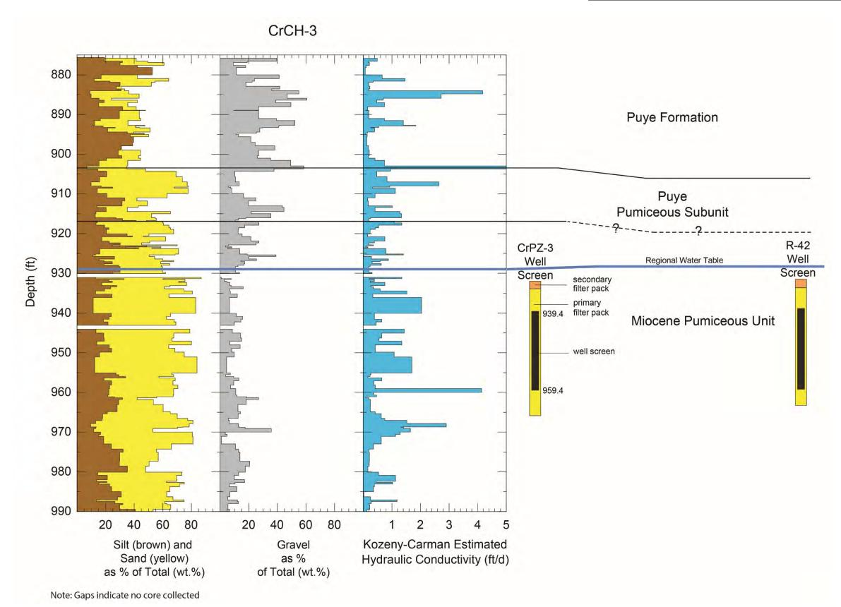
Figure 3.3-9 CrCH-3 grain-size variations for beds making up strata in the upper part of the regional aquifer. CrPZ-3 (completed in the CrCH-3 borehole) and R-42 well screens are shown for reference.
