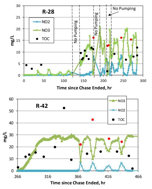
Figure 3.3-3 Total organic carbon (TOC) concentrations superimposed on  $NO_3^-$  and  $NO_2^-$  concentrations during R-28 (top) and R-42 (bottom) push-pull tests. Note the higher TOC concentration (red dots) tend to occur when  $NO_3^-$  concentrations drop and  $NO_2^-$  concentrations rise (i.e., when  $NO_3^-$  reduction seems to be occurring).
