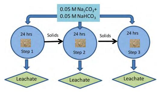
Figure 3.1-1 Workflow of sequential alkaline leaching procedure. Leachate to solid mass ratio was 10:1 in most tests.
