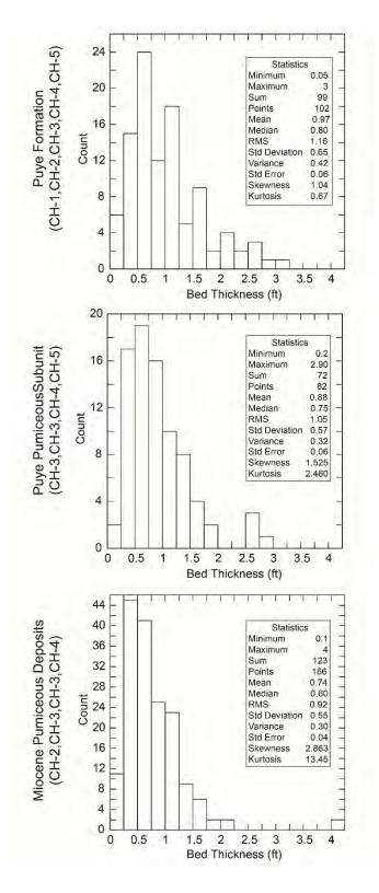
Figure 3.4-4 Histograms for bedding thickness of Pliocene and Miocene rocks in the upper regional aquifer beneath Mortandad Canyon
