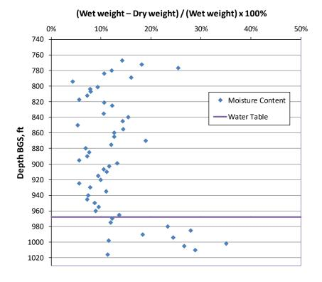
Figure A-3.0-21 Moisture content vs depth in CrCH-5
