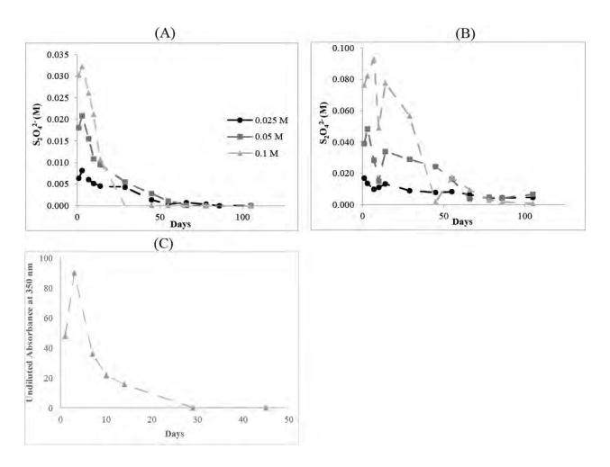
Figure 4.1.1 Dithionite decomposition through time in HCO<sub>3</sub><sup>-</sup>-buffered (A), EDTA/OH<sup>-</sup>-buffered (B), and unbuffered (C) solutions.
