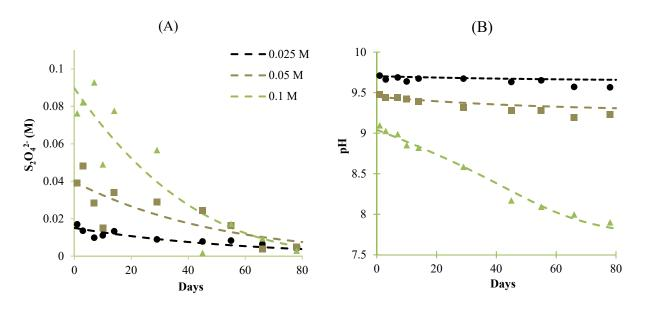
Figure 4.1-6 Simulation of experiments conducted in the EDTA/OH<sup>-</sup>-buffered solution. Panel (A) shows the dithionite concentration, and Panel (B) shows pH. The figure compares calibrated model curves (dashed lines) and experimental data (points) for the different concentrations of dithionite used in these experiments.
