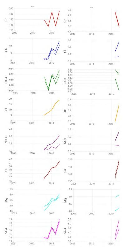
Figure 3.0-1 (continued) Observed versus estimated geochemical concentrations at all the site monitoring wells over time. Observed data are presented in Table 3.0-1. The estimated concentrations are based on NTFk ML analysis with seven distinct groundwater types (Table 3.0-2).
