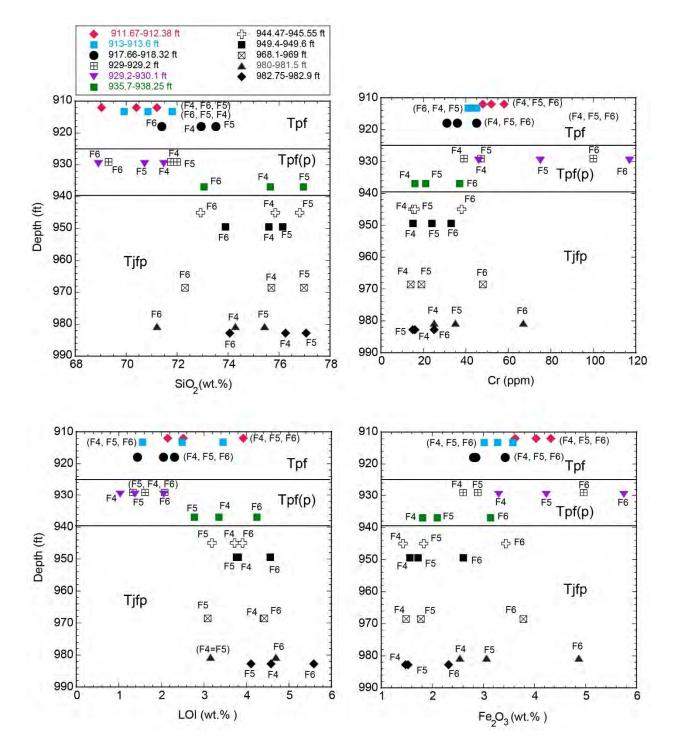
Figure E-2 Plots of major oxides versus depth of fine- to medium sand (F4), very fine to fine sand (F5), and silt (F6) fractions of core hole CrCH-2 core samples from the Puye Formation (Tpf), Puye pumiceous subunit [Tpf(p)], and Miocene pumiceous unit (Tjfp)
