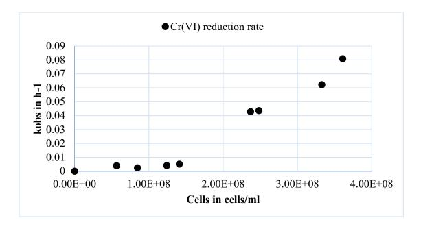
Figure 4.0-1 Observed rate of Cr(VI) reduction by cell suspensions of microbes grown anaerobically by biostimulation of R-42 water with acetate. The observed rates were determined by fitting the Cr(VI) concentration decay by a mono exponential equation. Cell numbers were determined by direct cell counts.
