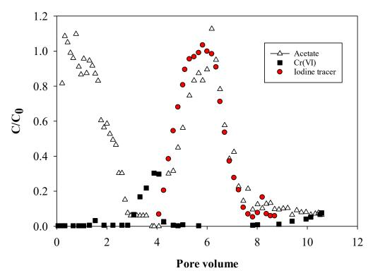
Figure 4.0-2 Breakthrough of Cr(VI), acetate, and iodine tracer from a column in response to two successive injections of an acetate pulse
