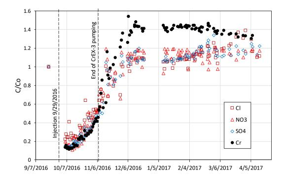
Figure 6.2-7 Concentrations of major anions and Cr(VI) in R-28 measured in passive samples collected from R-28 after the injection and chase, which were both potable water. Concentrations are expressed as fractions of pretest concentrations.
