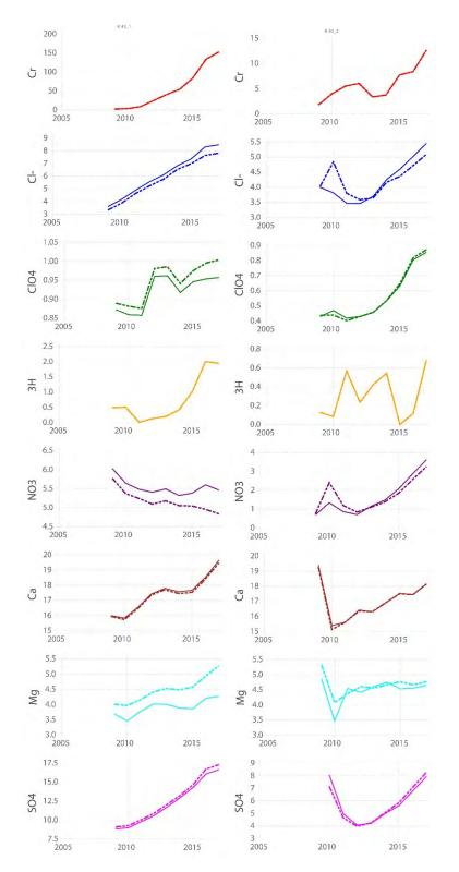
Figure 3.0-1 (continued) Observed versus estimated geochemical concentrations at all the site monitoring wells over time. Observed data are presented in Table 3.0-1. The estimated concentrations are based on NTFk ML analysis with seven distinct groundwater types (Table 3.0-2).
