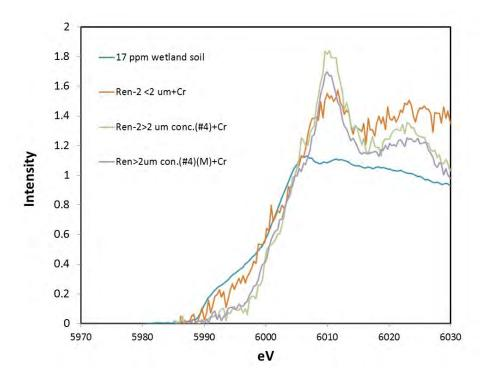
Figure 4.0-3 XANES spectra of Sandia wetland sample and various outcrop (Puye formation) samples after exposure to Cr(VI) solutions
