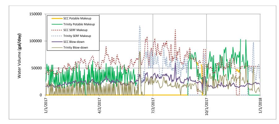
Figure 1.4-4 Daily cooling water usage and discharge information for the SCC and Trinity cooling towers during 2017. Included are effluent (blowdown) volumes from the SCC and Trinity cooling towers and makeup water sources (potable or SERF-blended water) used at the SCC and Trinity cooling towers. During 2017, all SCC and Trinity cooling tower blowdown was released to Outfall 001.
