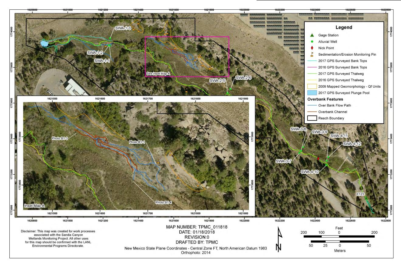
Figure B-4.3-2 Map of reach S-2 highlighting overbank flow features in the northcentral portion of the reach
