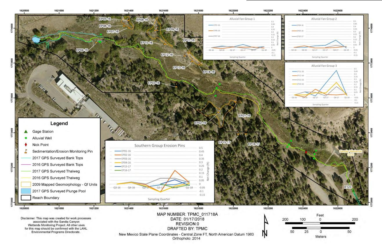
Figure B-4.4-2 Map of reach S-2 highlighting net change documented at erosion pins in their respective groups
