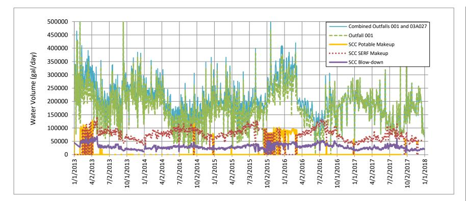
Figure 1.4-2 Daily water volumes (gpd) from November 2012 to December 2017 for effluent released from combined Outfalls 001 and 03A027 and Outfall 001 only. Also included are effluent (blowdown) volumes from the SCC cooling towers and makeup water sources (potable or SERF-blended water) used at the SCC cooling towers. The SCC cooling tower blowdown was released to Outfall 03A027 until September 8, 2016; since September 9, 2016, the blowdown has been released to Outfall 001.
