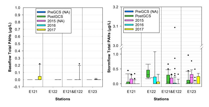
Figure D-2.0-7 (continued) Box-and-whisker plots of peak discharge TSS/SSC, total PCBs, unfiltered chromium and Cr(VI), and total PAHs for base flow and storm flow at gaging stations E121, E122, and E123, pre- and post-construction of the GCS, respectively, in 2015, 2016, and 2017. (NA = Not analyzed.)
