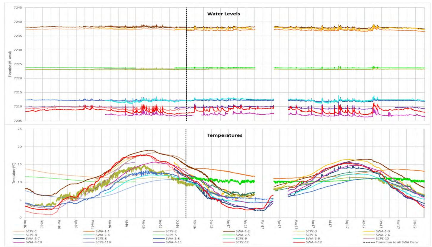
Notes: The sonde in SWA-4-11 had software malfunction errors during mid-September 2017 and was replaced in November 2017.
