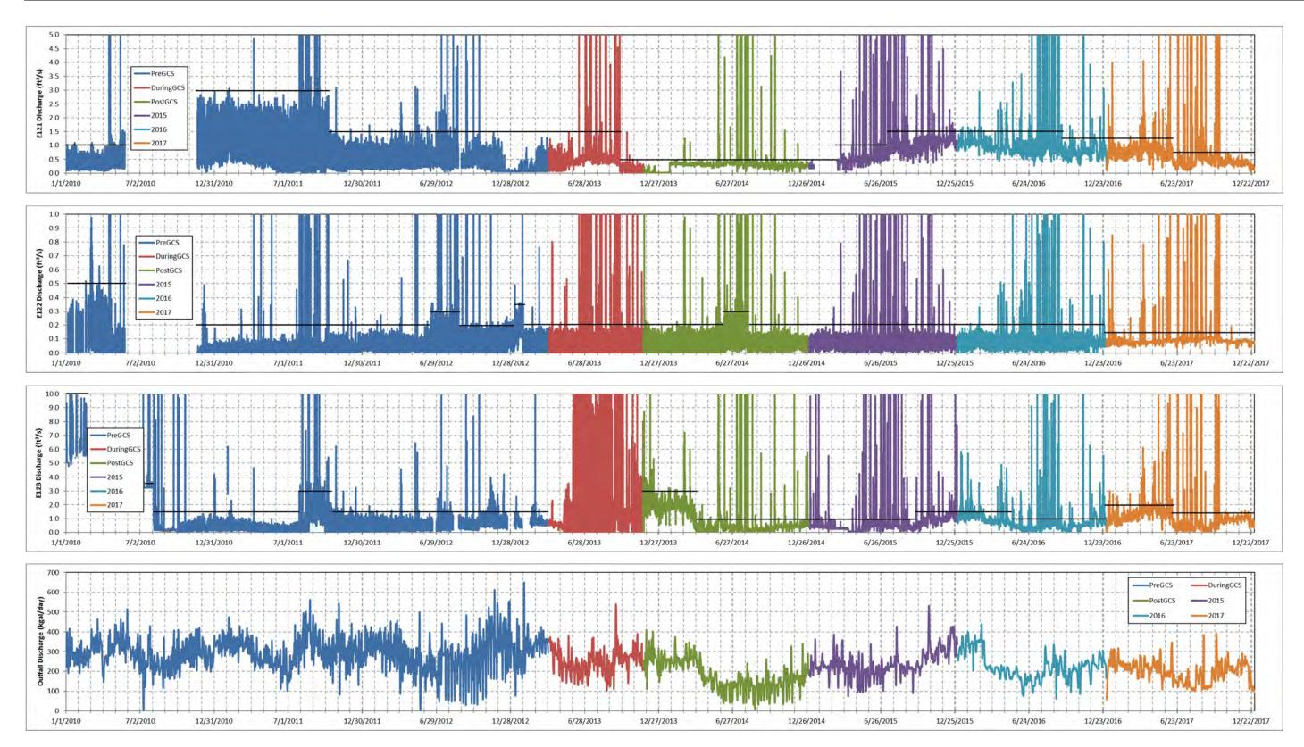
Figure D-2.0-6 Time-series plots from 2010 to 2017 showing discharge at E121, E122, and E123 and total discharge from Outfalls 001, 03A027, and 03A199; solid black horizontal lines indicate approximate base flow discharge at the surface-water gaging stations, which vary throughout the 8-yr period
