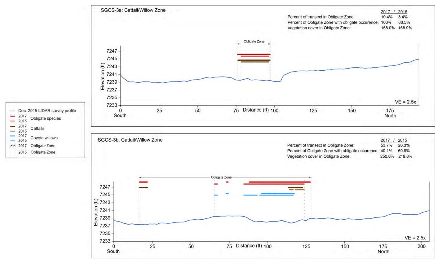
Note: Topographic profiles extracted from 2015 LiDAR survey based DEM.
