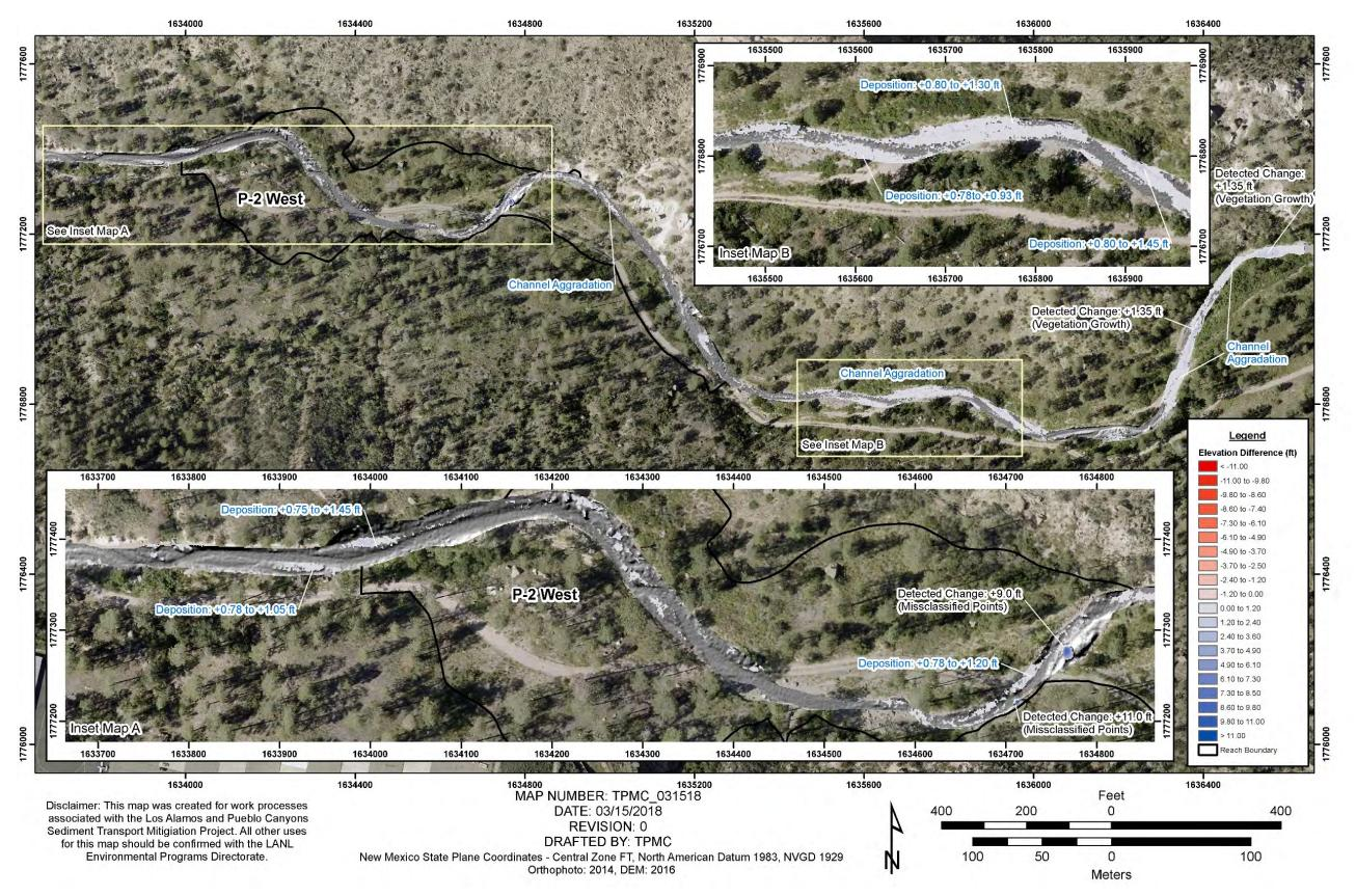
2014 orthophoto with 2016 hillshade DEM and 2014 to 2016 GCD results at the Pueblo Canyon Background Monitoring Area. FIS calibration was based on observable changes between DEMs. Figure A3-3.1-1
