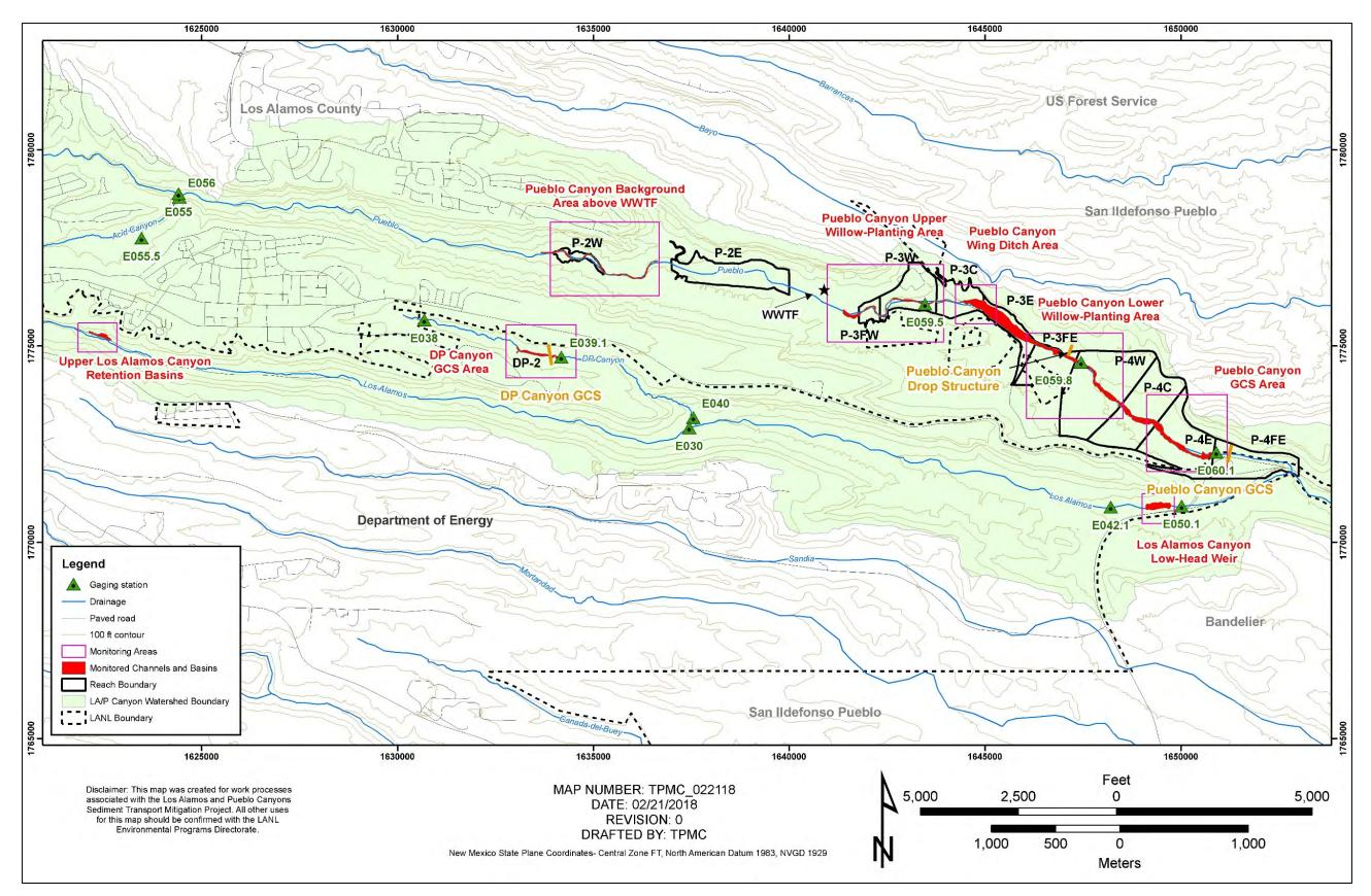
Figure A3-1.0-1 Los Alamos, Pueblo, and DP Canyon channel systems showing sediment transport monitoring areas, monitoring area extents, and stream gages
