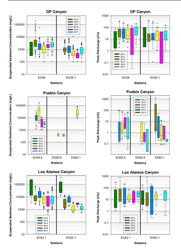
Figure 3.4-1 Box-and-whisker plots of SSC (left) and peak discharge (right) upstream and downstream of the watershed mitigations in DP (top), Pueblo (middle), and Los Alamos (bottom) Canyons over the past 6 yr of monitoring
