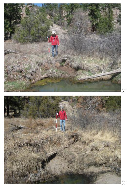
Photo A1-8 Detected change above the DP Canyon GCS in 2016 due to bank collapse (erosion of ~1 ft) (top) compared with the same view in 2017 (bottom), showing no observable change in 2017
