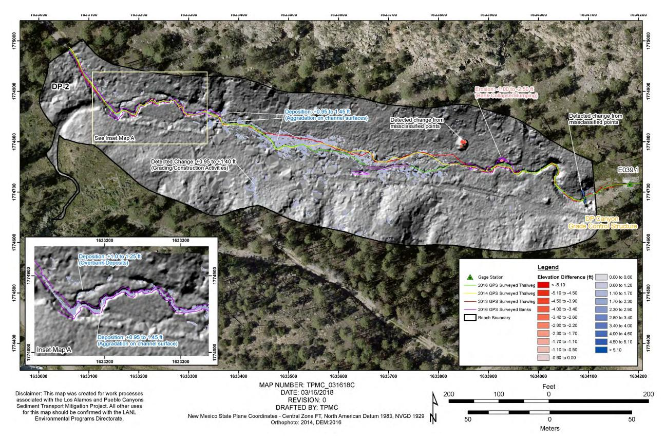
Figure A3-3.1-6 2014 orthophoto with 2016 hillshade DEM and 2014 to 2016 GCD results at the DP Canyon Monitoring Area. FIS calibration was based on observed differences between DEMs and field observations.
