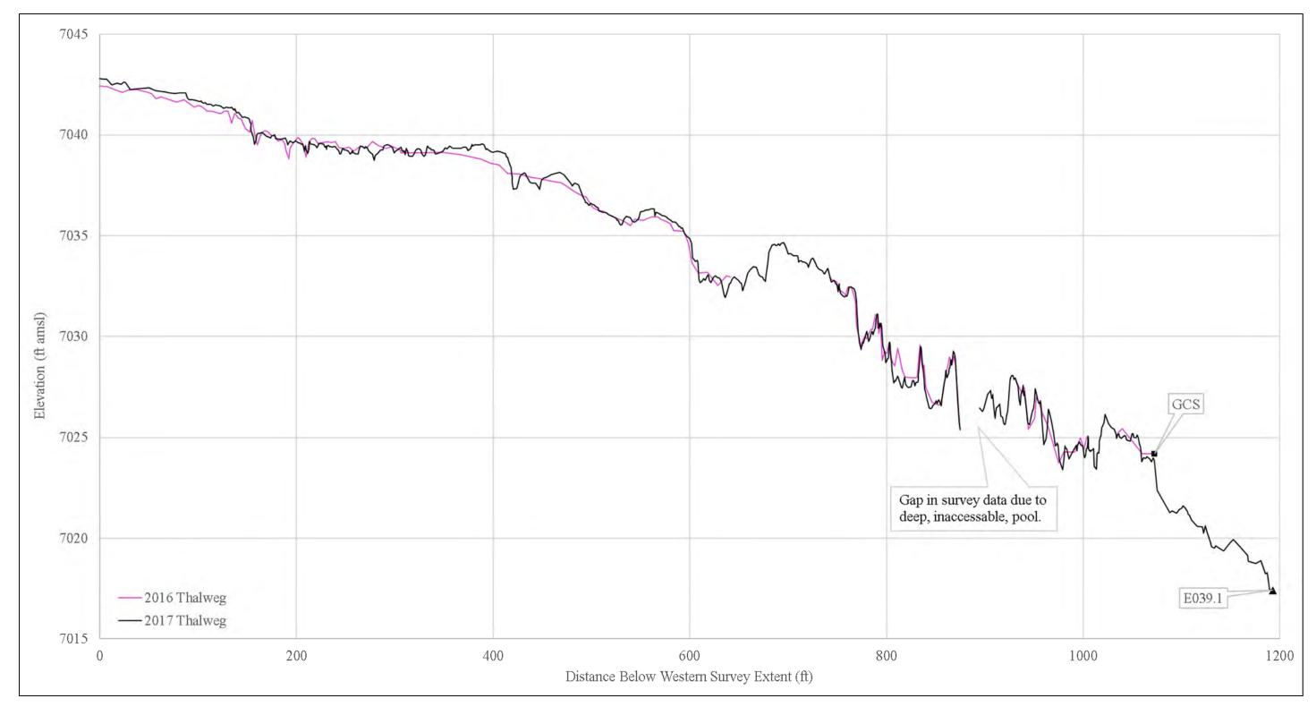
Figure A-4.8-2 Thalweg profile in DP Canyon GCS area (~25 times vertical exaggeration)
