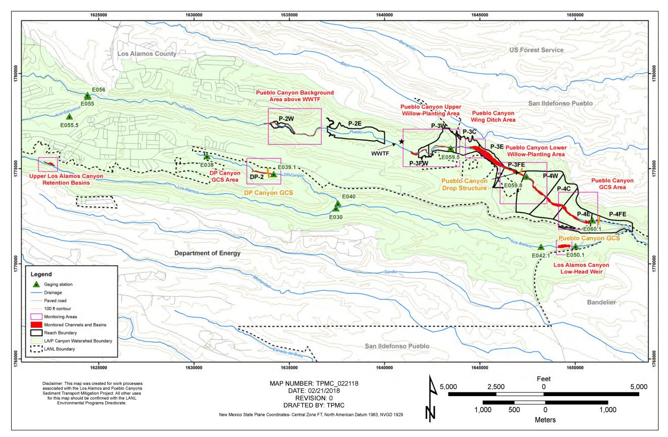
Figure A-1.0-1 Los Alamos, Pueblo, and DP Canyon channel systems showing sediment transport monitoring areas, monitoring area extents, and stream gages
