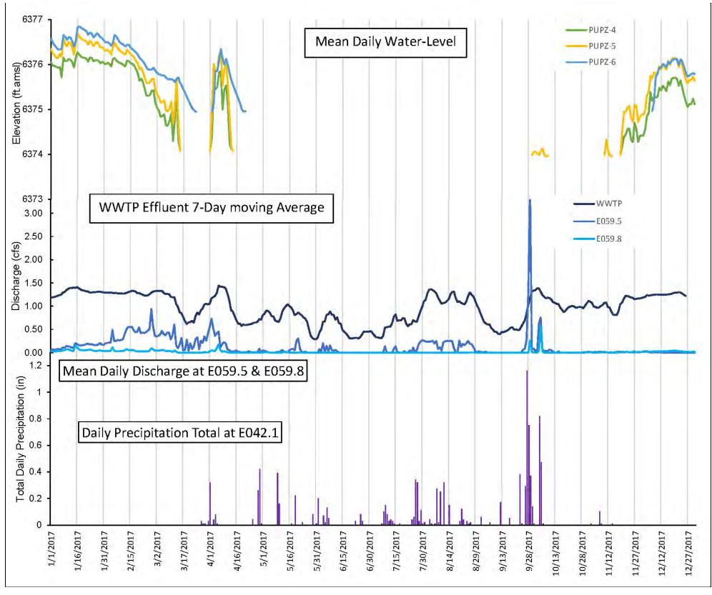
Figure B-2.0-2 Mean daily water level (ft amsl) in piezometers PUPZ-4, PUPZ-5, and PUPZ-6; 7-d moving average of Los Alamos WWTP effluent discharge; mean daily discharge at gaging stations E059.5 and E059.8; and total daily precipitation at E042.1
