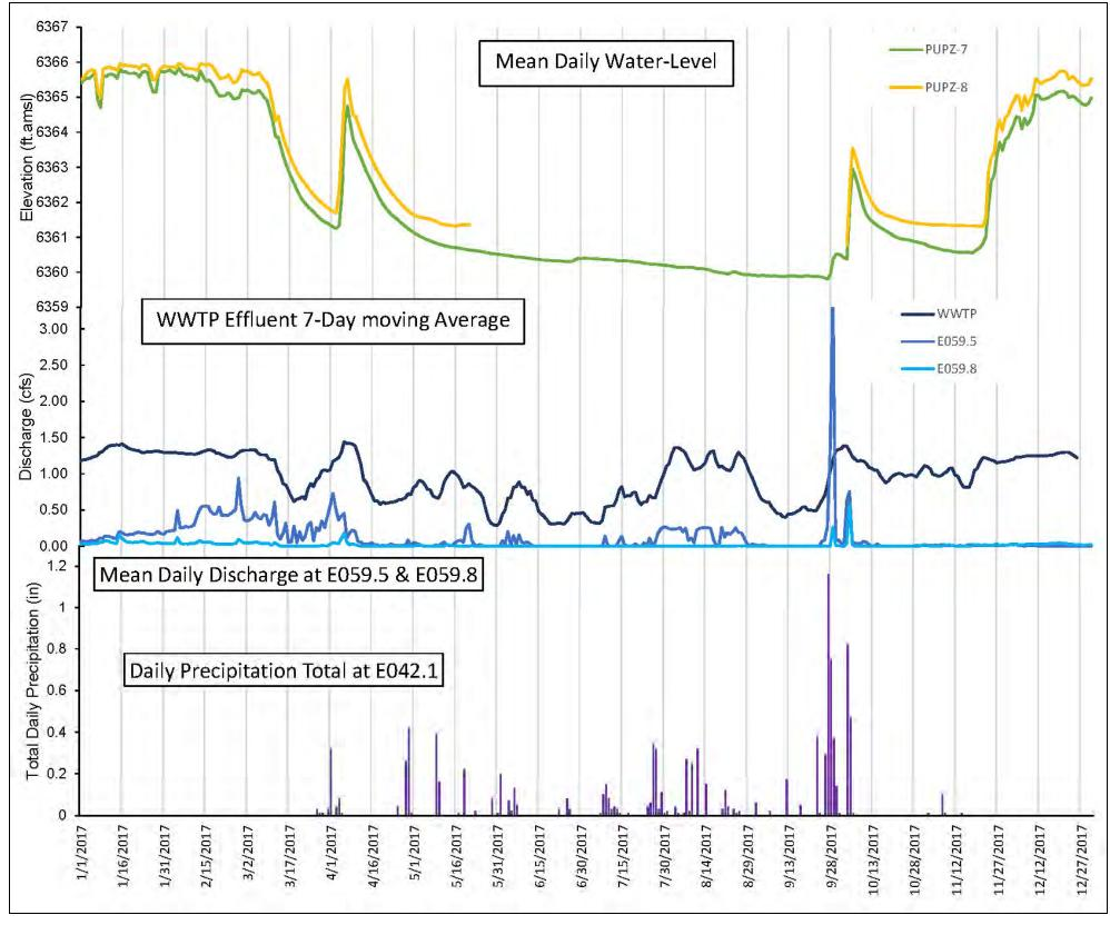
Mean daily water level (ft amsl) in piezometers PUPZ-7 and PUPZ-8; 7-d moving average of Los Alamos WWTP effluent discharge; mean Figure B-2.0-3 daily discharge at gaging stations E059.5 and E059.8; and total daily precipitation at E042.1
