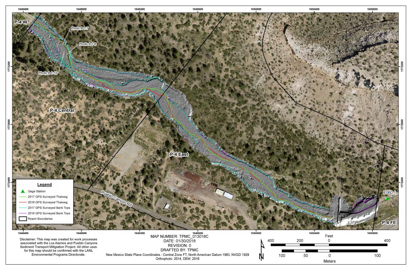
Figure A-4.5-1 2014 orthophoto with 2016 hillshade DEM and 2016 versus 2017 surveyed channel banks and thalweg at the Pueblo Canyon GCS area
