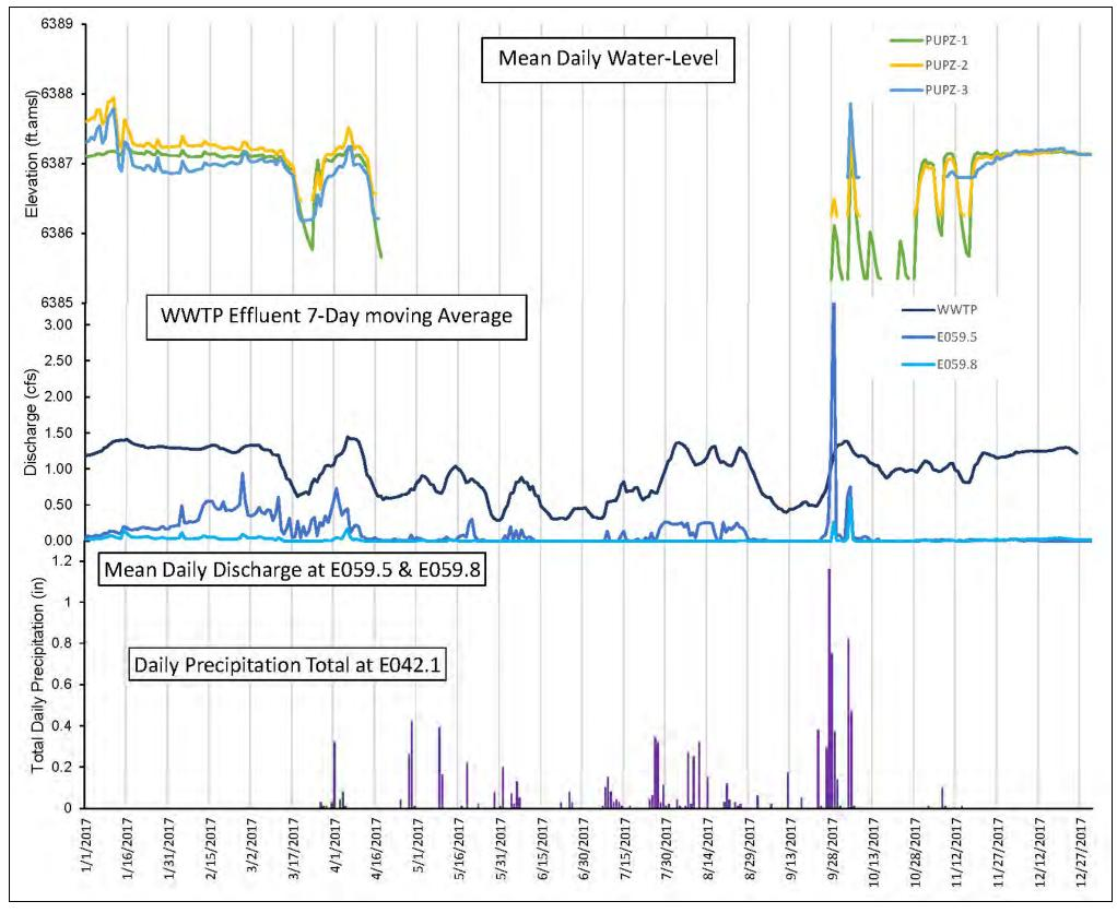
Mean daily water level (ft above mean sea level [amsl]) in piezometers PUPZ-1, PUPZ-2, and PUPZ-3; 7-d moving average of Los Alamos wastewater Figure B-2.0-1 treatment plant (WWTP) effluent discharge; mean daily discharge at gaging stations E059.5 and E059.8; and total daily precipitation at E042.1
