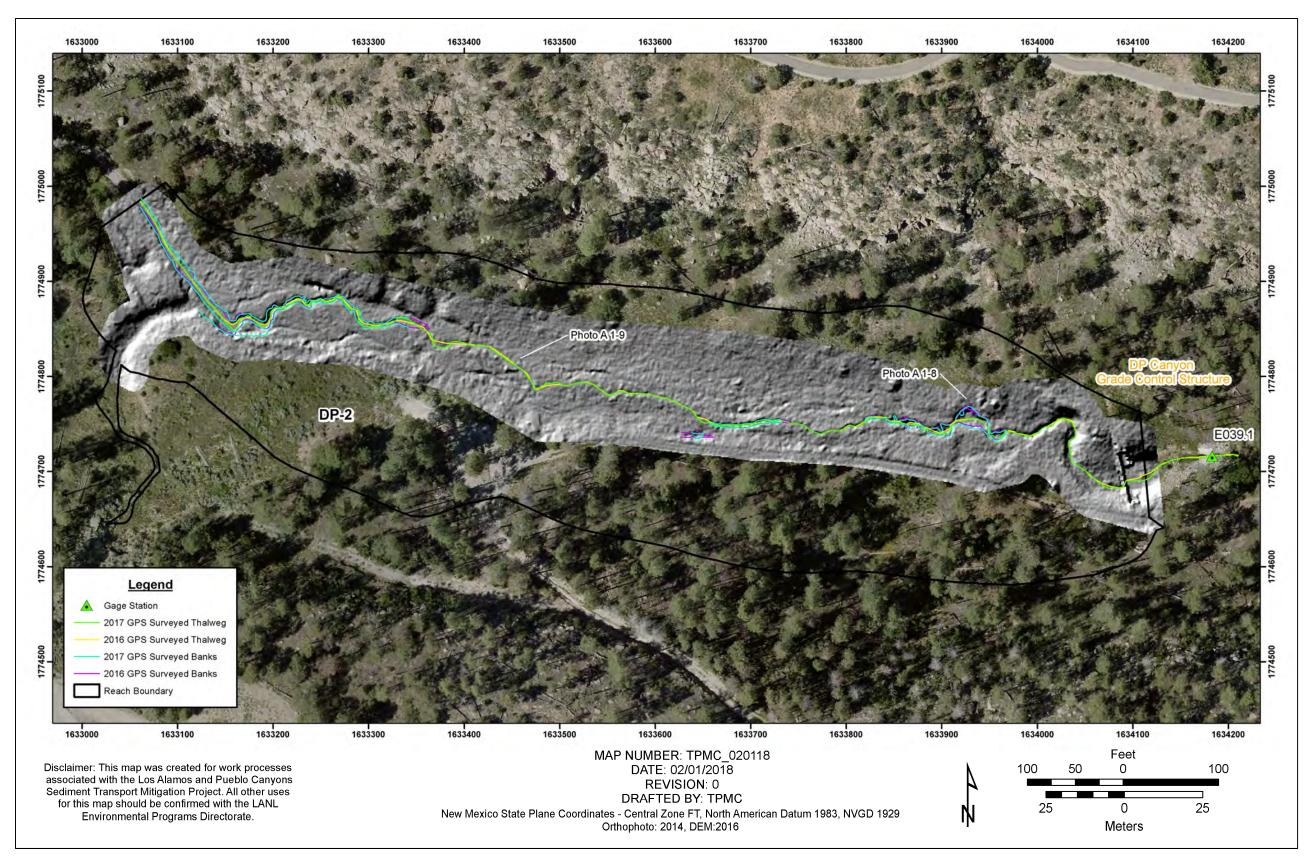
Figure A-4.8-1 2014 orthophoto with 2016 hillshade DEM and 2016 versus 2017 surveyed channel banks and thalweg at the DP Canyon GCS area
