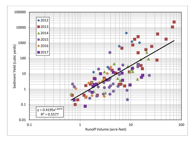
Figure 3.2-5 Relationship between SSC-based sediment yield and runoff volume over the past 6 yr of monitoring
