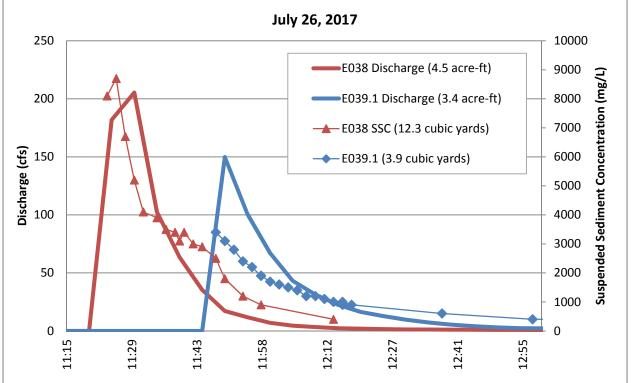
Figure 3.4-2 Discharge and SSC at E038 and E039.1 in upper Los Alamos Canyon on days when sampling of the same runoff event occurred
