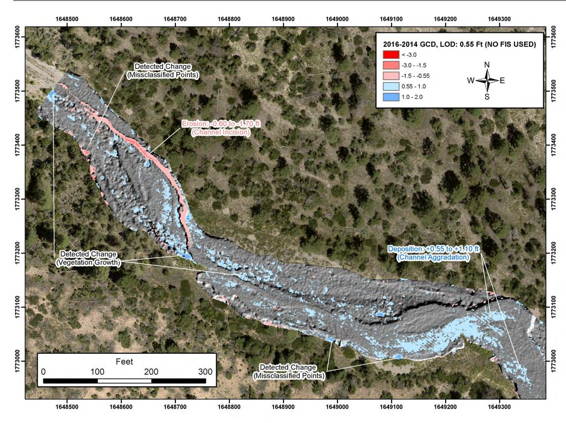
GCD analysis with a Min. LoD of 0.55 ft. 2014 orthophoto with 2016 hillshade DEM and 2014 to 2016 GCD results at the Pueblo Canyon grade-control structure area. Many non-geomorphic Figure A3-2.4-1 detections from vegetation growth, issues with modeling steep banks, and poor point classification are evident using the Min. LoD method for thresholding changes.
