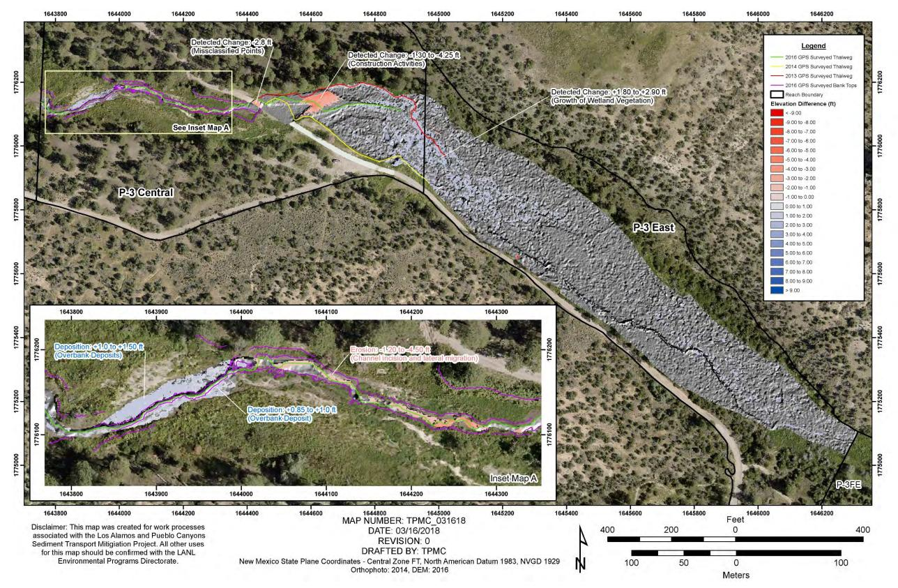
2014 orthophoto with 2016 hillshade DEM and 2014 to 2016 GCD results at the Pueblo Canyon Wing Ditch Monitoring Area. FIS calibration was based on calculated difference between GPS and Figure A3-3.1-3 DEM elevation values.
