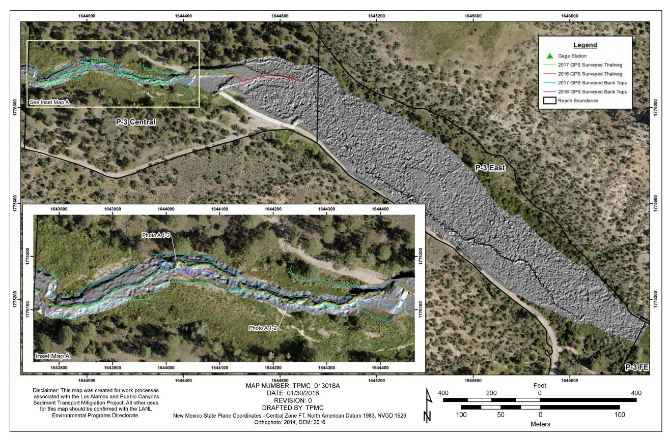
Figure A-4.3-1 2014 orthophoto with 2016 hillshade DEM and 2016 versus 2017 surveyed channel banks and thalweg at the Pueblo Canyon wing ditch area
