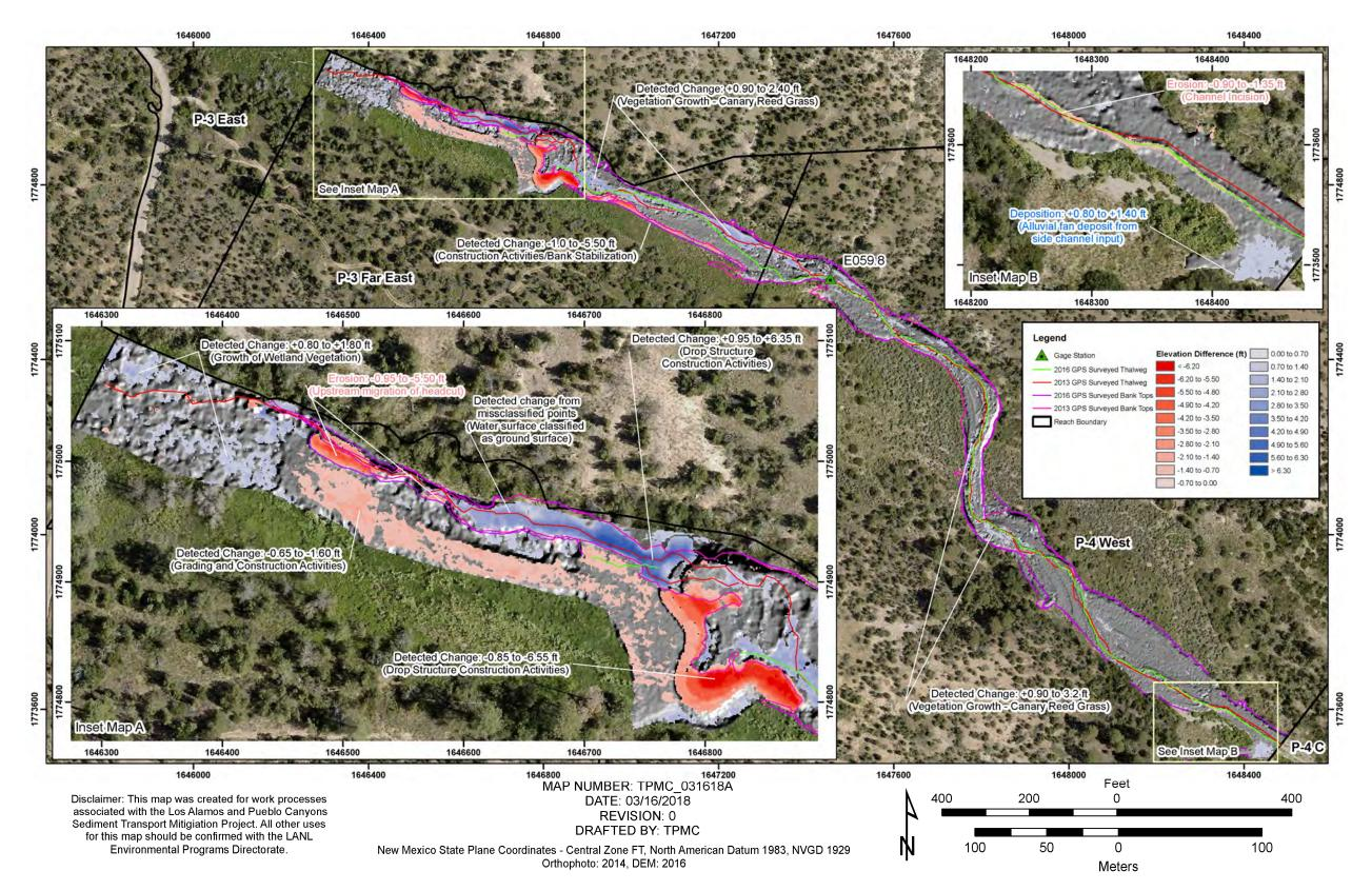
2014 orthophoto with 2016 hillshade DEM and 2014 to 2016 GCD results at the Lower Pueblo Canyon Willow Planting Monitoring Area. FIS calibration was based on observed differences between Figure A3-3.1-4 DEMs and field observations.
