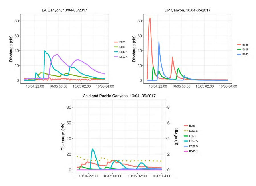
Figure 3.2-3 (continued) Hydrographs during each sample-triggering runoff event for each canyon from up- to downstream reaches
