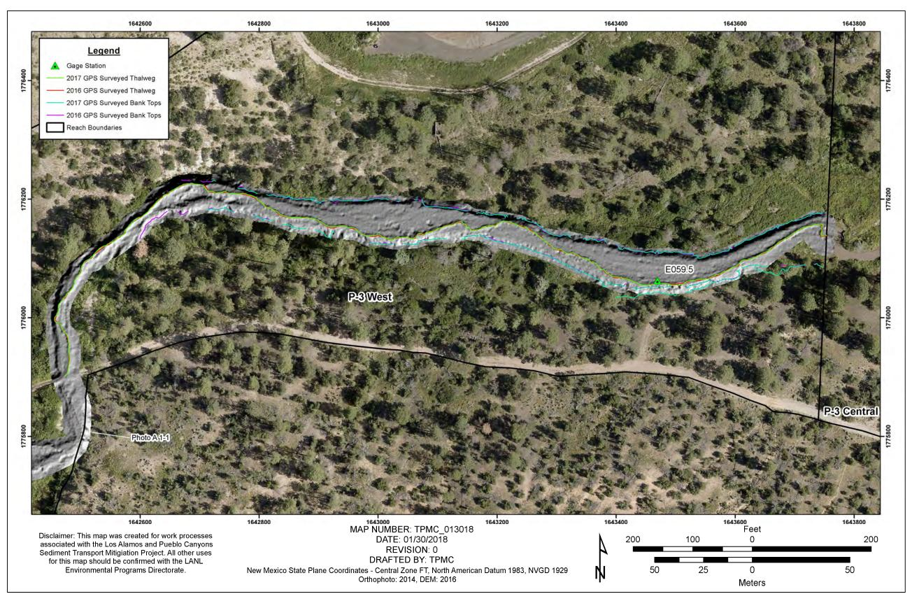
Figure A-4.2-1 2014 orthophoto with 2016 hillshade DEM and 2016 versus 2017 surveyed channel banks and thalweg at the Pueblo Canyon upper willow planting area
