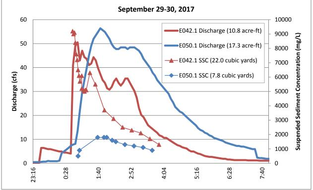
Figure 3.4-3 Discharge and SSC at E042.1 and E050.1 in upper Los Alamos Canyon on days when sampling of the same runoff event occurred
