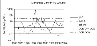
**Figure 5-17**. Average annual radioactivity in Mortandad Canyon surface water and alluvial groundwater.
