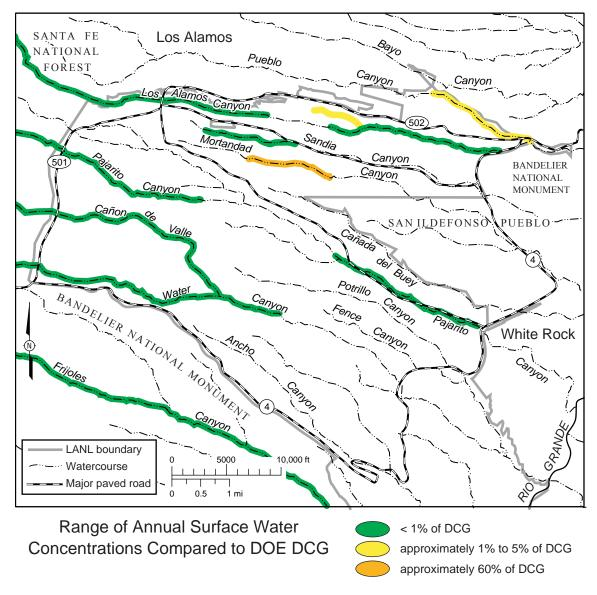
**Figure 6-7.** Annual average radioactivity in persistent surface waters compared with the DOE Derived Concentrations Guides (DGCs). Persistent waters include perennial and intermittent stream segments (Fisher 2003). The figure shows an integrated perspective of how the activities of a mixture of 9 key LANL radionuclides compare to the DCGs (see text for details).
