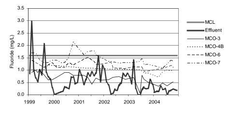
Fluoride in Mortandad Canyon Alluvial Groundwater 1999-2004
