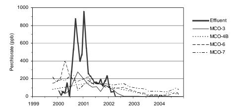
**Figure 5-16.** Fluoride, nitrate, and perchlorate in RLWTF effluent and Mortandad Canyon alluvial groundwater from 1999 through 2004.
