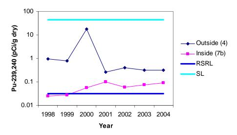
**Figure 7-5.** Plutonium-239,240 in surface soils collected from two selected (worst case) locations at Area G at TA-54 from 1998 to 2004 as compared to the regional statistical reference level (RSRL) and screening level (SL).
