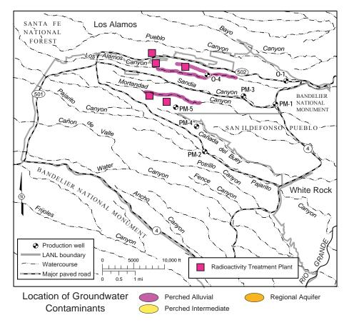
**Figure ES-4.** Location of groundwater contamination by strontium-90 above the 8 pCi/L EPA drinking water maximum contaminant limit. The extent of alluvial groundwater contamination lateral to the canyon is not to scale: contamination is confined to the alluvium within the canyon bottom and is narrow at the map scale.
