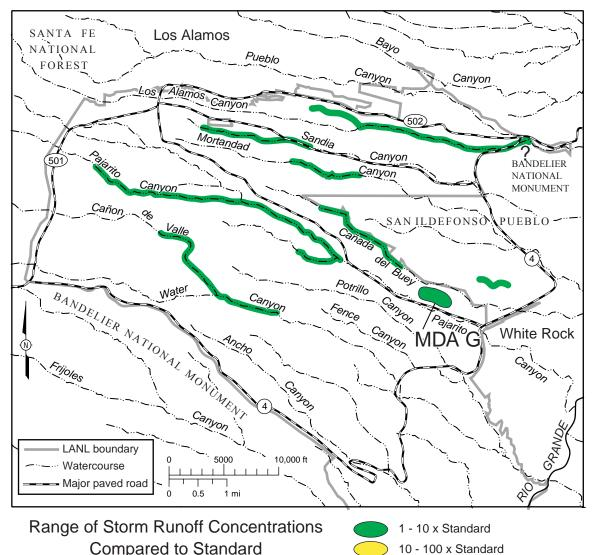
Figure 6-15. Location of storm runoff with dissolved copper above the New Mexico Acute Aquatic Life stream standard. Different colors indicate the proportion of concentration to the standard. The highest 200
