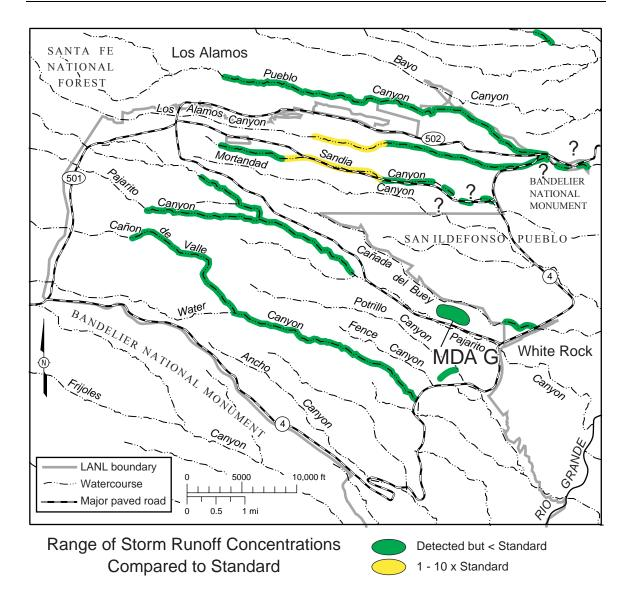
**Figure 6-14.** Location of storm runoff with total mercury above the New Mexico Wildlife Habitat stream standard. Different colors indicate the proportion of concentration to the standard. The highest 2004 watercourse values were in Los Alamos Canyon at 1.5 times the standard and in Sandia Canyon at 1.2 of the standard.
