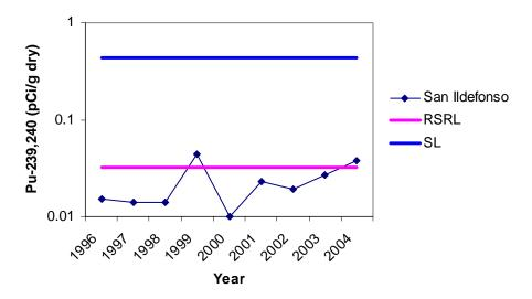
**Figure 7-2.** plutonium-239,240 concentrations in soil samples collected from San Ildefonso Pueblo lands over time approximately one-half mile northeast of Area G as compared to the regional statistical reference level (RSRL) and to the screening level (SL).
