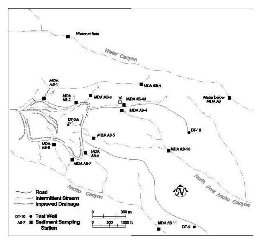
Figure 6-6. Sediment sampling stations at Area AB, TA-49.
