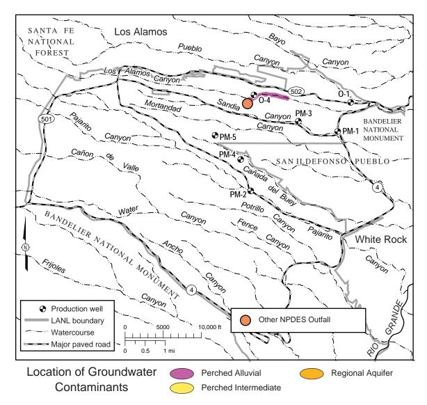
**Figure 5-13.** Location of groundwater contamination by molybdenum above the 1 mg/L New Mexico Groundwater Standard for Irrigation Use. The maximum 2004 value in Los Alamos Canyon alluvial groundwater was 105% of the groundwater standard. Different colors indicate the affected groundwater zones.
