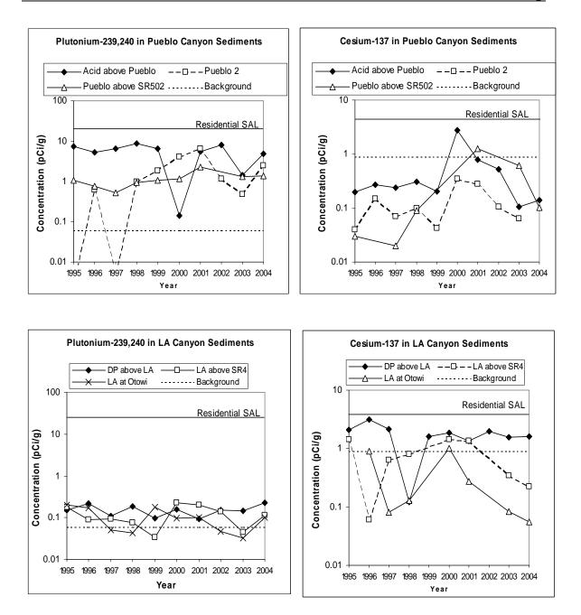
Figure 6-11. Long-term radioactivity trends in Los Alamos and Pueblo Canyon sediments. Note the logarithmic scale on the vertical axes of the graphs.
