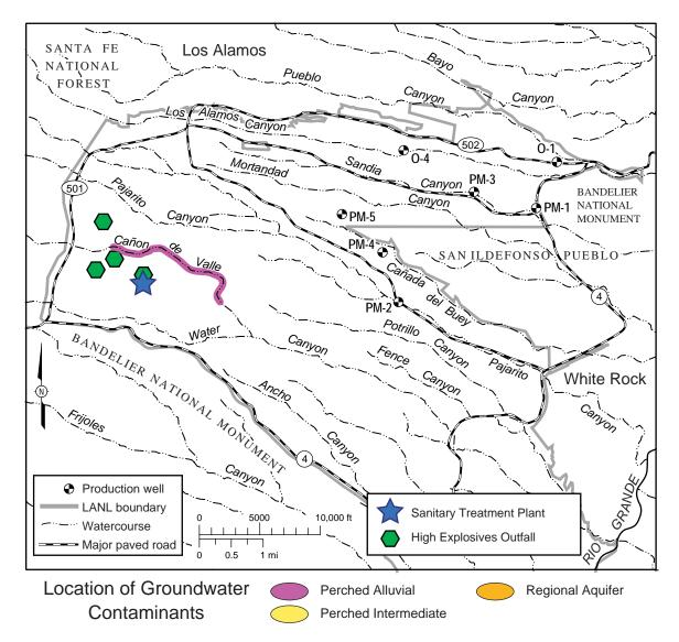
**Figure 5-18**. Location of groundwater contamination by RDX above the EPA Region VI screening level of 6.1 ppb and barium above the New Mexico groundwater standard of 1 mg/L in perched alluvial groundwater. This map is based on data obtained by the Environmental Restoration Project. Different colors indicate the affected groundwater zones.
