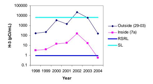
**Figure 7-4.** Tritium in surface soils collected from two selected (worst case) locations within and around Area G at TA-54 from 1998 to 2004 as compared to the regional statistical reference level (RSRL) and screening level (SL).
