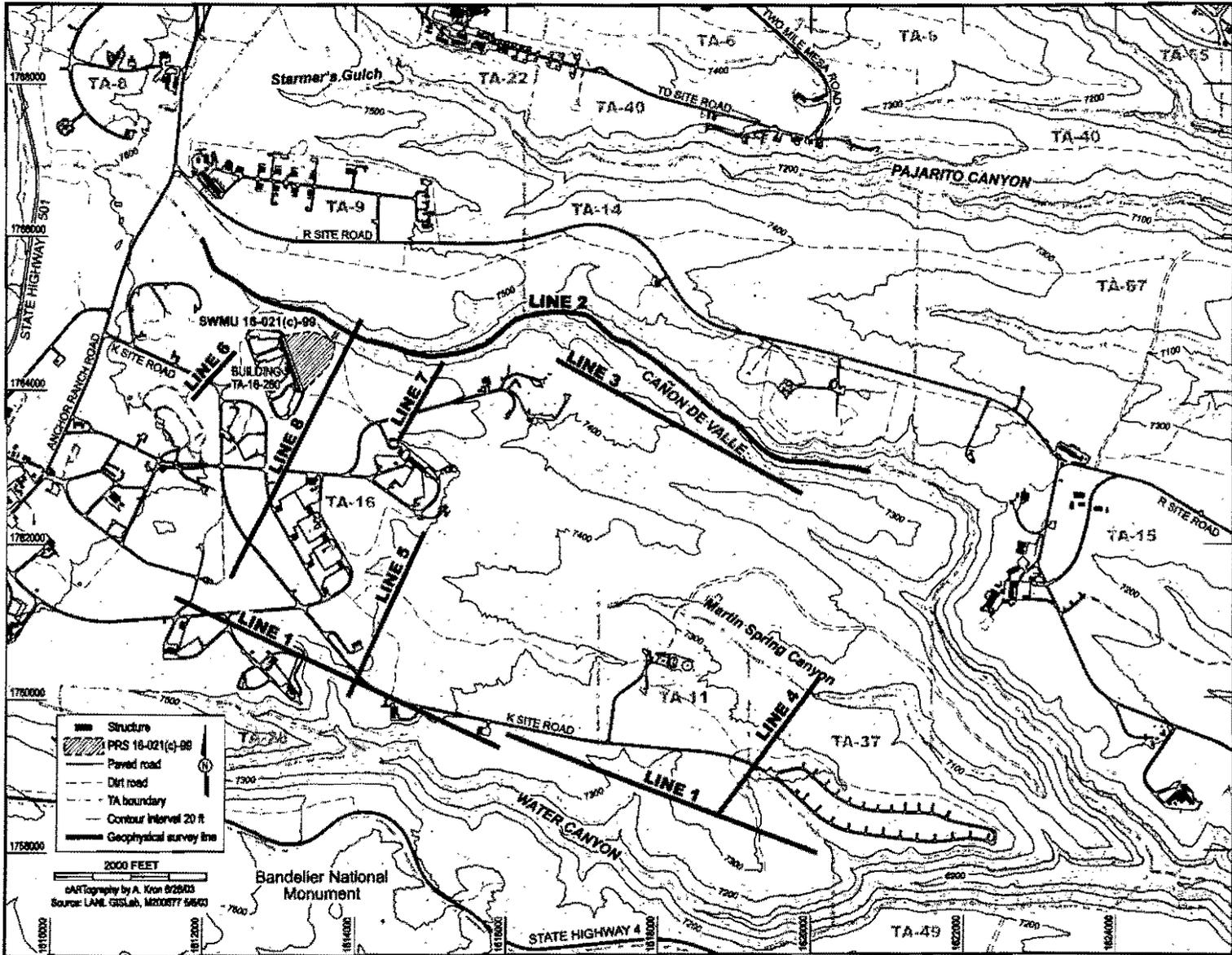
Figure 3.3-7. Locations of Geophysical Survey Lines for Controlled Source and Natural Source Audio-Frequency Magnetotelluric Survey (see Appendix D-3)
