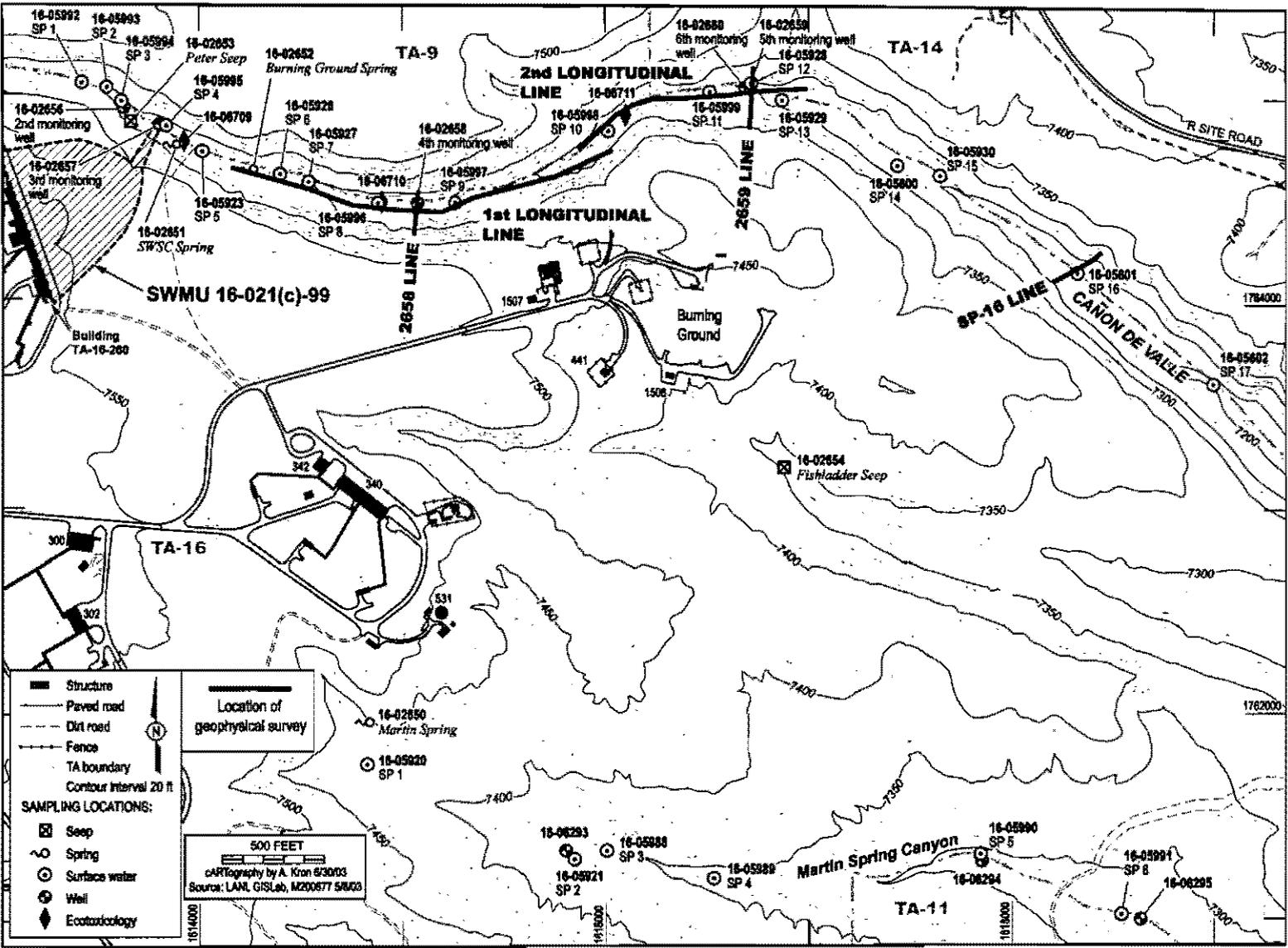
Figure 3.3-6. Locations for High Resolution Resistivity and Refraction Seismic Survey Lines (see Appendix D-2)
