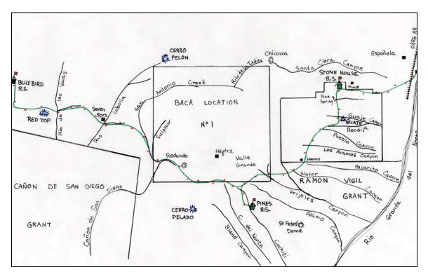
Fig. 1-4. Jemez Forest Reserve Telephone Line circa 1907. This graphic illustrates the location and extent of the early telephone line as described by Ben White. The line reached across the southern third of the Jemez Forest between Stone House and Blue Bird ranger stations, a distance of approximately seventy miles. The extent of that first section of line completed in December of 1906 was about the first half of that distance, reaching from Stone House to Pines Ranger Station.
