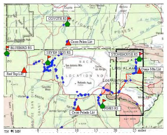
Fig. 5-10. Hemingray sites in Jemez Forest. Blue diamonds mark 219 glass sites in the Jemez Forest. Sites line up along telephone lines to ranger stations and lookouts as indicated on early maps. Heavy red line between Stone House and Pines Ranger Station traces the extent of the line in 1906. The black rectangle is the focus area identified as the Pajarito Plateau.
