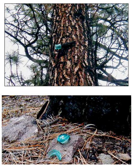
Fig. 4-3. Popped Top and Split Bottom. These two photos demonstrate the problems with the glass insulator and wood bracket. The insulator top has apparently popped off due to freezing and the end of the bracket has split and broken away as the girth of the tree expanded. This ponderosa is located on West Jemez Road. (Geographic positioning system [GPS] waypoint WJ1)
