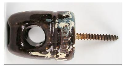
Fig. 4-21. Post-style Insulator. This insulator, designed to screw directly into the telephone pole, was the type used along a later section of telephone line that dropped into Los Alamos Canyon from the Army barracks on the canyon's north side.
