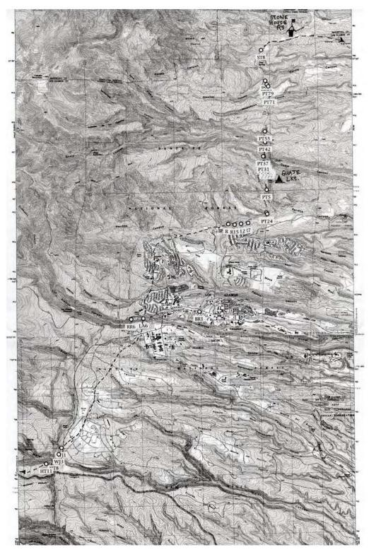
Fig. 5-11. Telephone Line Across the Pajarito Plateau. Twenty-six Hemingray sites help tie down the location of the early line across the Pajarito Plateau. The dotted line fills in the corridor and is a projection based on the 1913 and 1914 Forest Service maps. I identify this section of telephone line corridor as the old Pajarito Line, because much of it followed the Pajarito Trail across the plateau.
