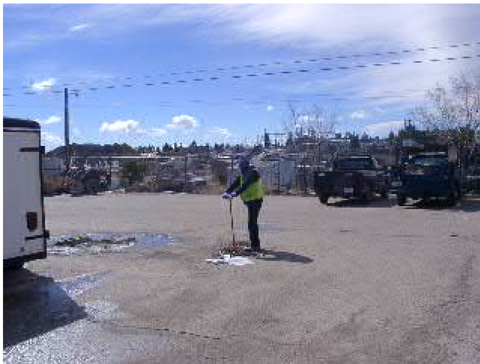
Figure B-4 Sampling using hand auger at SWMU 61-002 location 61-24310 (view looking south toward Los Alamos County Landfill)
