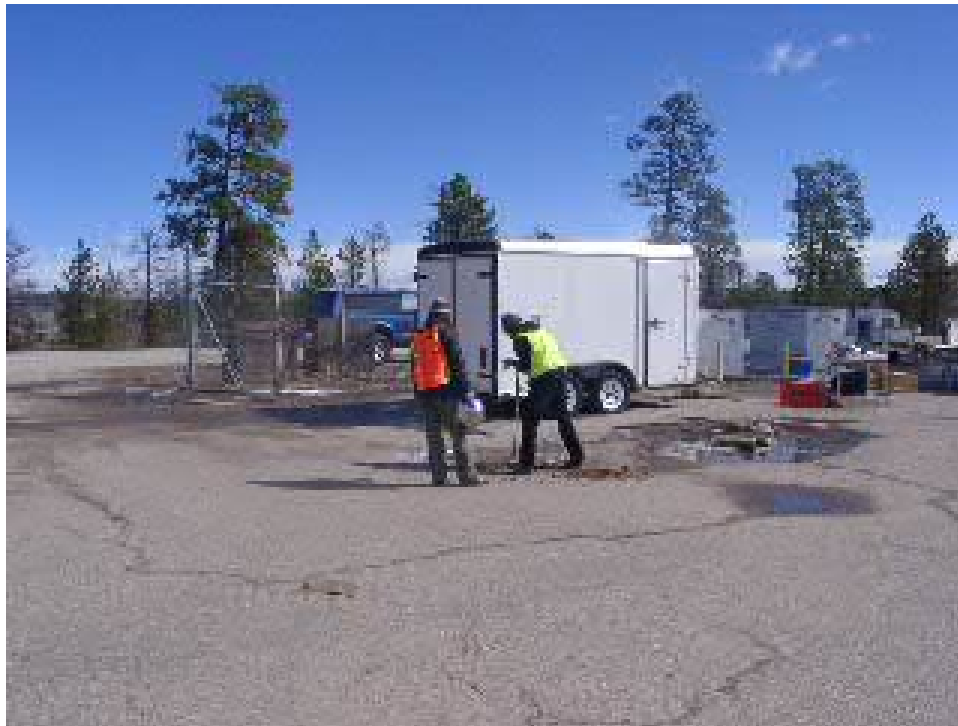
Figure B-3 Sampling using hand auger at SWMU 61-002 (location 61-24310; view looking north and West Jemez Road)
