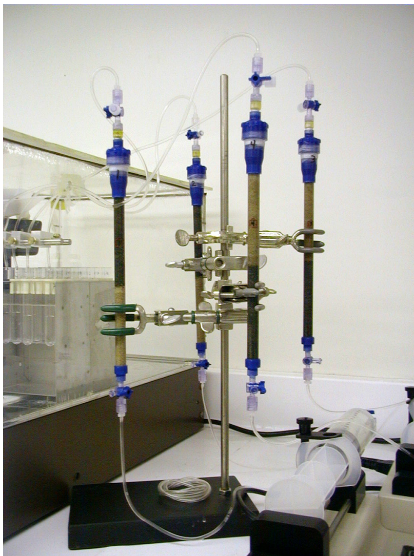
Figure B1-7 Photograph of columns 1–4 from the first set of column experiments. Note that columns are packed with two different reactive media in each.
