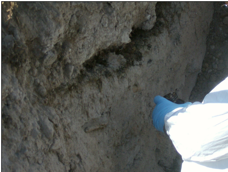
Photo 2 Close-up view of the 2-in.-thick layer of blackened debris found during excavation, May 2007
