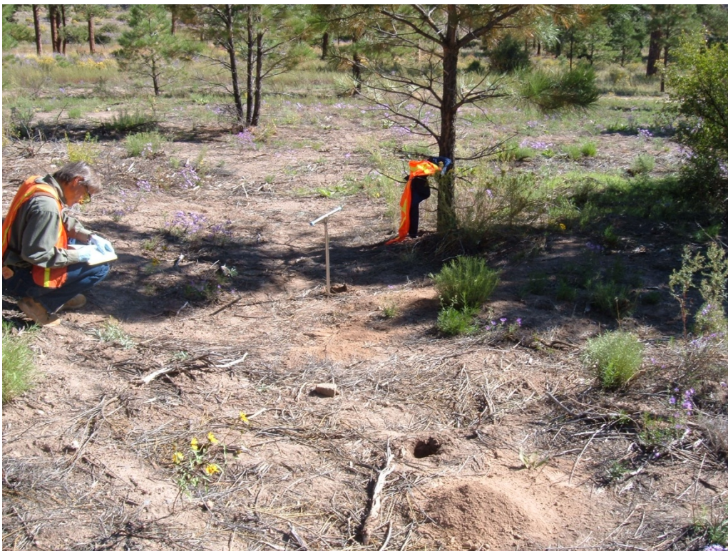
Figure D-20 Five auger holes and three test pits dug to investigate the subsurface (up to 3 ft bgs) in the SWMU 10-006 investigation area
