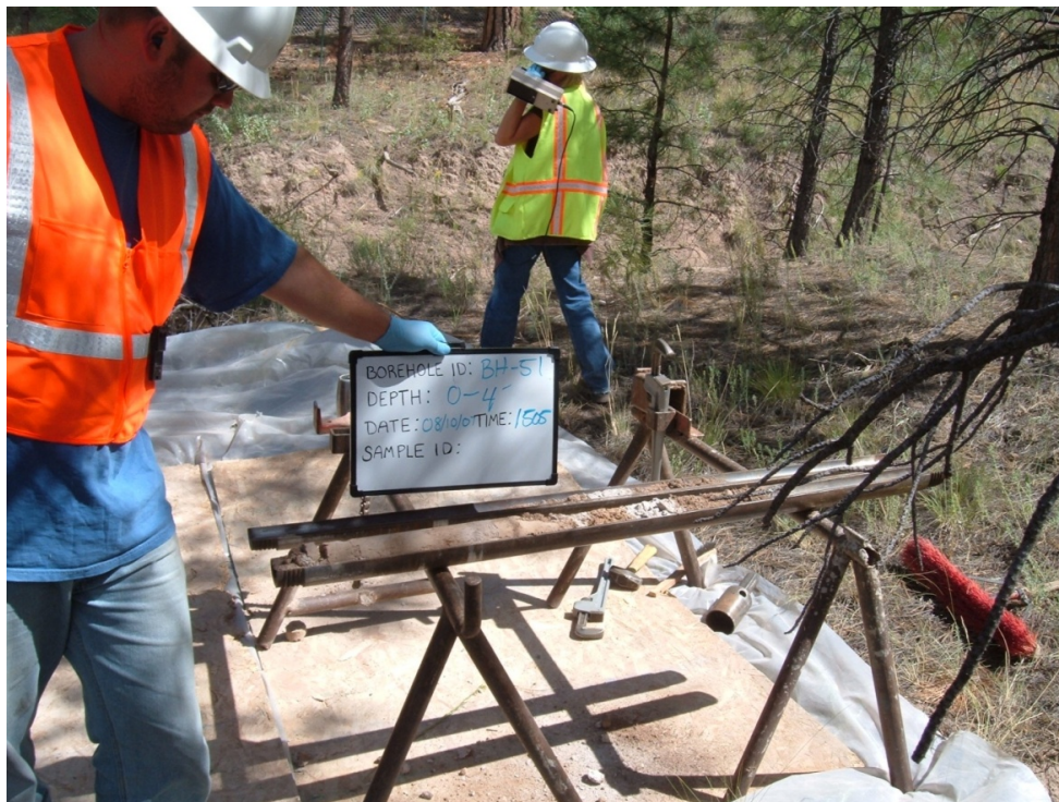
Figure D-6 BH-51 (10-601149), 0–4 ft below ground surface (bgs), Quaternary alluvium
