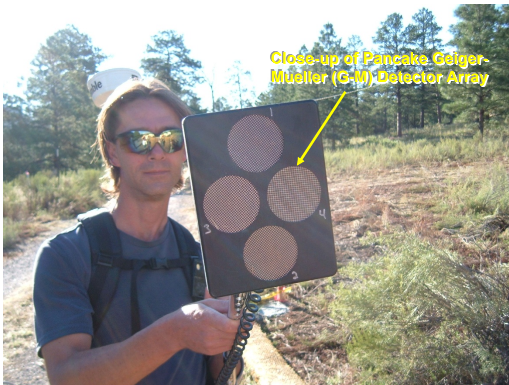
Figure D-4 Closeup of G-M detector array used to collected radiological survey data
