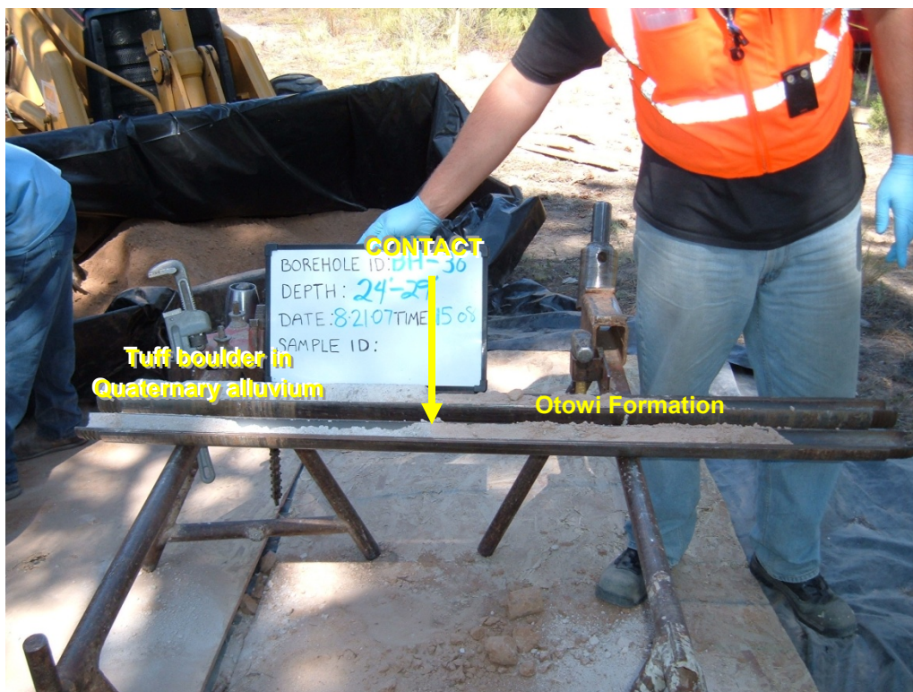
Figure D-10 Large welded tuff boulder in quaternary alluvium and contact with Otowi Member of the Bandelier Tuff at BH-36 (10-601175) from 24 to 29 ft bgs
