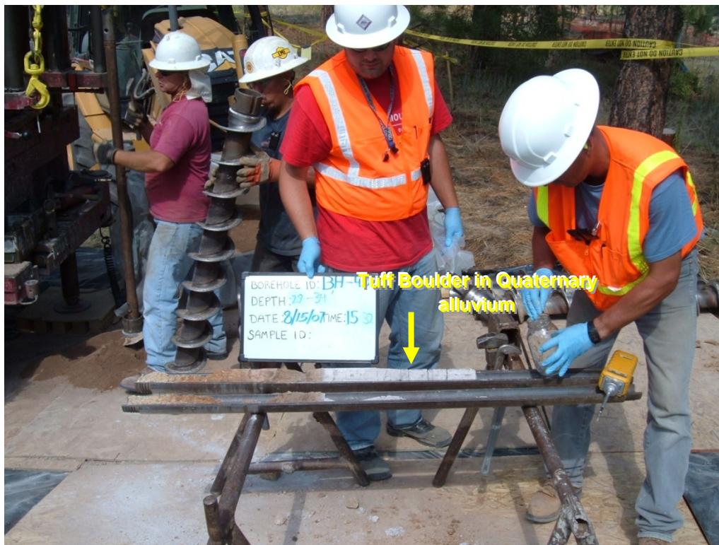
Figure D-9 Large welded tuff boulder in quaternary alluvium deposits at BH-40 (10-601179)
