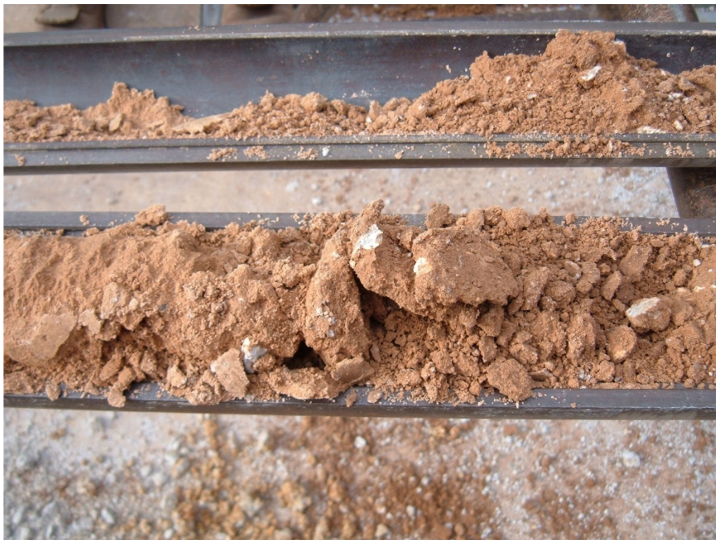
Figure D-15 Closeup of palesol above Cerros del Rio basalt
