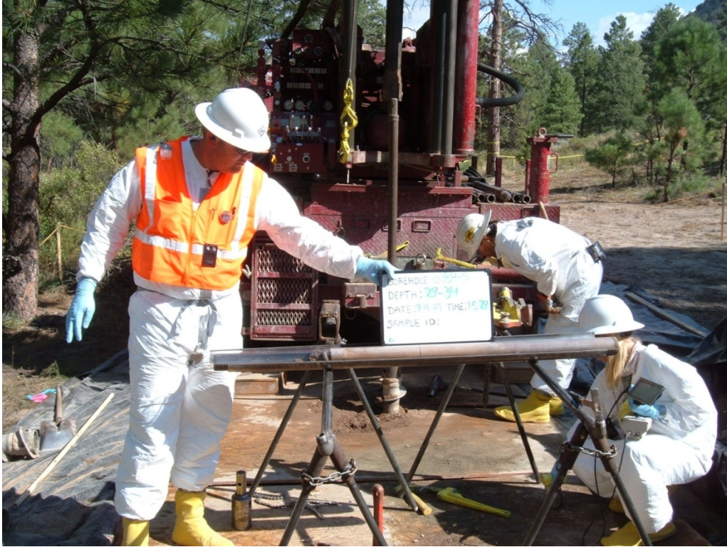
Figure D-16 Using lexan liner to collect geotechnical samples and to prevent radiological contamination of the core barrel
