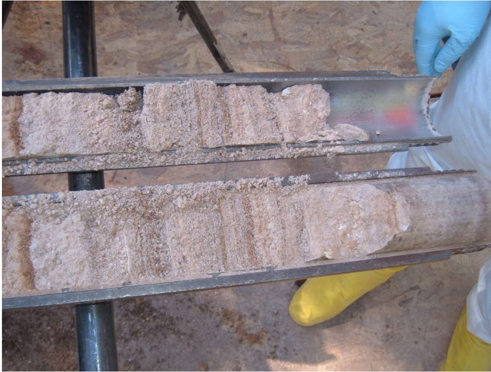
Figure D-8 Laminated to bedded sand, silt, clay, and pumice fragments typical of Quaternary alluvium deposits in Bayo Canyon
