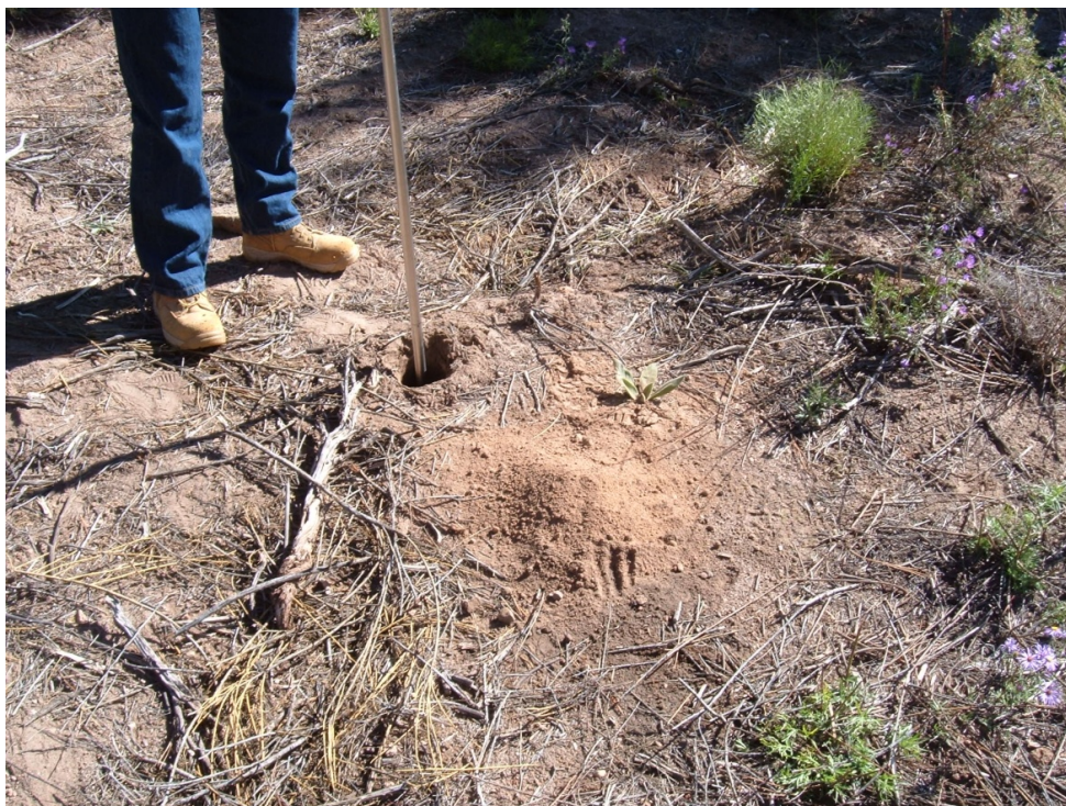
Figure D-18 Auger holes dug to investigate the subsurface (up to 3 ft bgs) in the investigation area
