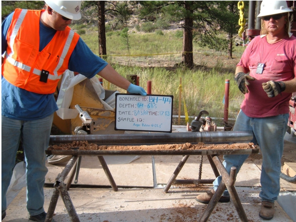
Figure D-14 BH-44 (10-601192), 64–68.5 ft bgs, borehole refusal in palesol above Cerros del Rio basalt
