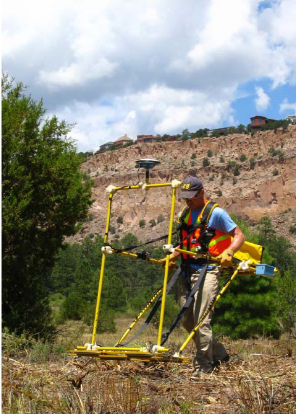
Figure D-2 TM-5emu geophysical survey instrument used to survey shrapnel distribution at Consolidated Unit 10-001(a)-99. View to north of Otowi Mesa in background.
