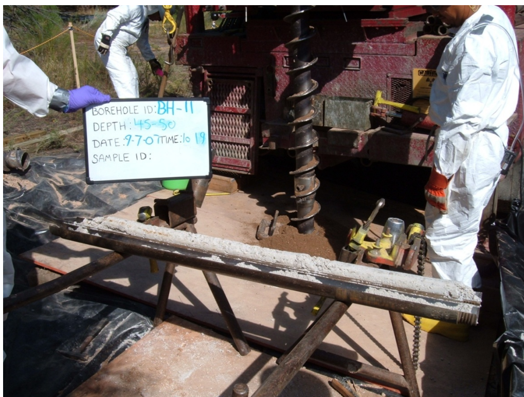
Figure D-11 Guaje Pumice Bed deposit at 45-50 ft bgs in BH-11 (10-601244)
