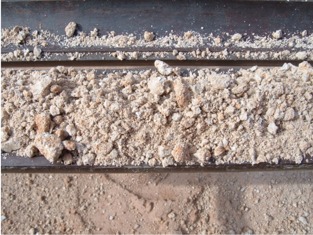
Figure D-12 Closeup of Guaje Pumice Bed deposit at 45–50 ft bgs in BH-11 (10-601244)
