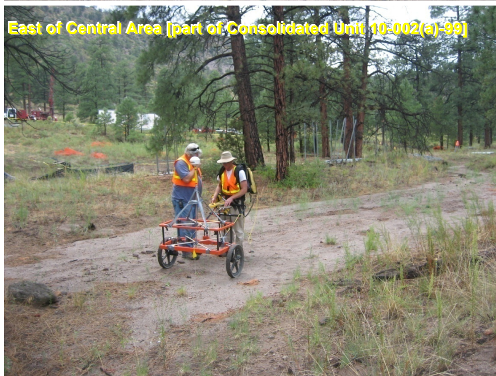
Figure D-1 EM31 and EM61 geophysical survey instruments coupled with a global positioning system (GPS) used to identify subsurface anomalies at various locations in Bayo Canyon
