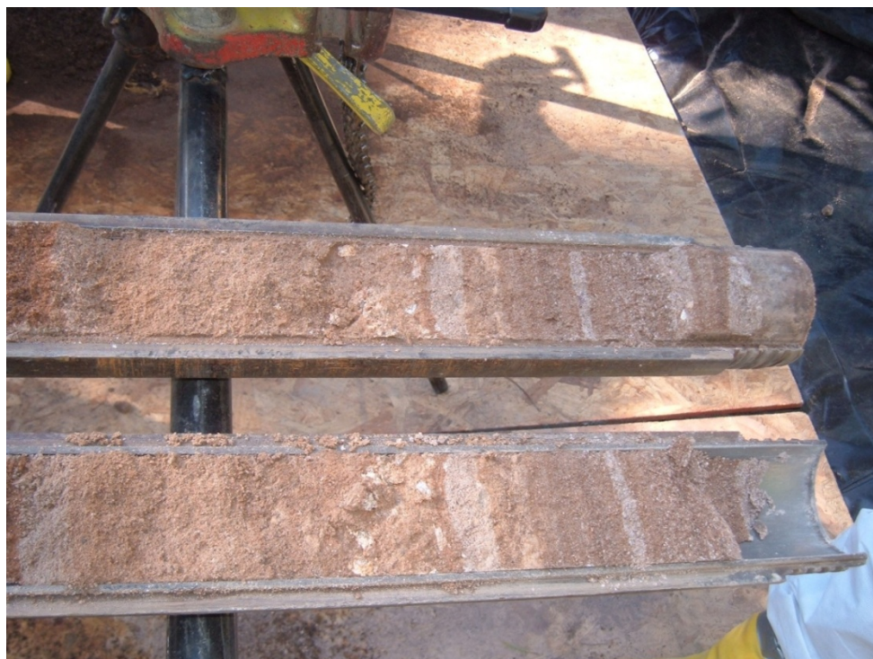
Figure D-7 Laminated to bedded sand, silt, clay, and pumice fragments typical of Quaternary alluvium deposits in Bayo Canyon
