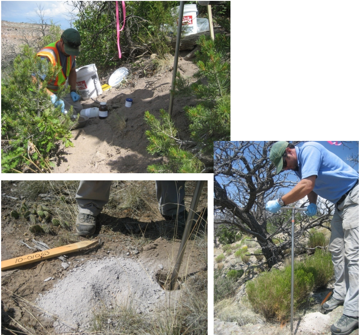
Figure D-5 Examples of surface and shallow subsurface sampling at various locations in Bayo Canyon. Surface samples were collected from soil, quaternary alluvium, and welded tuff (Qbt 3).
