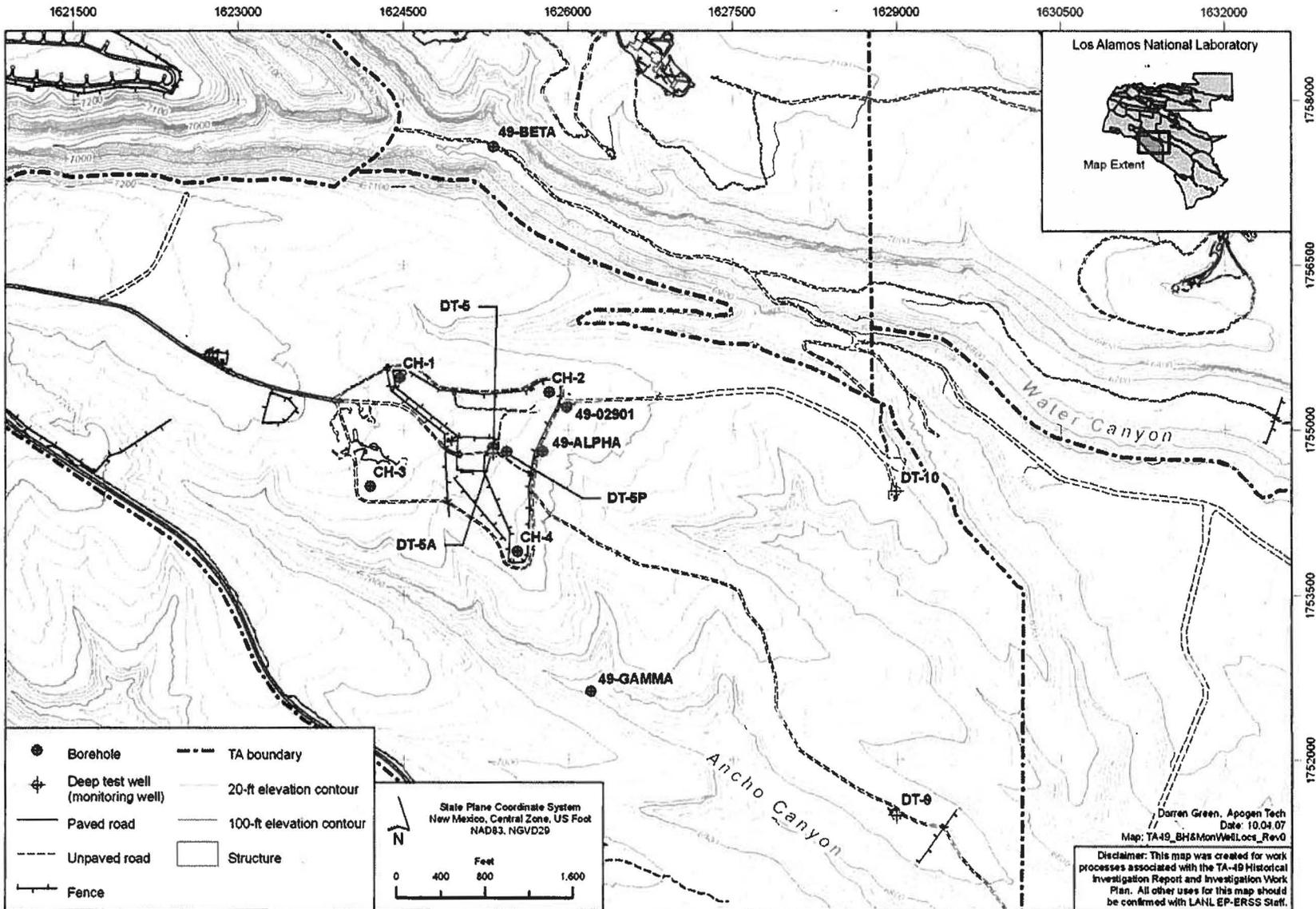
Figure 3.3-1 Locations of deep test wells and select boreholes at TA-49
