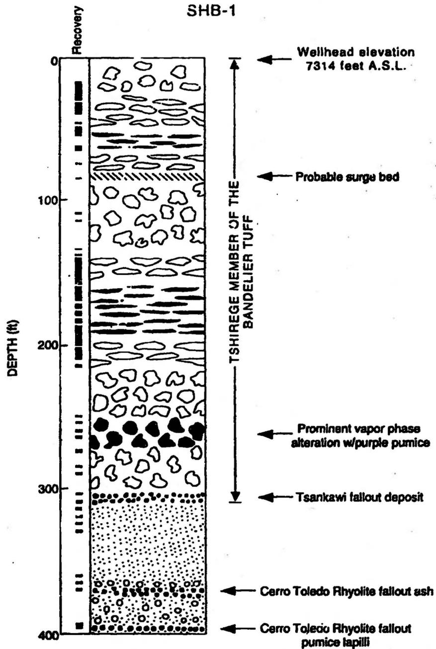
**Figure 6a:** Graphic lithology log for core hole SHB-1. Log is continued on next page. Black marks in recovery column indicate where core was recovered. See Table II for explanation of symbols.
