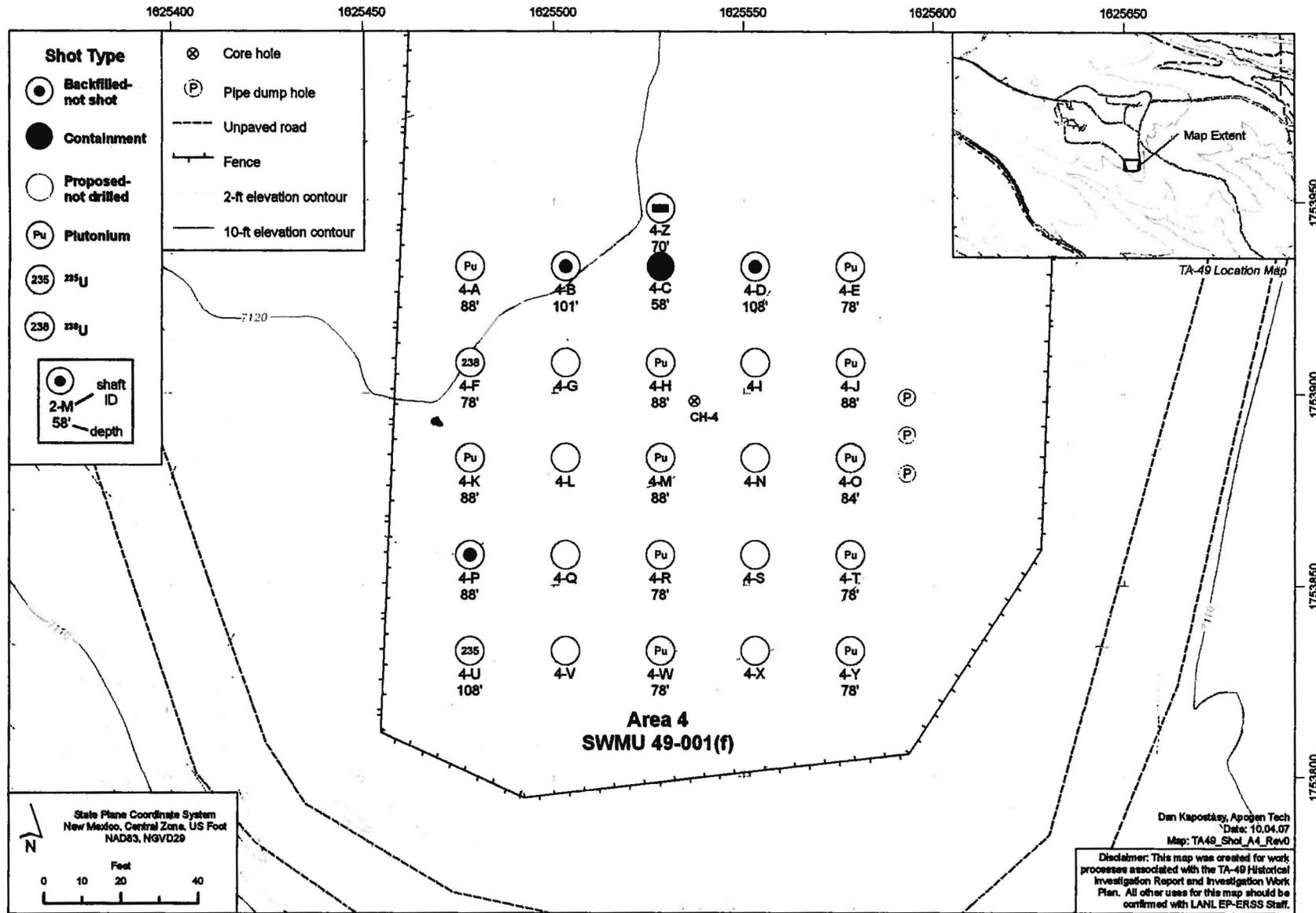
Figure 1.0-6 Area 4 experimental shaft details
