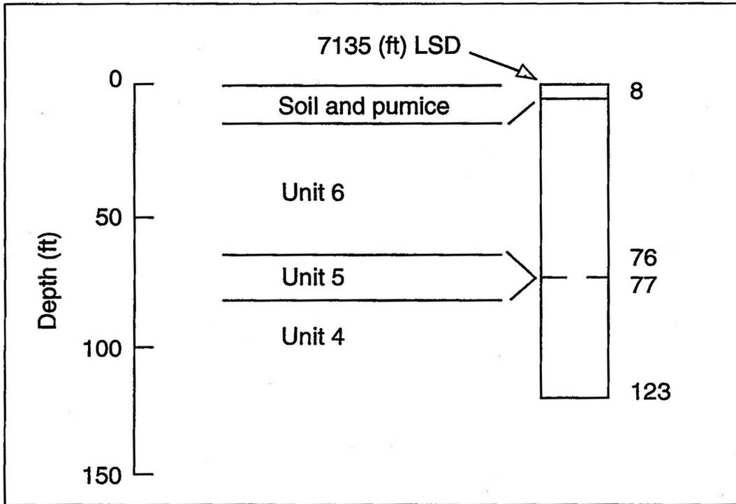
**Fig. IX-P.** Geologic log of Area 2 Test Hole 1, completed May 1980, dry (Purtymun 1994).
