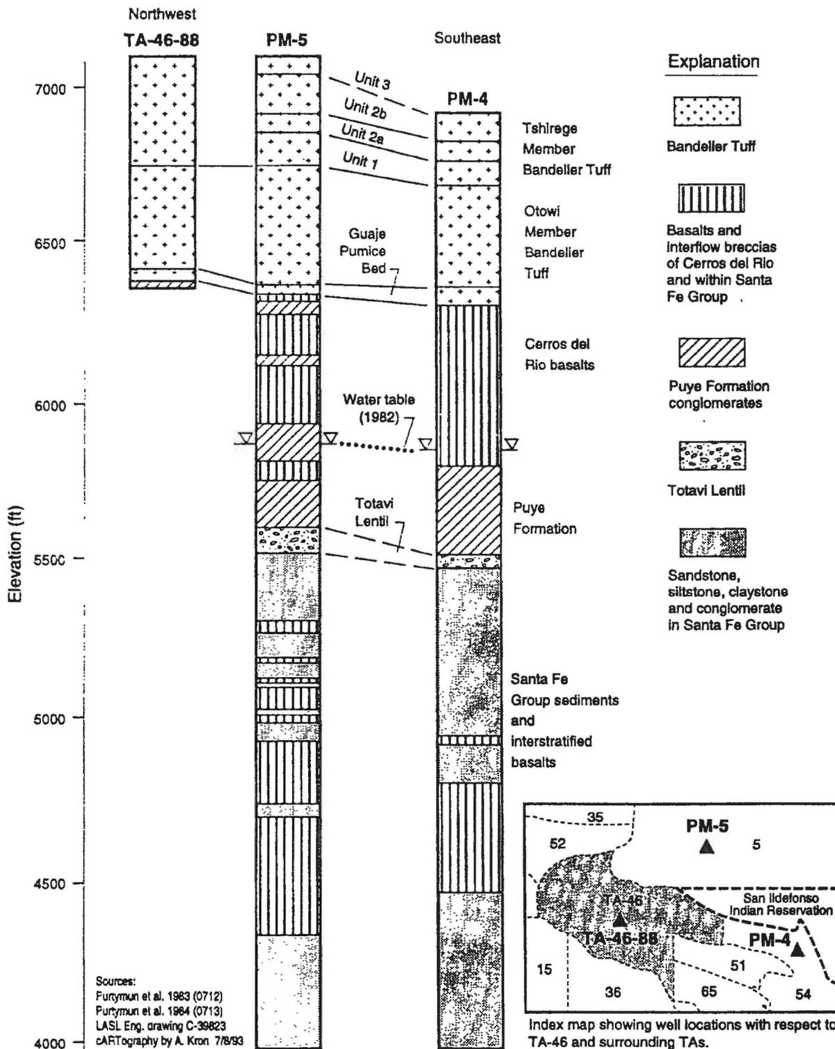
Fig. 3-4. Lithologic logs for borings near TA-46.
