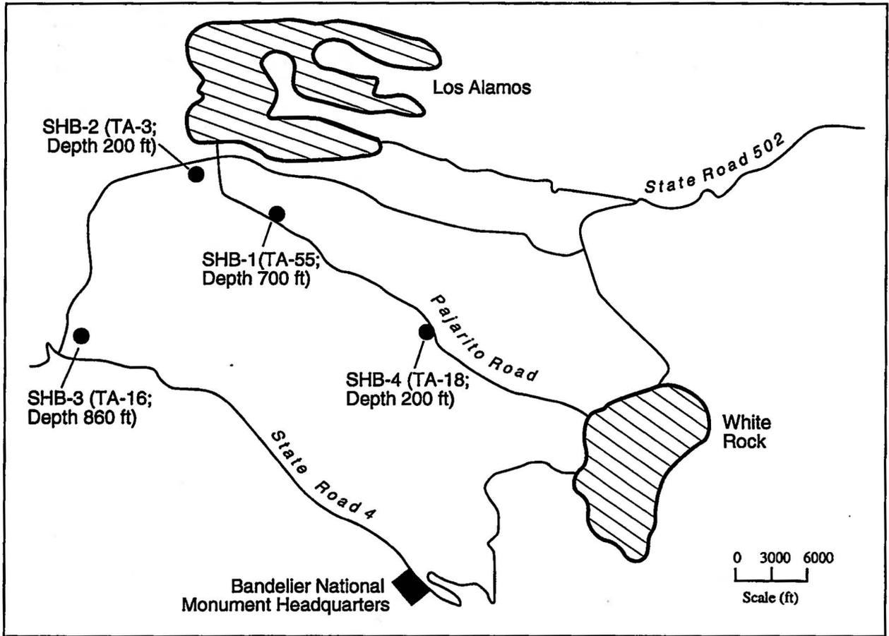
**Fig. XXIII-B.** Locations of test holes for seismic investigation.
