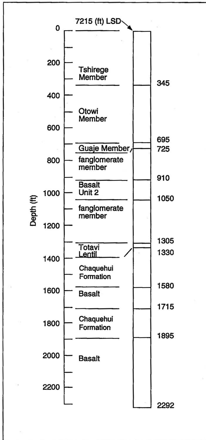
**Fig. XVII-K.** Geologic log of test hole Sigma Mesa, drilled July–November 1979, water level about 1330 ft (data from unpublished log by Carolyn Potzich modified by Purtymun; see text and Table XVII-B).
