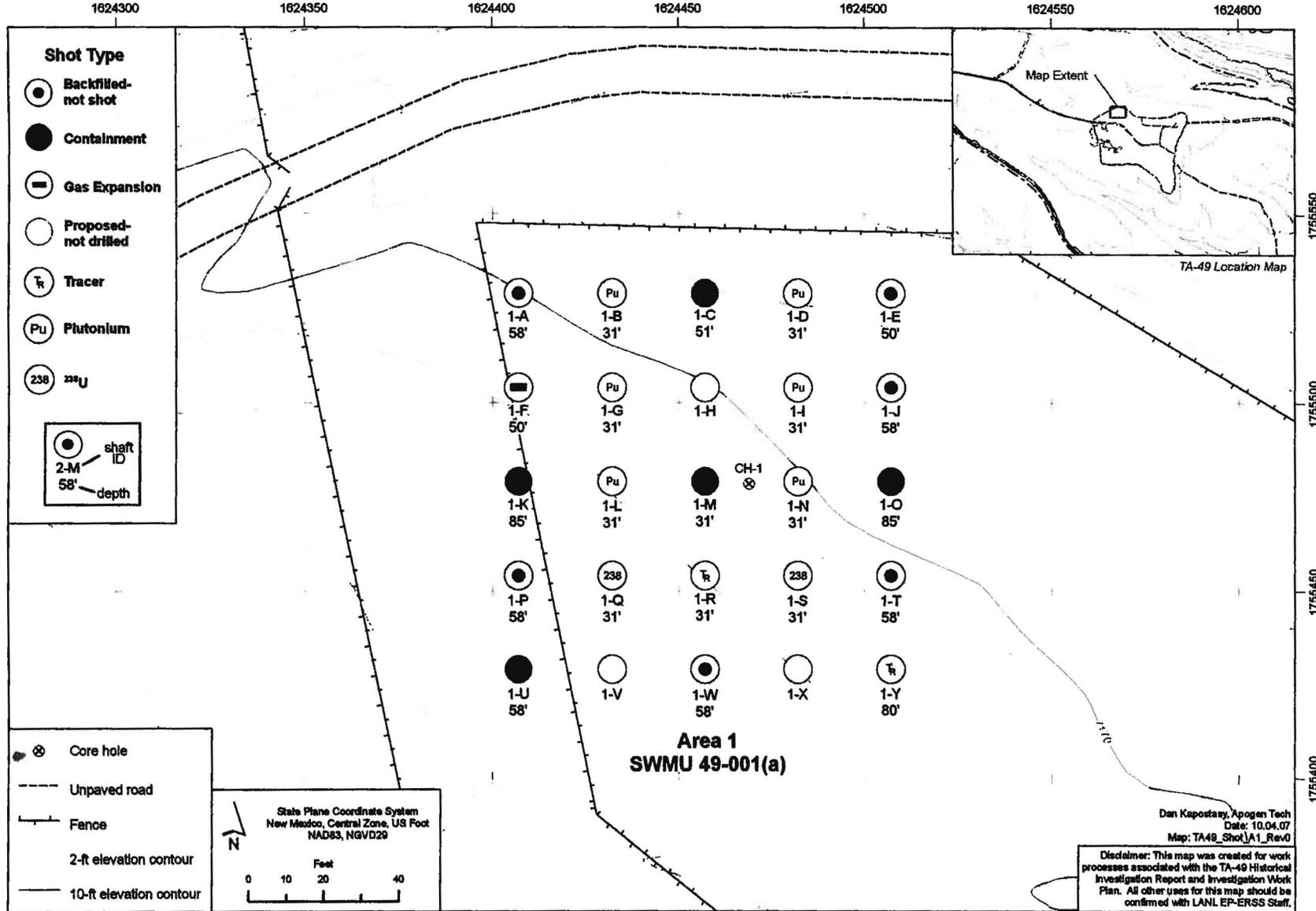
Figure 1.0-3 Area 1 experimental shaft details
