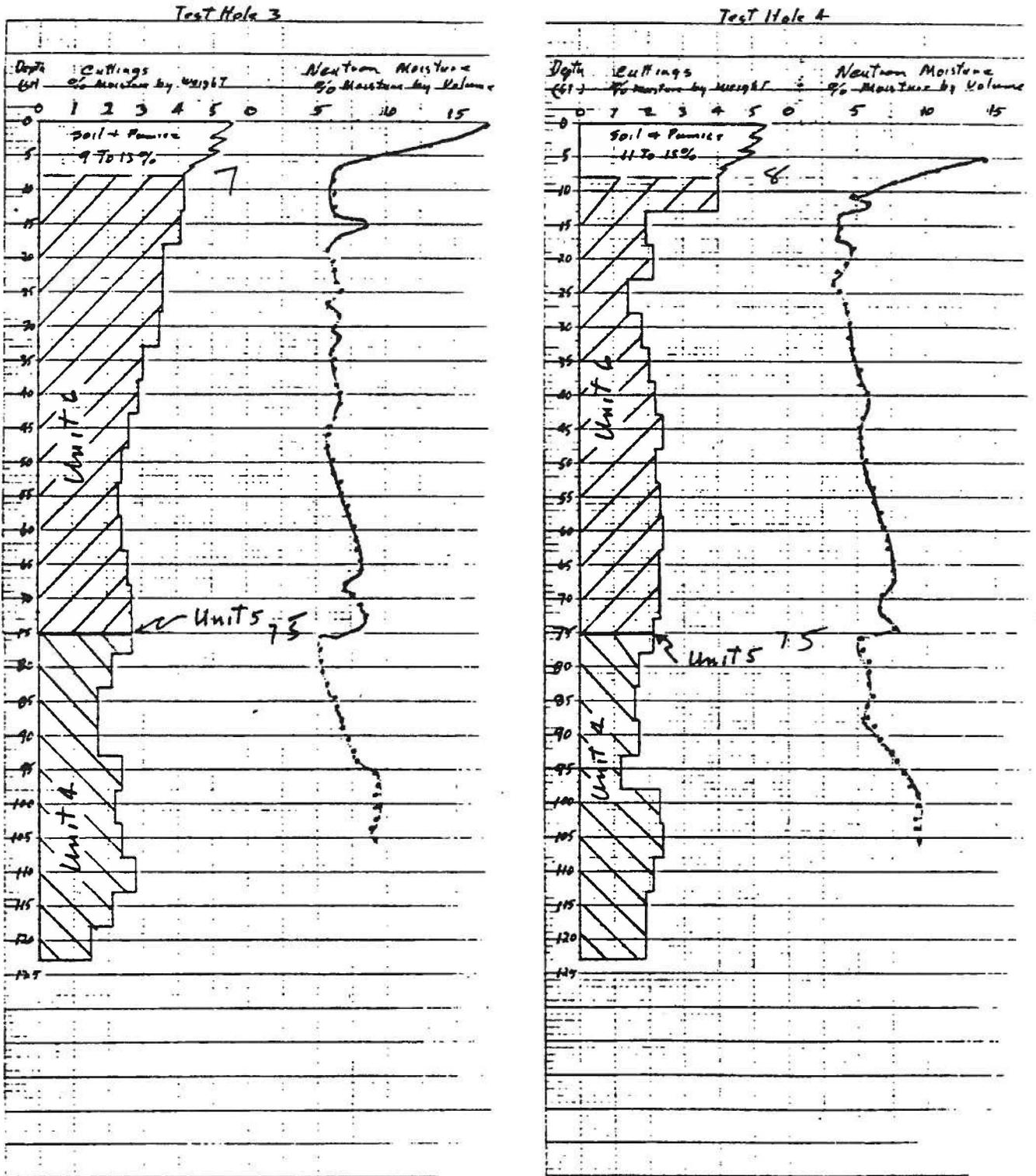
Fig. 3. Geologic and neutron logs of Test Holes TH-3 and TH-4.
