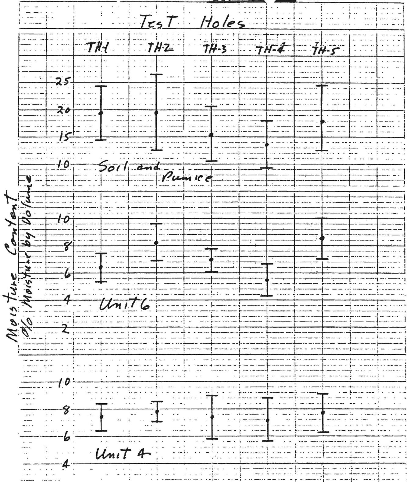
Fig. 5. Average moisture content of pumice and soil and tuff of Unit 4 and 6 in test holes.
