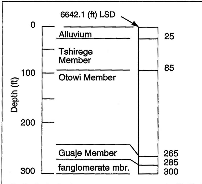
Fig. XVII-G. Geologic log of test hole TH-6, completed March 1950, dry (Griggs 1955).
