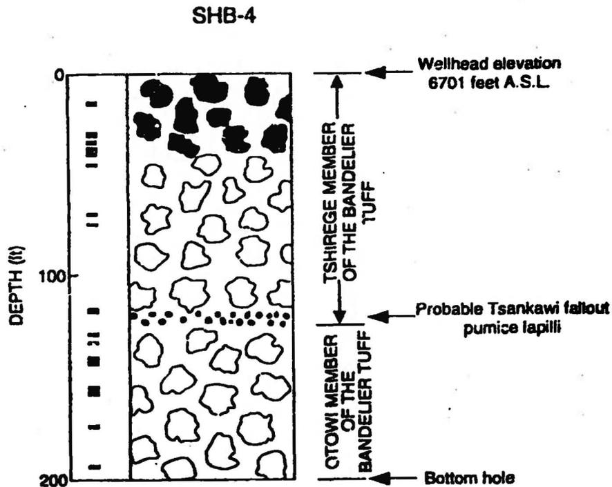
Figure 9: Graphic lithology log for core hole SHB-4. See Table II and Figure 6 for explanation of symbols.
