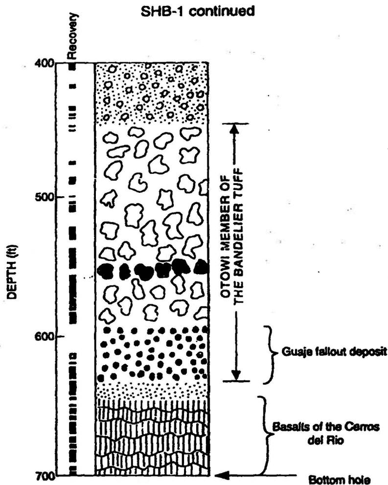
Figure 6b: Graphic lithology log for core hole SHB-1. Black marks in recovery column indicate where core was recovered. See Table II for explanation of symbols.
