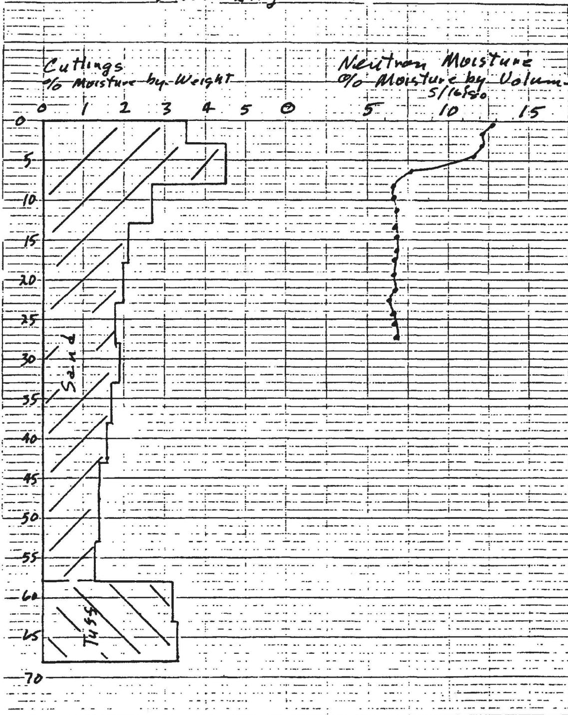
Fig. 8. Geologic and neutron logs of Shaft 2A-Y.
