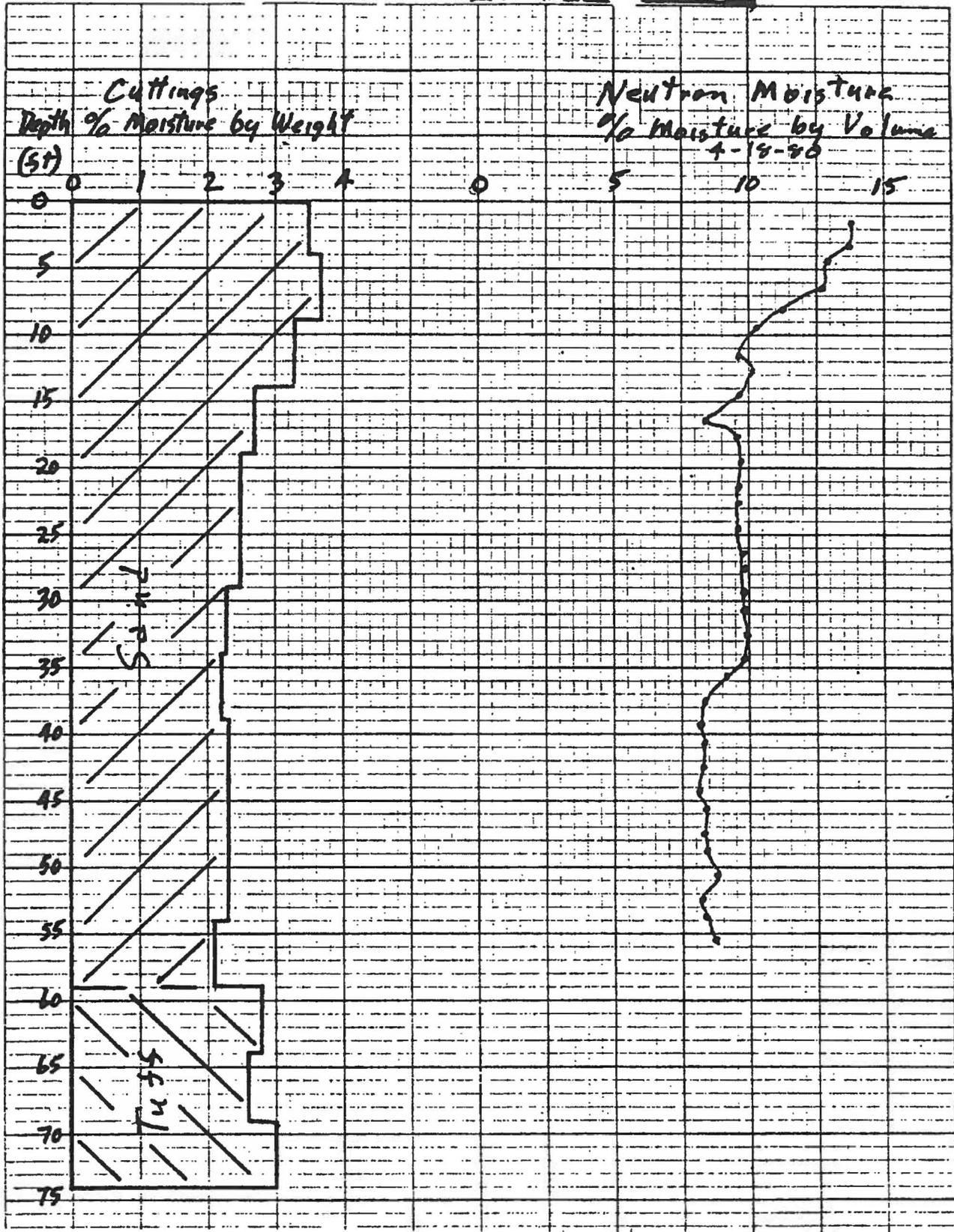
Fig. 6. Geologic and neutron logs of Shaft 2A-0.
