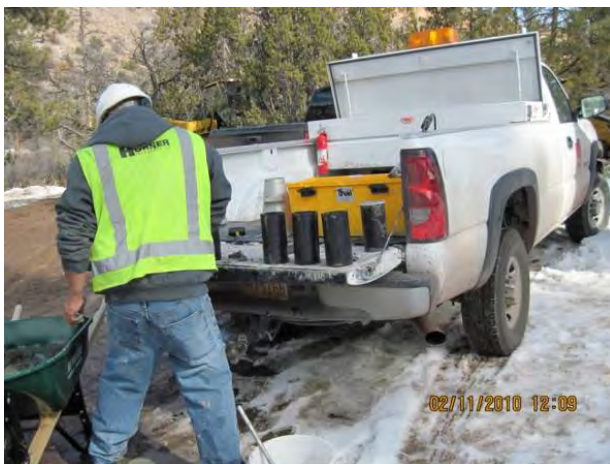
Photo 5 Flume concrete cylinder samples for lab testing
