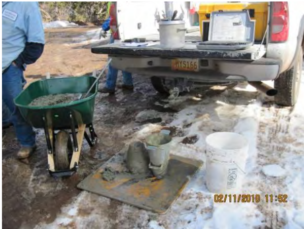
Photo 3 Flume concrete slump test
