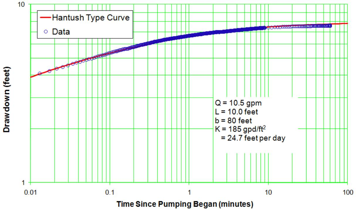
Figure C-8.2-3 Well R-53 screen 1 trial 2 drawdown—Hantush solution for anisotropy of 0.001
