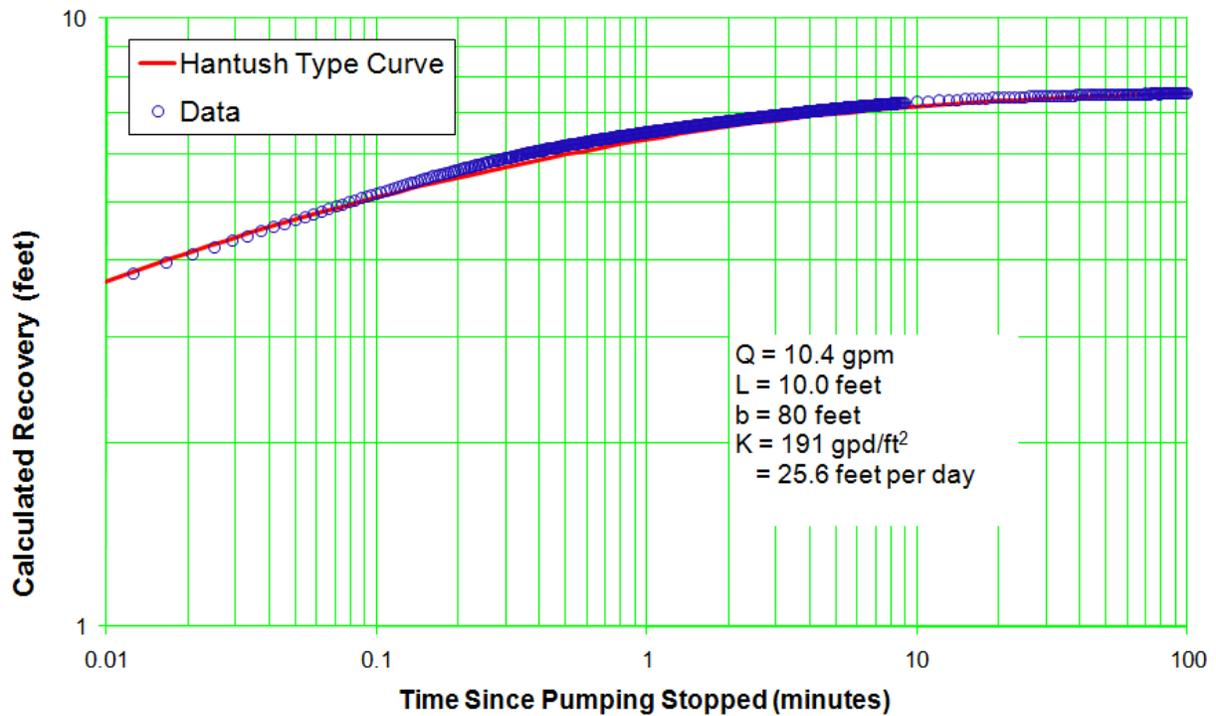
Figure C-8.2-6 Well R-53 screen 1 trial 2 recovery—Hantush solution for anisotropy of 0.001
