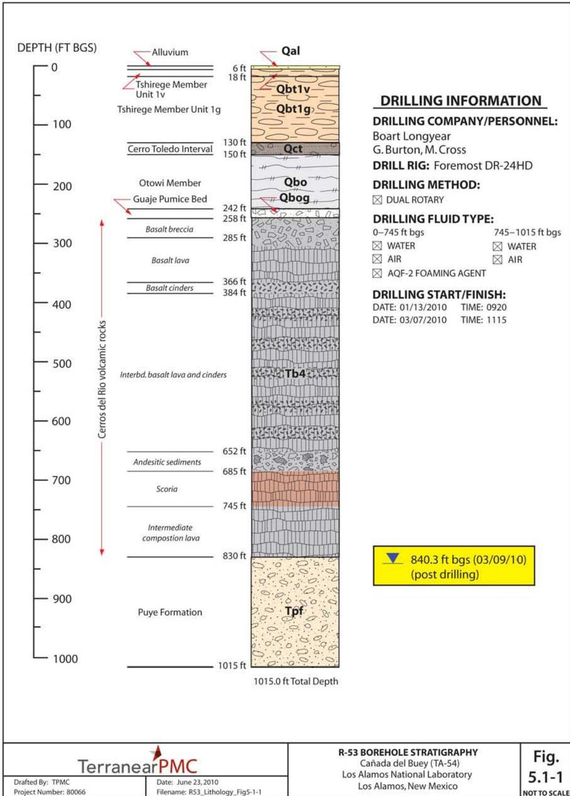
Figure 5.1-1 Monitoring well R-53 borehole stratigraphy
