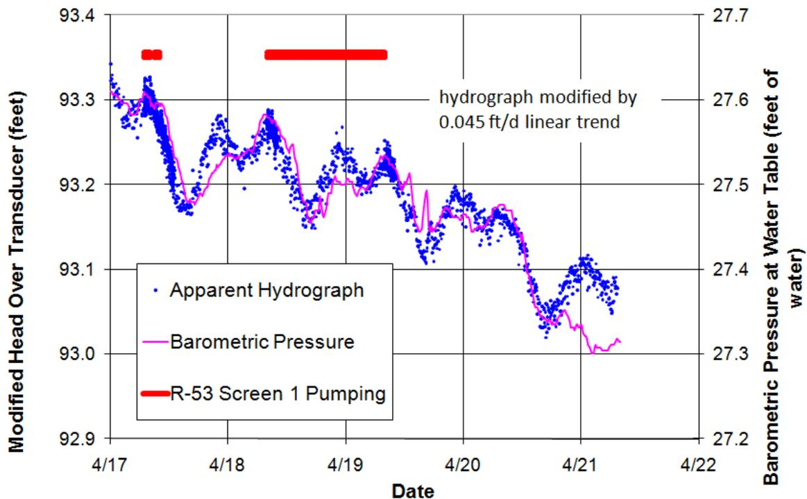
Figure C-7.0-3 Well R-53 screen 2 modified apparent hydrograph
