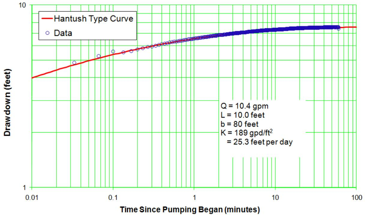
Figure C-8.1-5 Well R-53 screen 1 trial 1 drawdown—Hantush solution for anisotropy of 0.001
