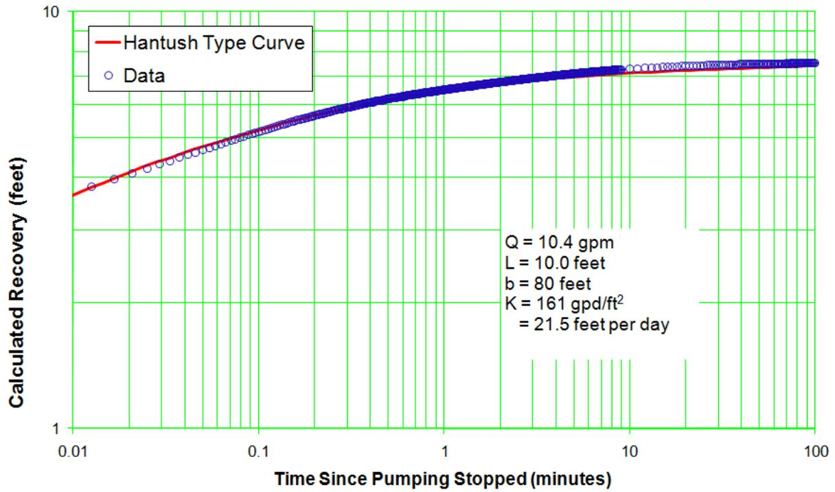
Figure C-8.2-5 Well R-53 screen 1 trial 2 recovery—Hantush solution for anisotropy of 0.01
