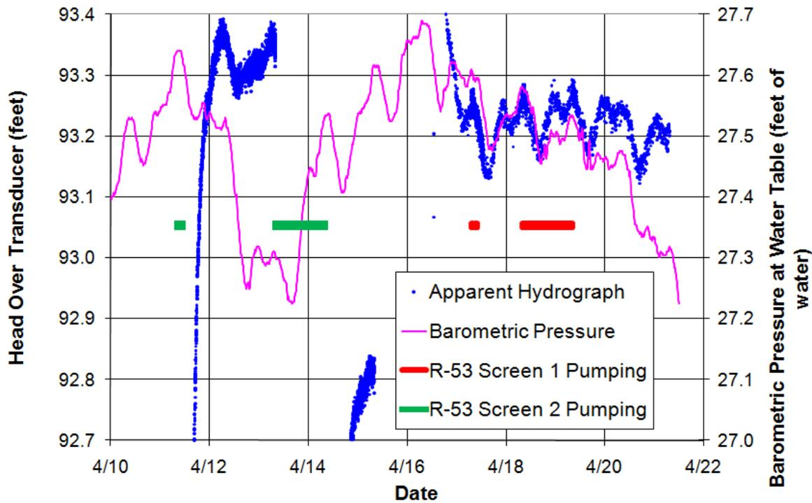
Figure C-7.0-2 Well R-53 screen 2 apparent hydrograph
