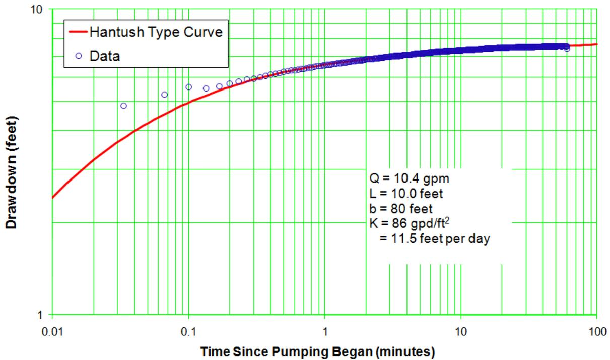
Figure C-8.1-2 Well R-53 screen 1 trial 1 drawdown—Hantush solution for anisotropy of 1.0
