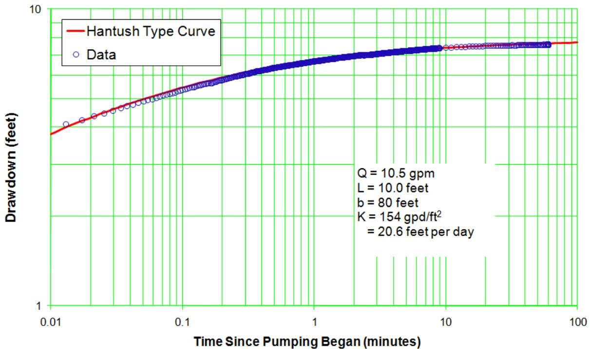
Figure C-8.2-2 Well R-53 screen 1 trial 2 drawdown—Hantush solution for anisotropy of 0.01
