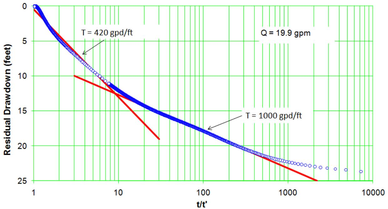
Figure C-9.2-2 Well R-53 screen 2 trial 2 recovery
