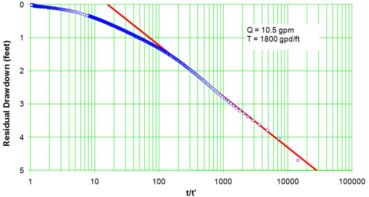
Figure C-8.2-4 Well R-53 screen 1 trial 2 recovery
