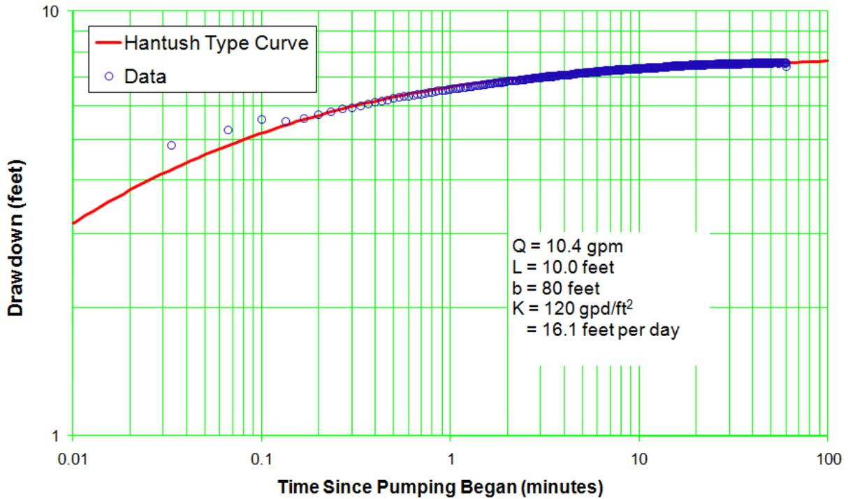
Figure C-8.1-3 Well R-53 screen 1 trial 1 drawdown—Hantush solution for anisotropy of 0.1
