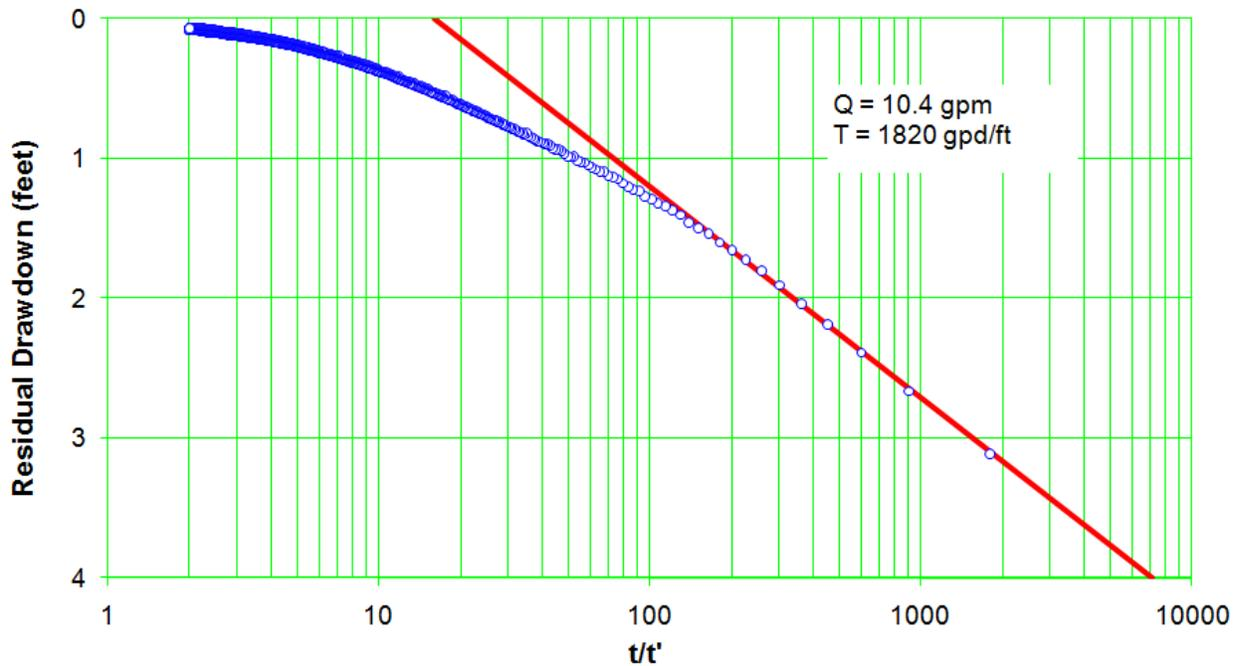
Figure C-8.1-6 Well R-53 screen 1 trial 1 recovery
