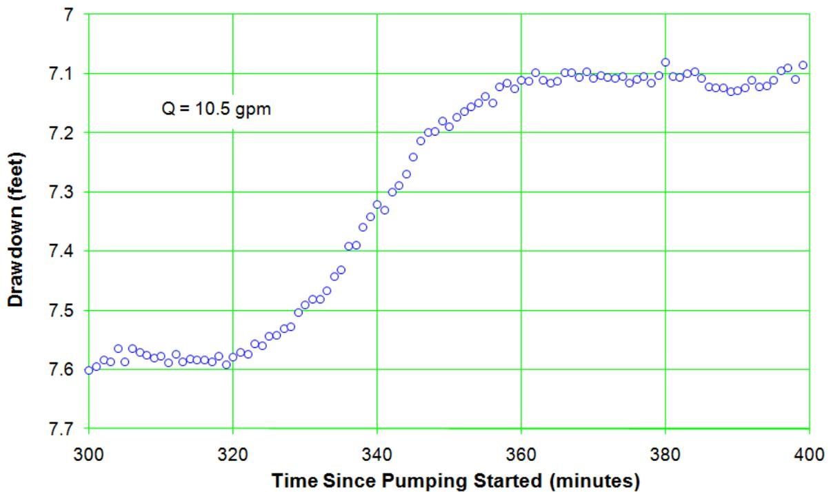
Figure C-8.3-2 Well R-53 screen 1 drawdown—expanded scale
