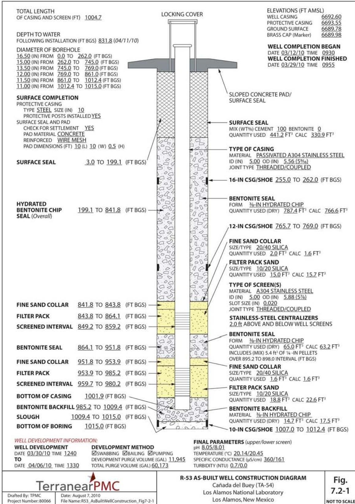
Figure 7.2-1 Monitoring well R-53 as-built well construction diagram
