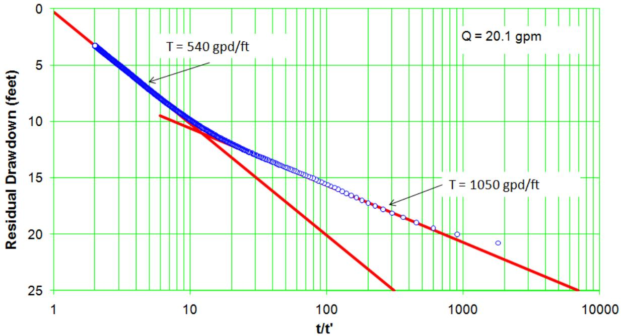
Figure C-9.1-2 Well R-53 screen 2 trial 1 recovery
