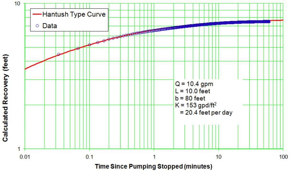
Figure C-8.1-7 Well R-53 screen 1 trial 1 recovery—Hantush solution for anisotropy of 0.01
