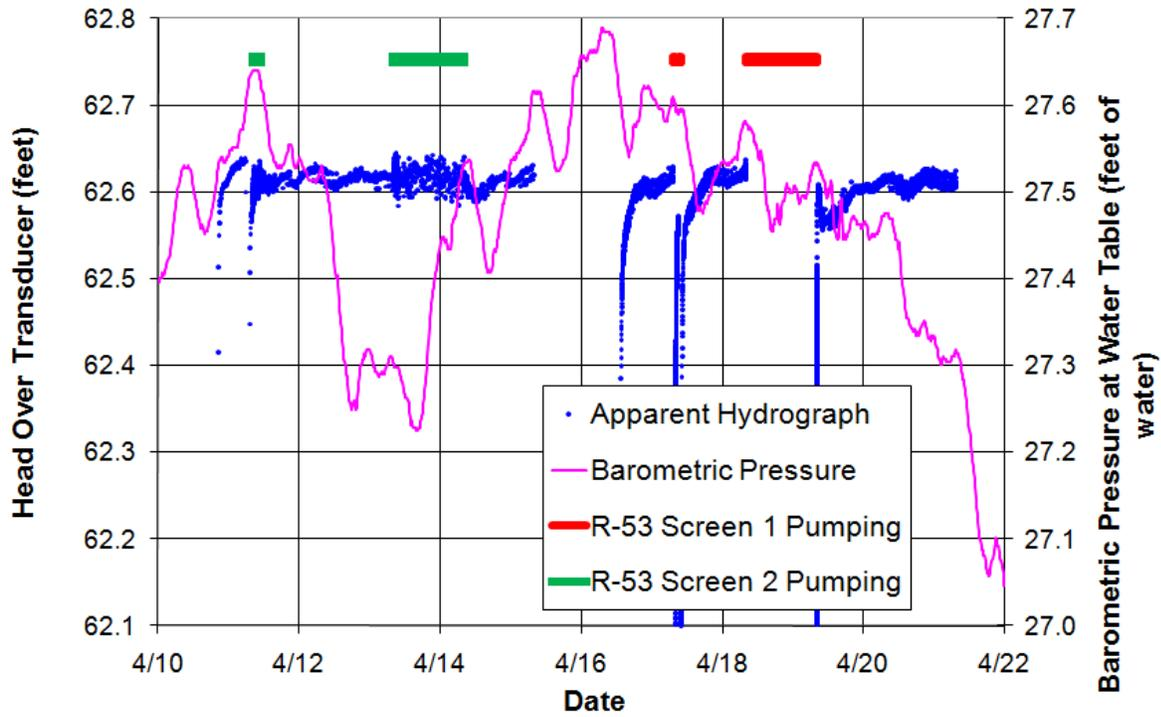
Figure C-7.0-1 Well R-53 screen 1 apparent hydrograph
