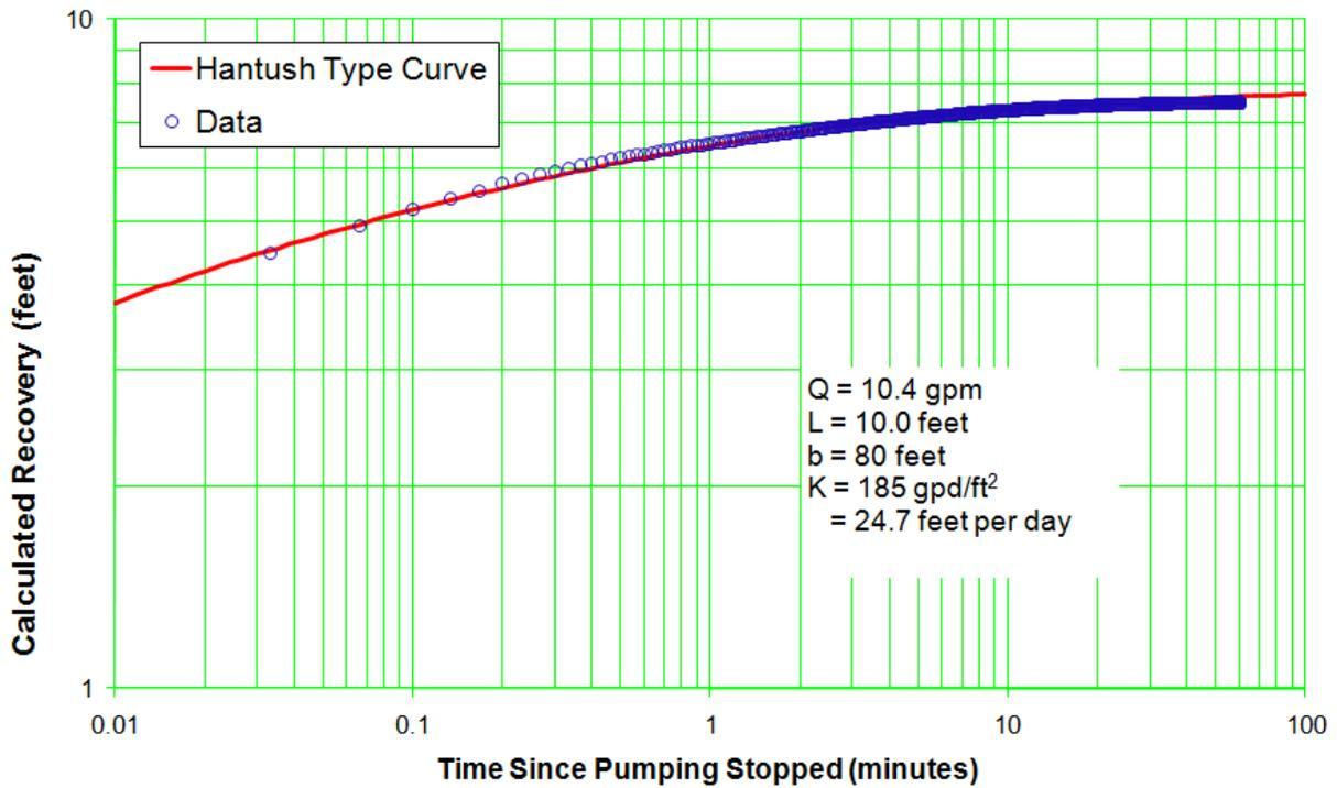
Figure C-8.1-8 Well R-53 screen 1 trial 1 recovery—Hantush solution for anisotropy of 0.001
