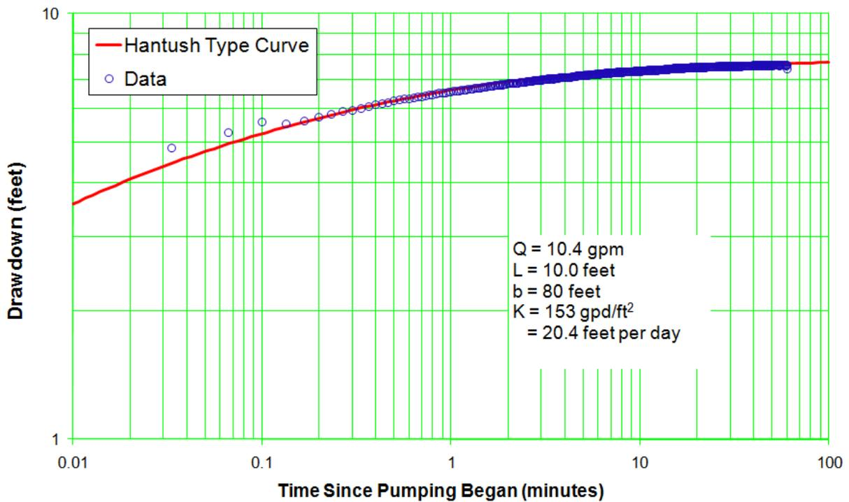
Figure C-8.1-4 Well R-53 screen 1 trial 1 drawdown—Hantush solution for anisotropy of 0.01
