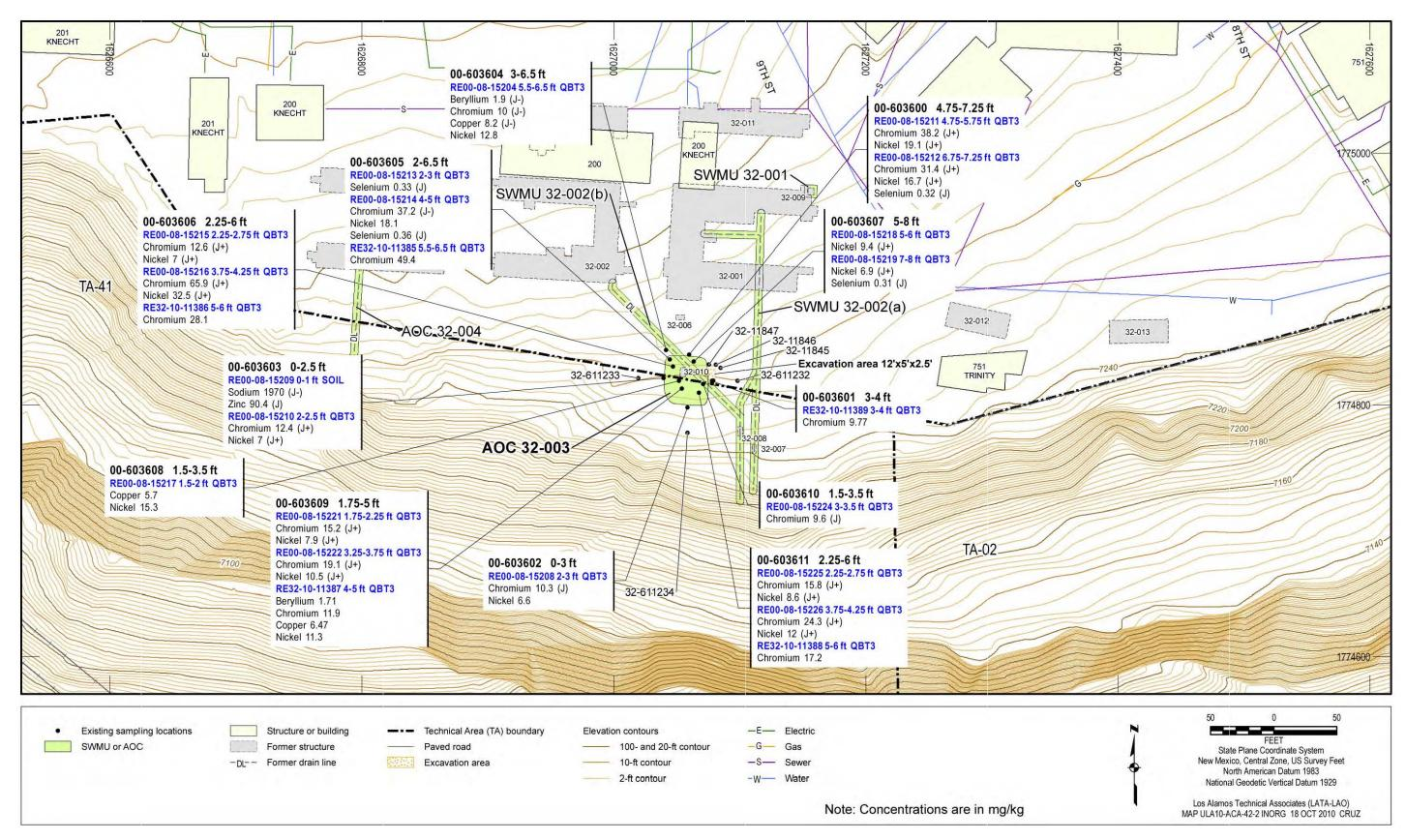
Figure 4.3-2 Inorganic COPCs detected or detected above BVs at AOC 32-003
