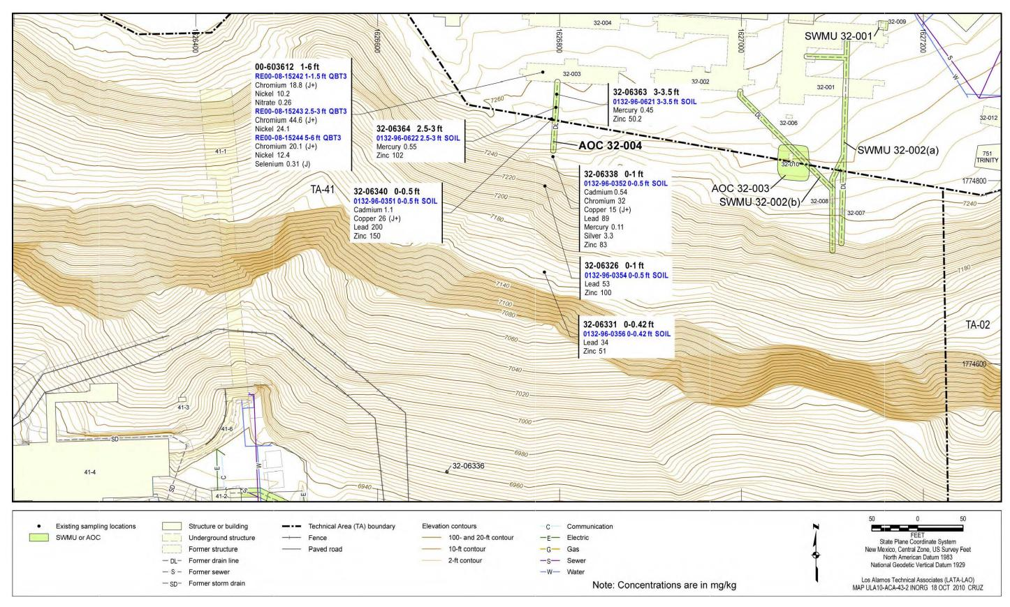
Figure 4.4-2 Inorganic COPCs detected or detected above BVs at AOC 32-004
