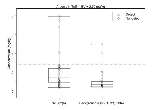
Figure E-1 Site concentrations of arsenic in tuff at SWMU 32-002(b) compared to background
