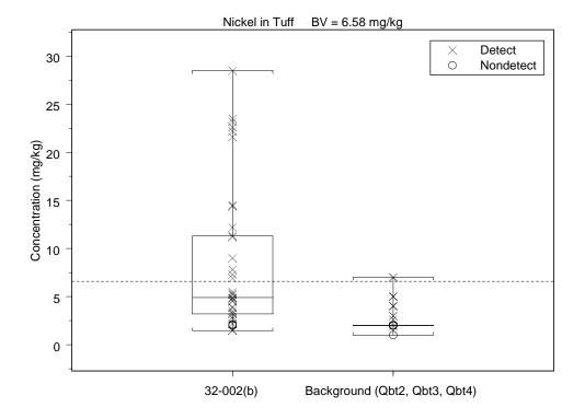
Figure E-7 Site concentrations of nickel in tuff at SWMU 32-002(b) compared to background
