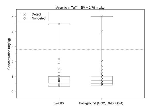
Figure E-14 Site concentrations of arsenic in tuff at AOC 32-003 compared to background
