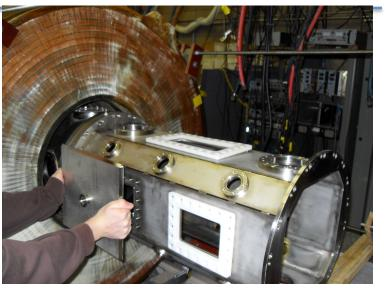
3d positioning ports allow unique diagnostic access.
