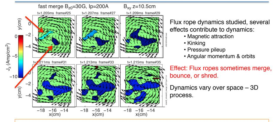
x-y cutplane data: two flux ropes initially fast merge, then "shred" into several smaller flux ropes.
