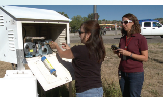
Environmental scientists collect ambient air samples that will be sent to an external analytical lab for analysis.
