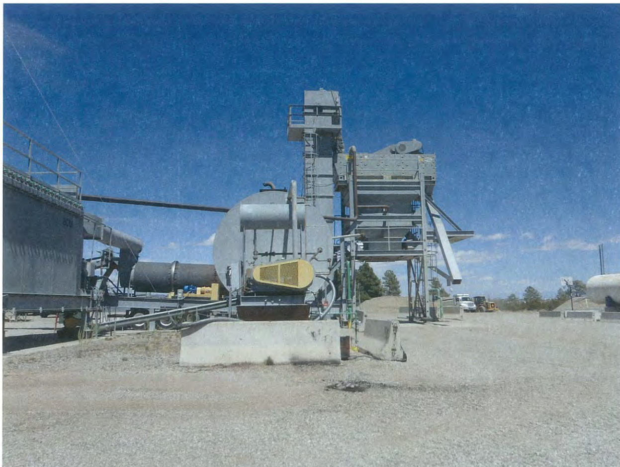
Photograph 2. Close up view of two tanks 115 gal. tank (forefront) and 15,000 gal. asphalt cement tank.
