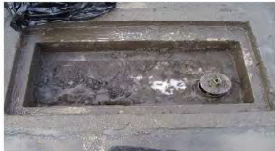
The second set of dirt filters are removed finally showing some clean filter on the bottom. The dirt had made it to the second set of dirt filters but did not impact the Barrier-Box.
