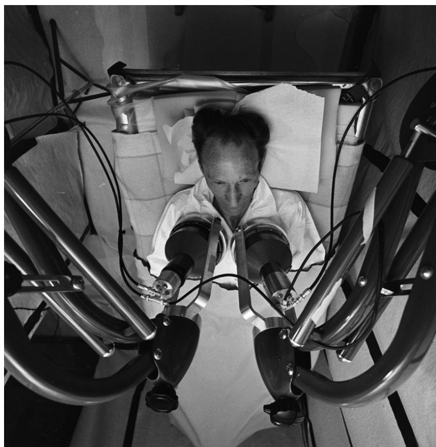
Figure 3-13. Plutonium lung counter in use, October 1, 1970 (LANL image, negative no. PUB-70222-7).
