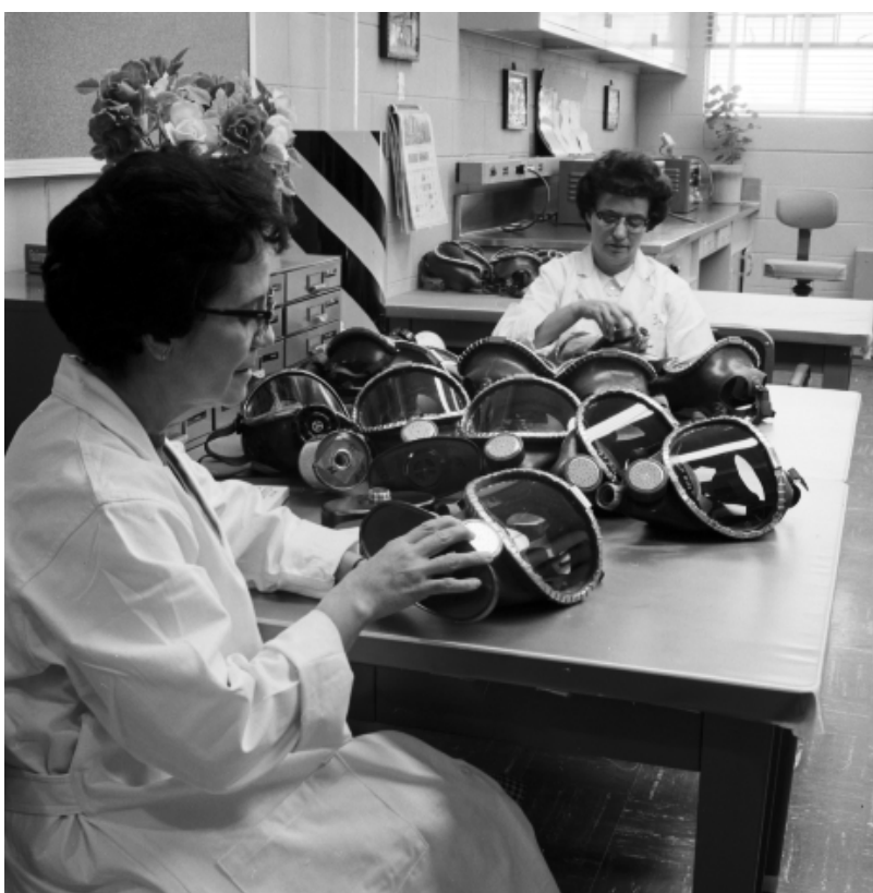
Figure 3-22. Respirator testing by women of the H-5 Group in HRL, November 1965 (LANL image, negative no. PUB-6150-11).
