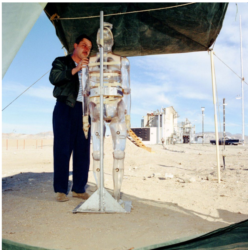
Figure 3-27. Payne S. Harris, H-4 alternate group leader and subsequently H-8 group leader, setting up Plastic Man named REMAB in advance of a Kiwi-A3 run, 1960 (LANL image, negative no. PUB60-0413-C).
