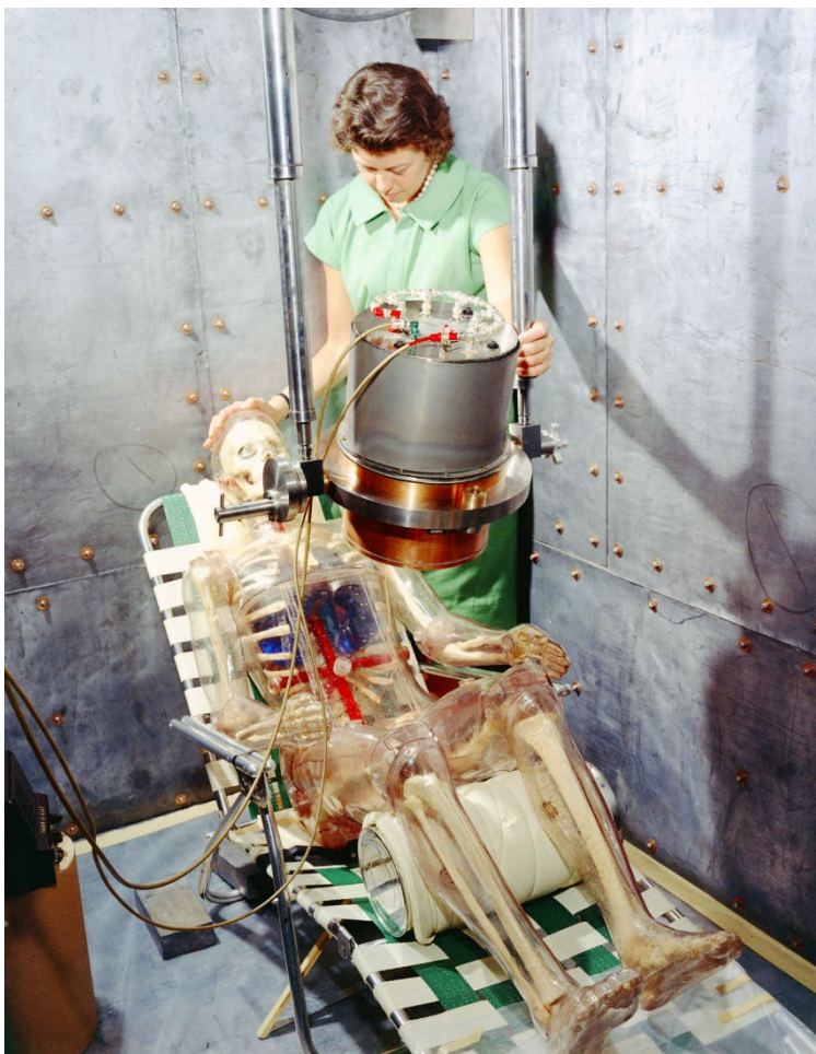
Figure 3-9. Plastic Man under crystal spectrometer, June 1959 (LANL image, negative no. CN59-222).
